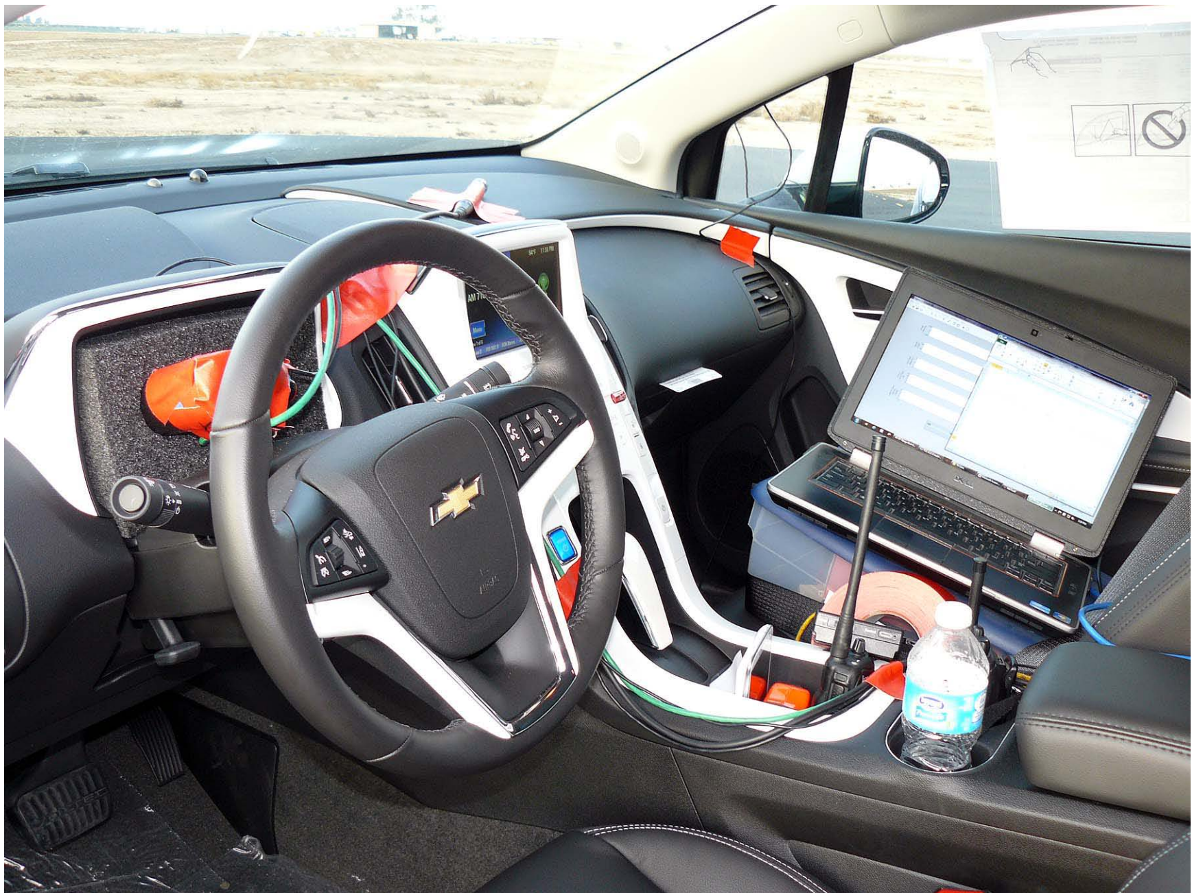
Figure A9. Computer Installed in Subject Vehicle
