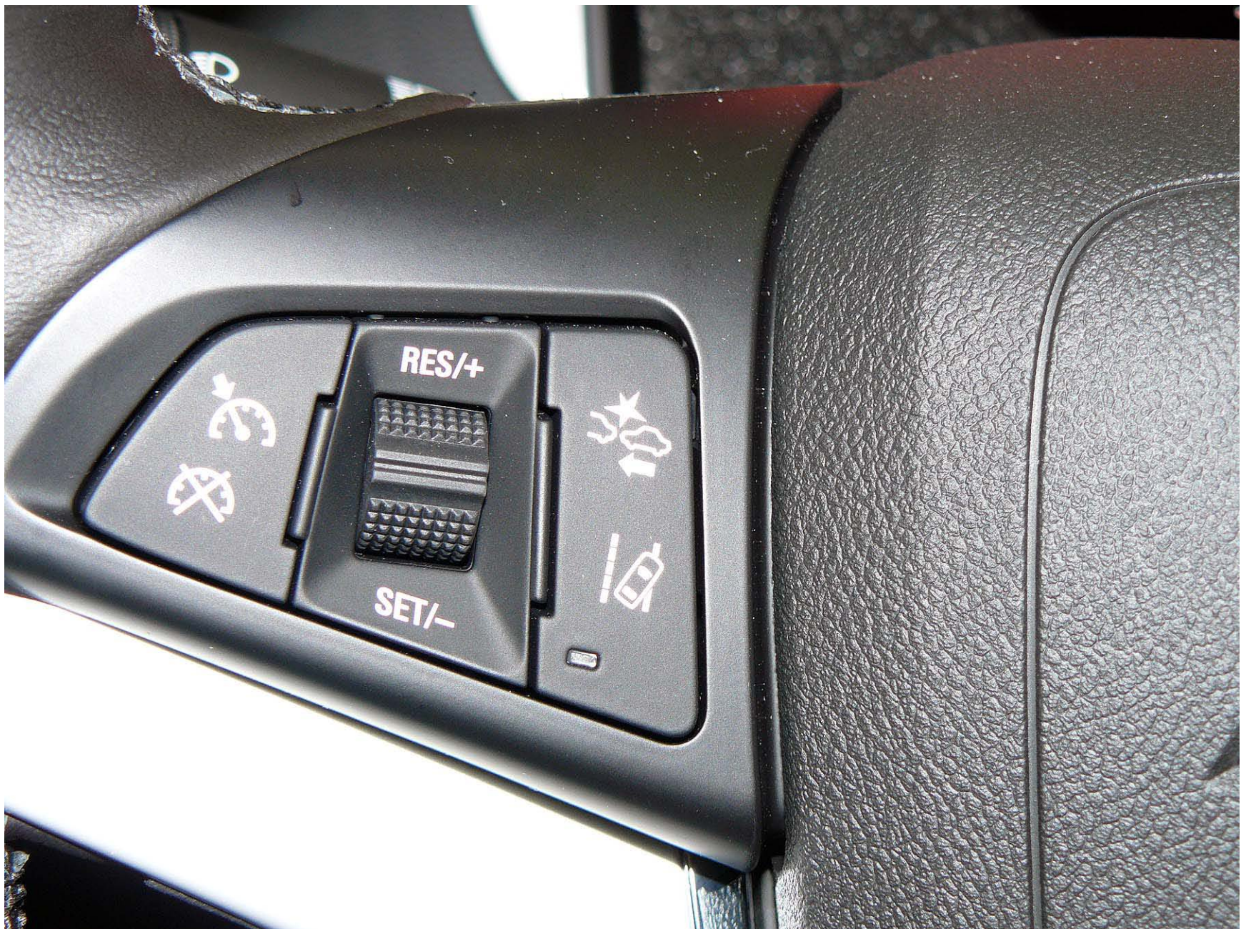
Figure A12. Warning System On-Off and Settings Adjustment Switch
