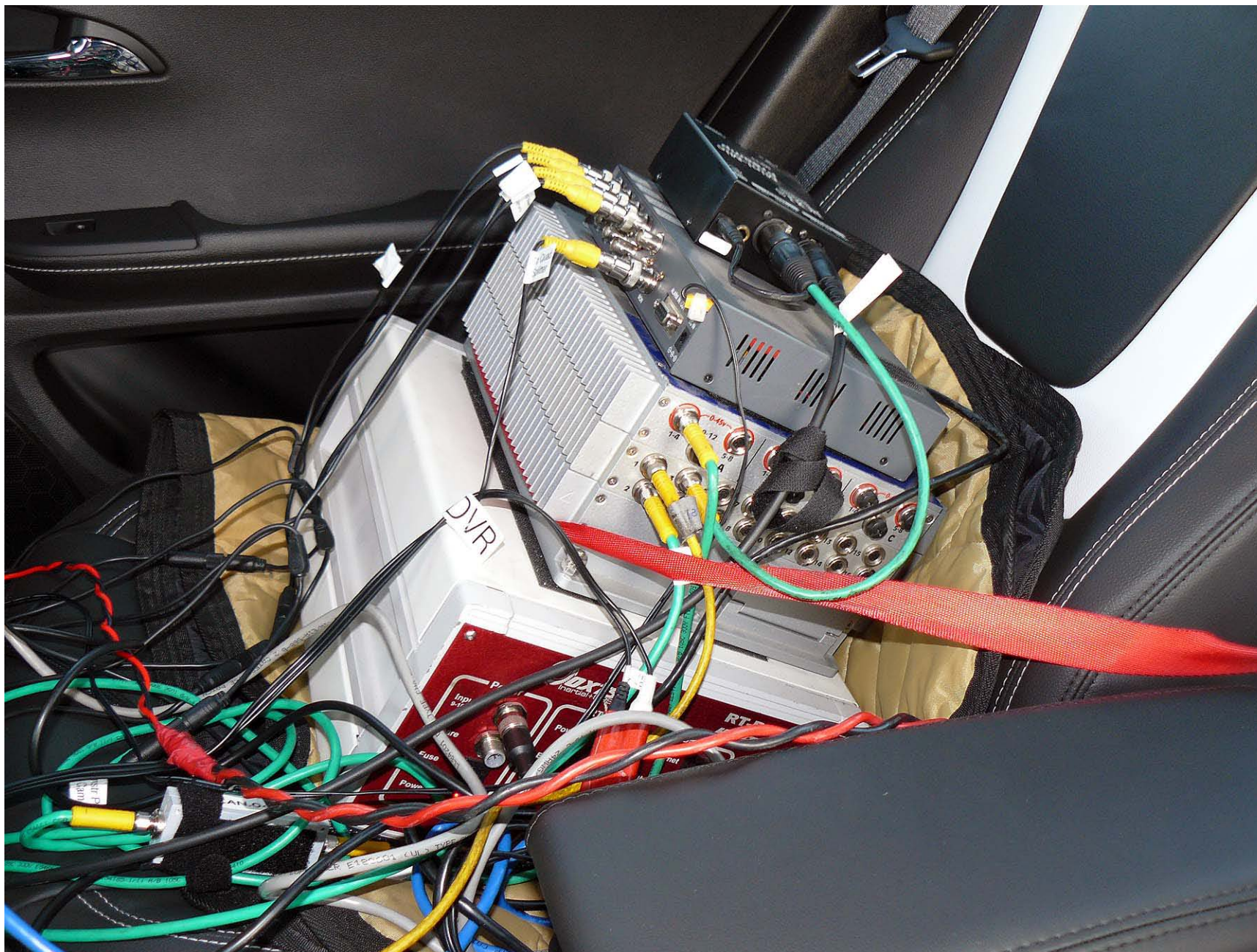
Figure A8. Data Acquisition System Installed in Subject Vehicle
