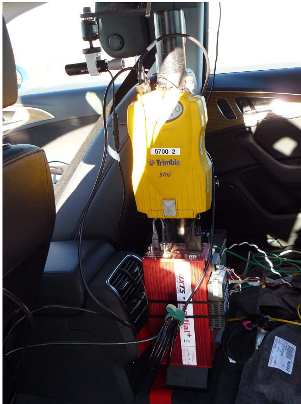
Figure A7. DGPS and Inertial Measurement Unit Installed in Subject Vehicle
