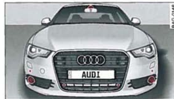
Fig. 82 Front of the vehicle: sensors and video camera
