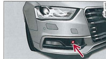
Fig. 96 Front of the vehicle: Position of radar sensor
