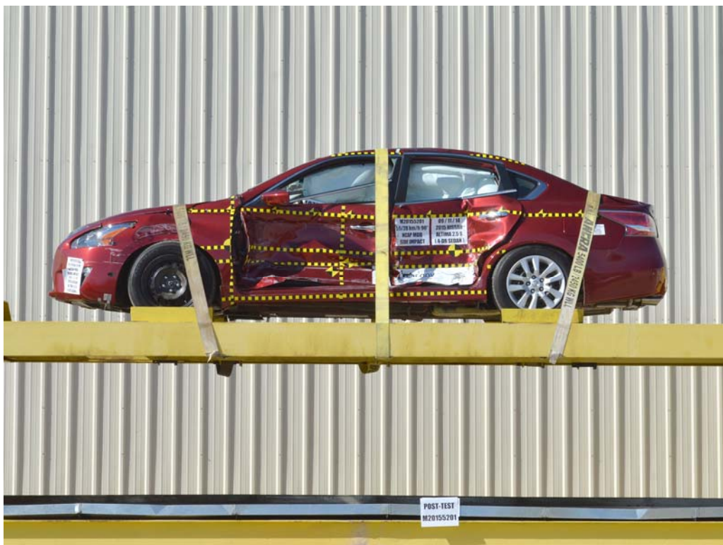
FIGURE 100. FMVSS No. 301 Static Rollover 360 Degrees
