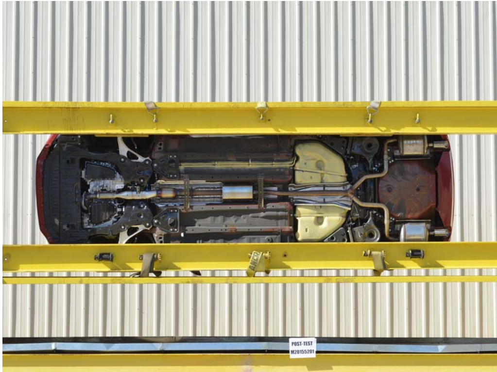
FIGURE 99. FMVSS No. 301 Static Rollover 270 Degrees
