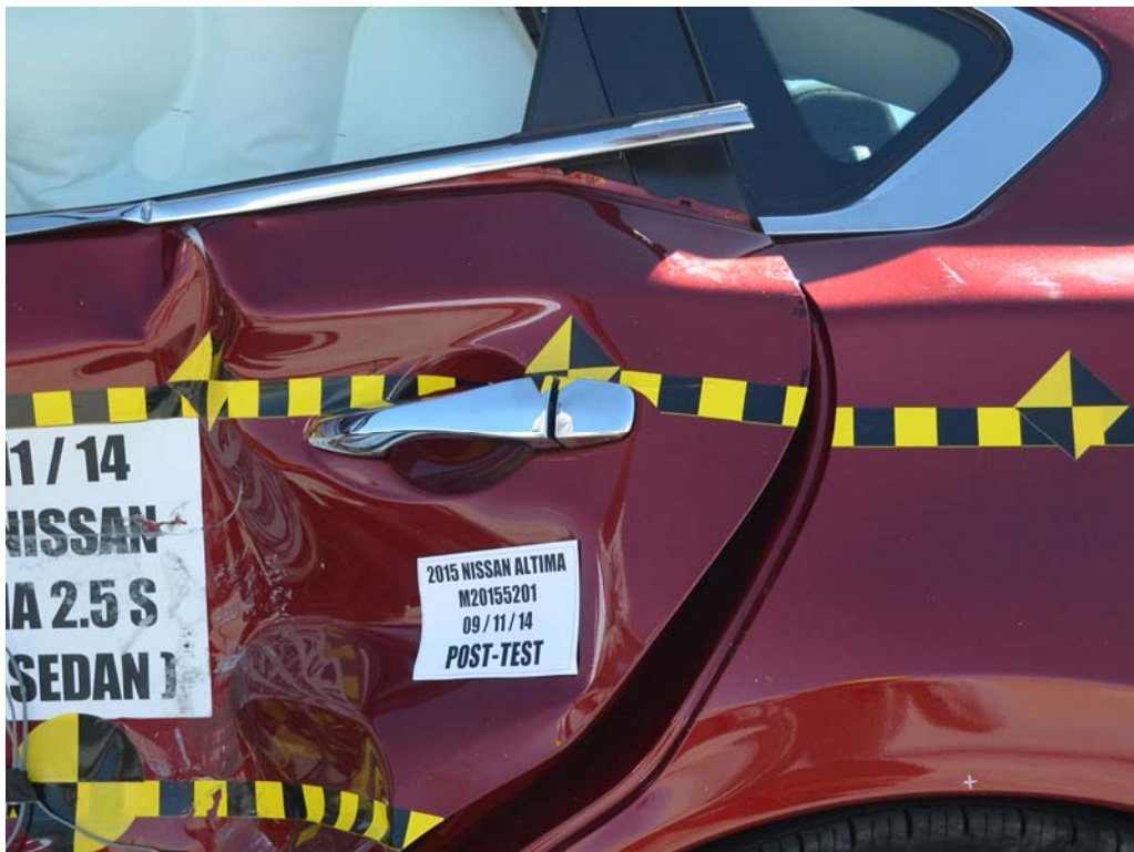
FIGURE 24. Post-Test Left Rear Door Latch Close-Up
