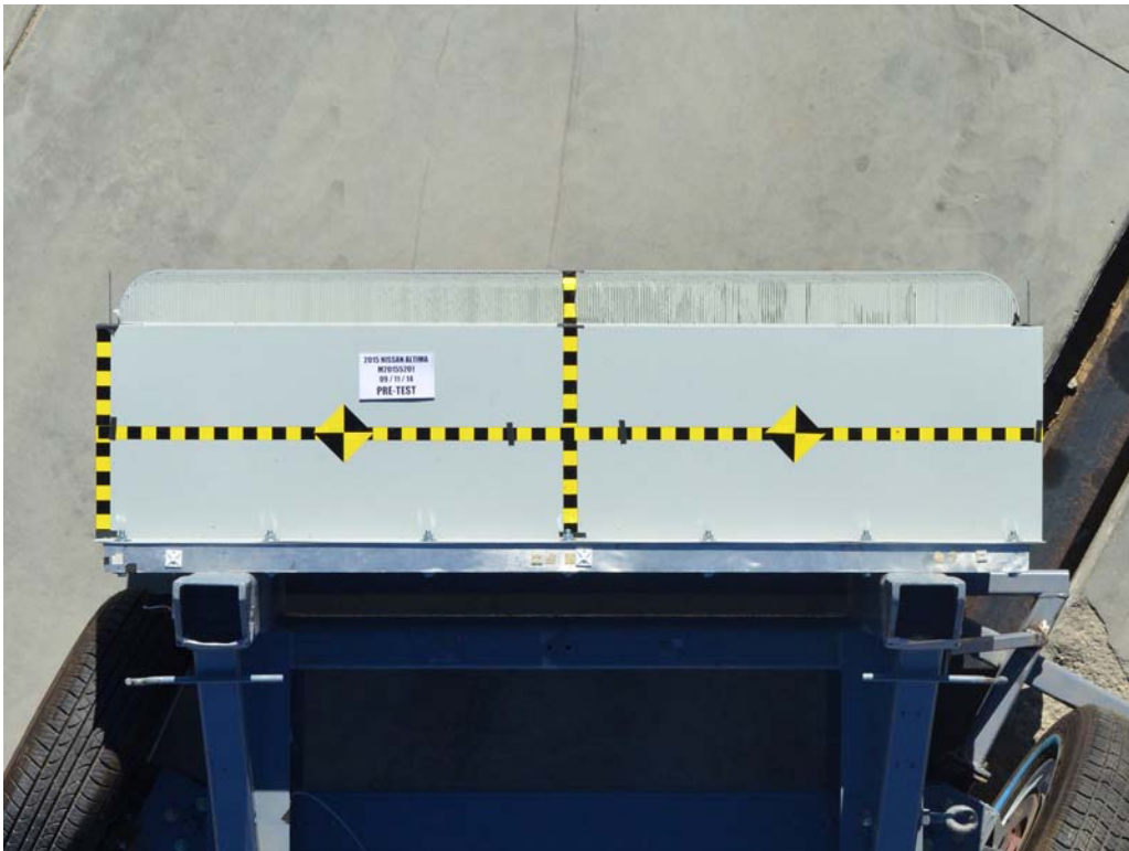
FIGURE 86. Pre-Test Top View of MDB Impactor Face
