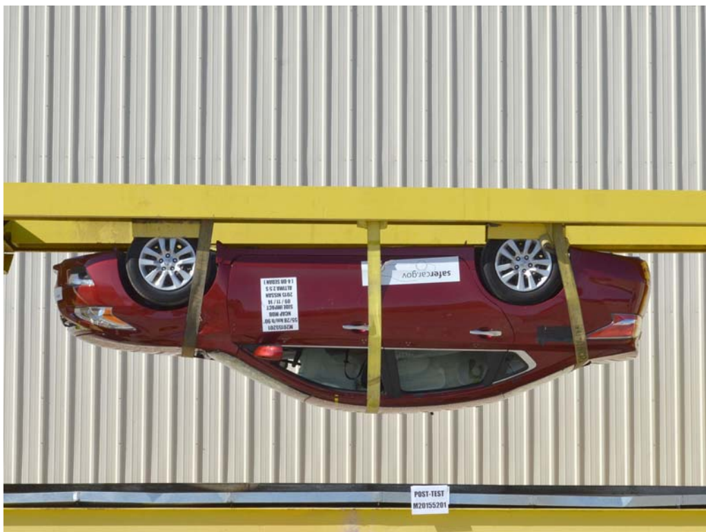
FIGURE 98. FMVSS No. 301 Static Rollover 180 Degrees
