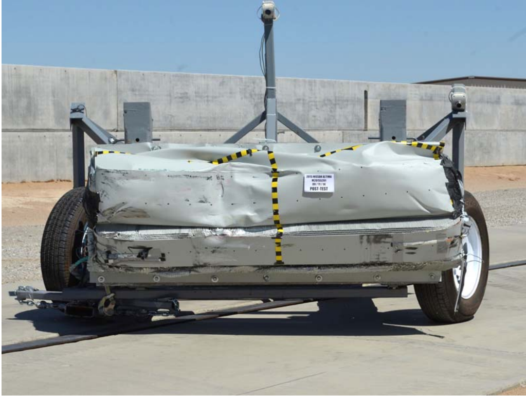
FIGURE 85. Post-Test Front View of MDB Impactor Face
