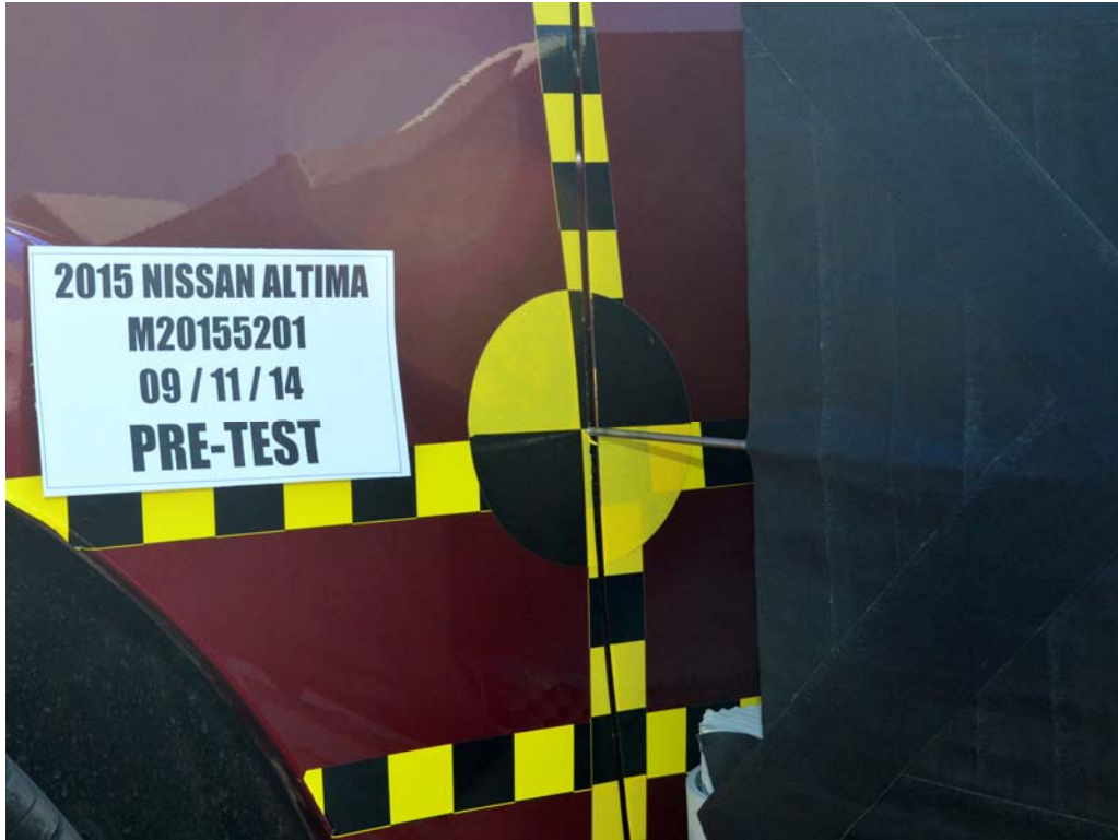
FIGURE 19. Pre-Test Close-Up View of Impact Point Target
