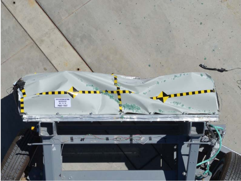
FIGURE 87. Post-Test Top View of MDB Impactor Face
