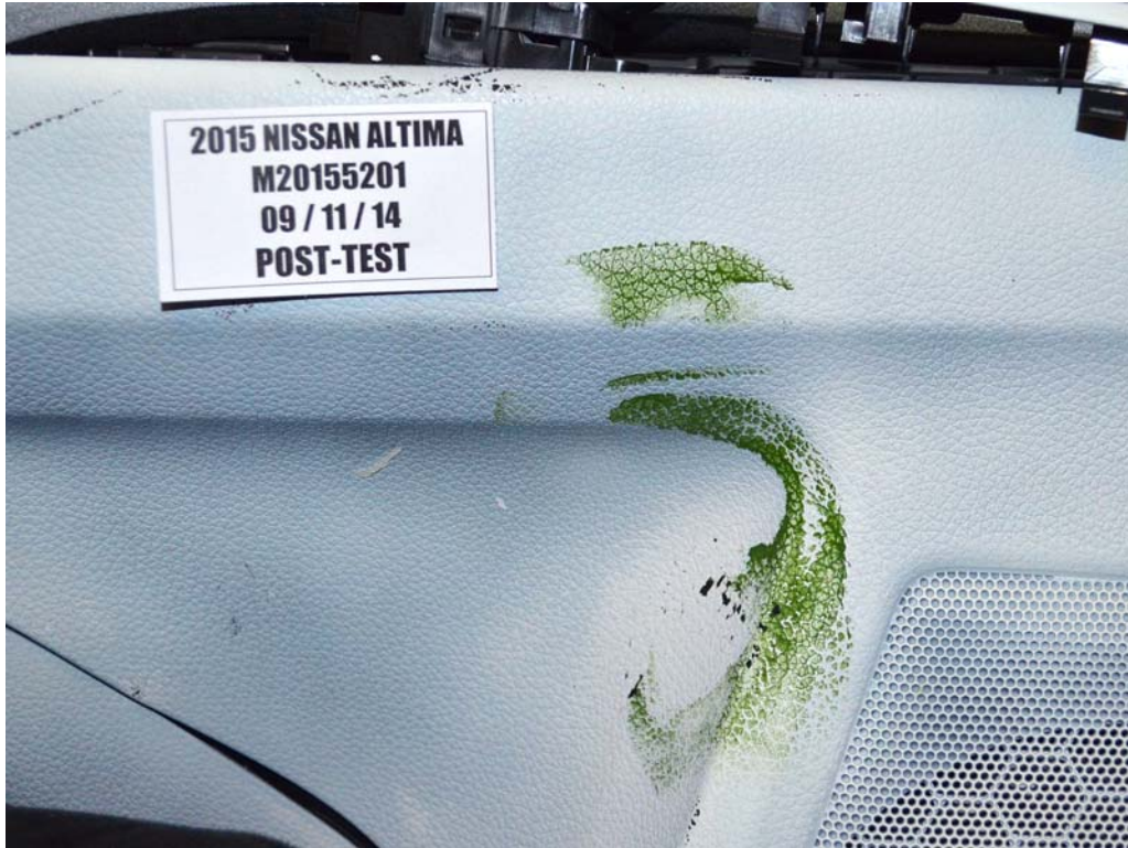
FIGURE 81. Post-Test Rear Passenger Dummy Close-Up Knee Contact View
