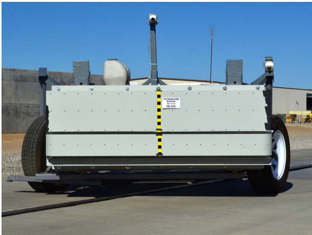
FIGURE 84. Pre-Test Front View of MDB Impactor Face
