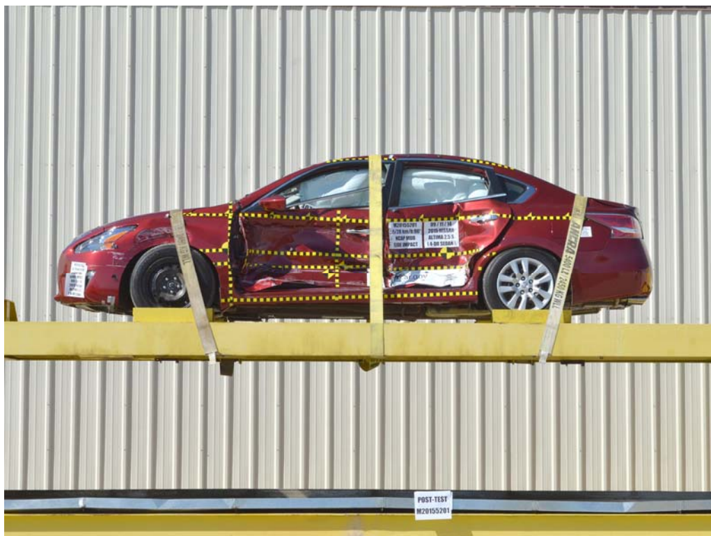
FIGURE 96. FMVSS No. 301 Static Rollover 0 Degrees
