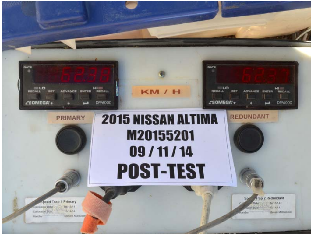
FIGURE 95. Post-Test Primary and Redundant Speed Trap Read-Out
