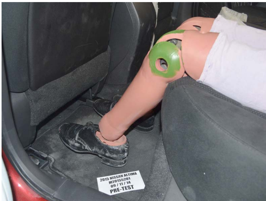
FIGURE 64. Pre-Test Placement of Rear Passenger Dummy's Feet
