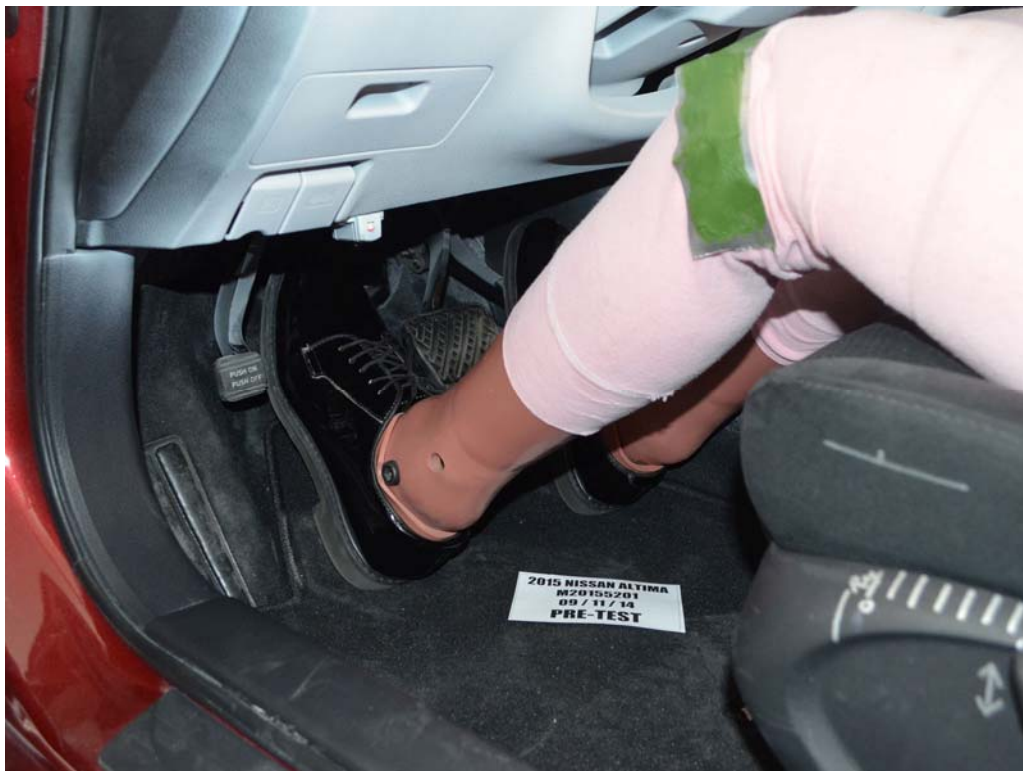
FIGURE 34. Pre-Test Placement of Driver Dummy's Feet
