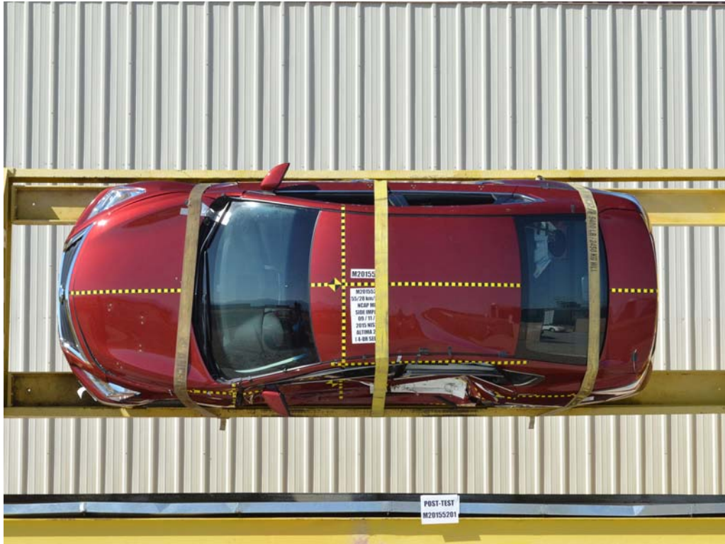
FIGURE 97. FMVSS No. 301 Static Rollover 90 Degrees
