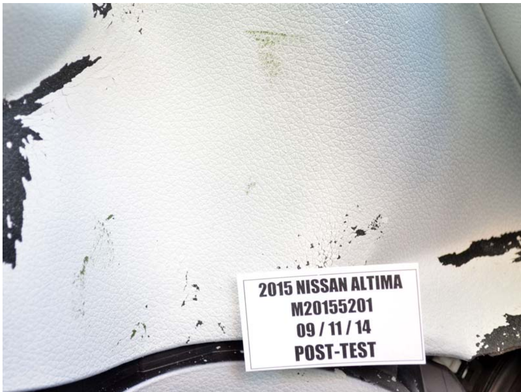
FIGURE 54. Post-Test Driver Dummy Close-Up Knee Contact View
