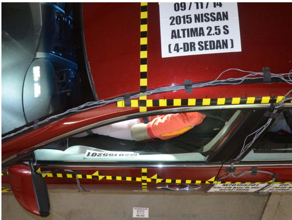
FIGURE 42. Pre-Test Driver Dummy and Door Clearance View
