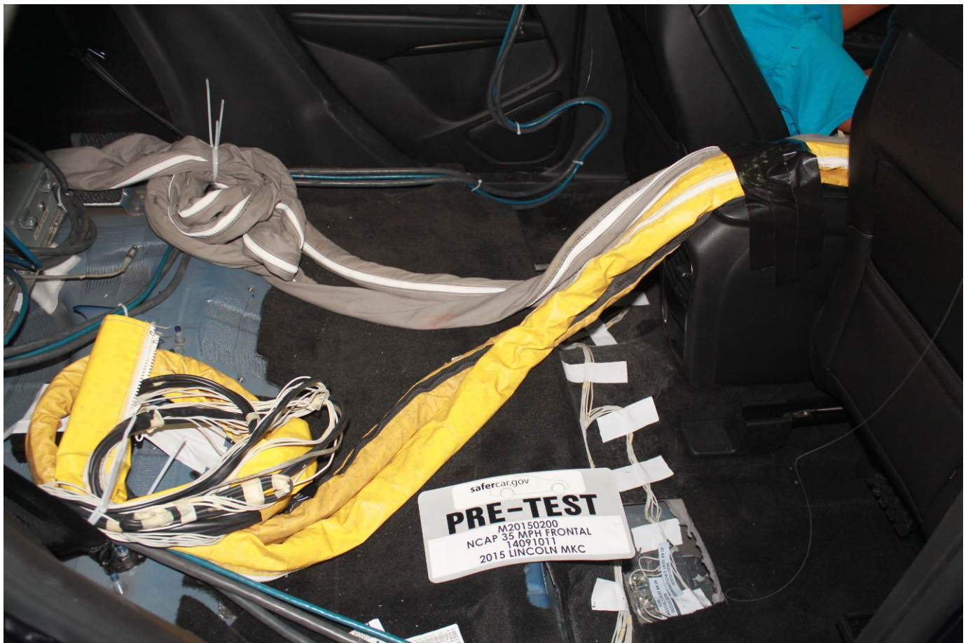
Pre-Test Dummy Cable Routing
