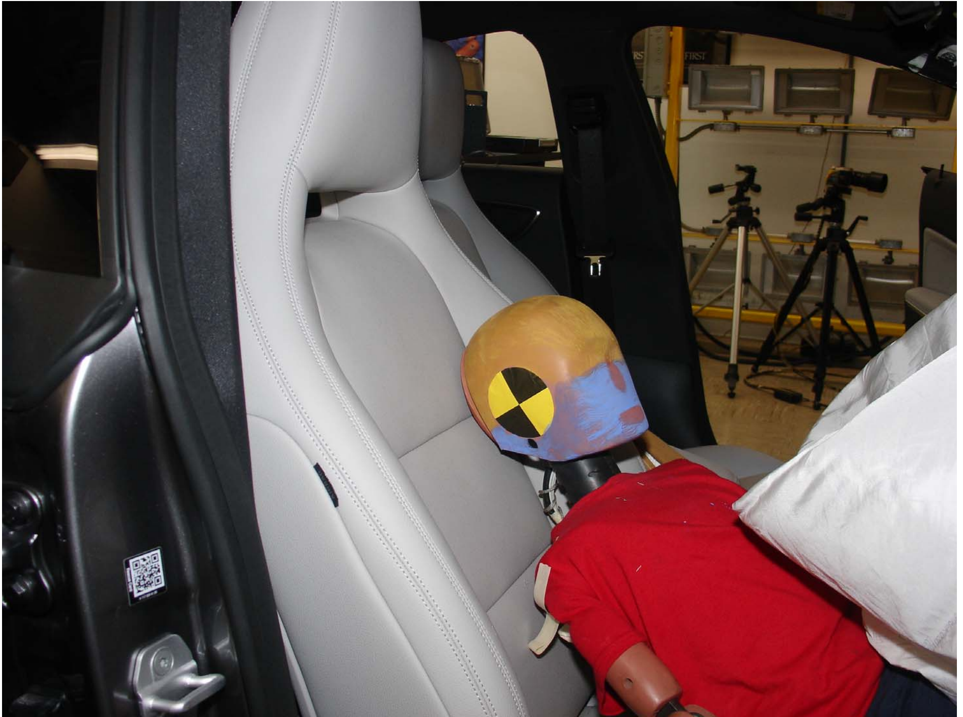
Photo No. 38 - Post-Test 6YO P2 Passenger Dummy Head Contact (seat back)
