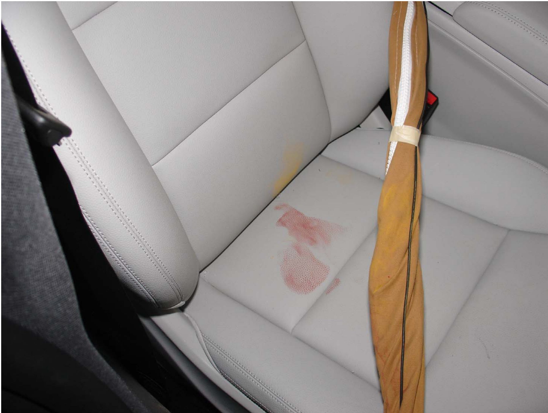
Photo No. 32 - Post-Test 6YO P1 Passenger Dummy Head Contact (seat cushion)
