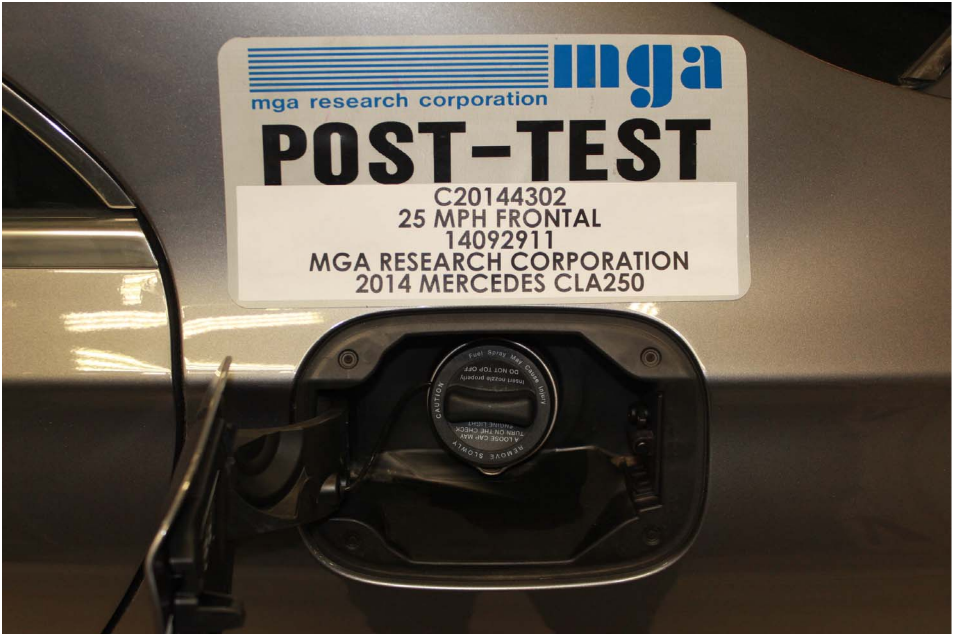
Photo No. 24 - Post-Test Fuel Filler Cap View
