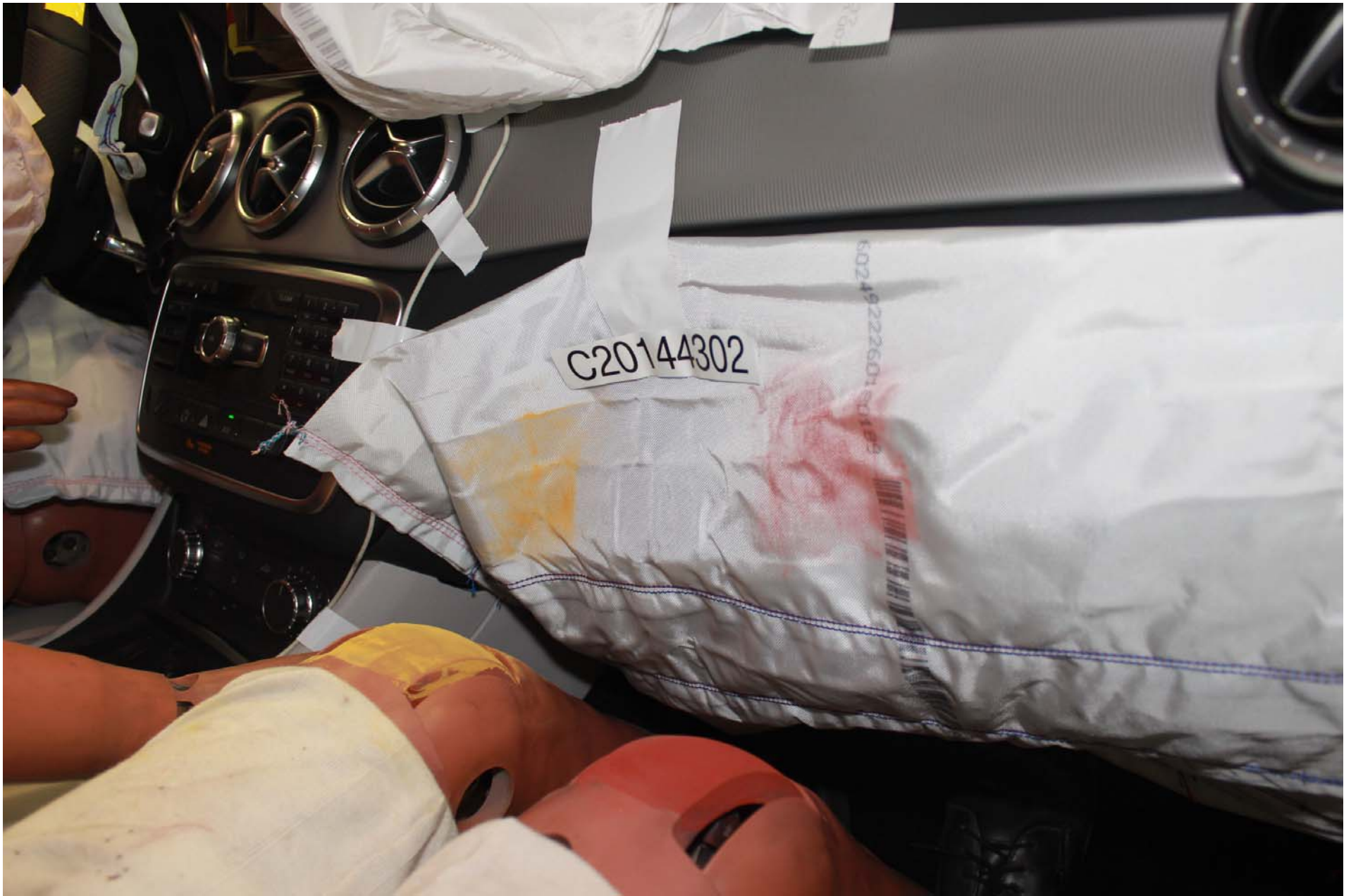
Photo No. 62 - Post-Test Passenger Dummy Knee Contact (knee airbag)
