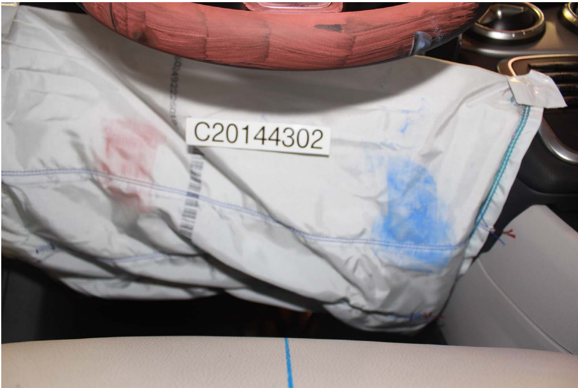
Photo No. 46 - Post-Test Driver Dummy Knee Contact (knee airbag)
