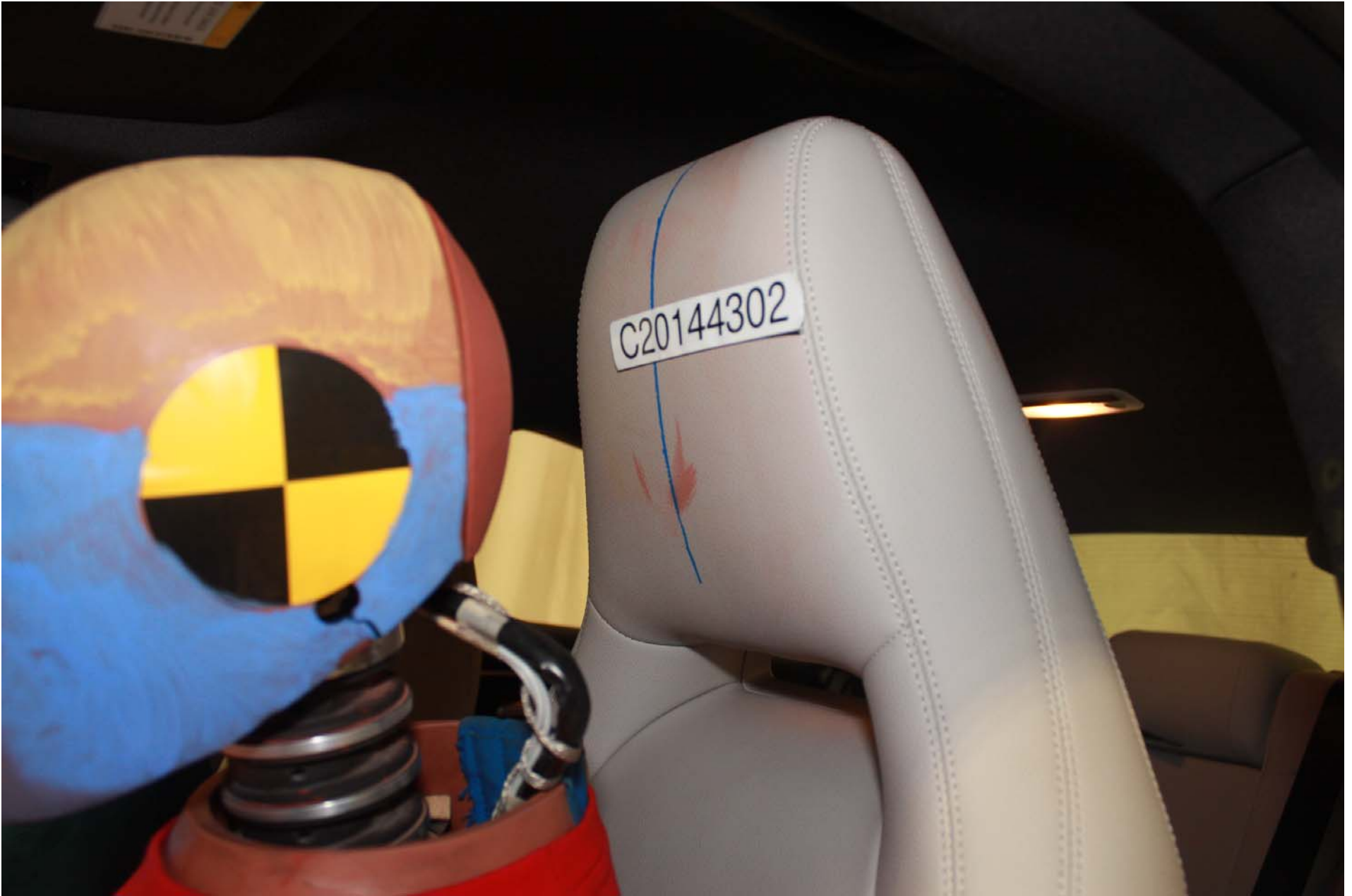
Photo No. 48 - Post-Test Driver Dummy Head Contact (headrest)
