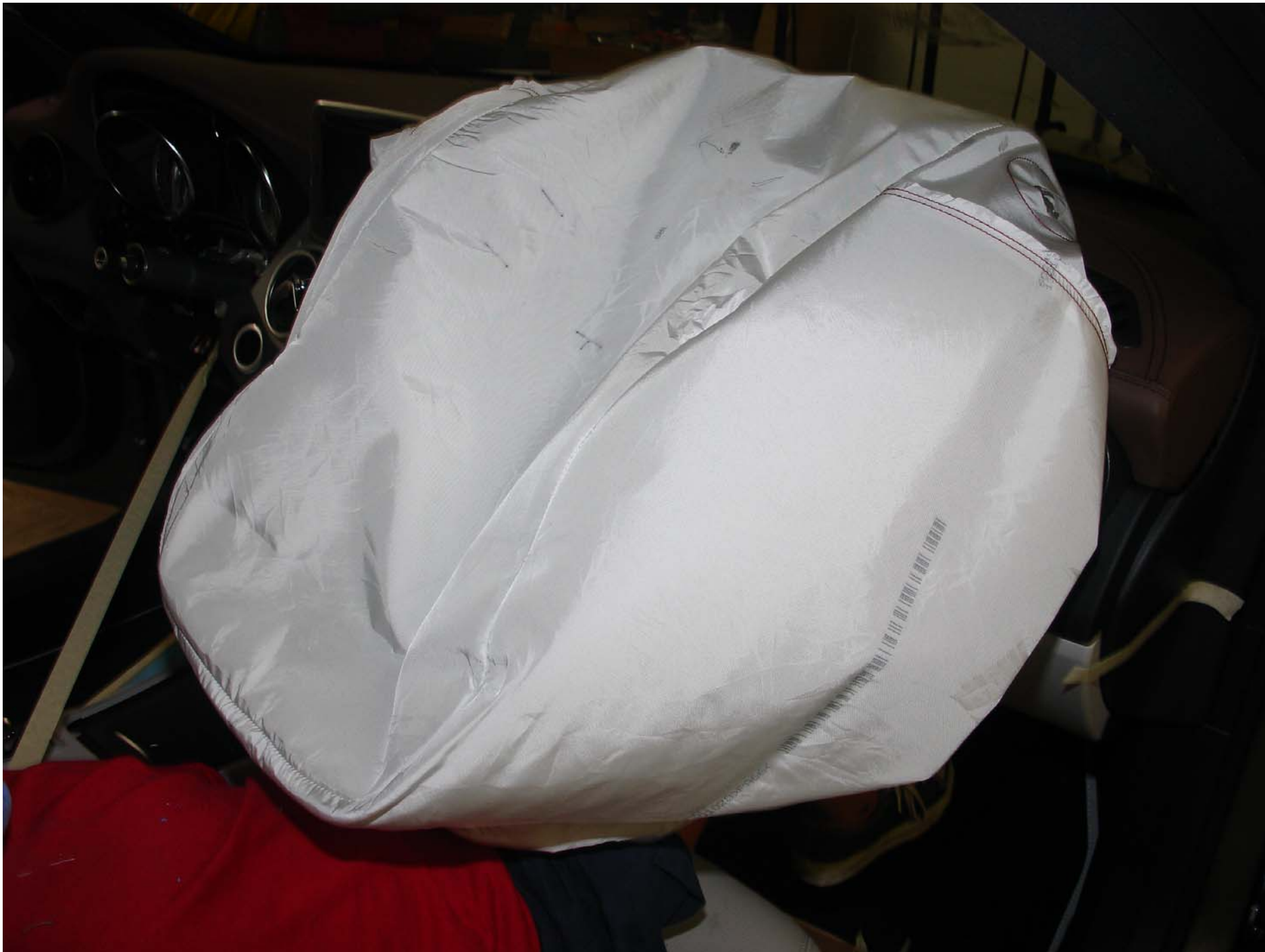
Photo No. 37 - Post-Test 6YO P2 Passenger Dummy Airbag Right Side View
