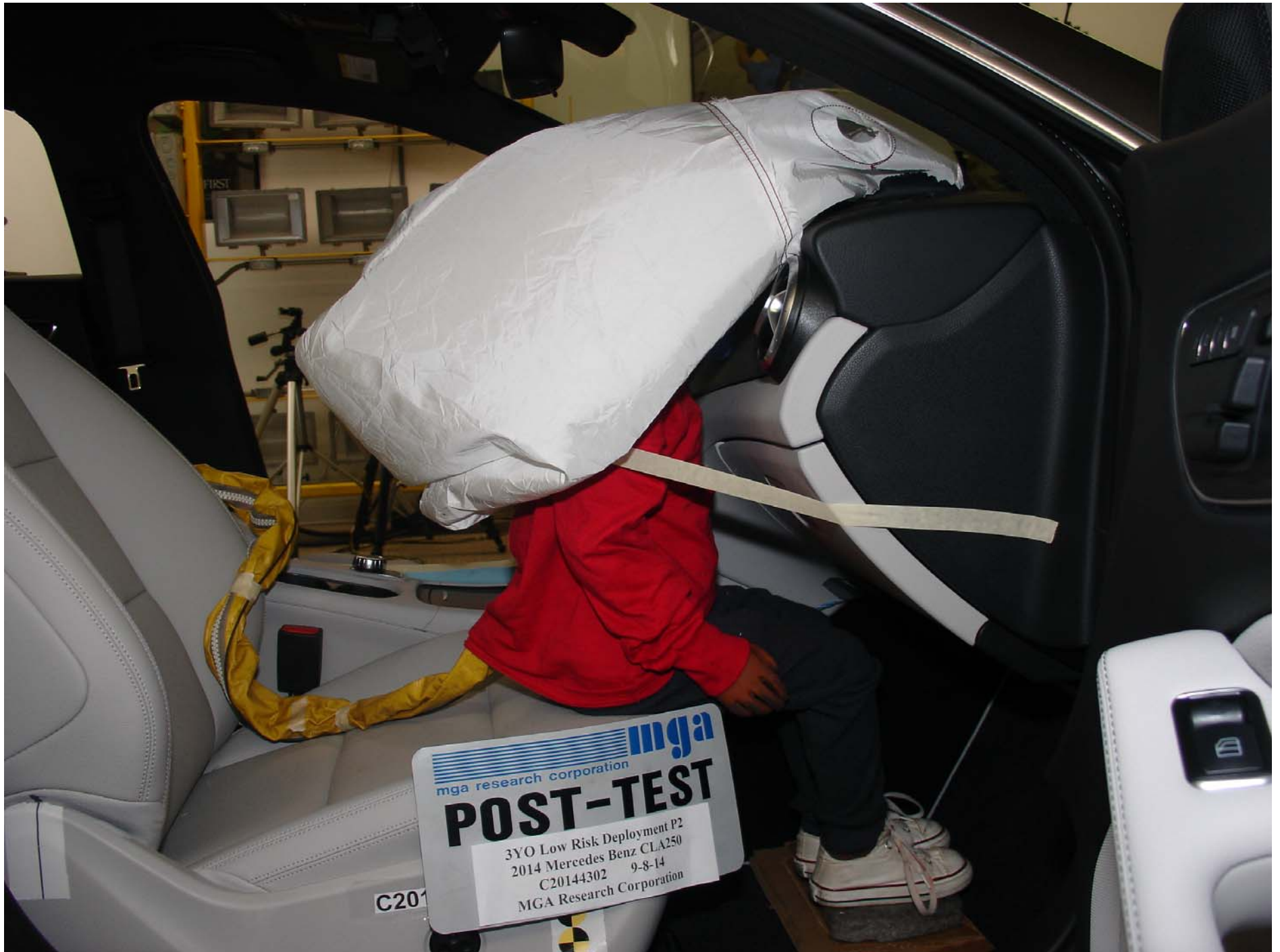
Photo No. 25 - Post-Test 3YO P2 Passenger Dummy Right Side View
