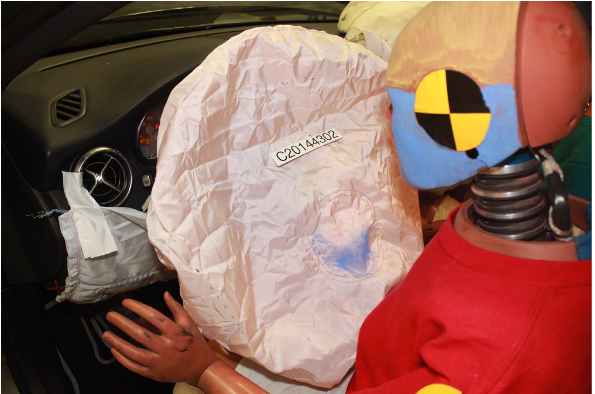
Photo No. 45 - Post-Test Driver Dummy Airbag Contact
