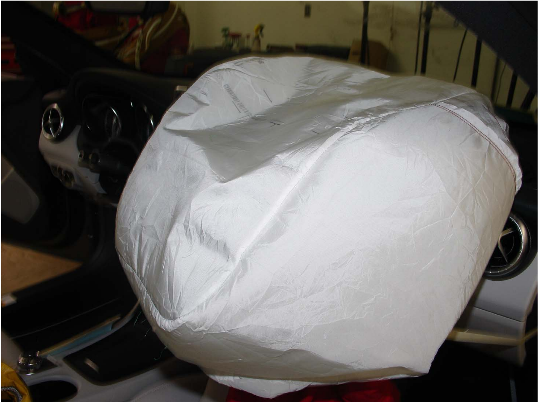
Photo No. 26 - Post-Test 3YO P2 Passenger Dummy Airbag Right Side View
