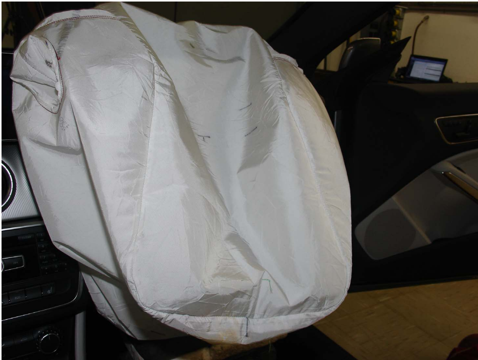
Photo No. 31 - Post-Test 6YO P1 Passenger Dummy Airbag Left Side View
