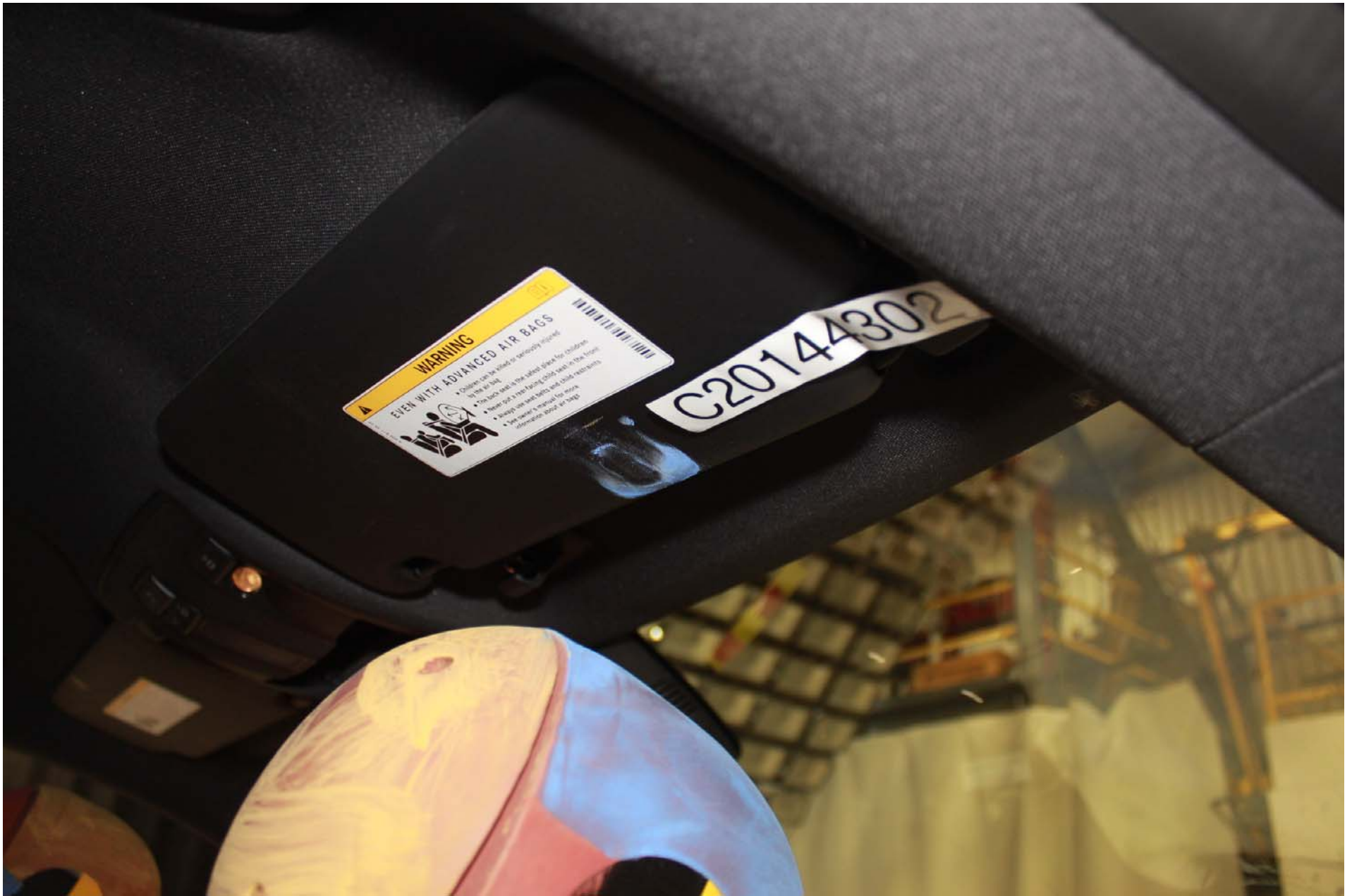
Photo No. 63 - Post-Test Passenger Dummy Head Contact (visor)
