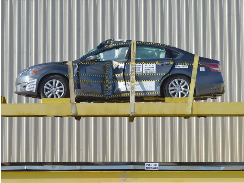
FIGURE 67. FMVSS No. 301 Static Rollover 360 Degrees
