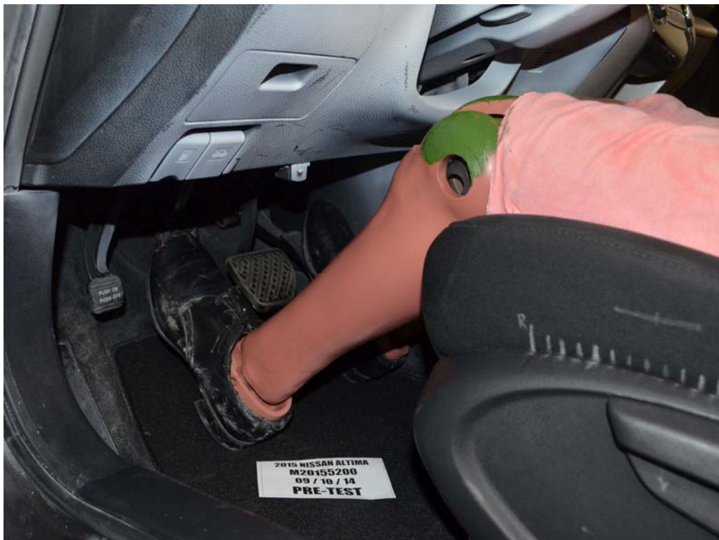
FIGURE 32. Pre-Test Placement of Dummy's Feet
