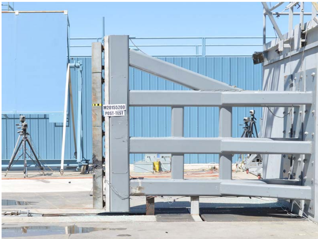
FIGURE 60. Post-Test Pole Barrier Side View
