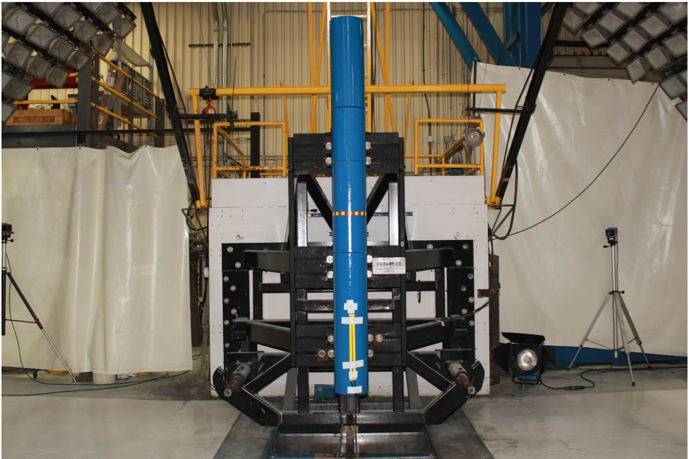
Pre-Test Pole Barrier Front View
