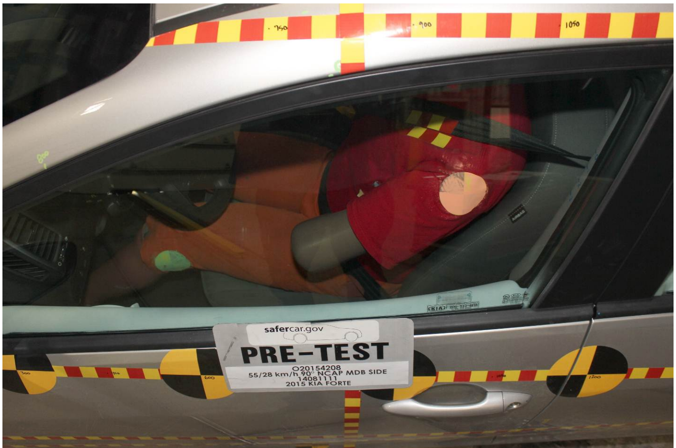
Pre-Test Driver Dummy and Door Clearance View
