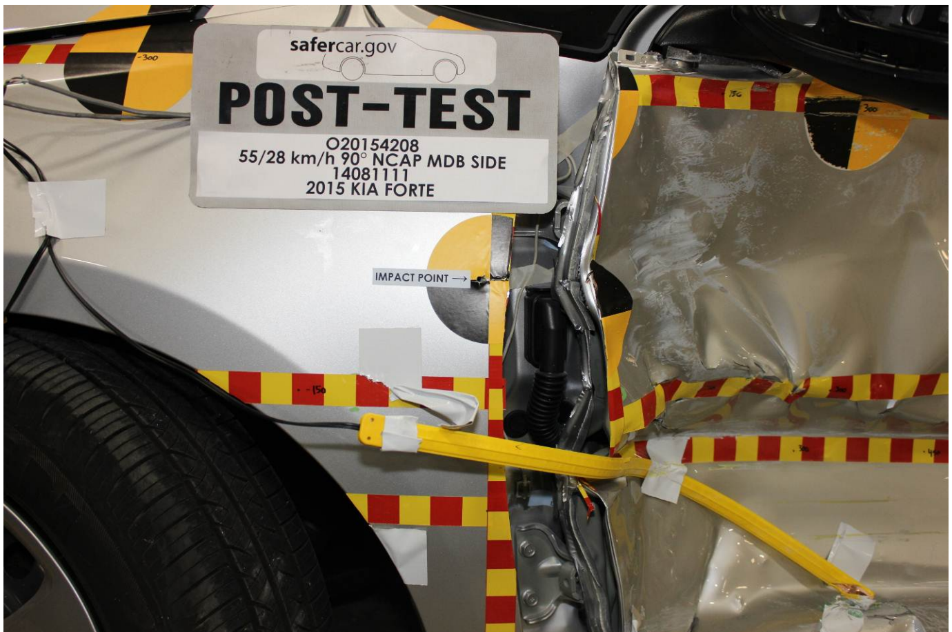
Post-Test Close-Up View of Impact Point Target
