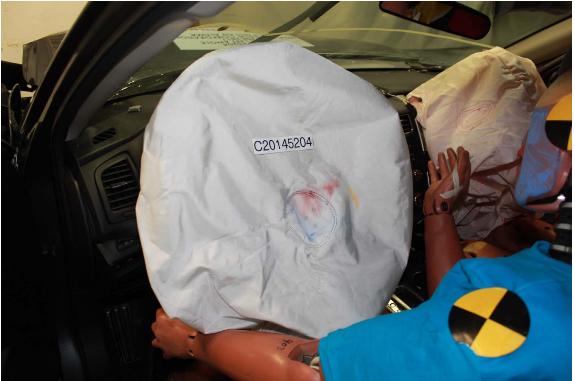
Photo No. 45 - Post-Test Driver Dummy Airbag Contact
