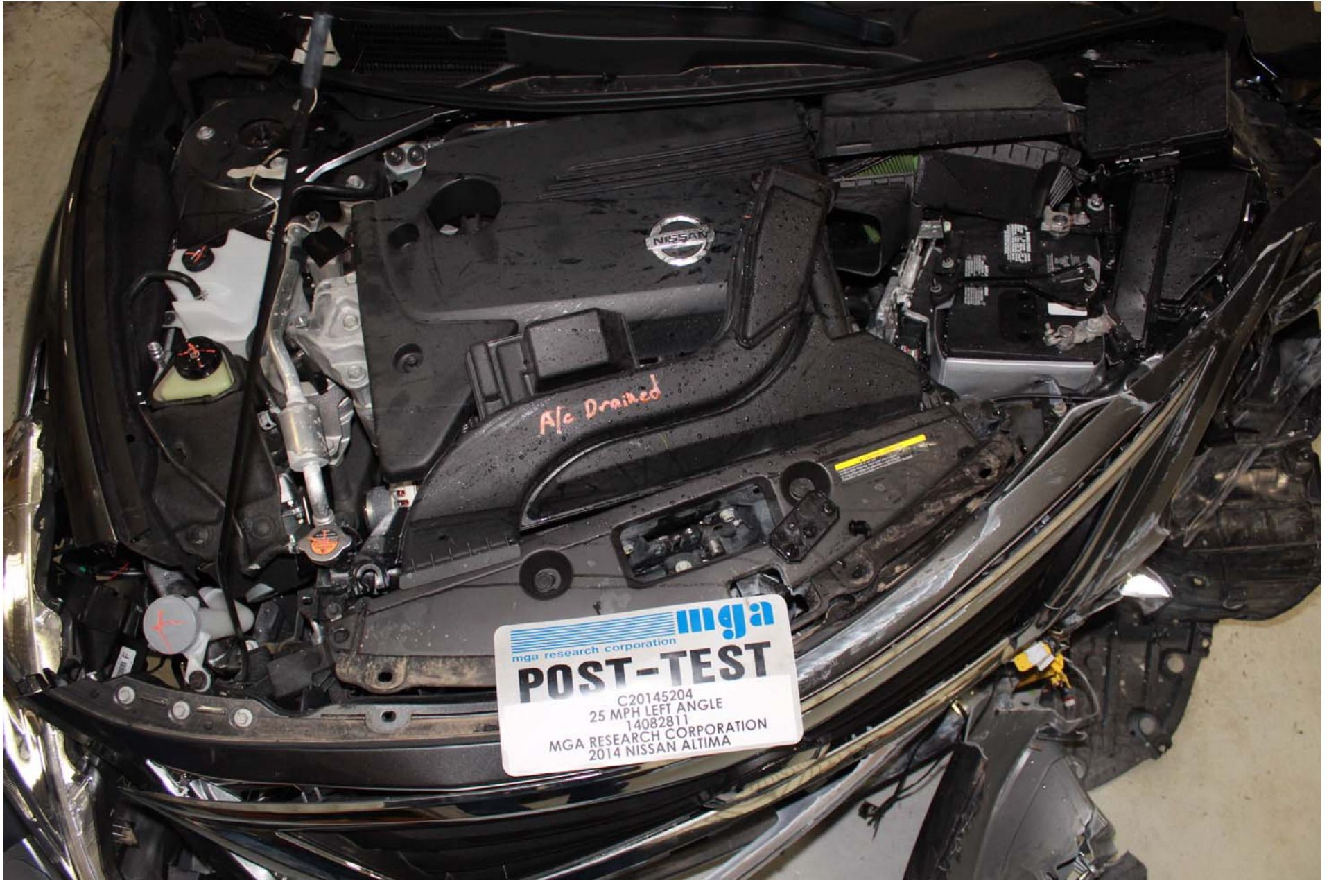
Photo No. 22 - Post-Test Engine Compartment View
