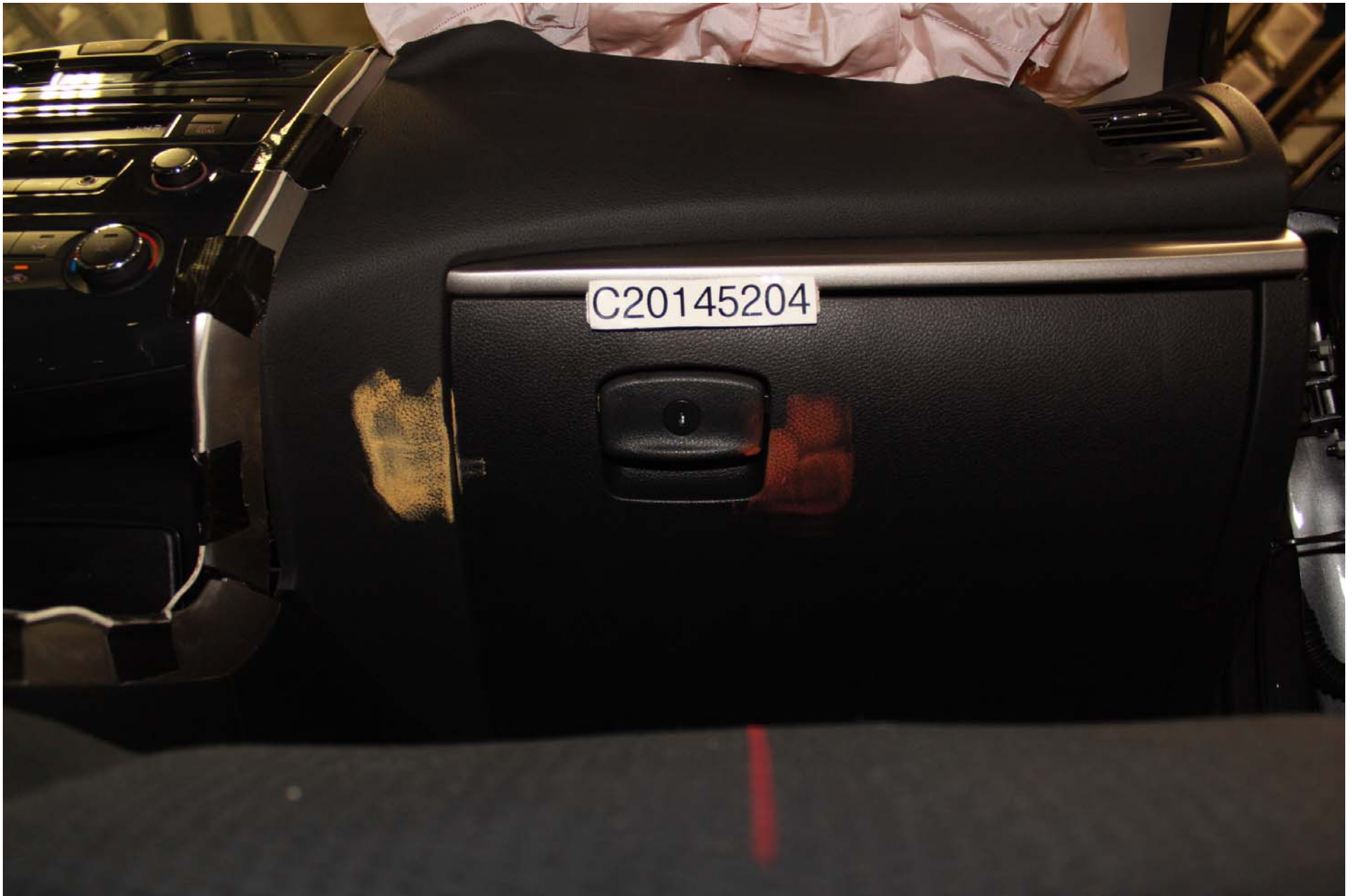
Photo No. 64 - Post-Test Passenger Dummy Knee Contact (glovebox)
