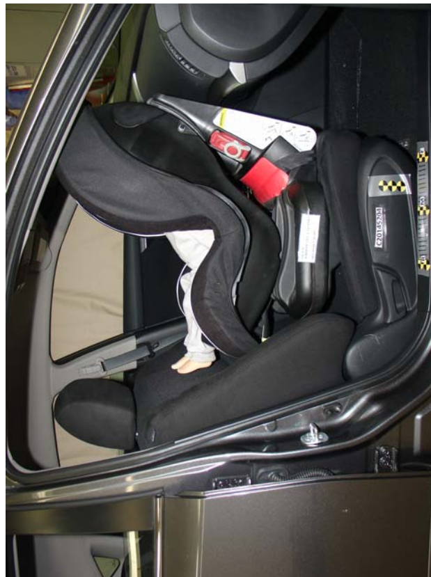
Graco Toddler Safeseat Step 2 Rear Facing, Unbelted, Forward Seat Track
