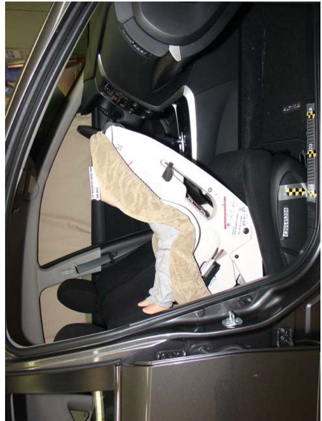
Britax Roundabout Rear Facing, Unbelted, Forward Seat Track
