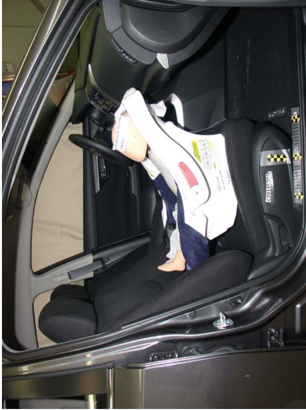
Cosco Arriva WOut Base, Unbelted, Rear Facing, Middle Seat Track
