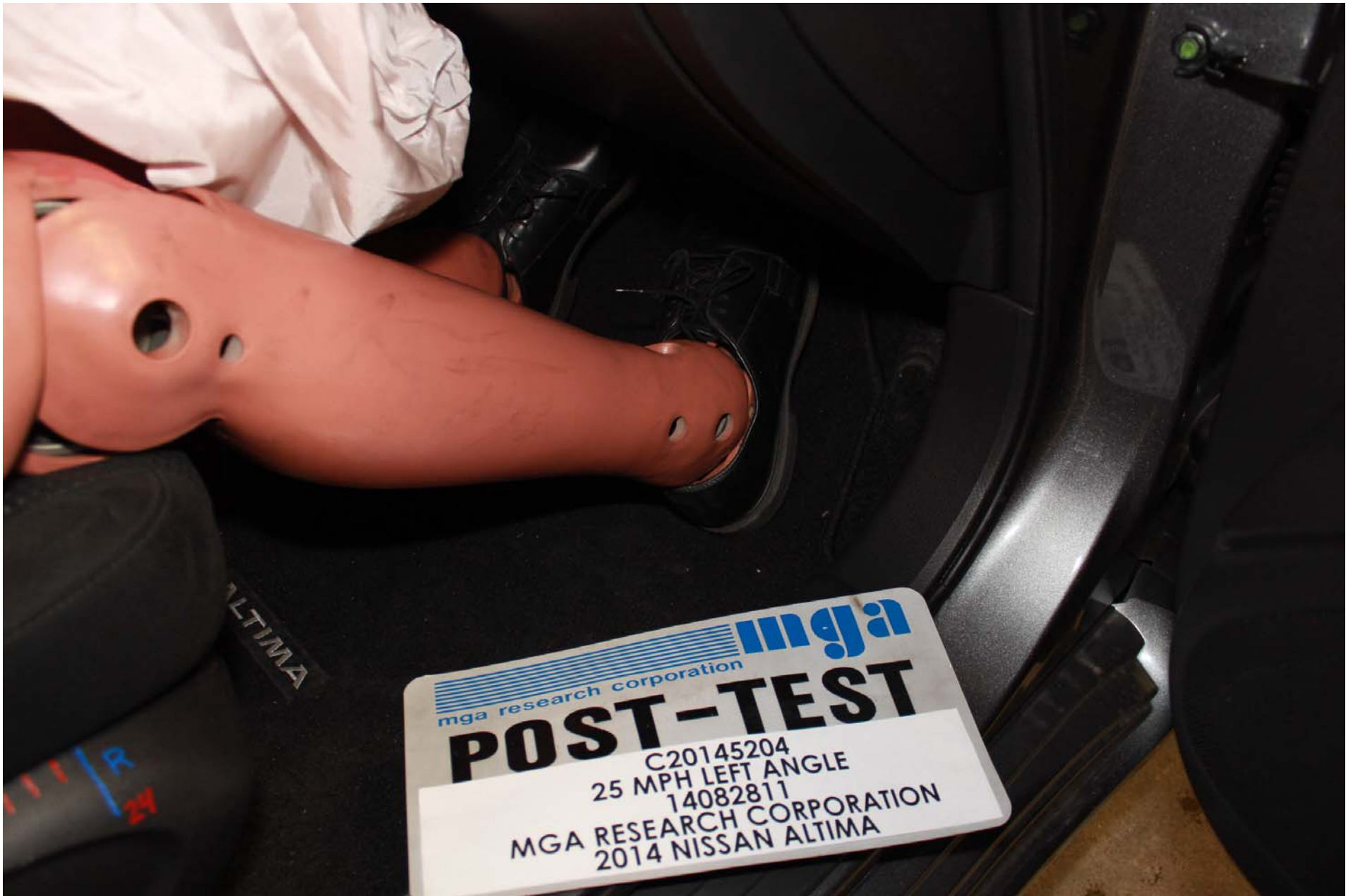
Photo No. 60 - Post-Test Passenger Dummy Feet Position
