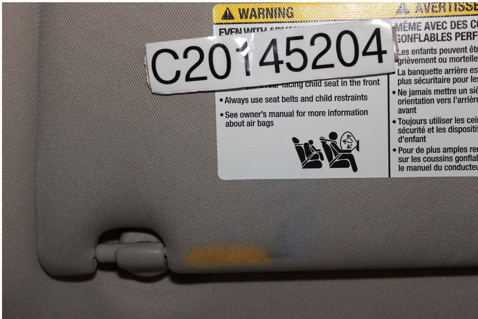
Photo No. 65 - Post-Test Passenger Dummy Head Contact (visor)
