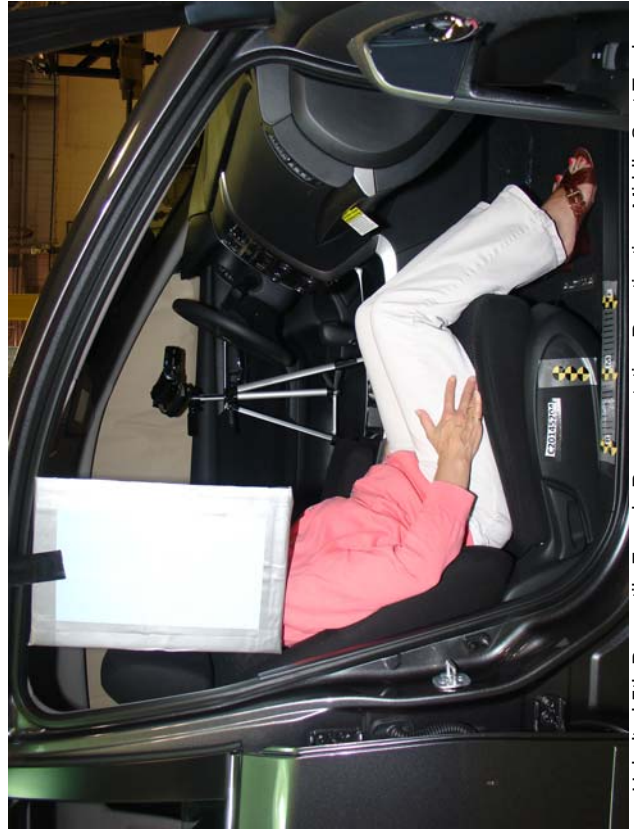
Unbelted 5th Percentile Female Representative Reactivation, Middle Seat Track
