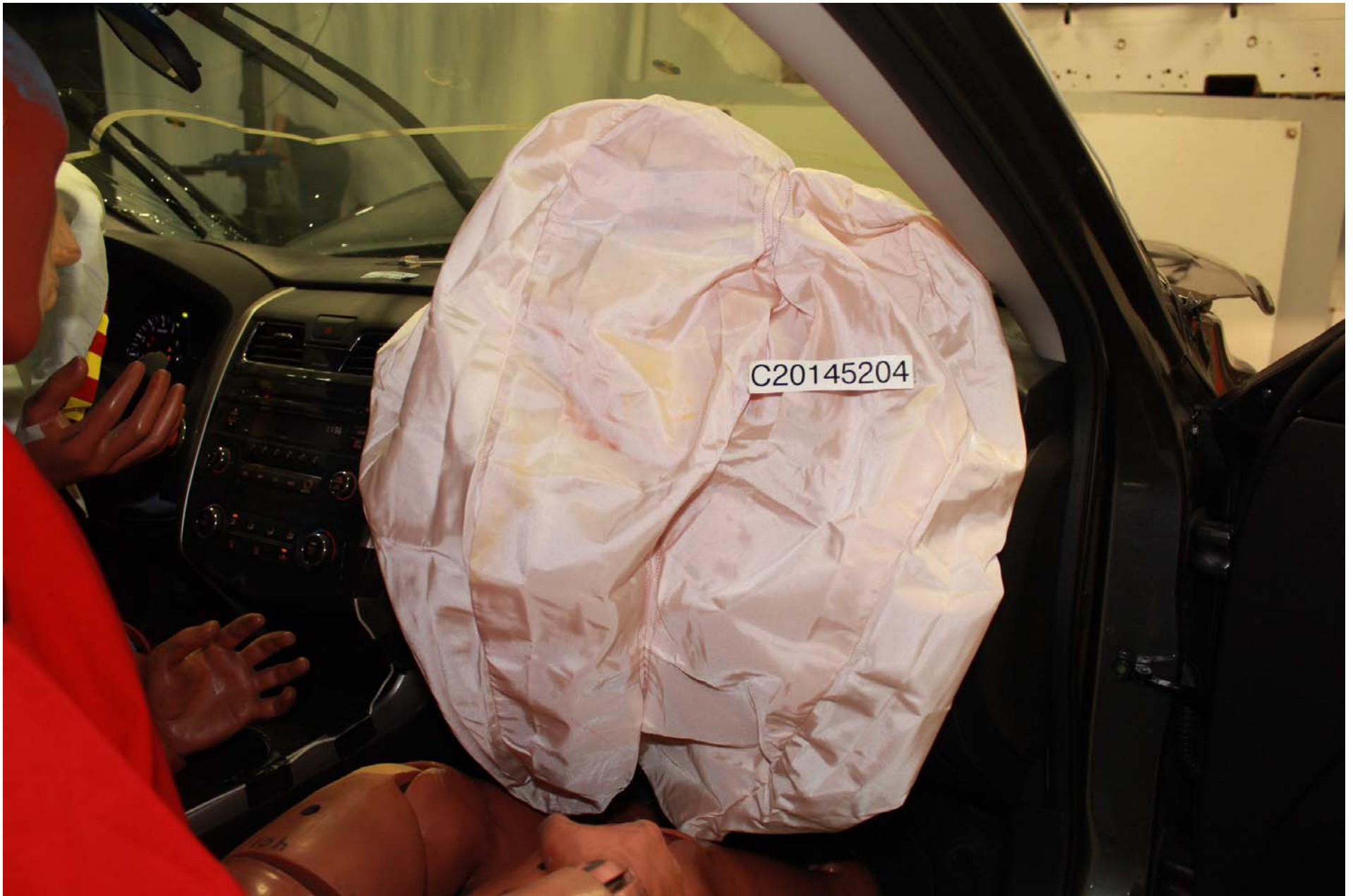
Photo No. 63 - Post-Test Passenger Dummy Airbag Contact
