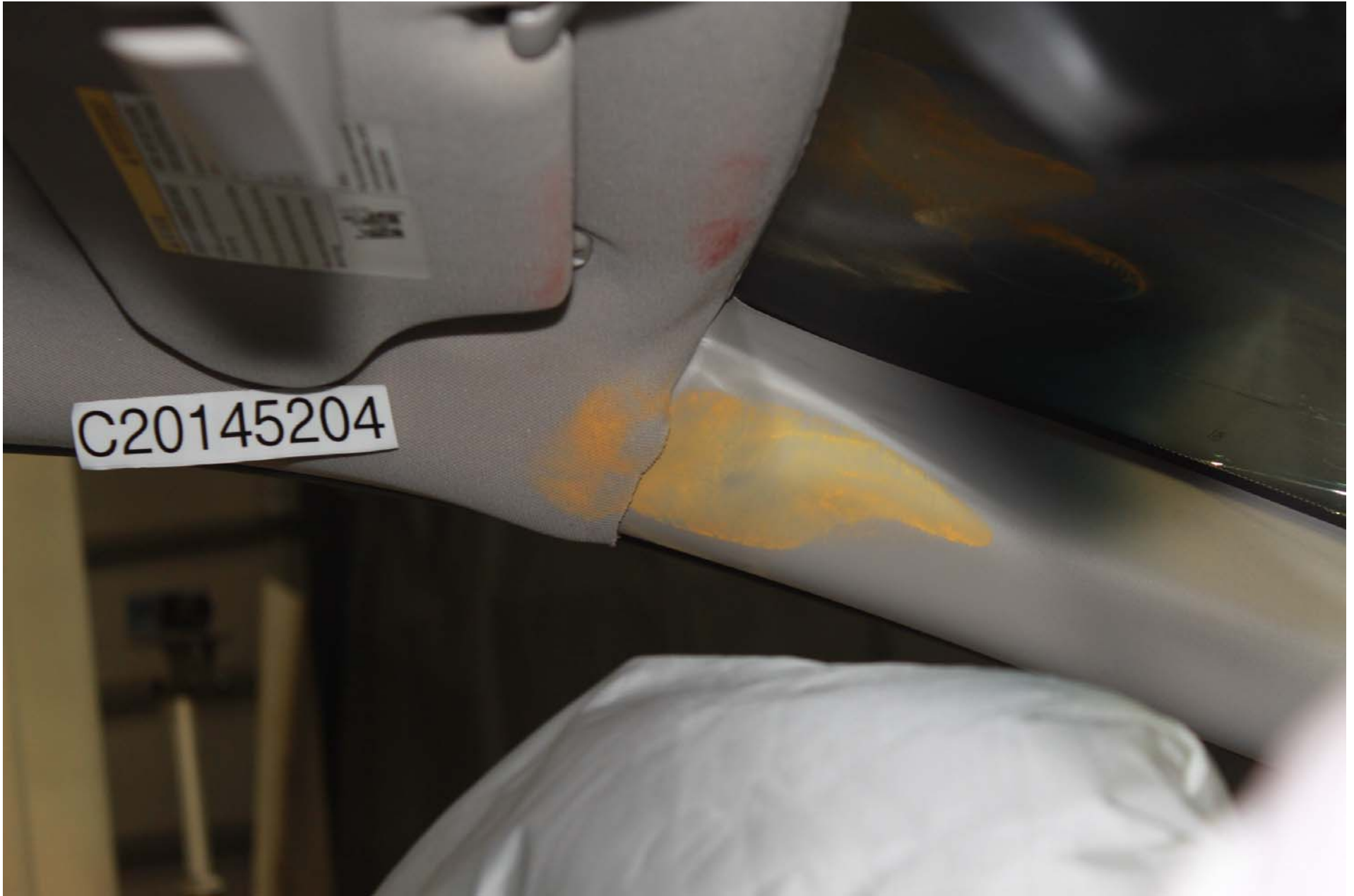
Photo No. 47 - Post-Test Driver Dummy Head Contact (A-pillar)
