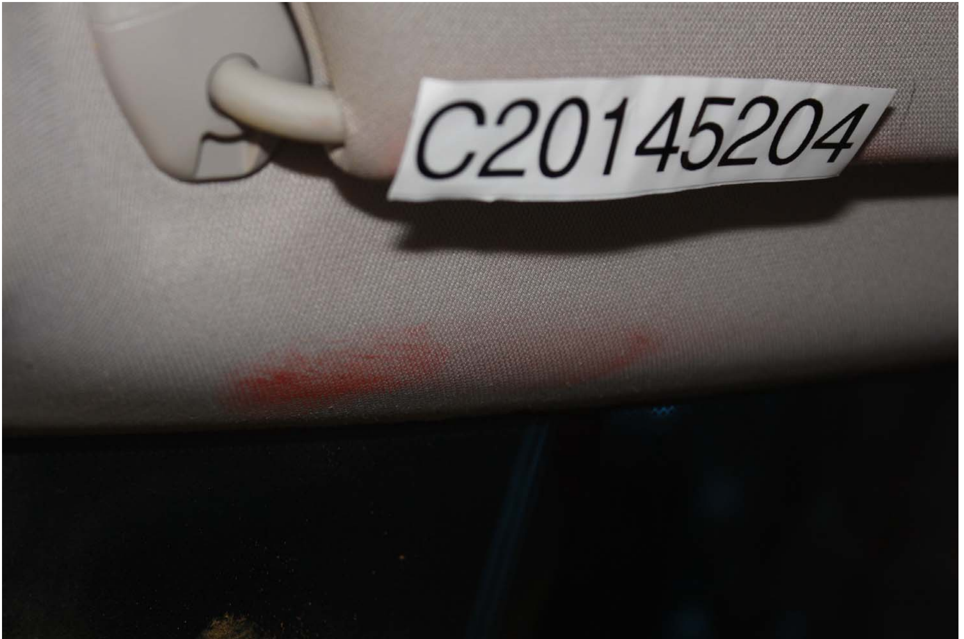
Photo No. 49 - Post-Test Driver Dummy Head Contact (headliner)
