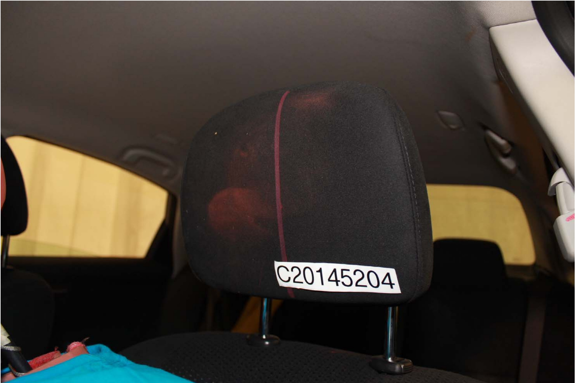
Photo No. 50 - Post-Test Driver Dummy Head Contact (headrest)
