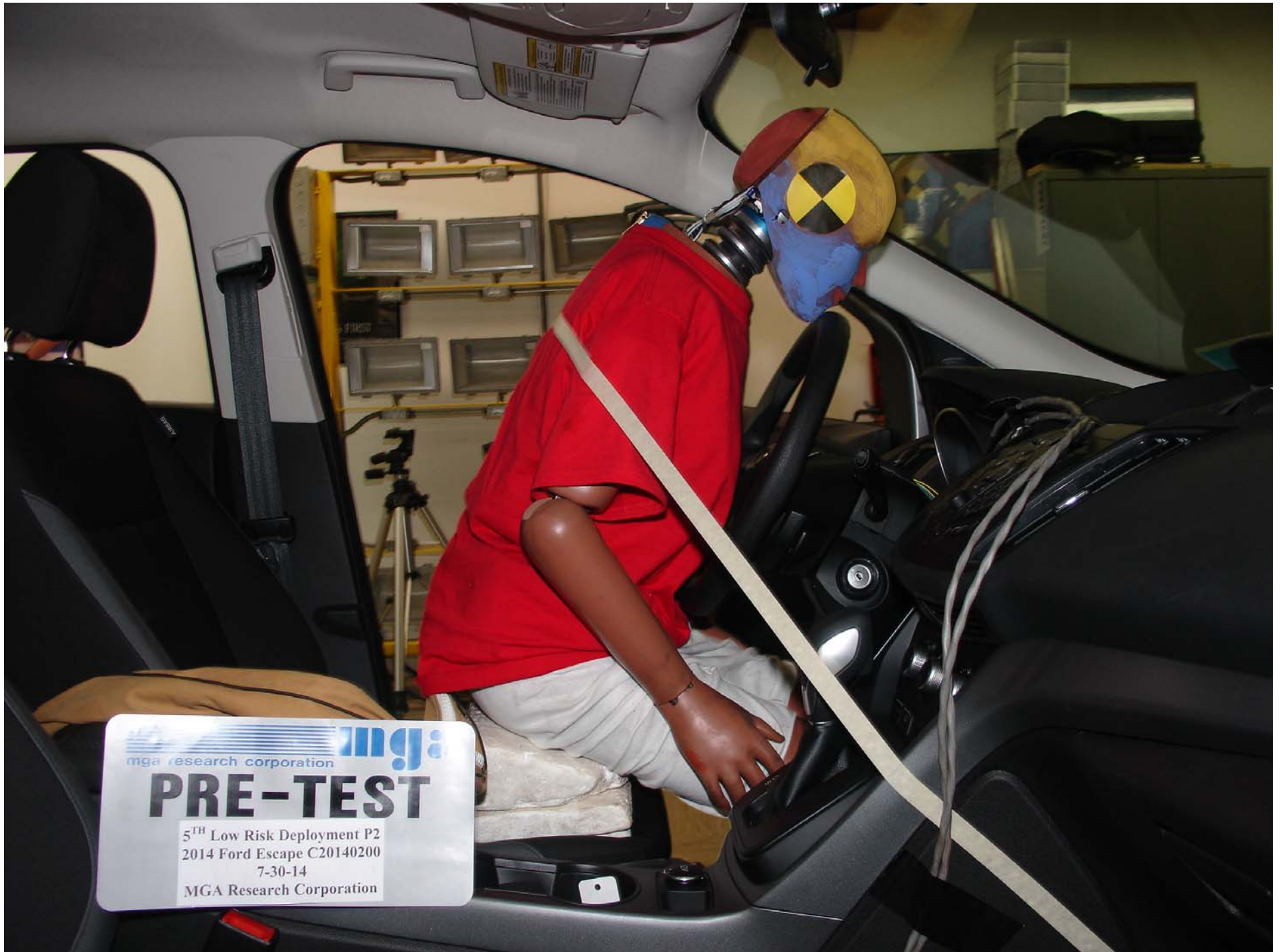
Photo No. 10 - Pre-Test 5th Fem. P2 Driver Dummy Right Side View
