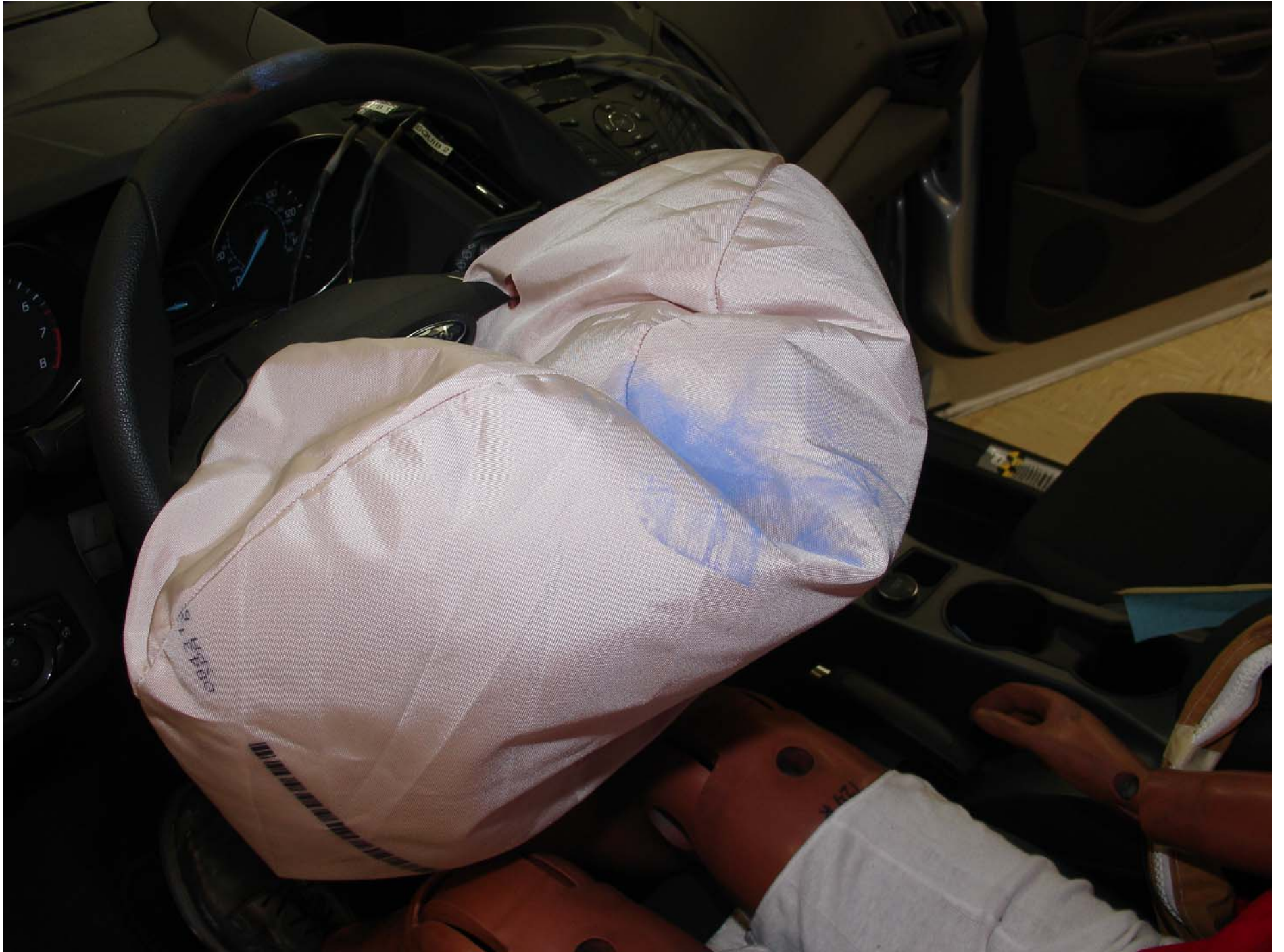
Photo No. 12 - Post-Test 5th Fem. P2 Driver Dummy Airbag Left Side View
