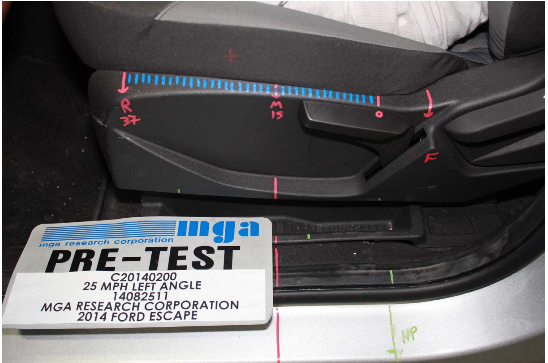
Photo No. 39 - Pre-Test Driver Dummy Seat Position
