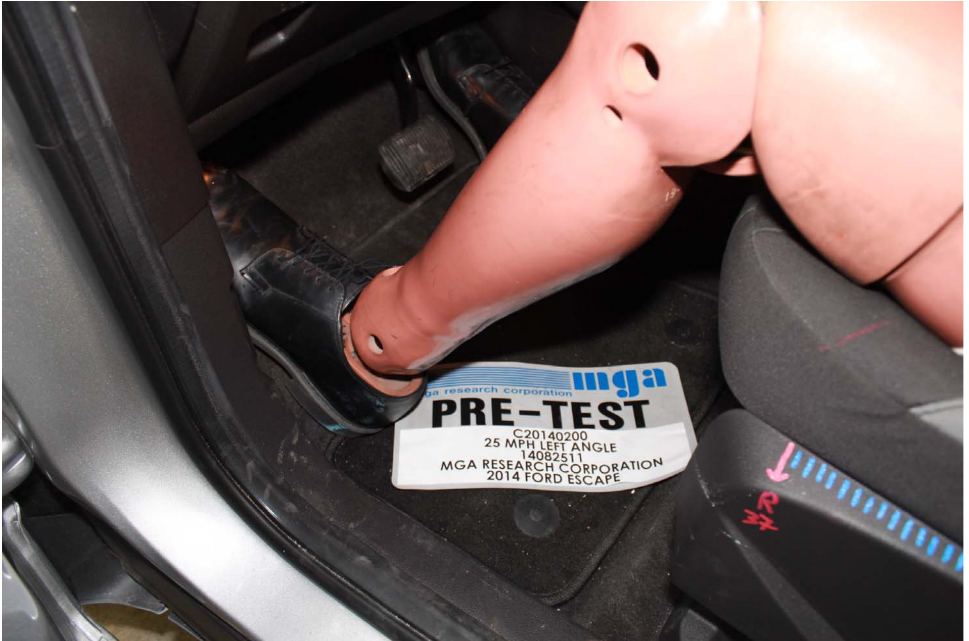
Photo No. 41 - Pre-Test Driver Dummy Feet Position
