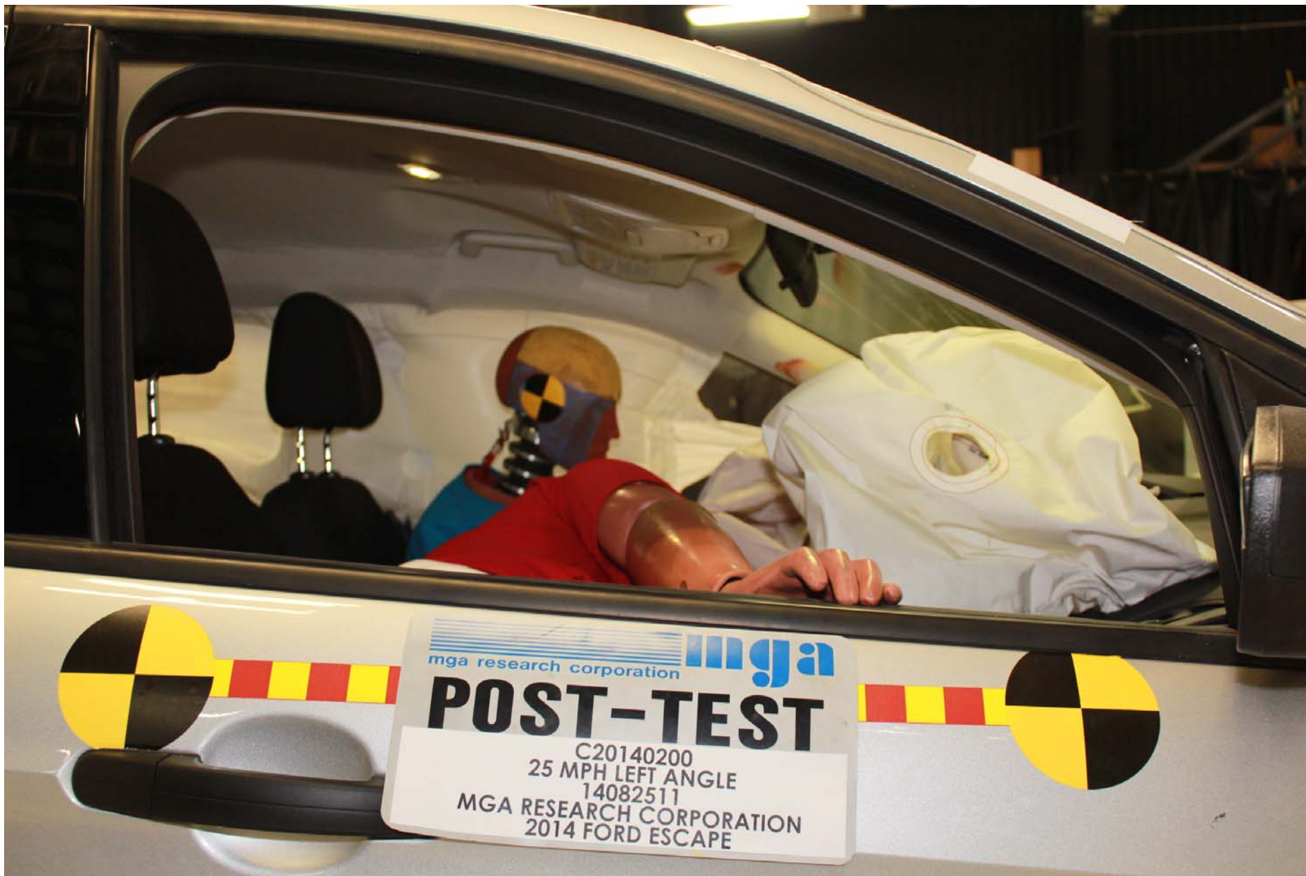
Photo No. 54 - Post-Test Passenger Dummy Position Right Side View
