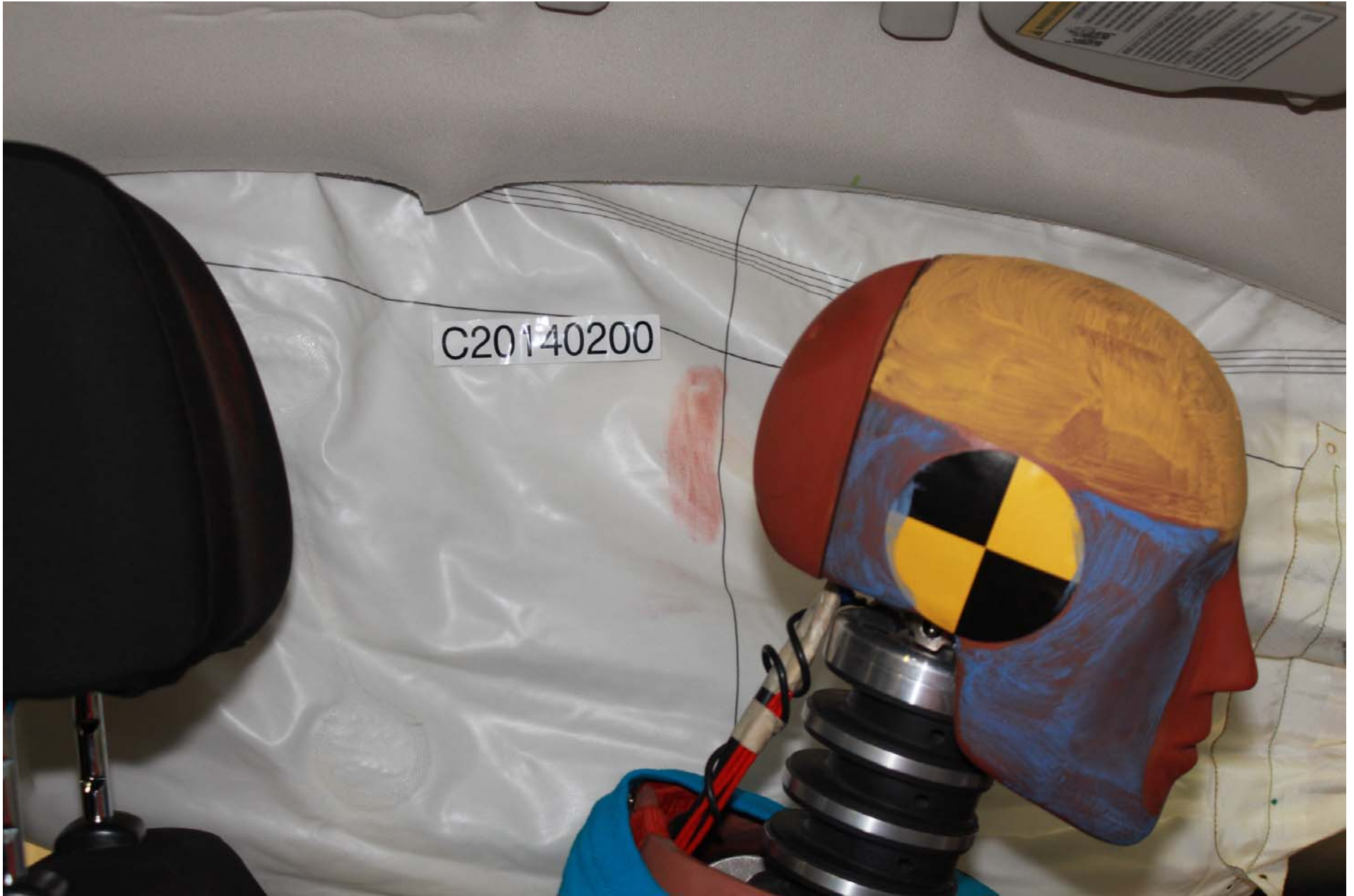
Photo No. 47 - Post-Test Driver Dummy Head Contact (curtain airbag)
