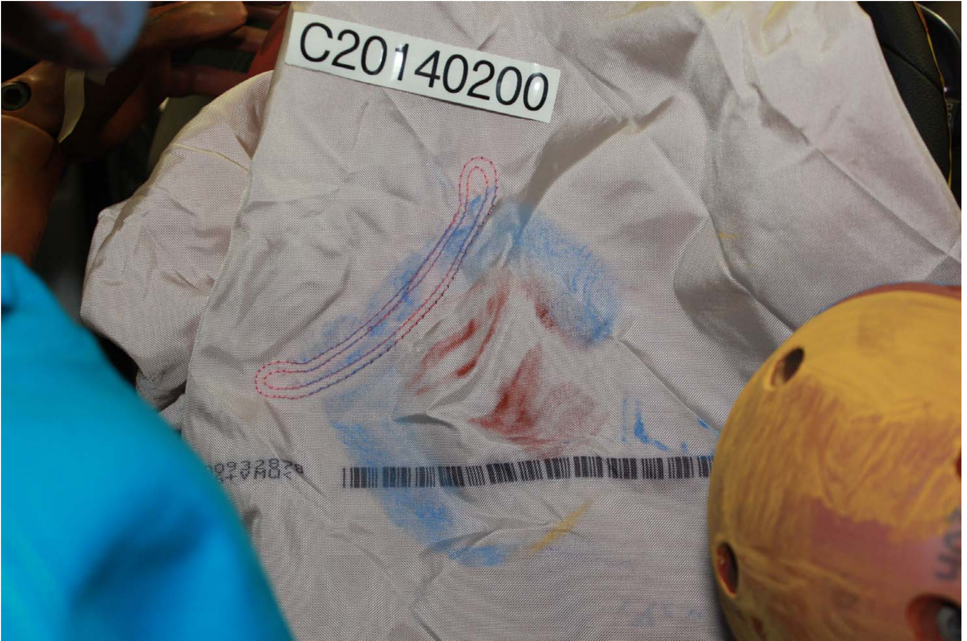
Photo No. 45 - Post-Test Driver Dummy Airbag Contact
