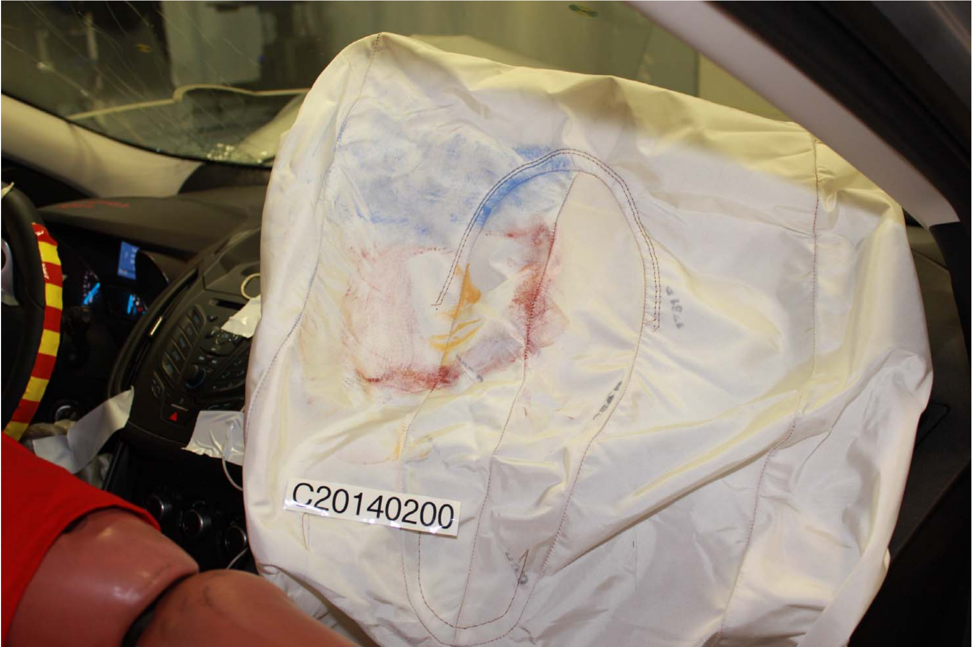
Photo No. 63 - Post-Test Passenger Dummy Airbag Contact
