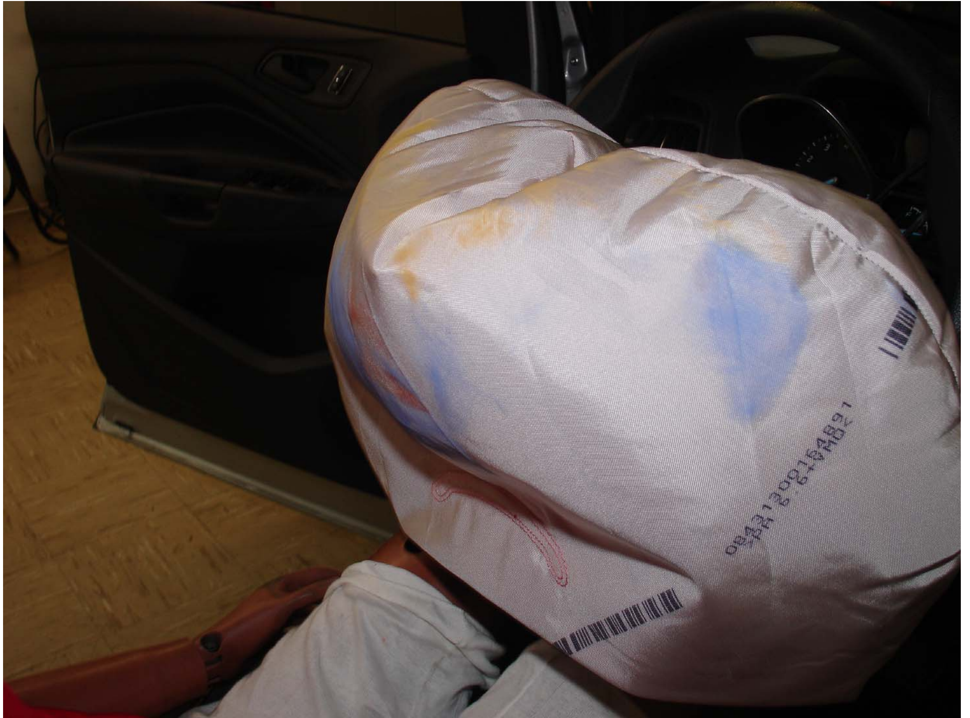
Photo No. 6 - Post-Test 5th Fem. P1 Driver Dummy Airbag Right Side View
