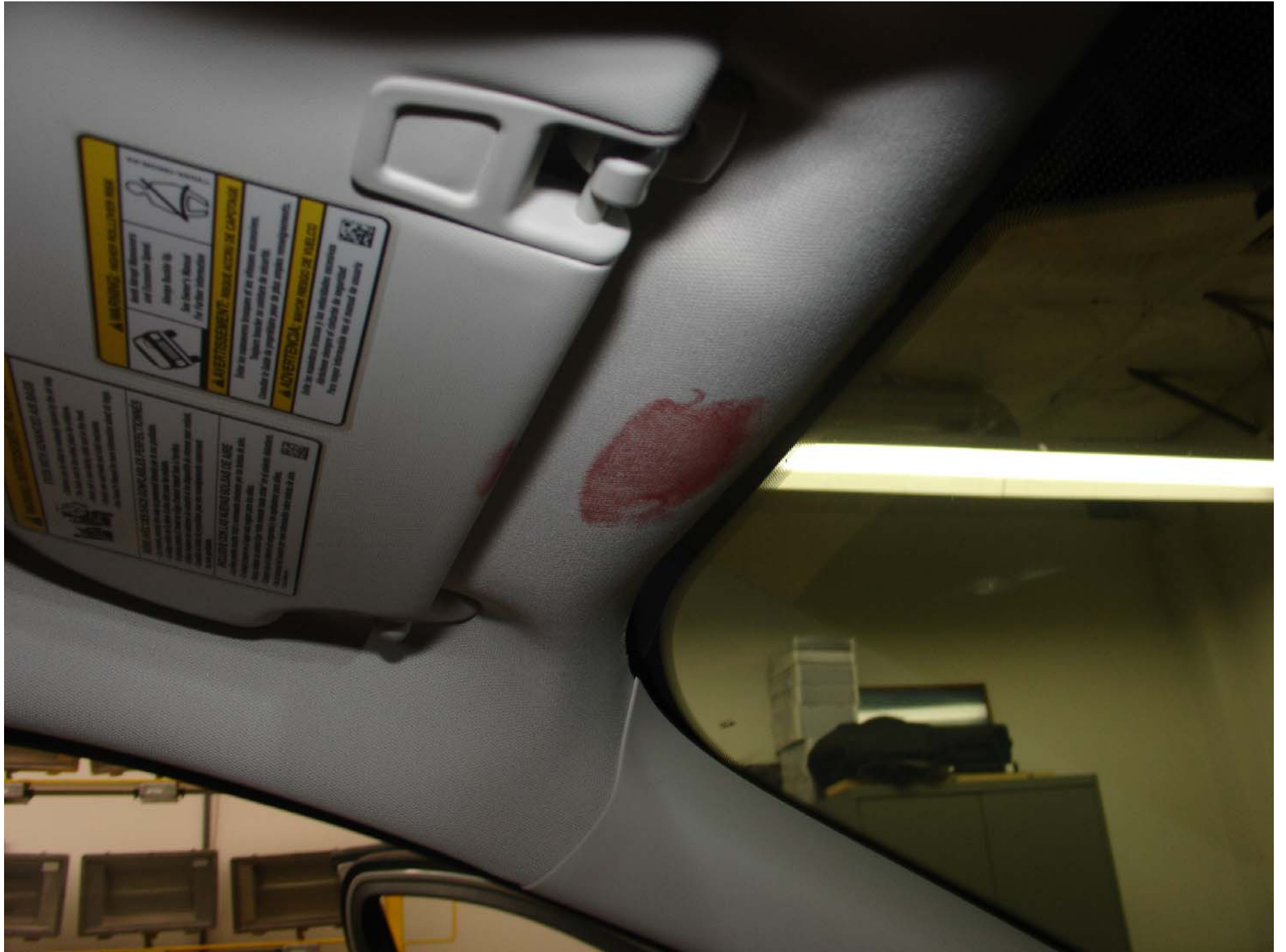
Photo No. 15 - Post-Test 5th Fem. P2 Driver Dummy Head Contact (headliner-visor)
