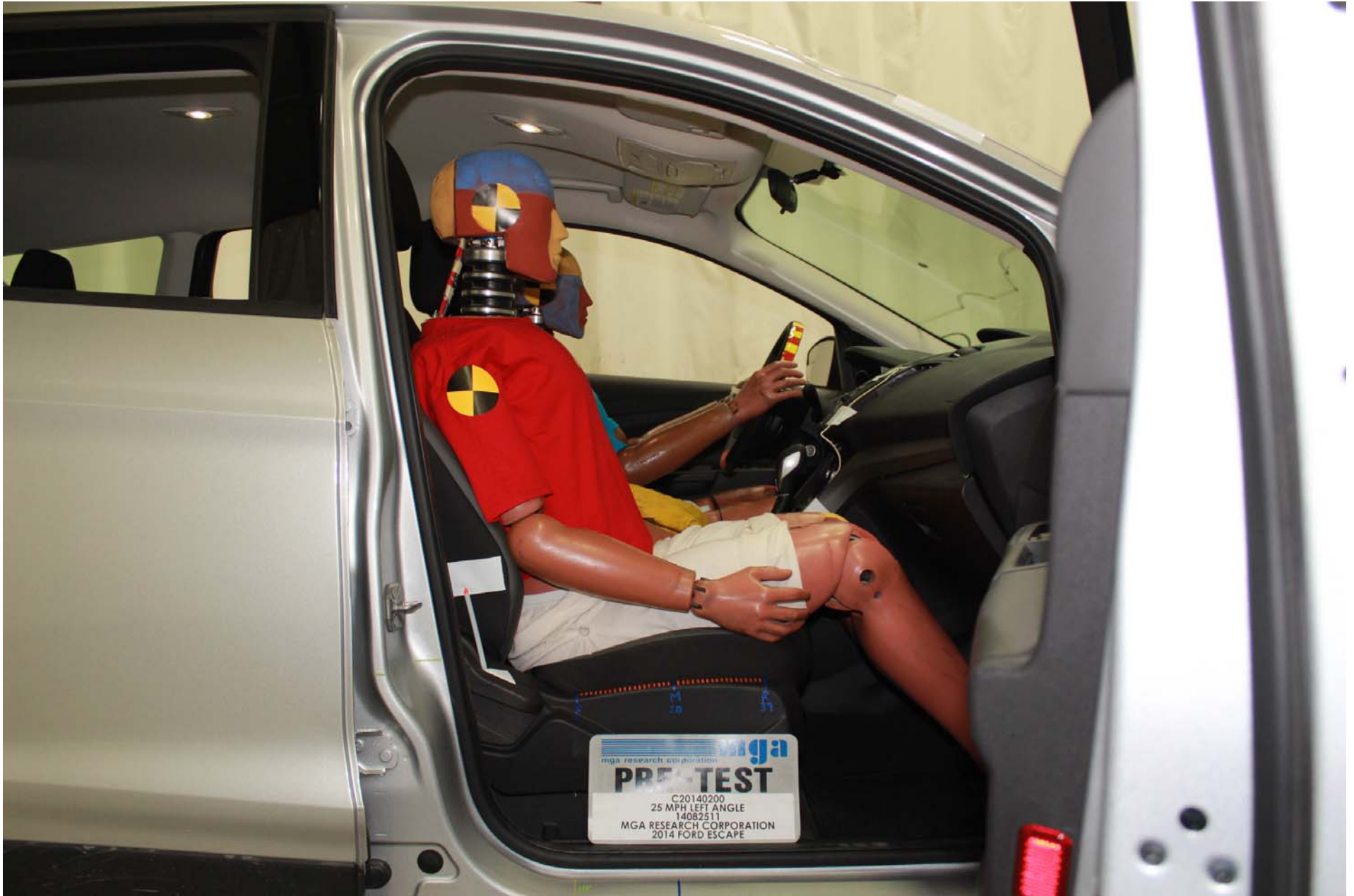
Photo No. 55 - Pre-Test Passenger Dummy Position Right Side View (door open)
