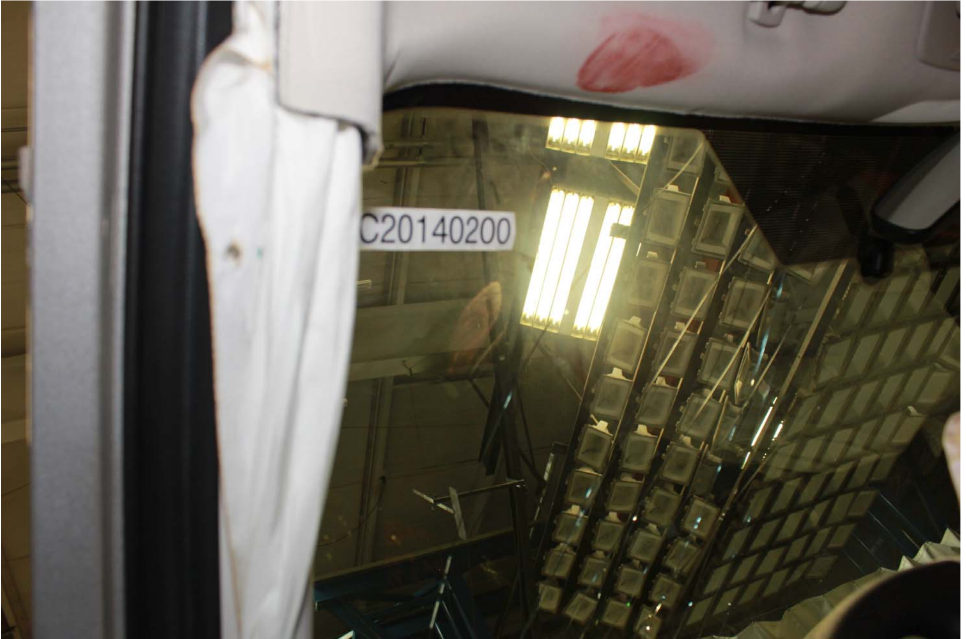
Photo No. 49 - Post-Test Driver Dummy Head Contact (windshield)
