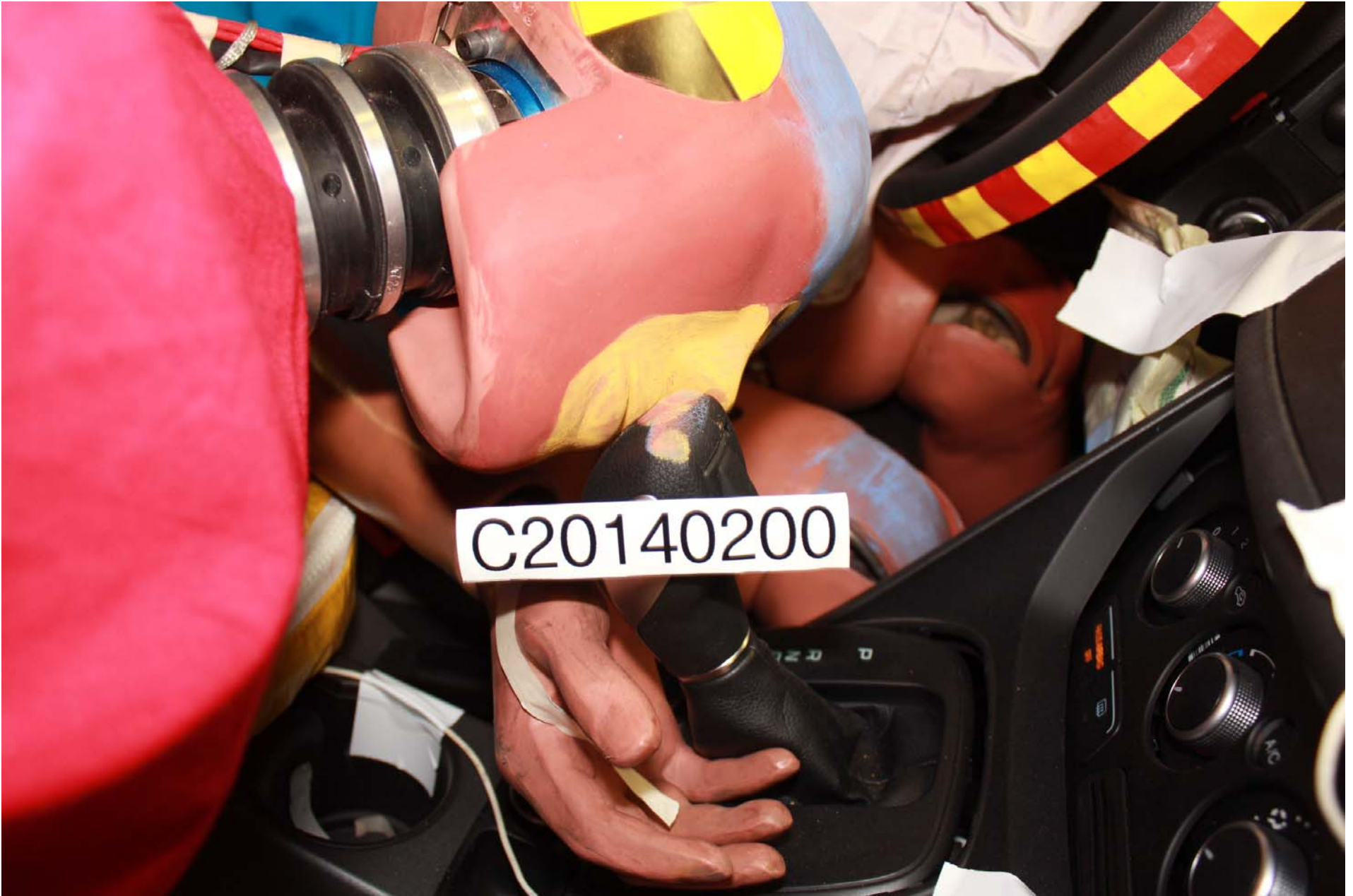
Photo No. 65 - Post-Test Passenger Dummy Head Contact (shifter)
