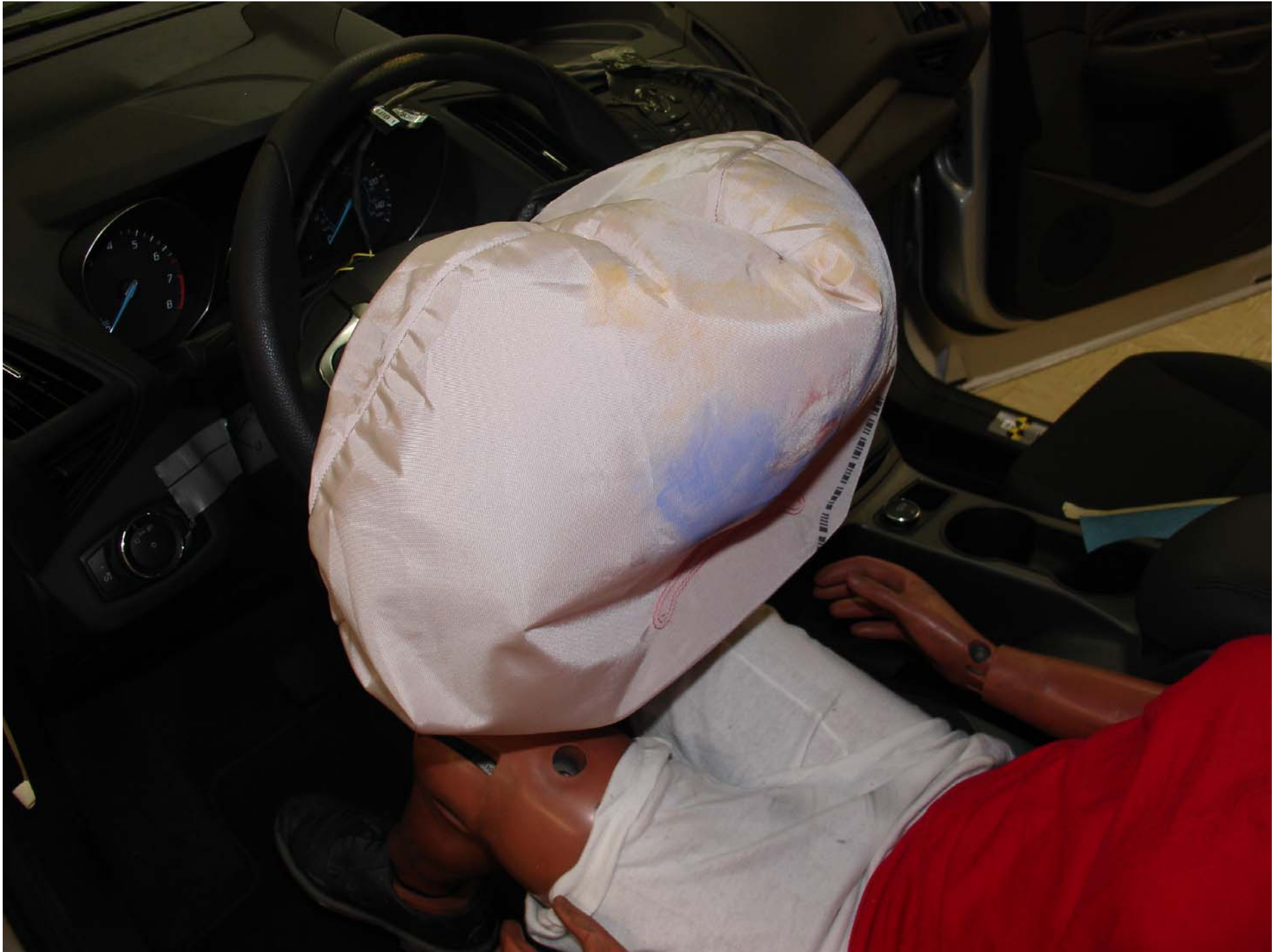
Photo No. 5 - Post-Test 5th Fem. P1 Driver Dummy Airbag Left Side View
