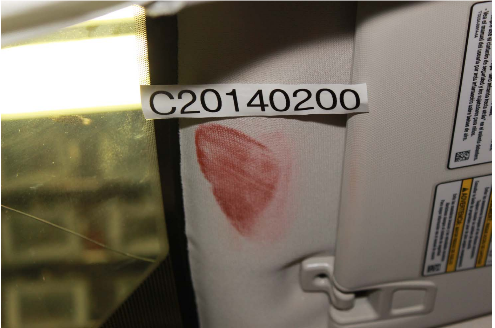
Photo No. 50 - Post-Test Driver Dummy Head Contact (headliner)
