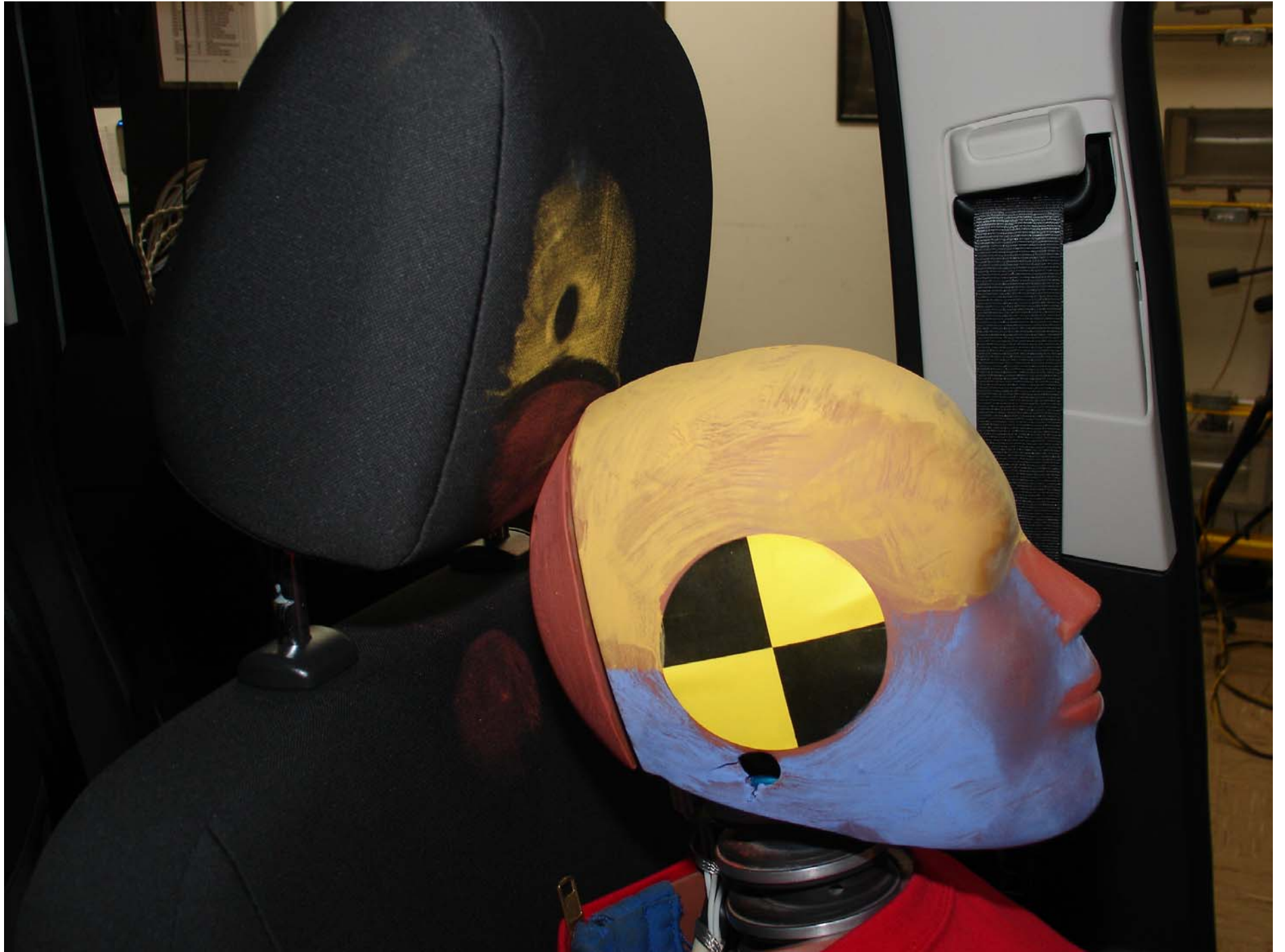
Photo No. 7 - Post-Test 5th Fem. P1 Driver Dummy Head Contact (headrest-seat back)
