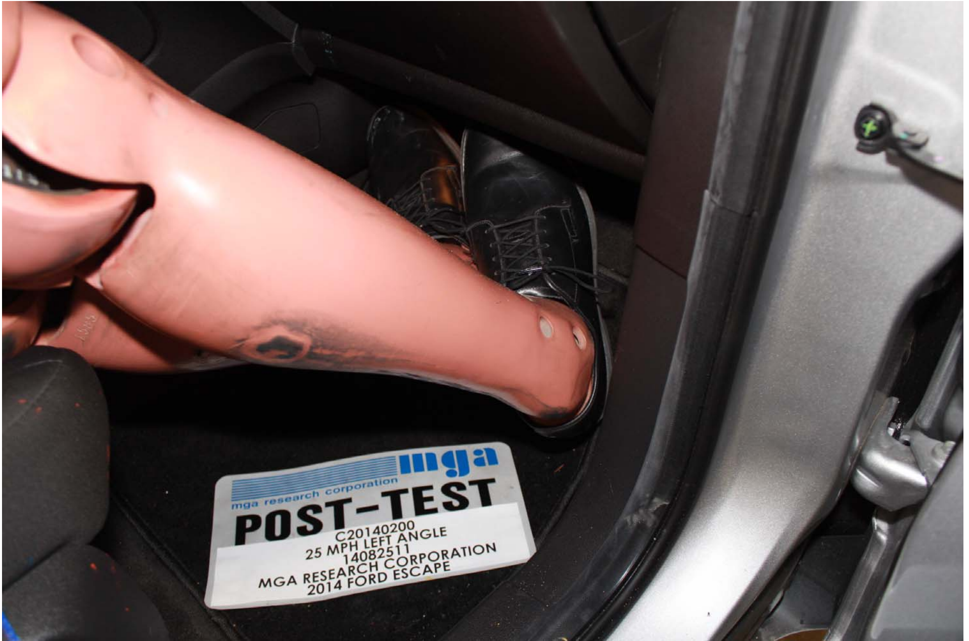
Photo No. 60 - Post-Test Passenger Dummy Feet Position
