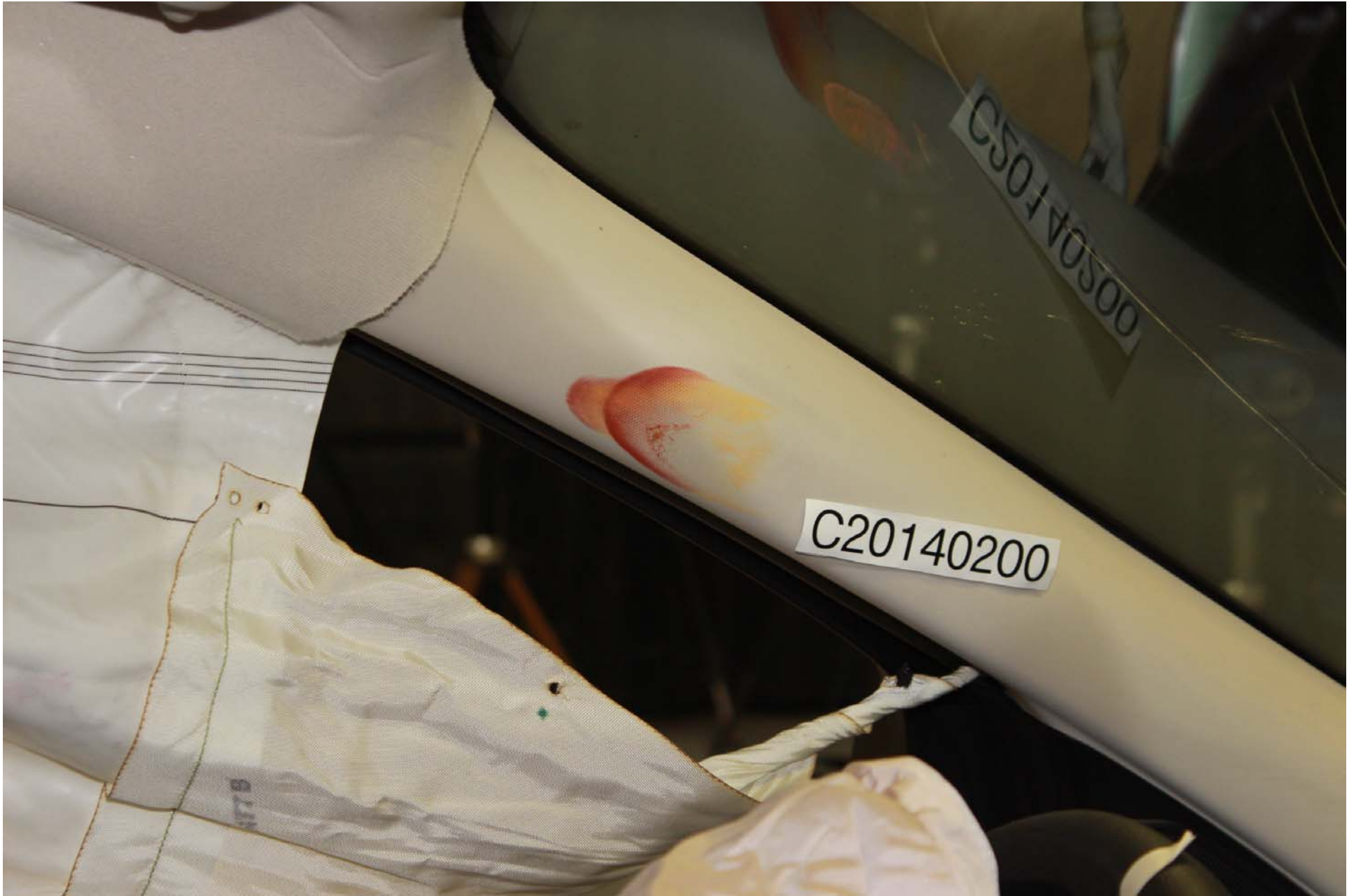
Photo No. 48 - Post-Test Driver Dummy Head Contact (A-pillar)
