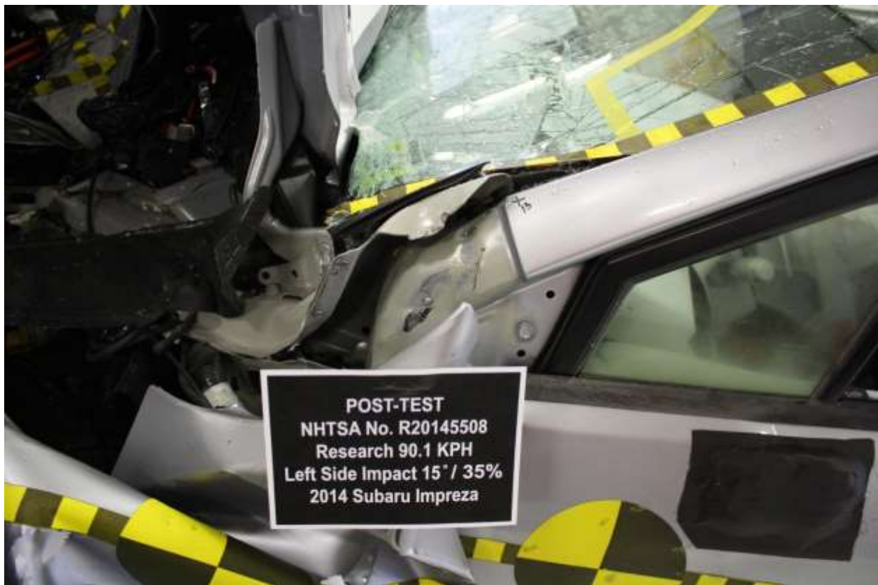
No. 161 Post-Test View of Windshield Separation
