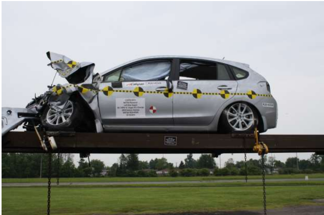
No. 184 Vehicle at 360 Degrees on Static Rollover Device
