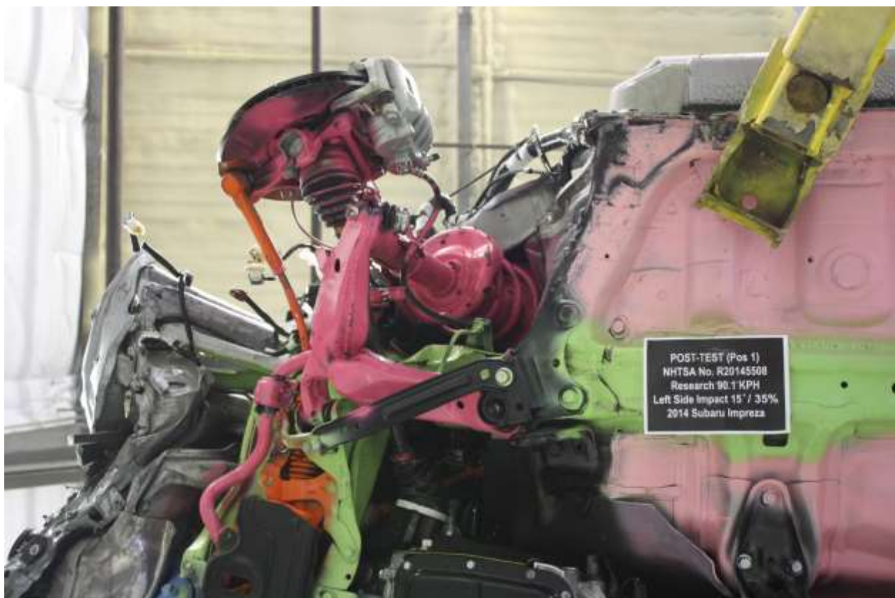
No. 141 Post-Test Frame Rail with tire removed
