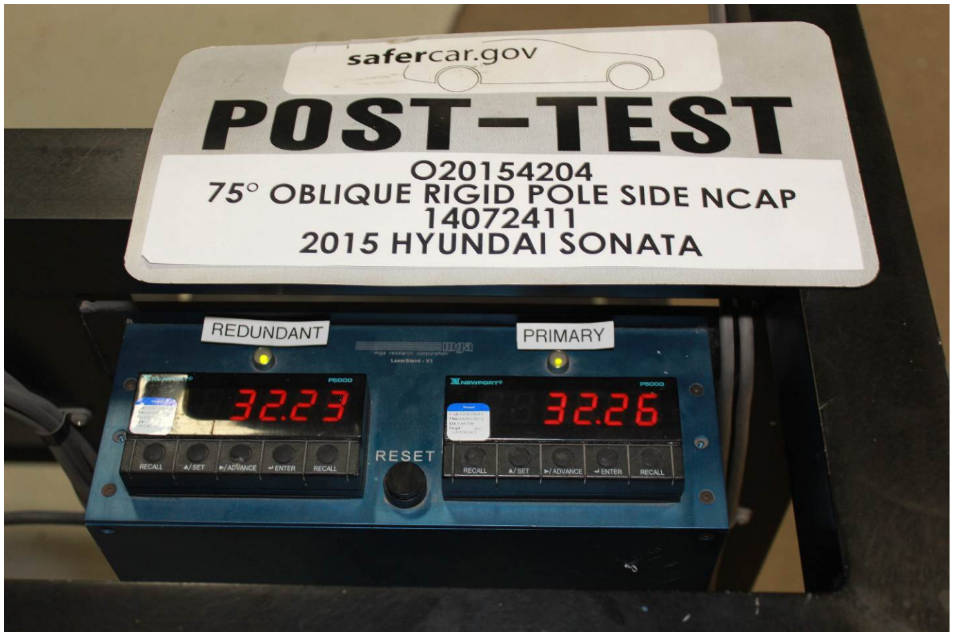
Post-Test Primary and Redundant Speed Trap Read-Out
