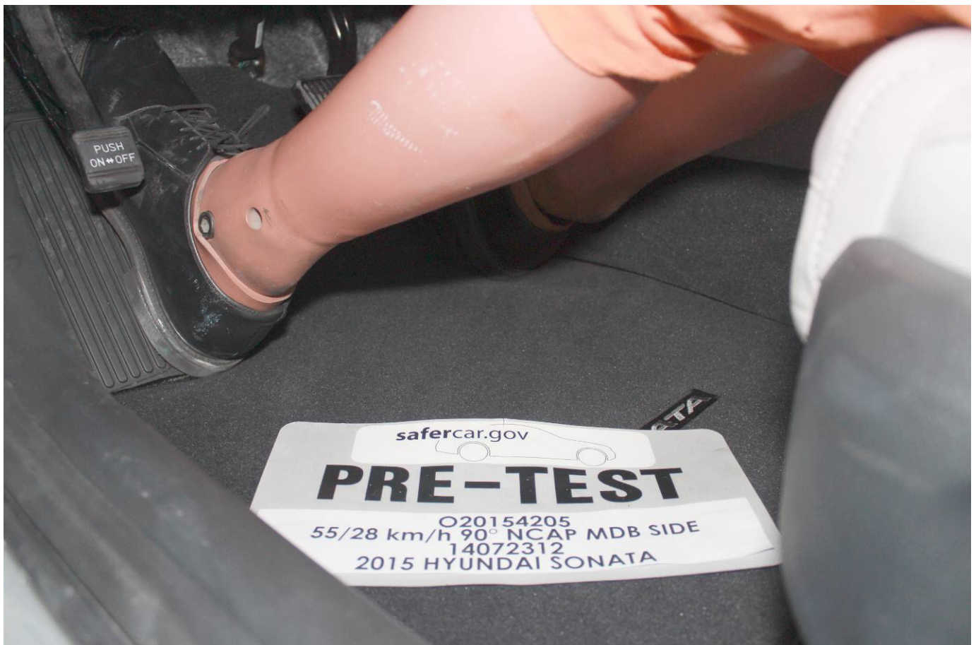
Pre-Test Placement of Driver Dummy's Feet
