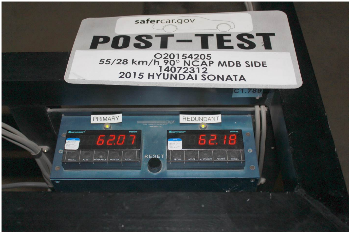
Post-Test Primary and Redundant Speed Trap Read-Out
