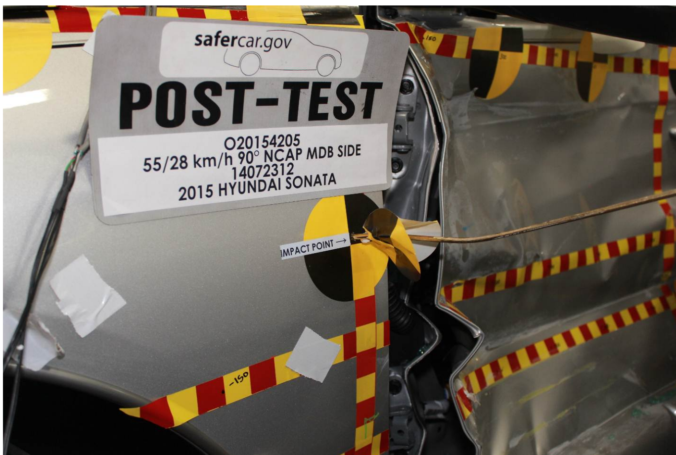
Post-Test Close-Up View of Impact Point Target
