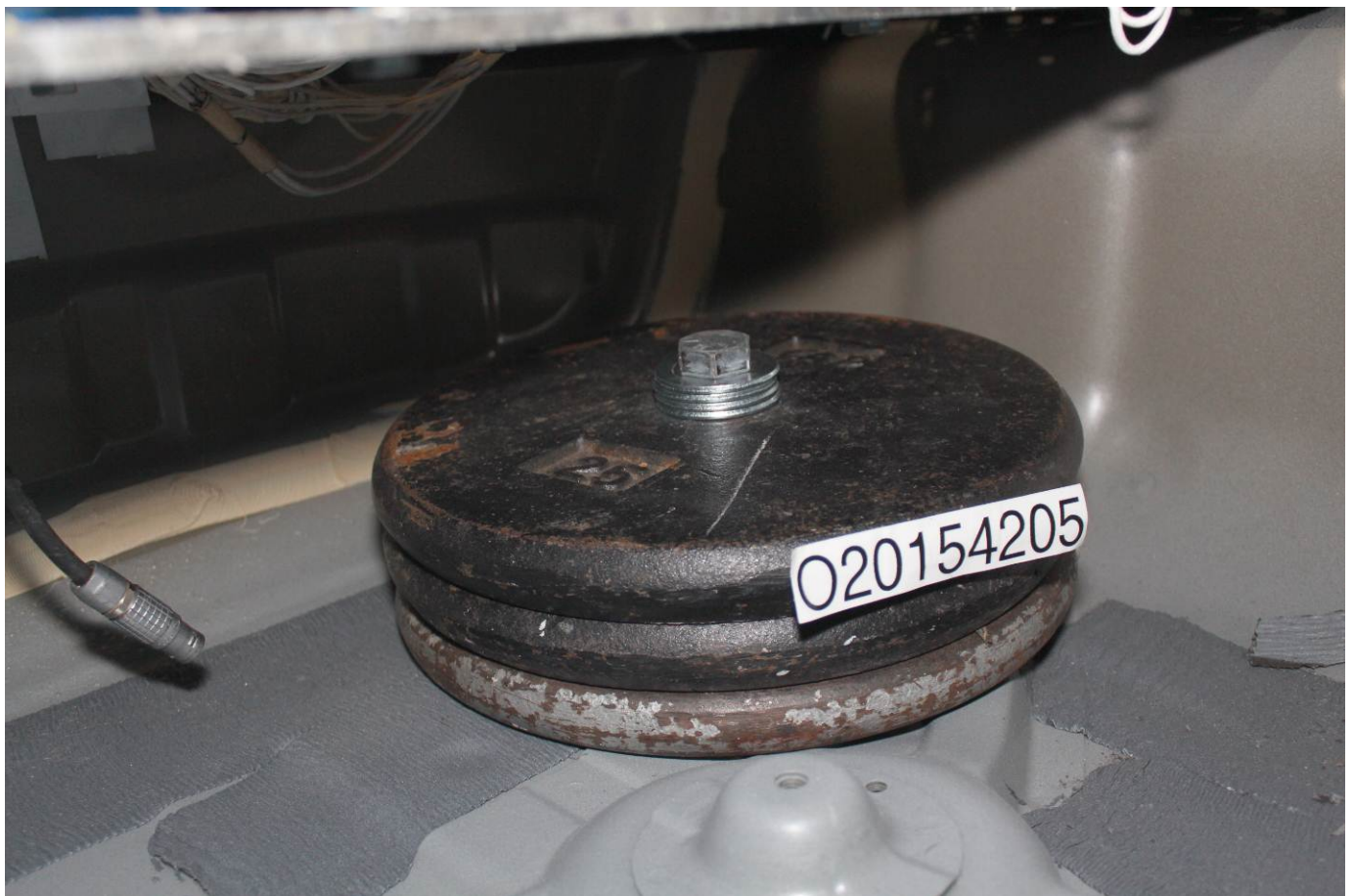
Pre-Test Ballast View
