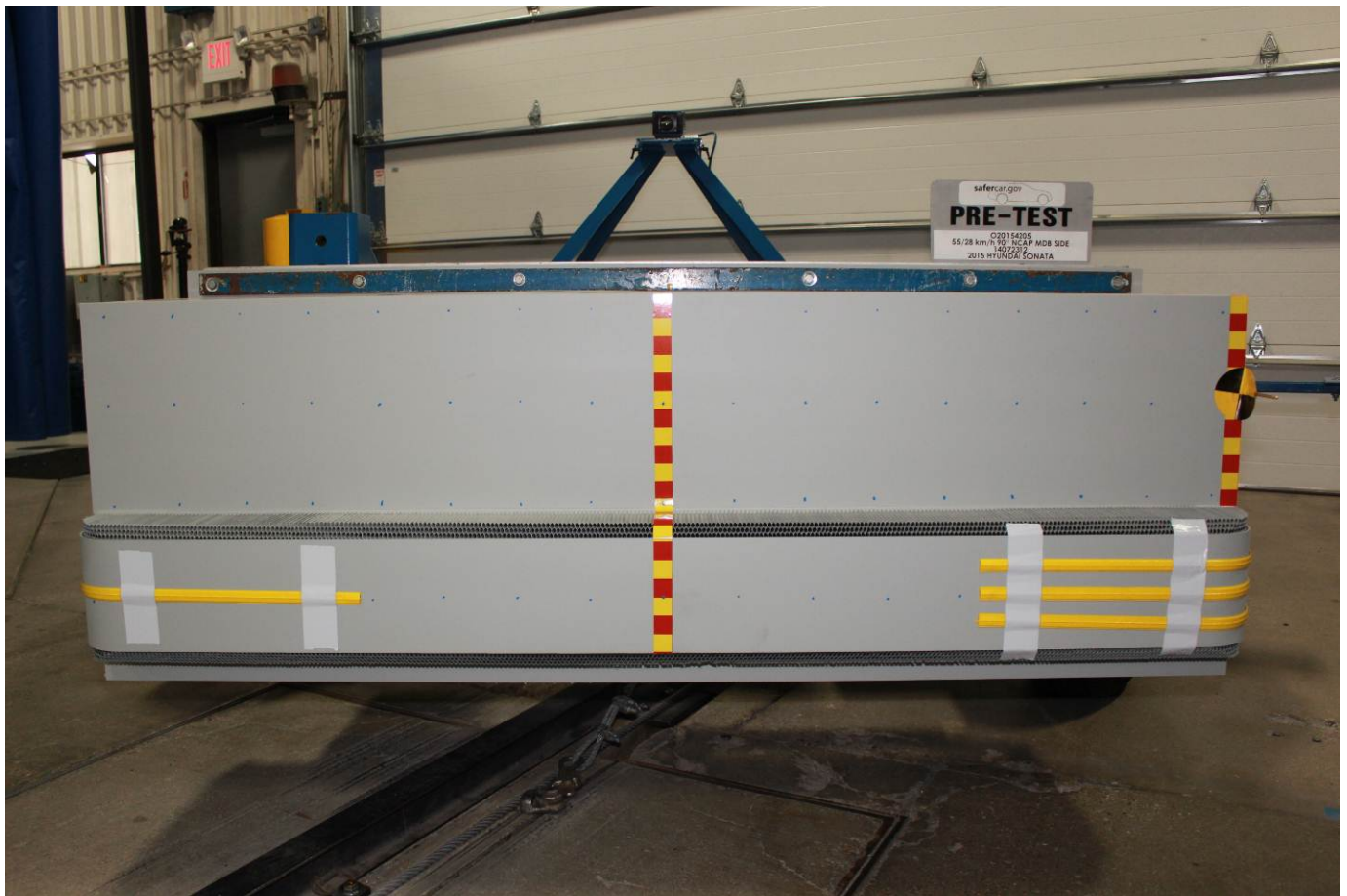
Pre-Test Front View of MDB Impactor Face
