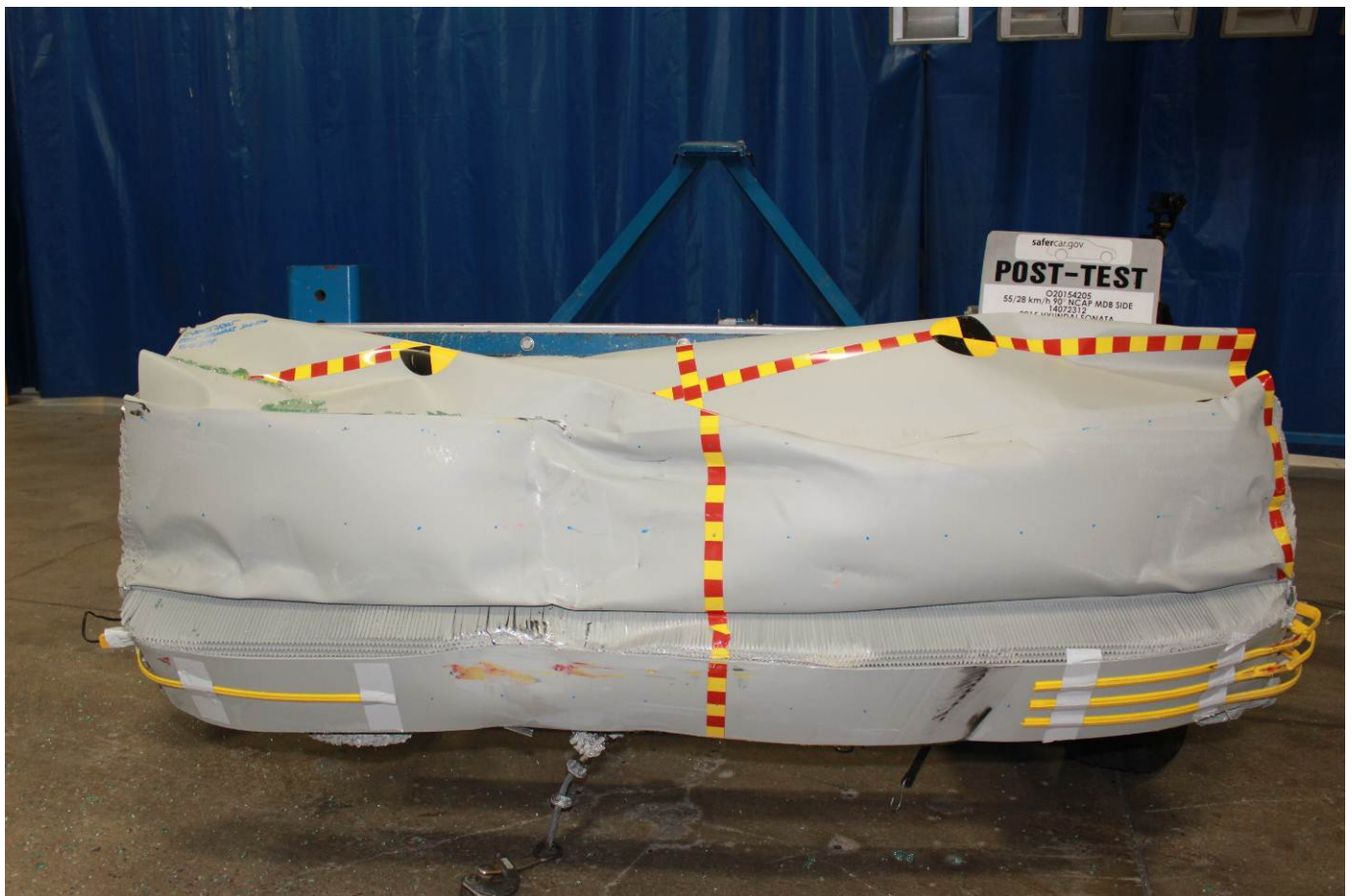
Post-Test Front View of MDB Impactor Face
