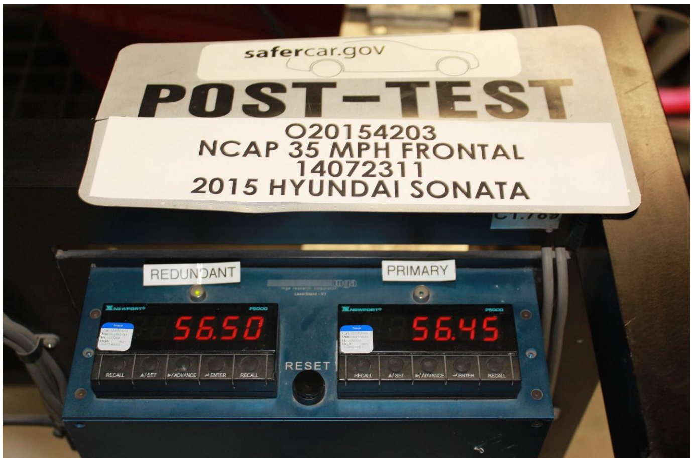
Post-Test Speed Trap Read-Out
