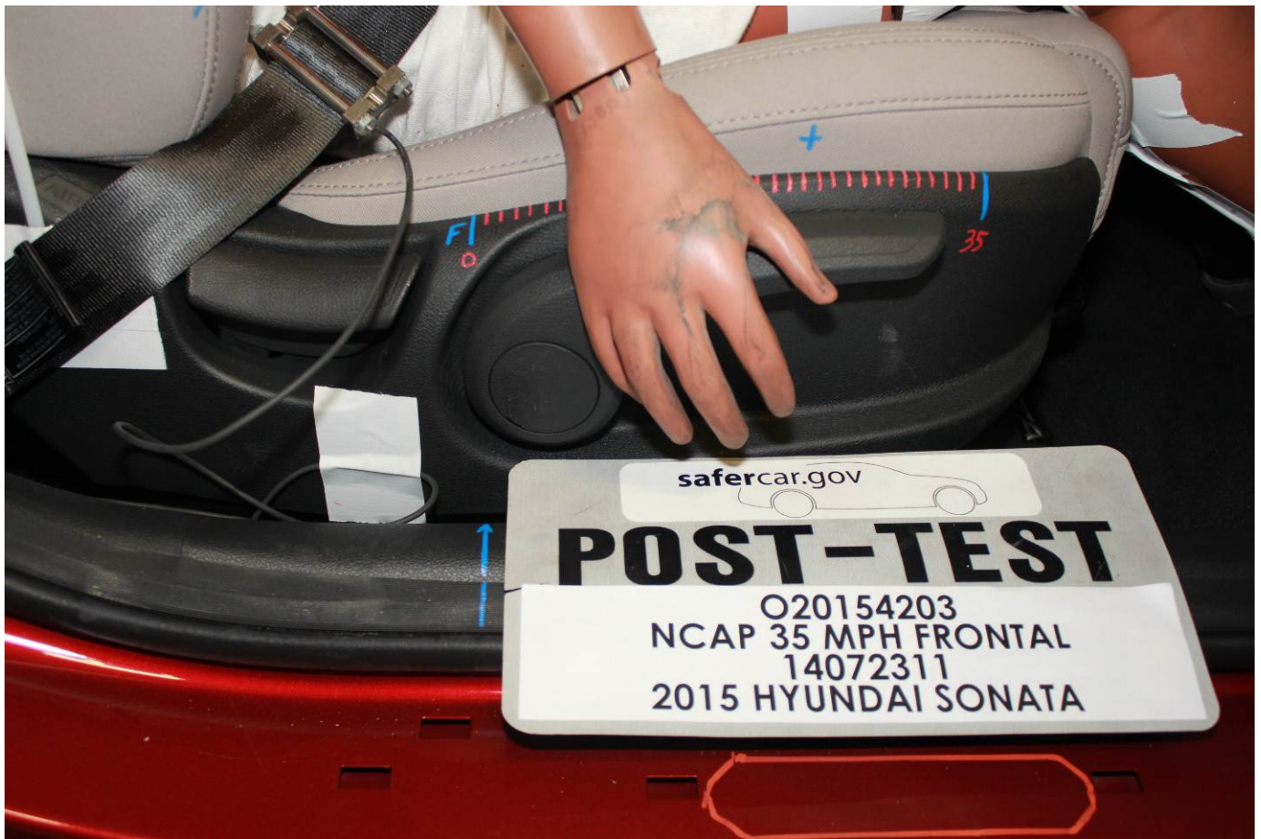
Post-Test Passenger's Seat Fore-Aft Markings
