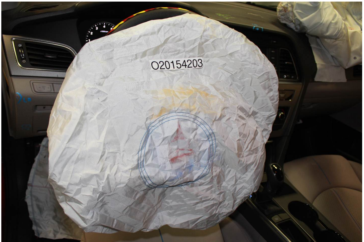
Post-Test Driver Dummy Contact with Airbag
