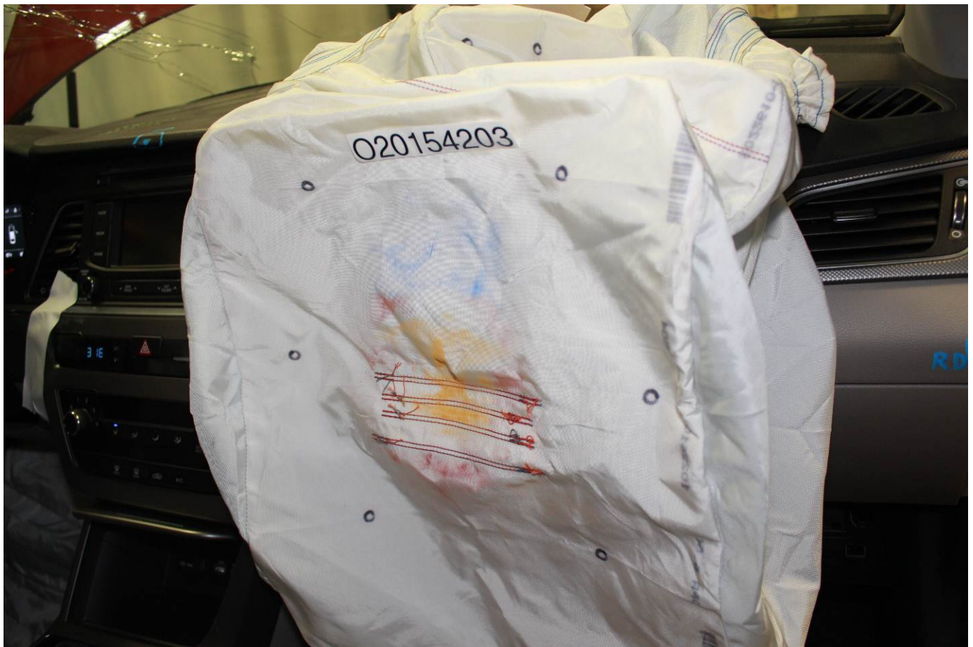
Post-Test Passenger Dummy Contact with Airbag
