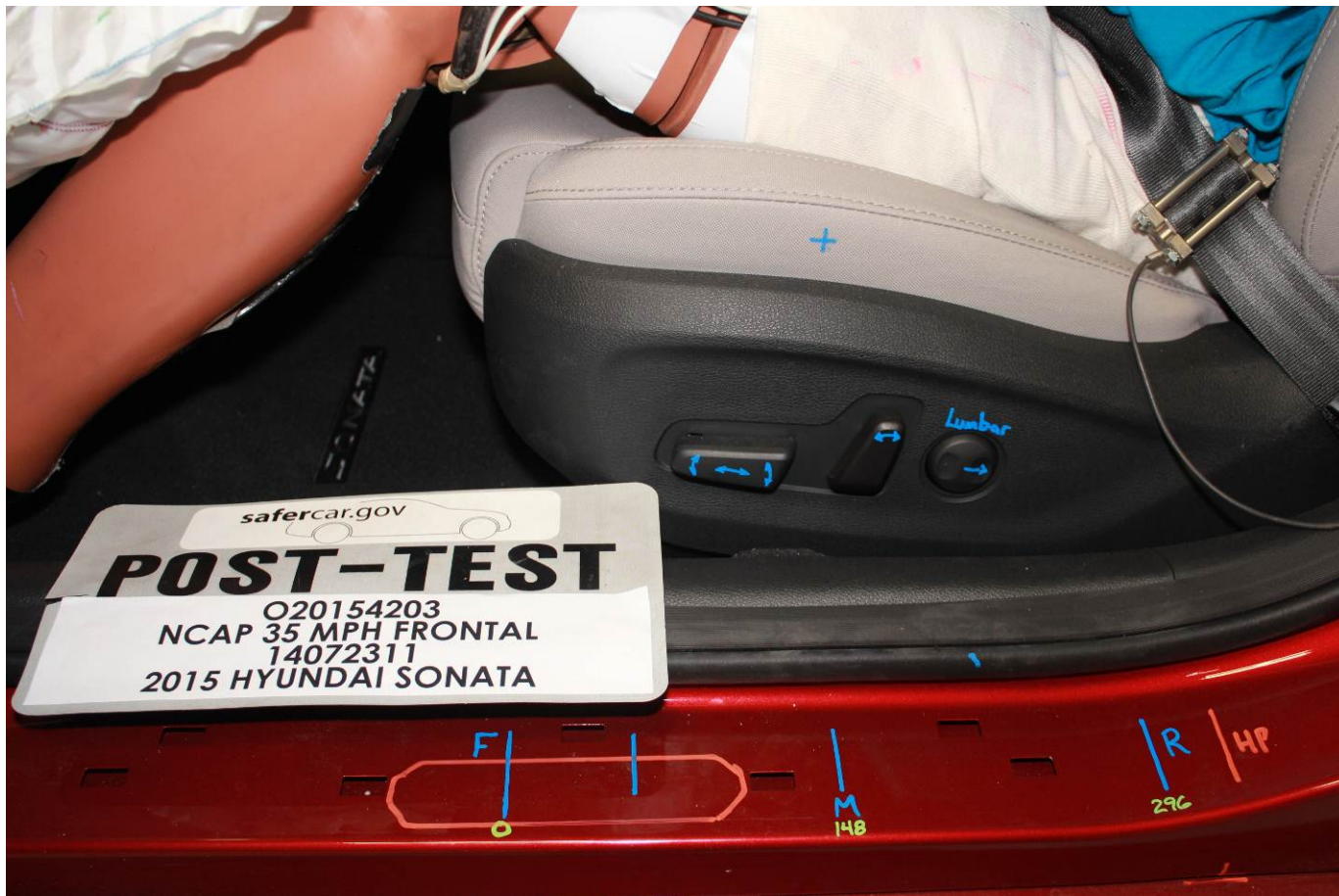
Post-Test Driver's Seat Fore-Aft Markings
