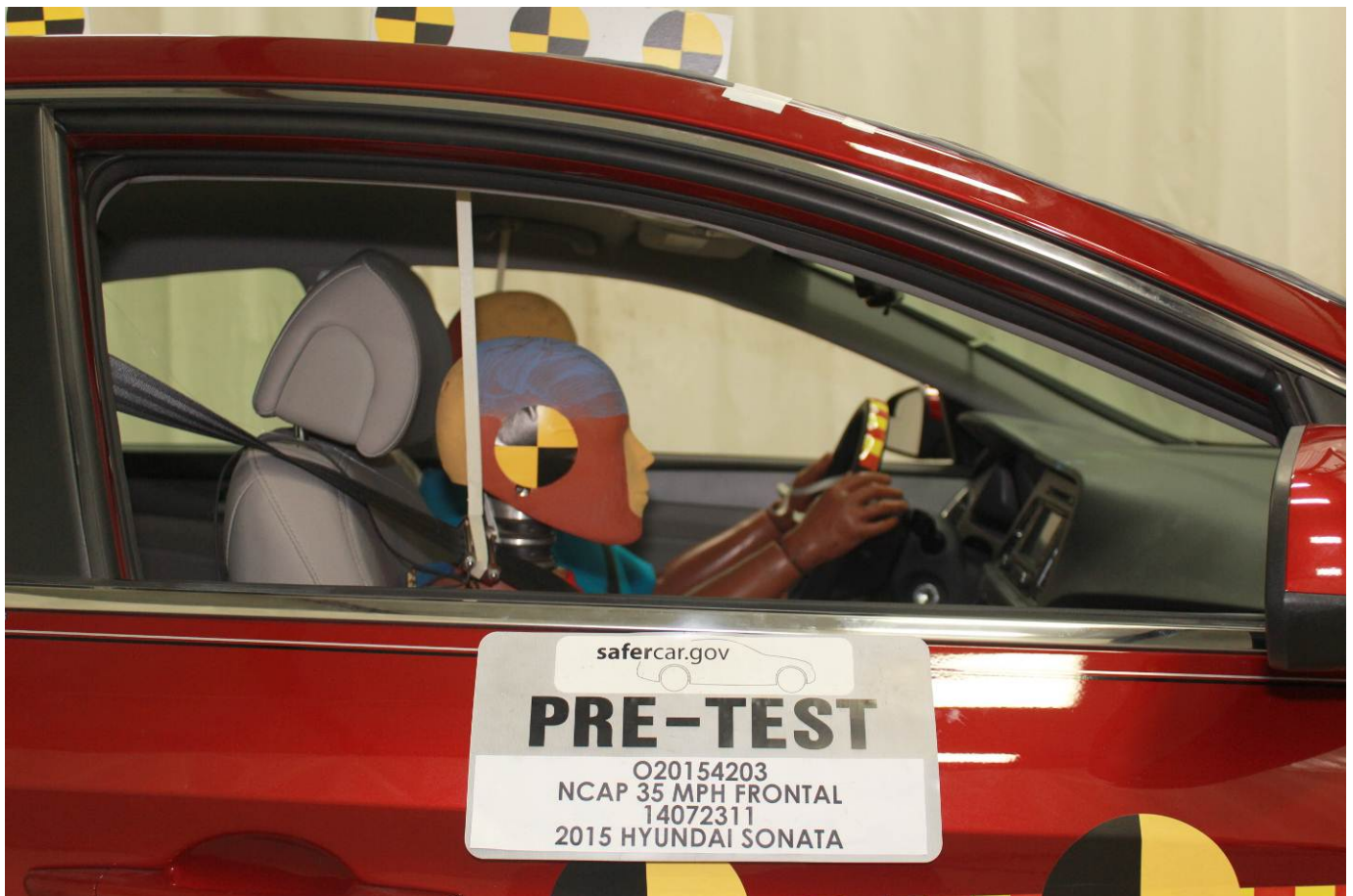
Pre-Test Passenger Dummy Window View
