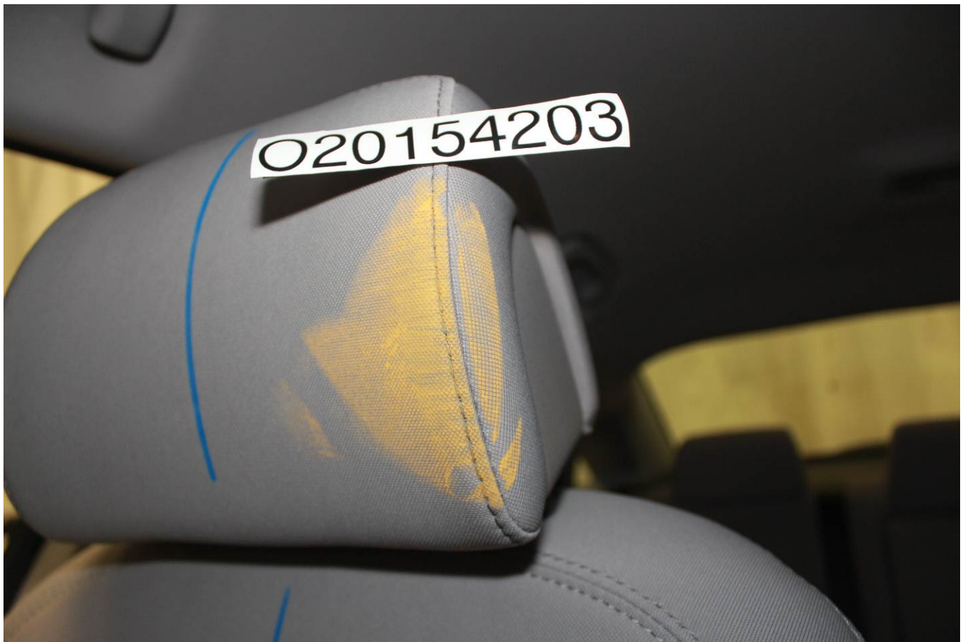
Post-Test Passenger Dummy Contact with Headrest
