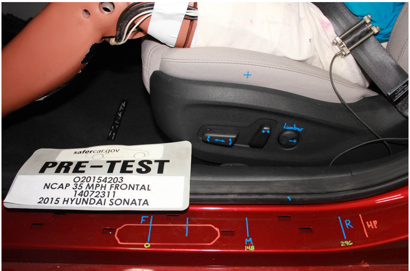
Pre-Test Driver's Seat Fore-Aft Markings
