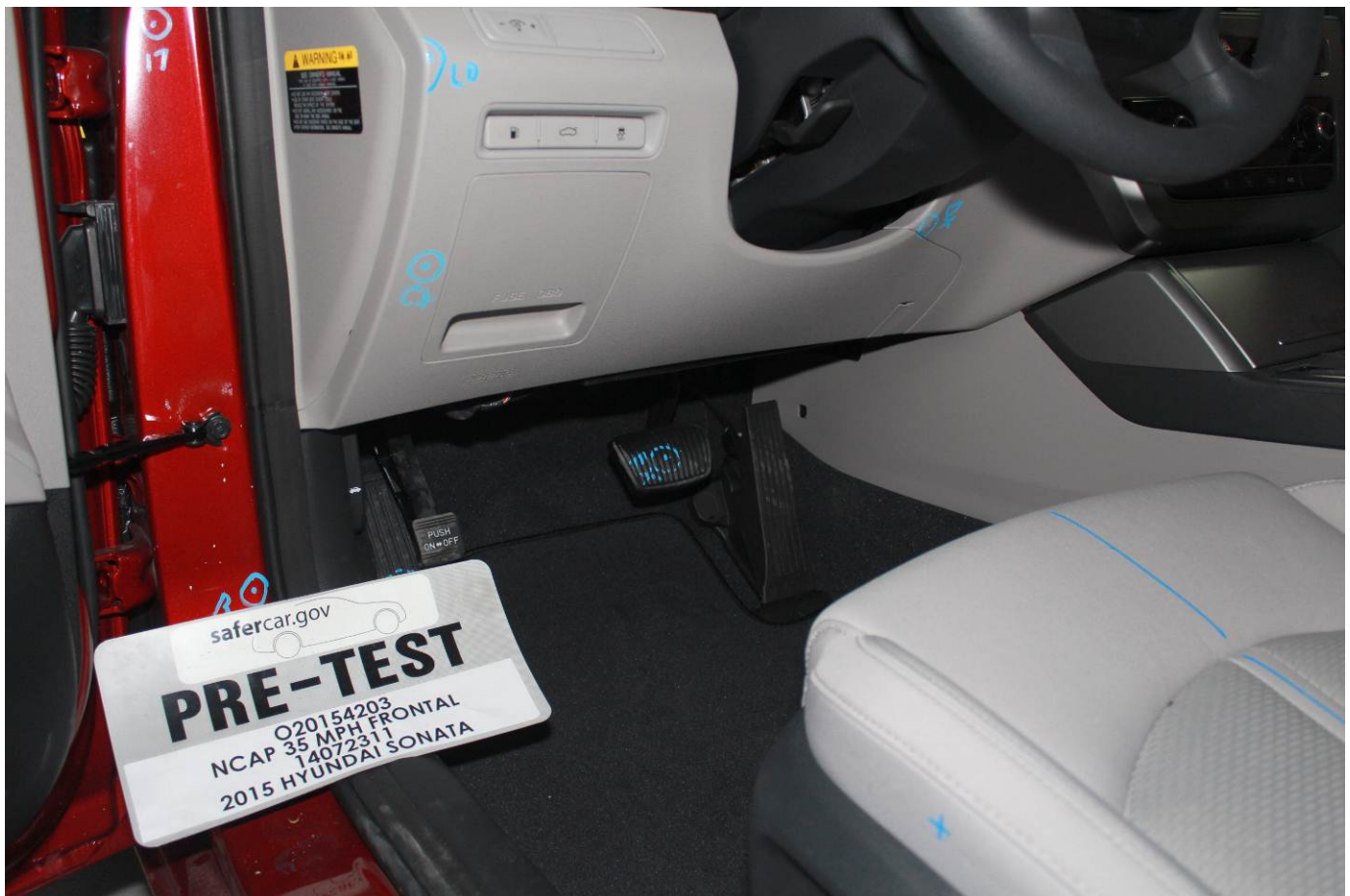
Pre-Test Driver's Side Knee Bolster (without dummy)
