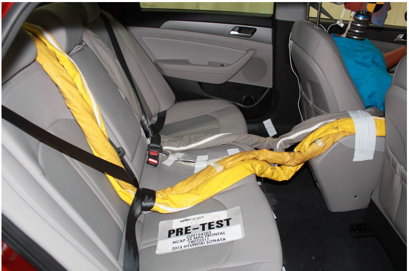
Pre-Test Dummy Cable Routing
