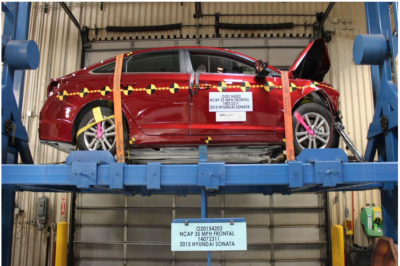
Vehicle at 360 Degrees on Static Rollover Device
