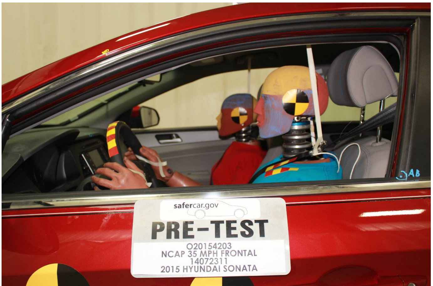
Pre-Test Driver Dummy Window View
