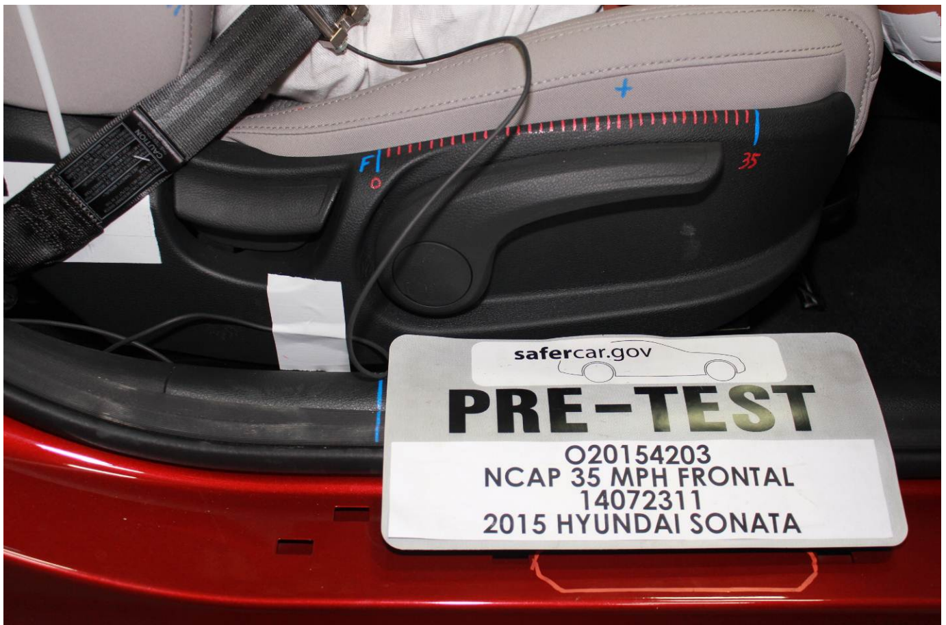
Pre-Test Passenger's Seat Fore-Aft Markings
