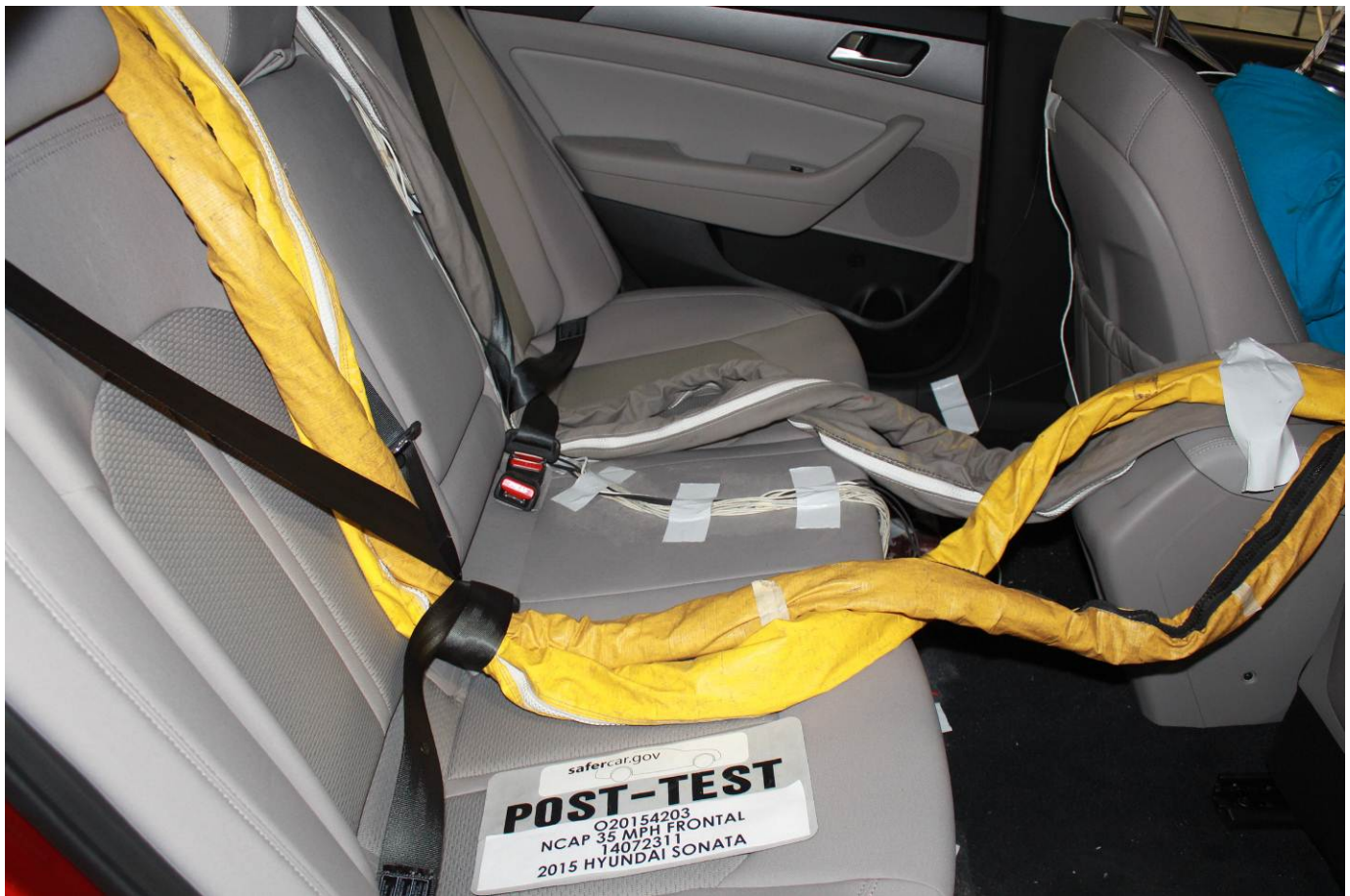
Post-Test Dummy Cable Routing
