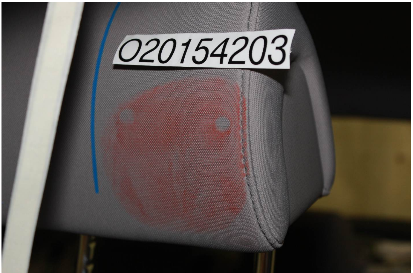
Post-Test Driver Dummy Contact with Headrest
