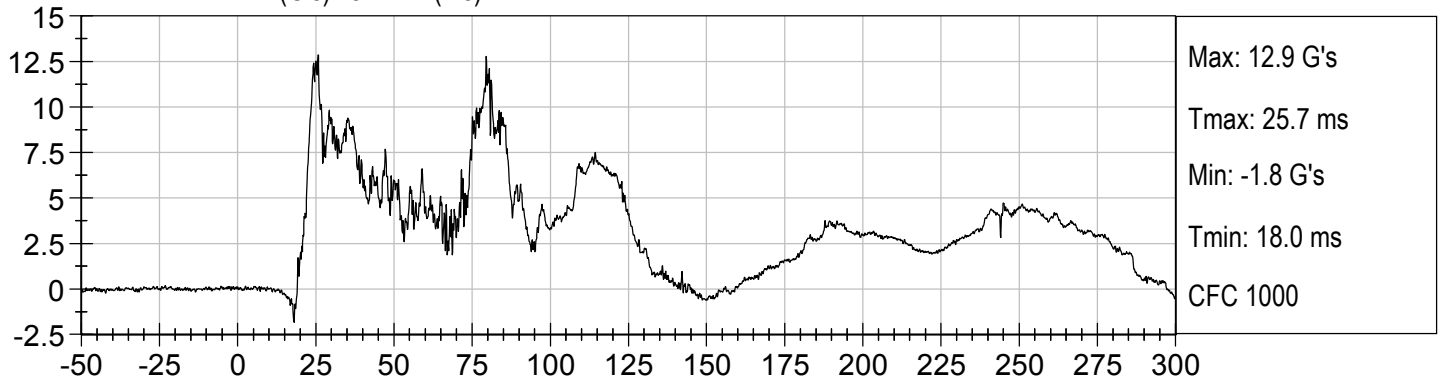
DRIVER HEAD Resultant (G's) vs TIME (ms)
