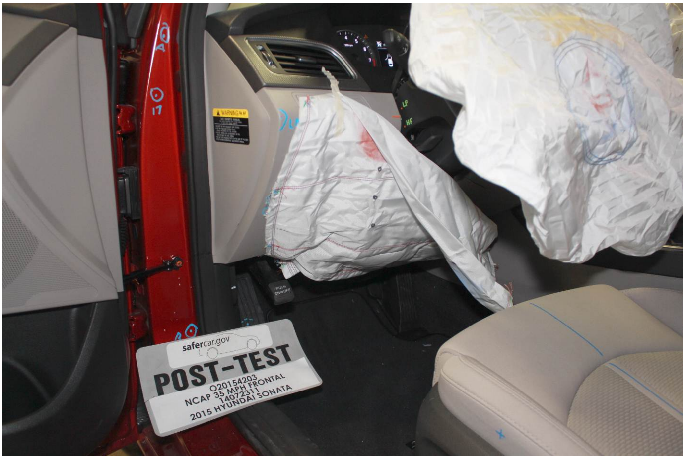
Post-Test Driver's Side Knee Bolster (without dummy)
