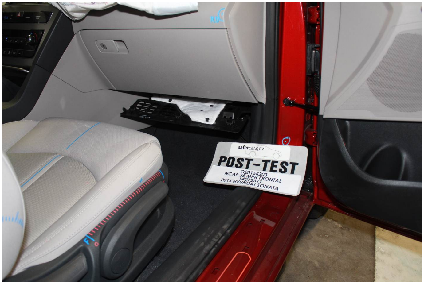
Post-Test Passenger's Side Knee Bolster (without dummy)
