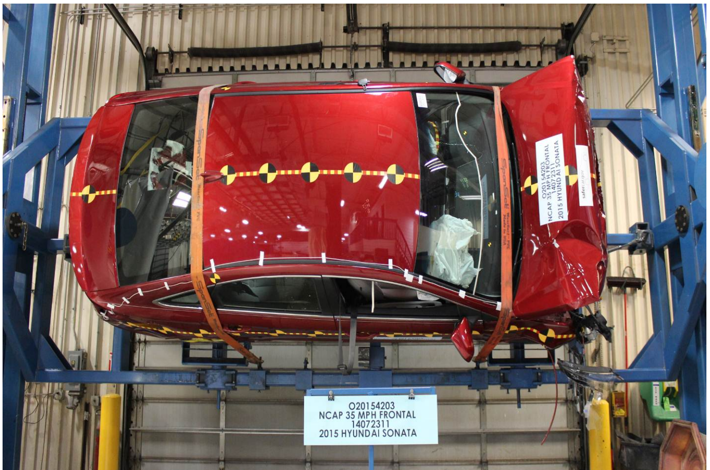
Vehicle at 270 Degrees on Static Rollover Device
