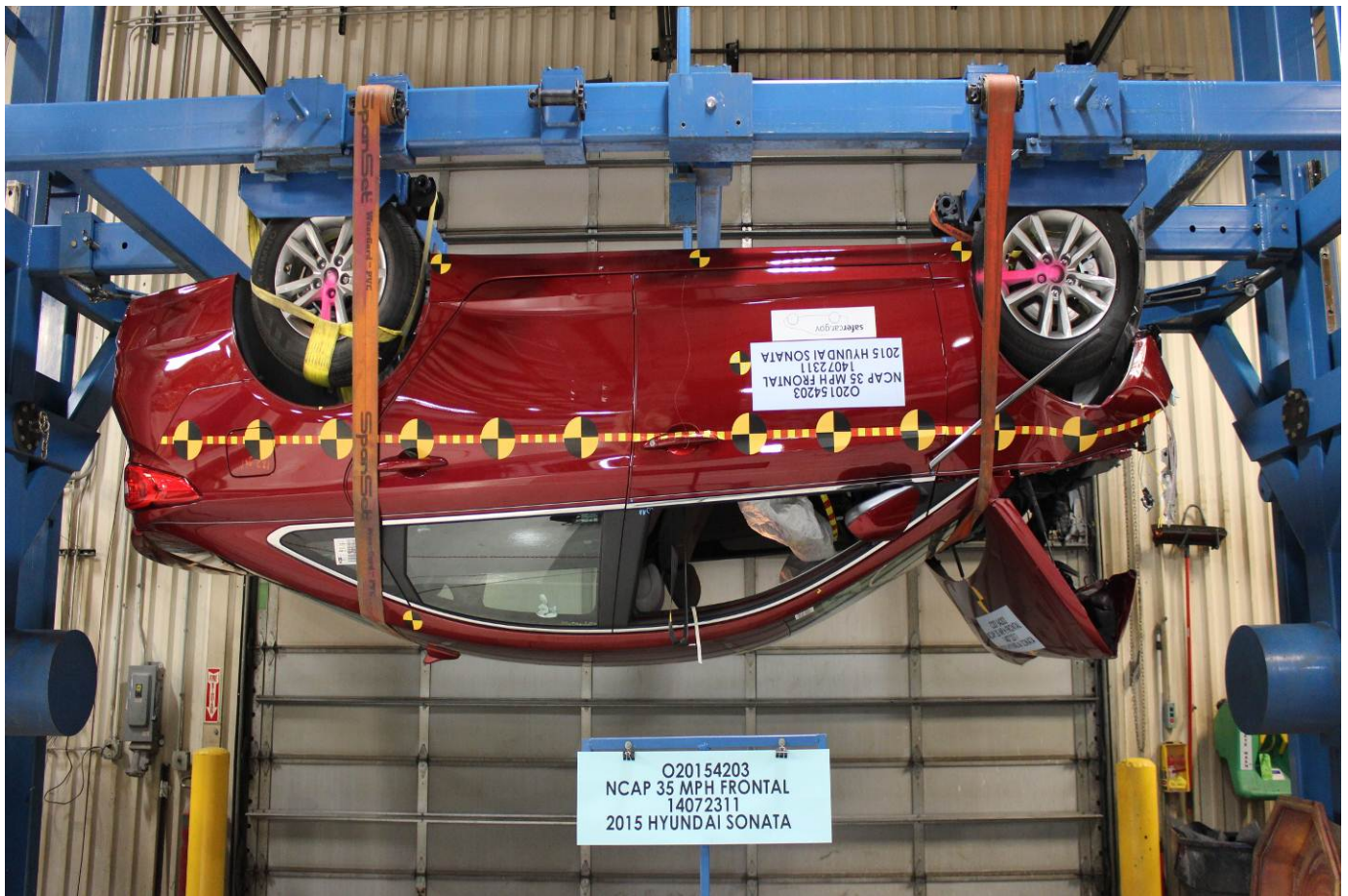
Vehicle at 180 Degrees on Static Rollover Device
