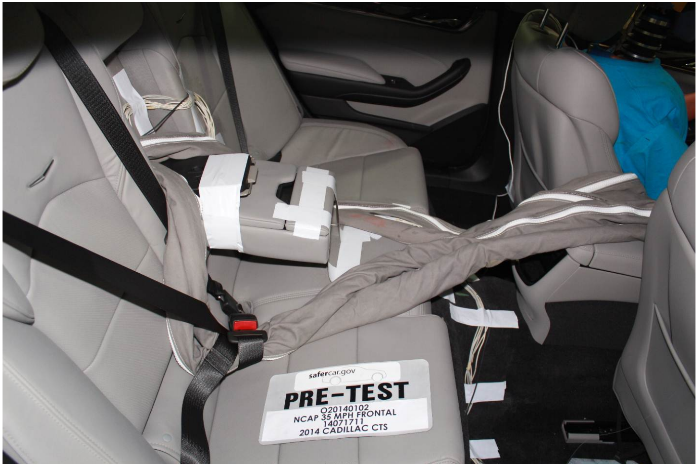
Pre-Test Dummy Cable Routing
