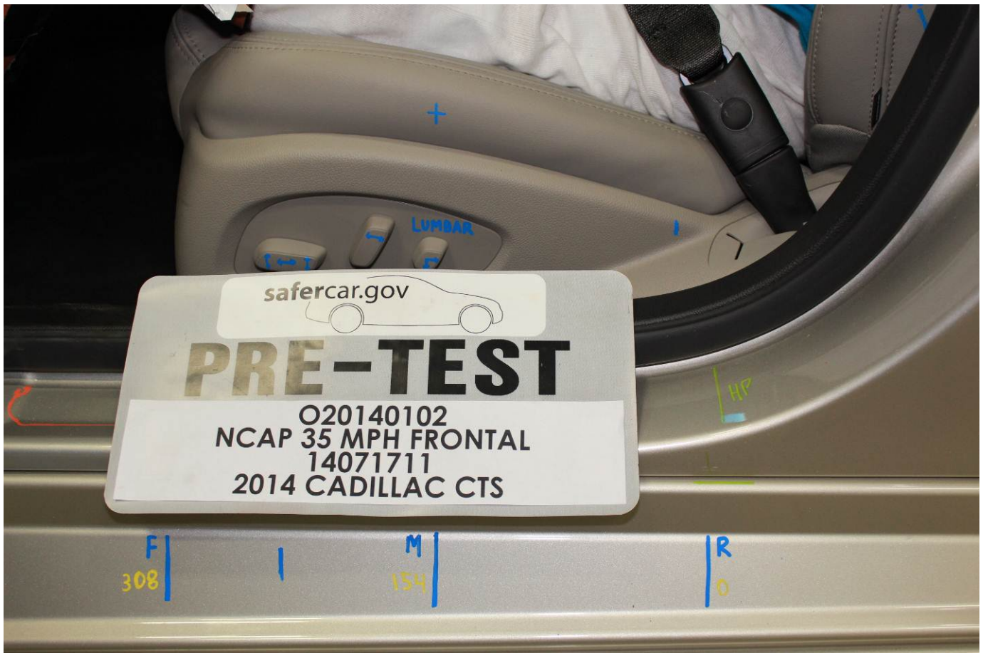
Pre-Test Driver's Seat Fore-Aft Markings
