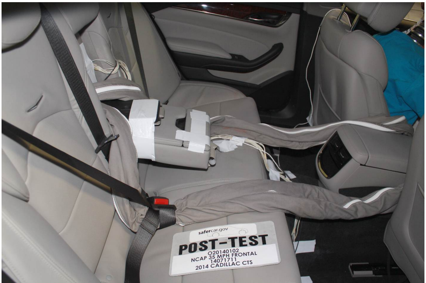
Post-Test Dummy Cable Routing
