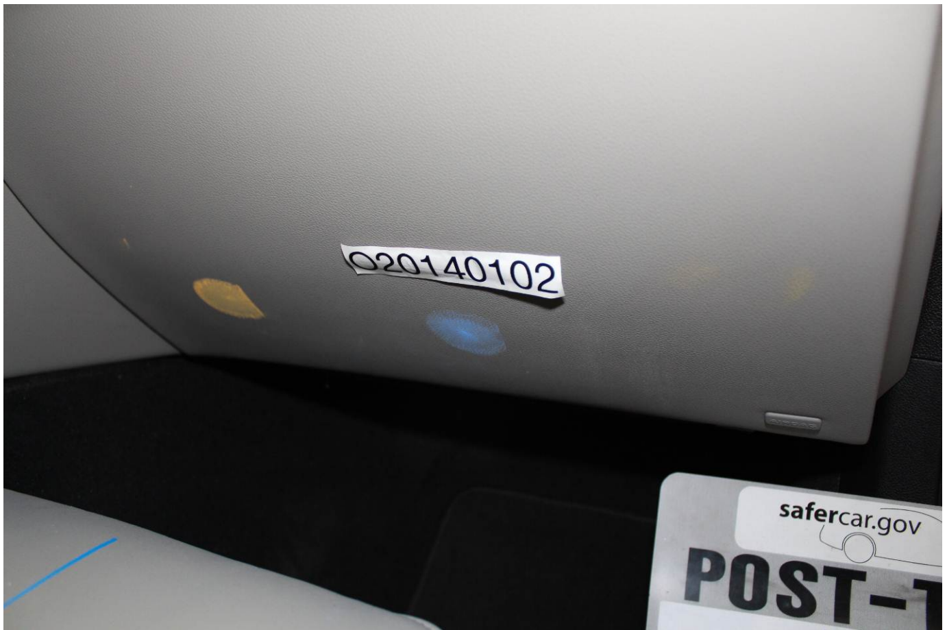
Post-Test Passenger Dummy Contact with Glovebox
