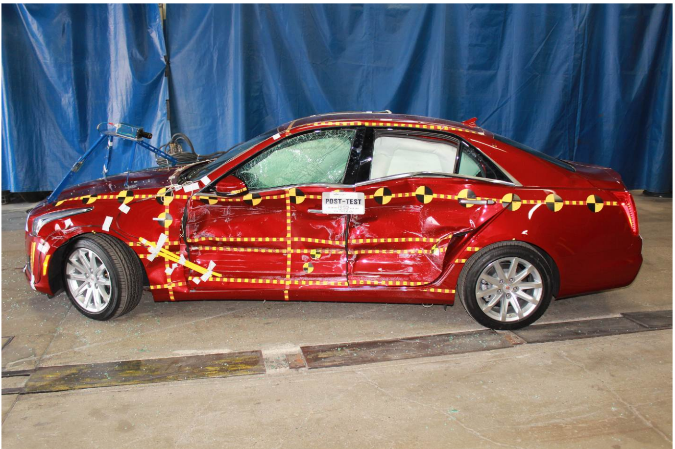
Post-Test Left Side View of Test Vehicle
