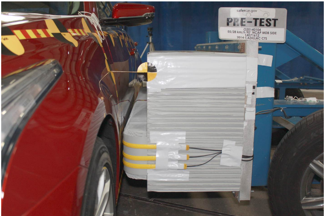
Pre-Test Left Side View of MDB Positioned Against Side of Test Vehicle
