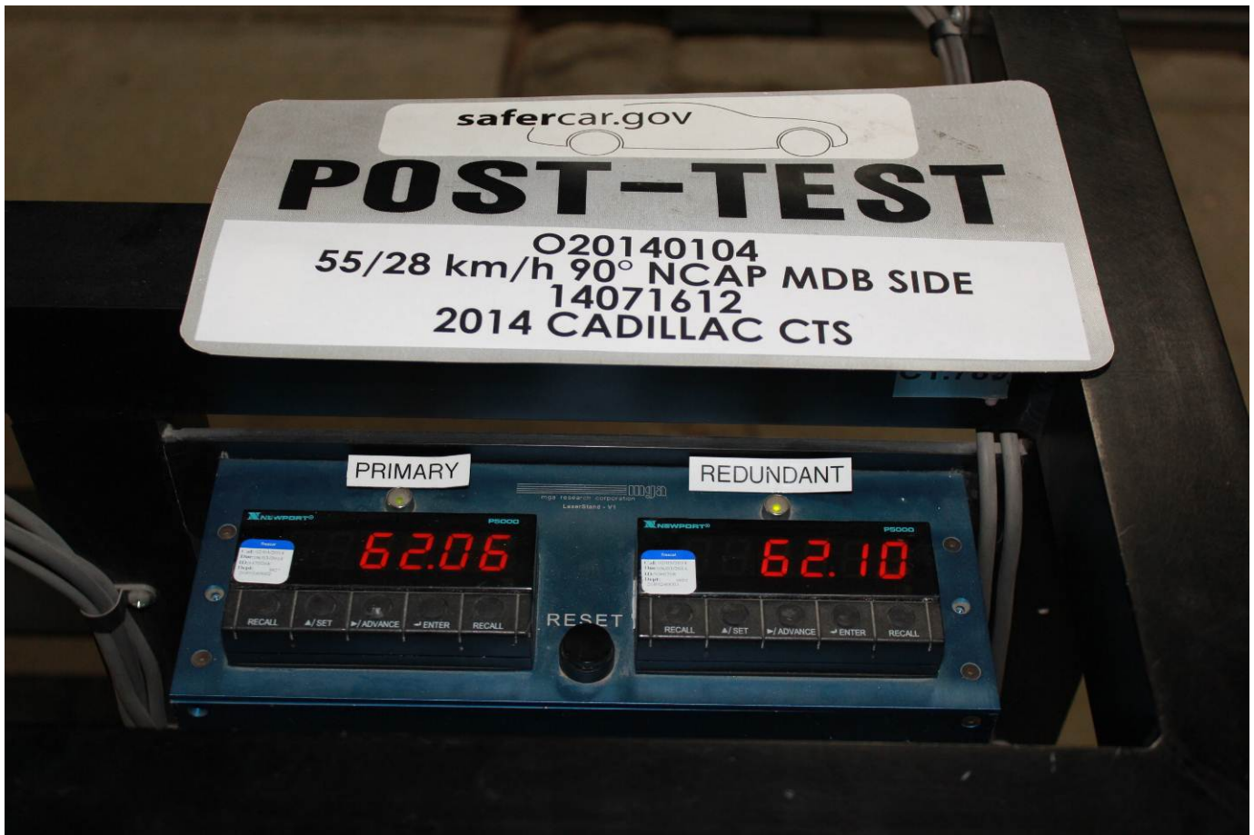
Post-Test Primary and Redundant Speed Trap Read-Out
