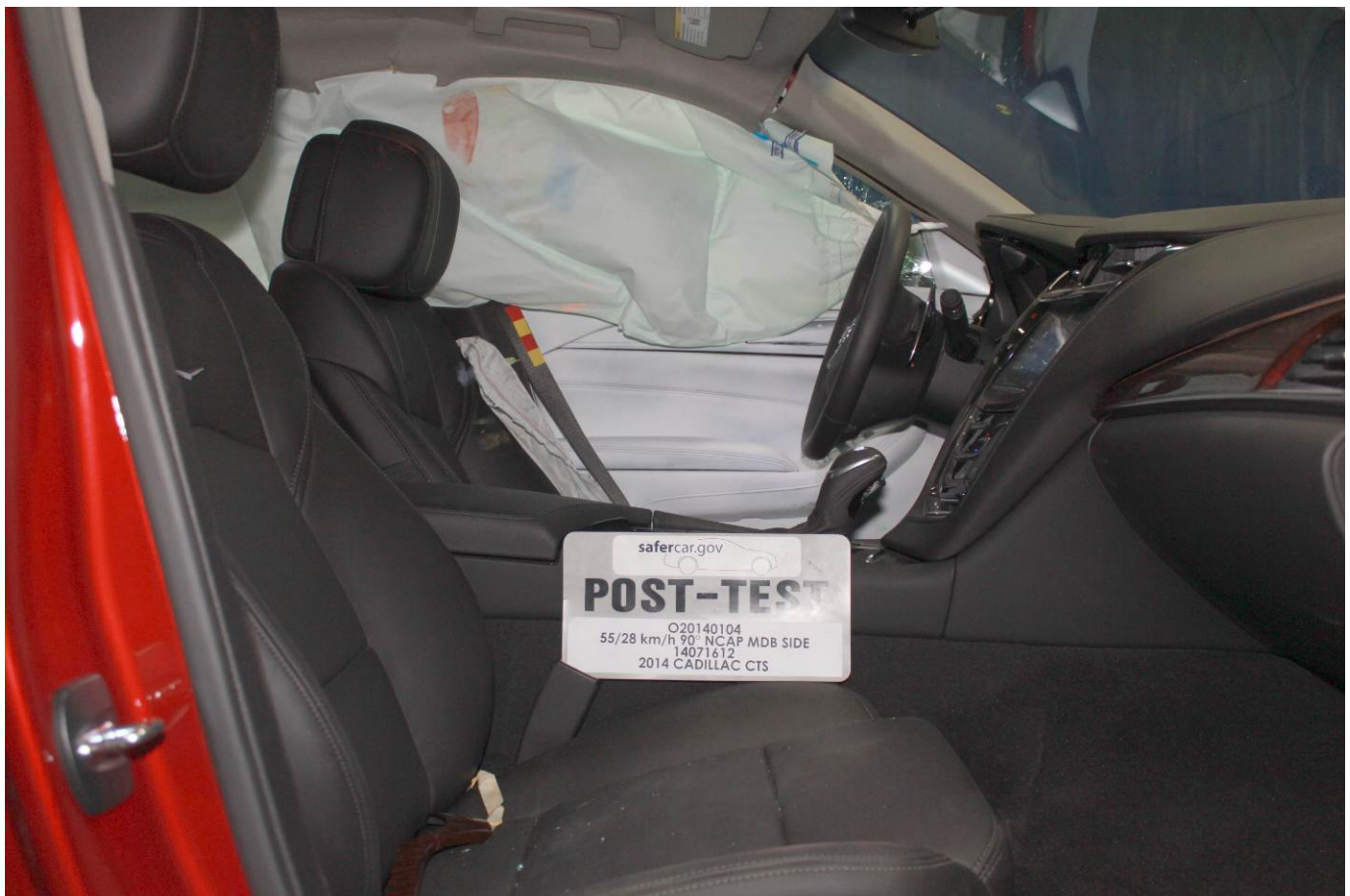
Post-Test Driver Inner Door Panel View
