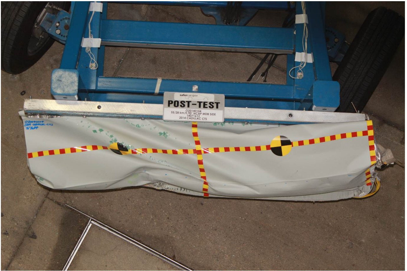
Post-Test Top View of MDB Impactor Face
