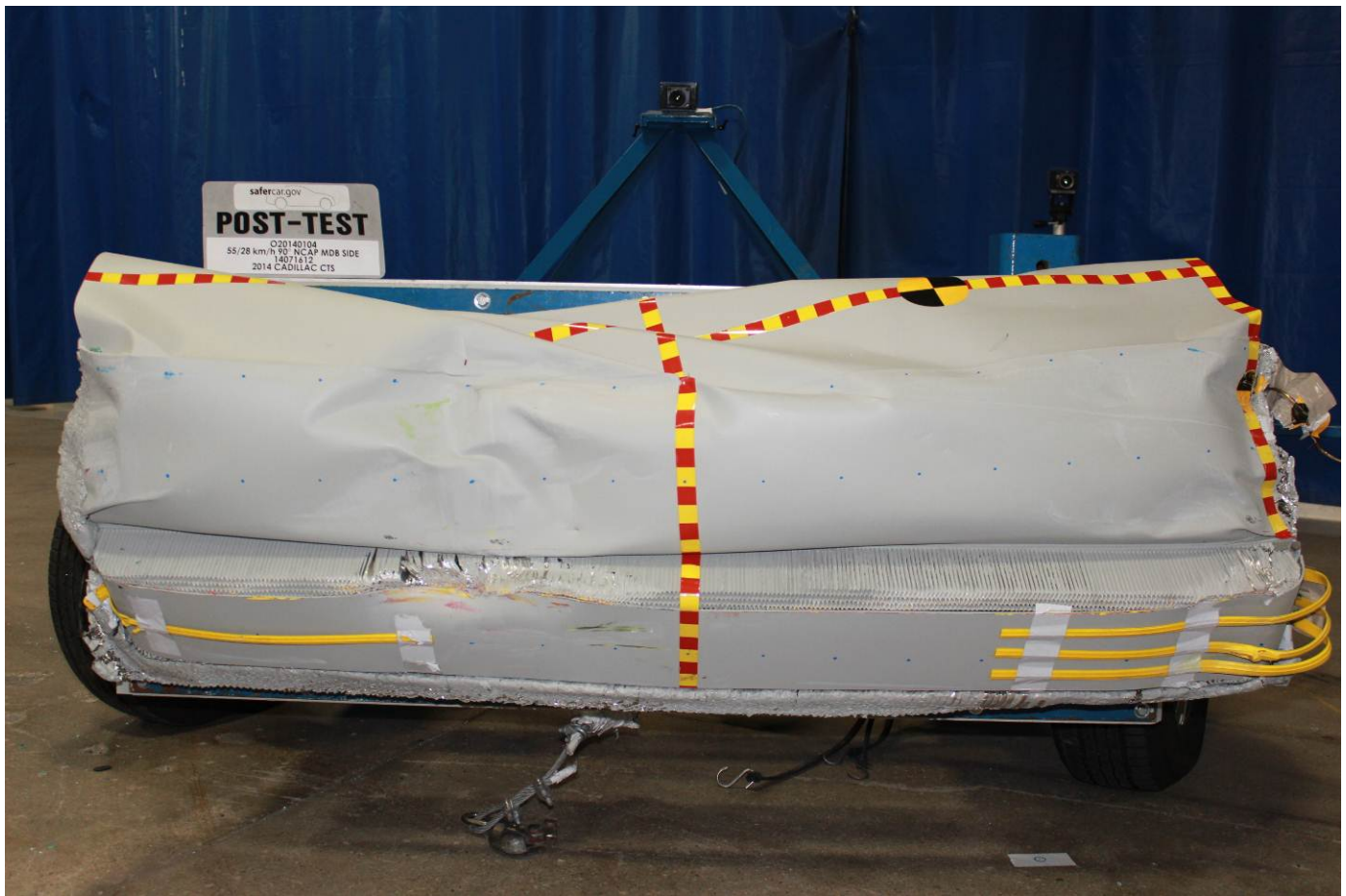
Post-Test Front View of MDB Impactor Face
