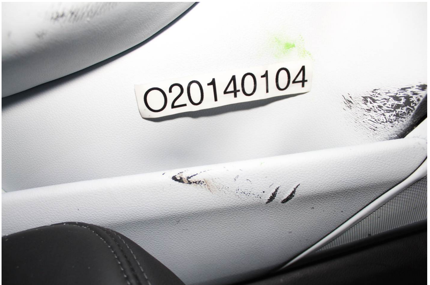
Post-Test Driver Dummy Close-up Knee Contact View
