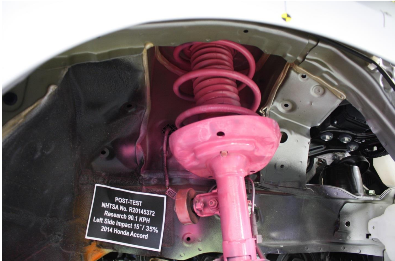
No. 154 Post-Test Front Passenger Close up View of Suspension w/ Tire Removed
