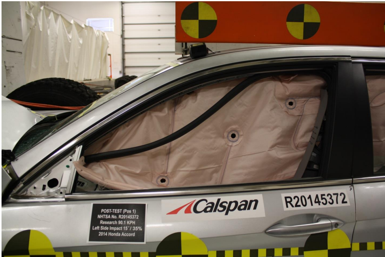
No. 057 Post-Test Left Side Driver Window View
