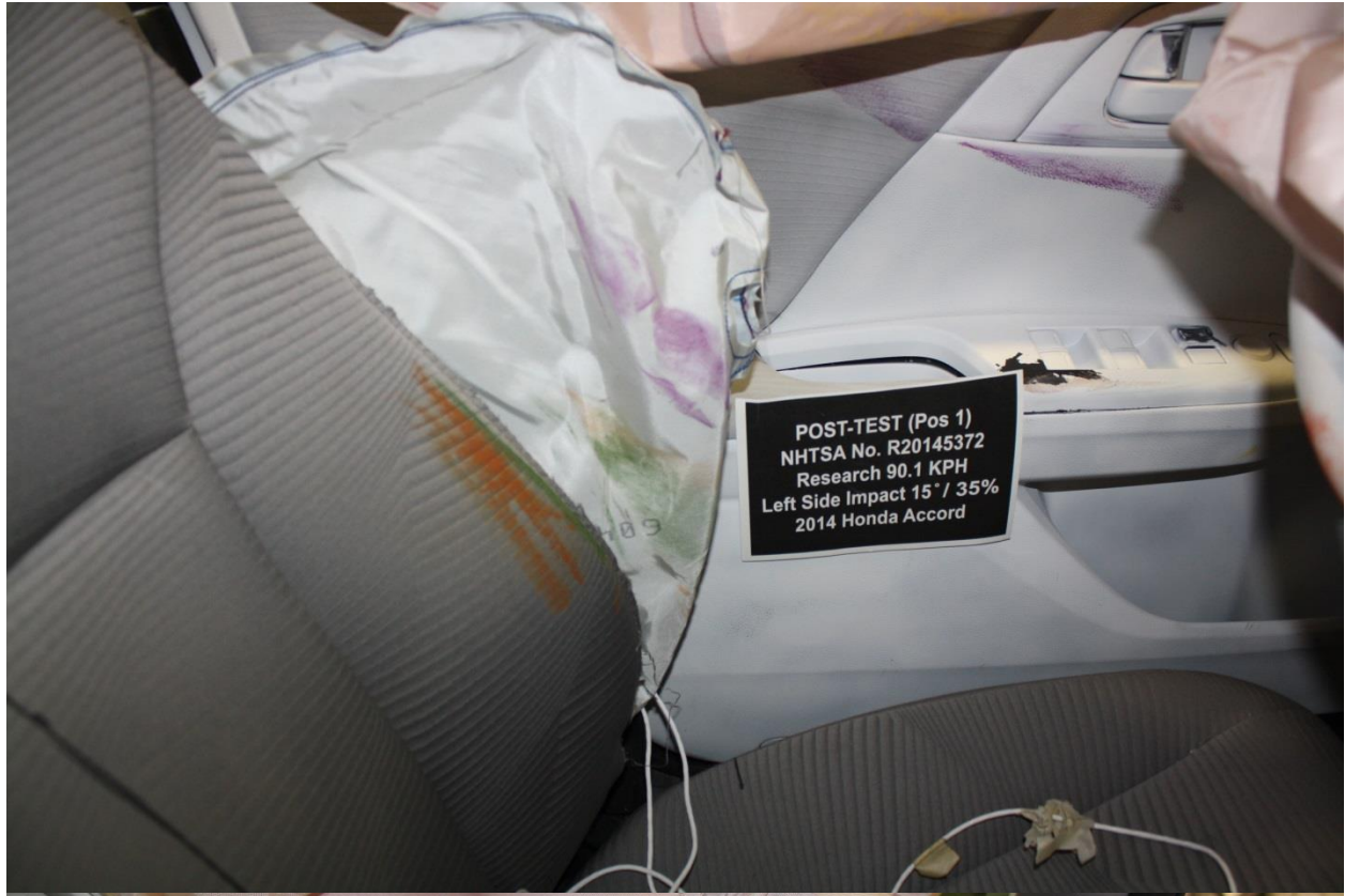
No. 081b Post-Test View of Driver Body Contact with Vehicle Interior - C
