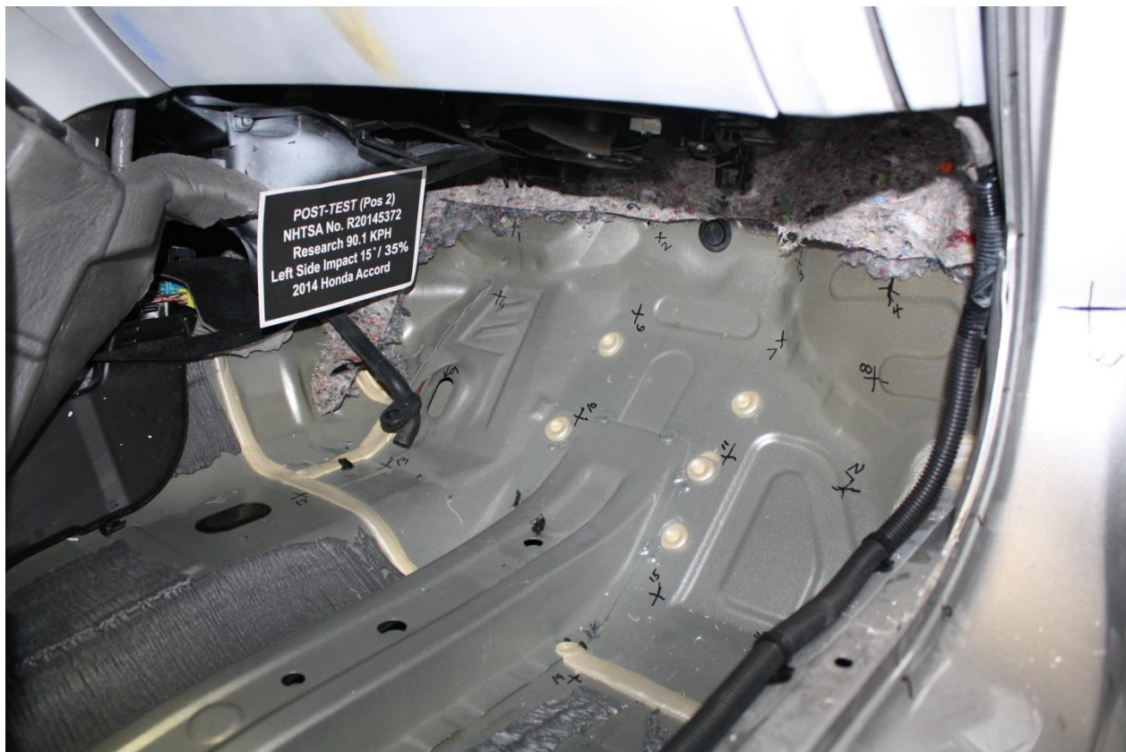
No. 093 Post-Test View of Passenger Floor pan at Left sill level, w/o carpet
