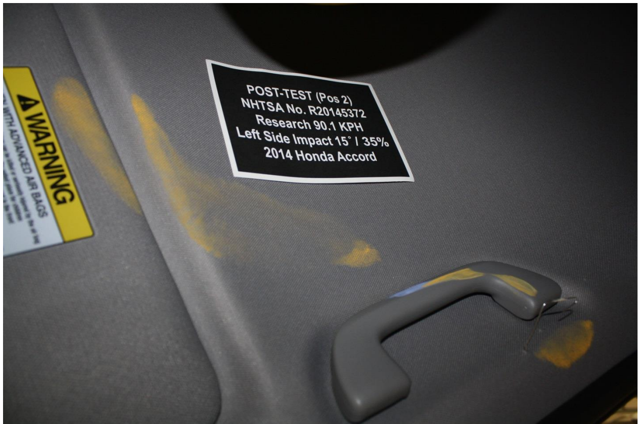
No. 121a Post-Test View of Passenger Head contact with Interior
