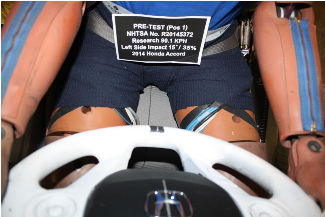
No. 066 Pre-Test Overhead View of Driver Thighs on Seat
