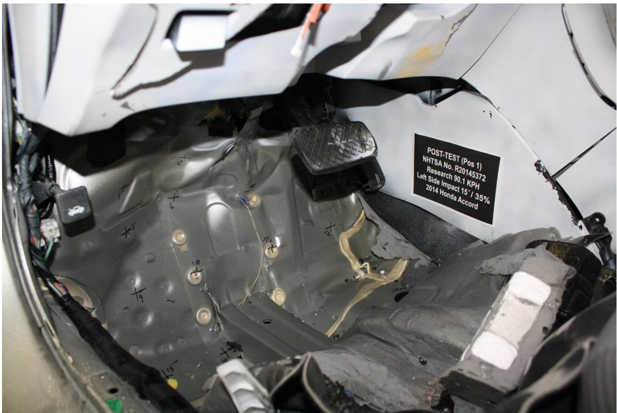
No. 049 Post-Test View of Driver Floor pan at Left sill level, w/o carpet
