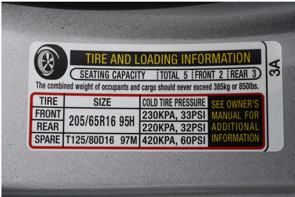
No. 004 Test Vehicle Tire Placard
