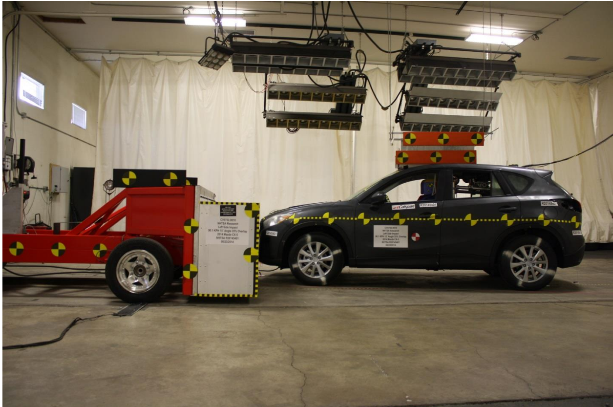
No. 170 Pre-Test RMDB & Vehicle, Right Side
