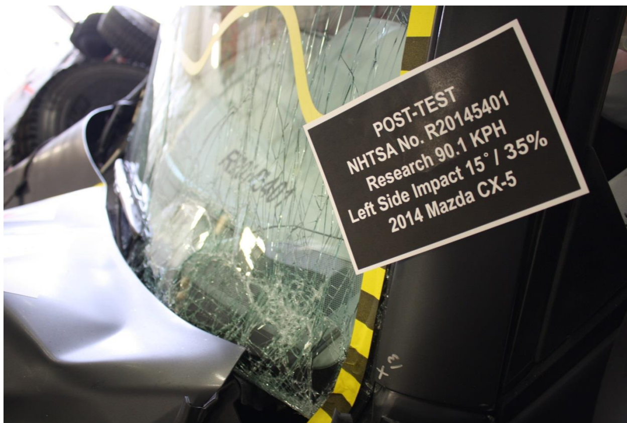
No. 161 Post-Test View of Windshield Separation
