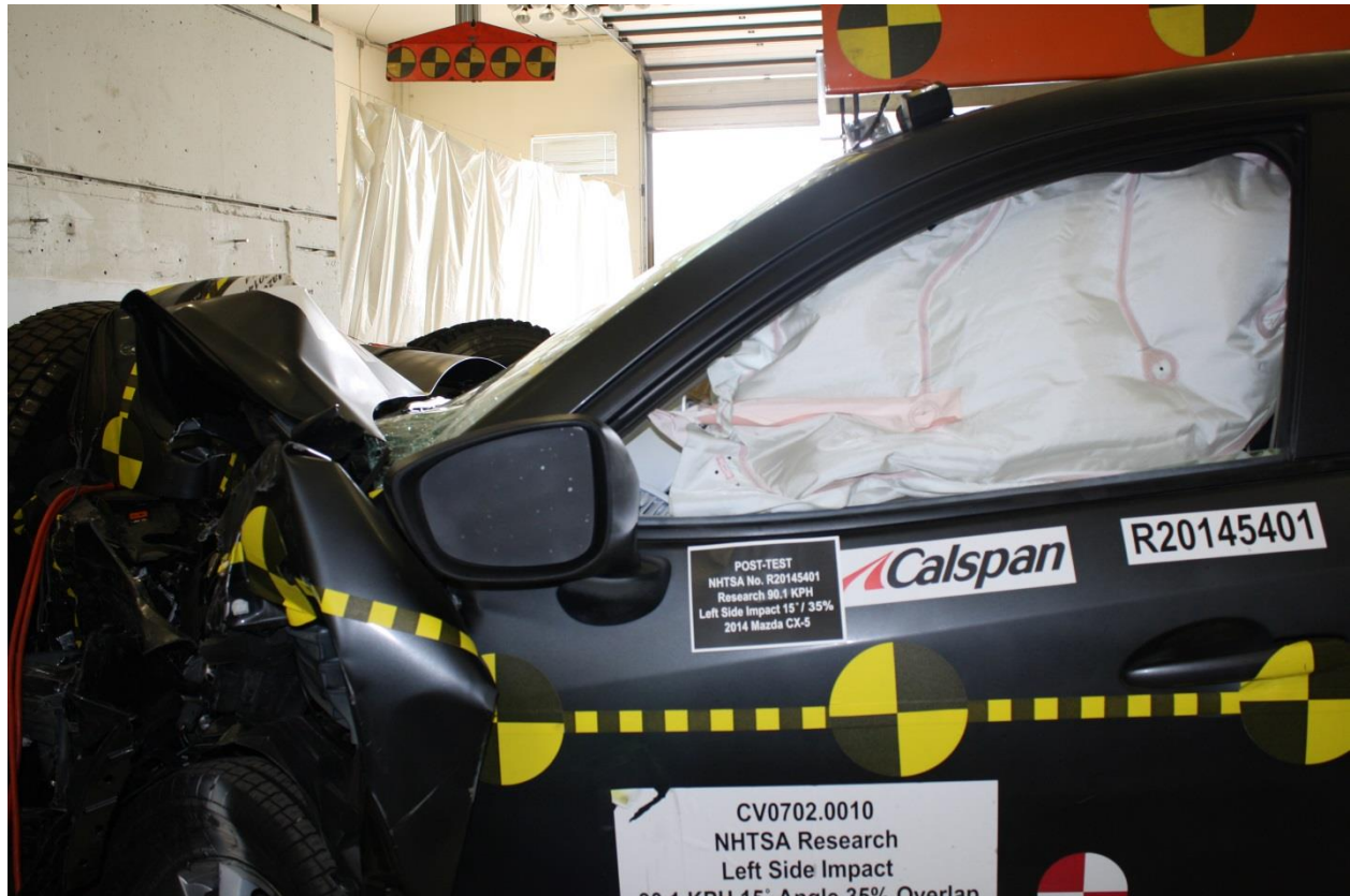
No. 156 Post-Test View of Deformation of A pillar-Struck Side
