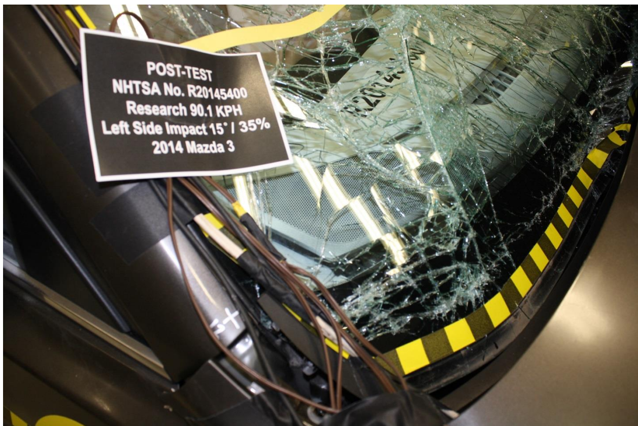
No. 161 Post-Test View of Windshield Separation
