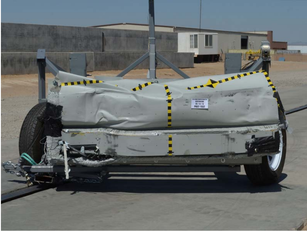
FIGURE 85. Post-Test Front View of MDB Impactor Face
