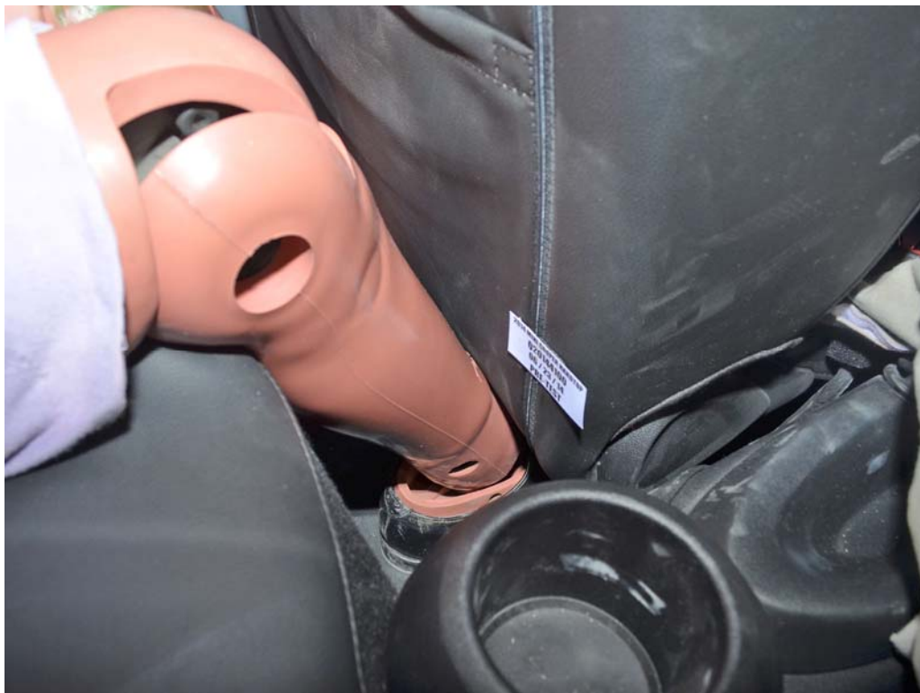
FIGURE 64. Pre-Test Placement of Rear Passenger Dummy's Feet
