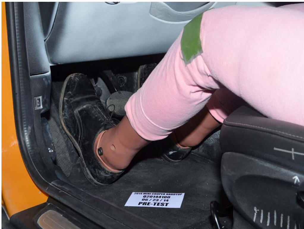
FIGURE 34. Pre-Test Placement of Driver Dummy's Feet
