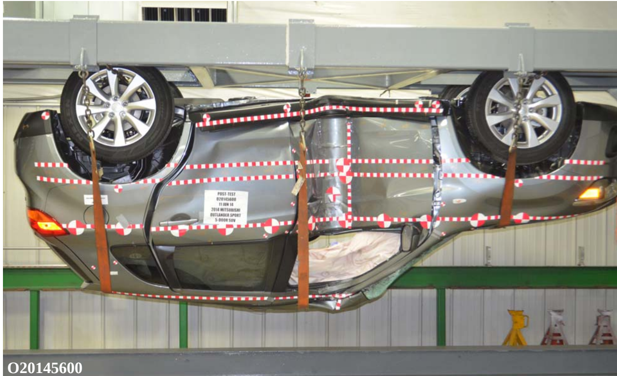
Figure 065: FMVSS No. 301 Static Rollover 180 Degrees
