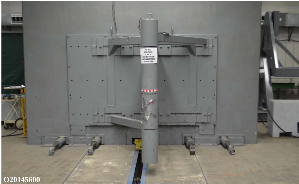
Figure 057: Pre-Test Pole Barrier Front View
