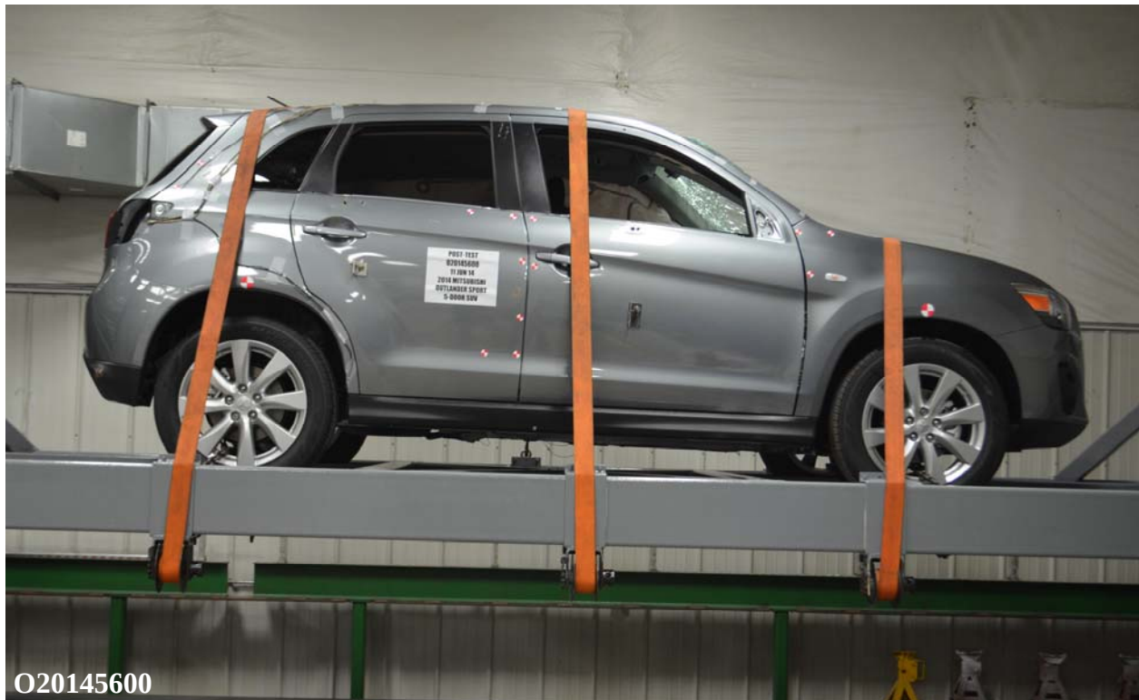
Figure 063: FMVSS No. 301 Static Rollover 0 Degrees
