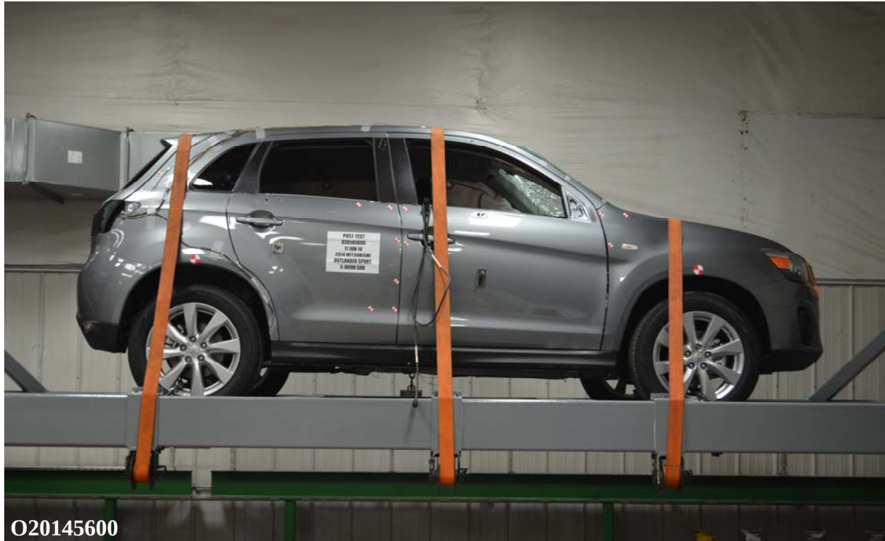
Figure 067: FMVSS No. 301 Static Rollover 360 Degrees
