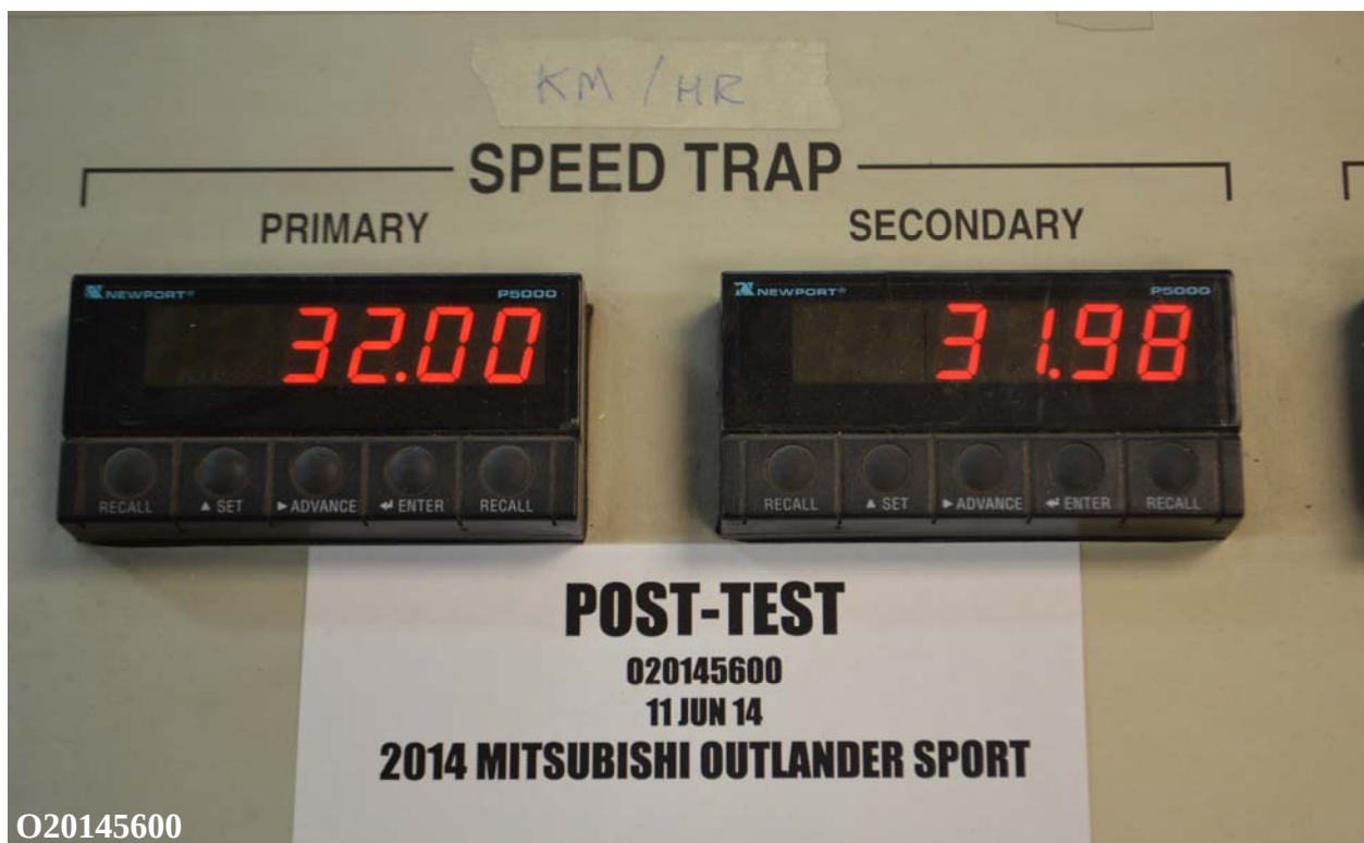
Figure 062: Post-Test Primary and Redundant Speed Trap Read-Out
