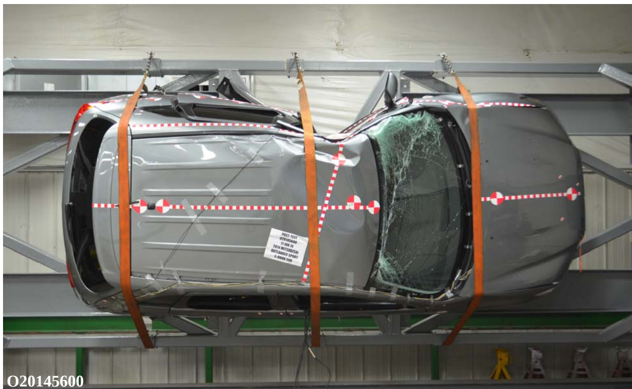
Figure 066: FMVSS No. 301 Static Rollover 270 Degrees
