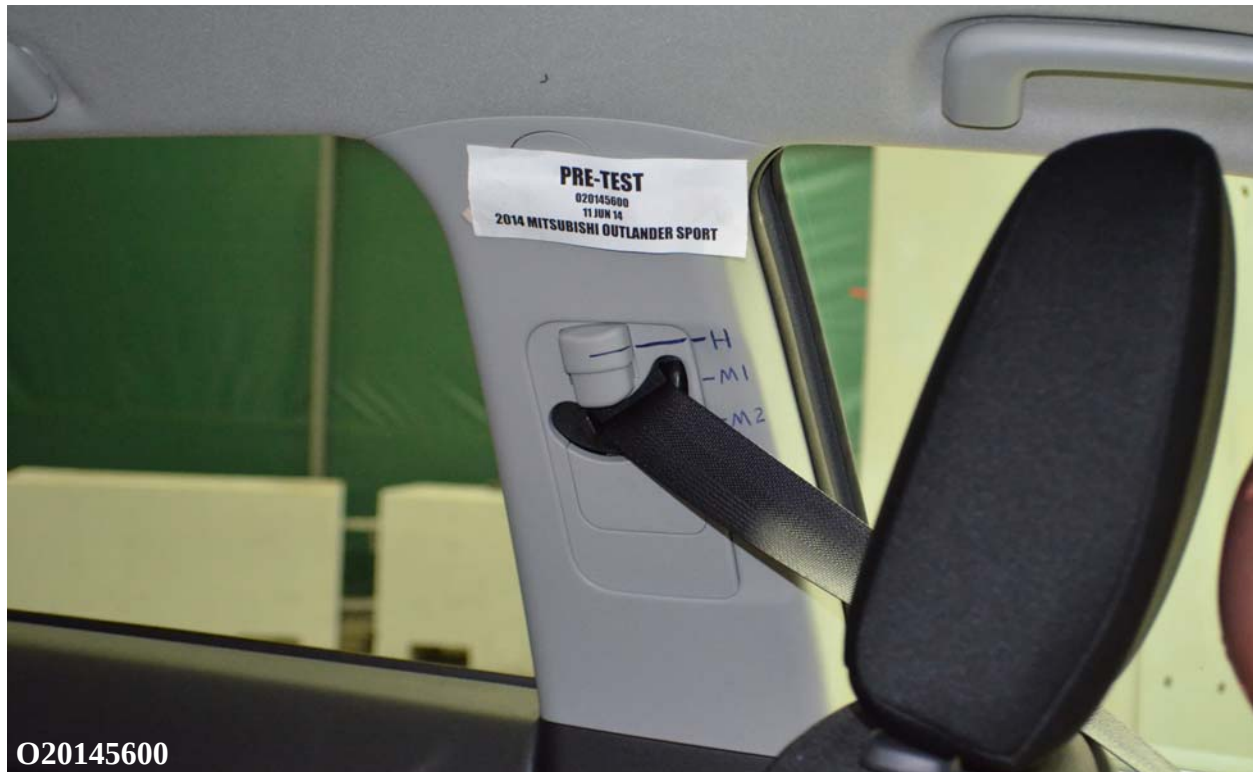
Figure 033: Pre-Test View of Belt Anchorage for Dummy
