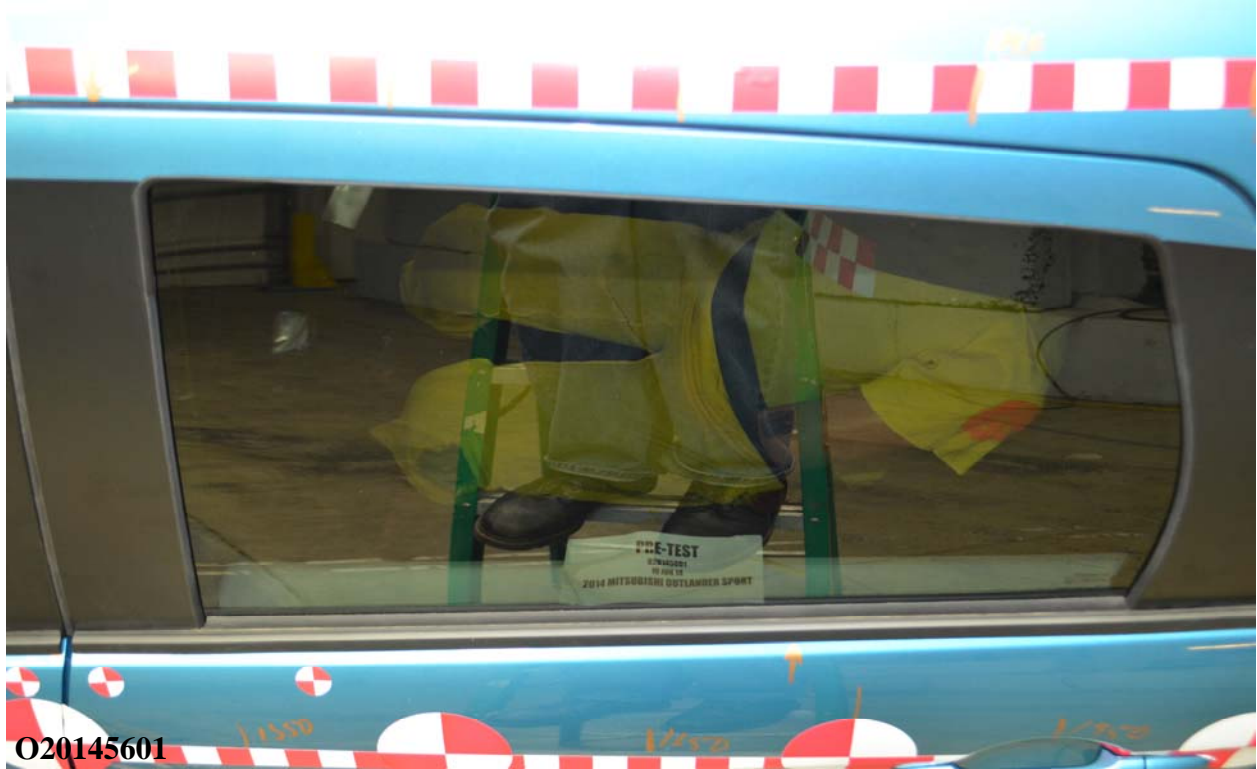
Figure A-69: Pre-Test Rear Passenger Dummy and Door Clearance View
