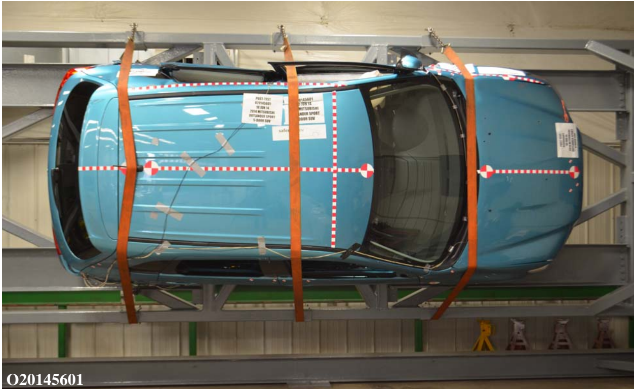
Figure A-99: FMVSS No. 301 Static Rollover 270 Degrees
