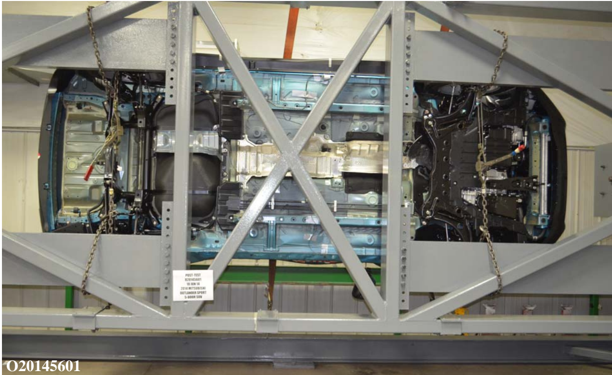
Figure A-97: FMVSS No. 301 Static Rollover 90 Degrees
