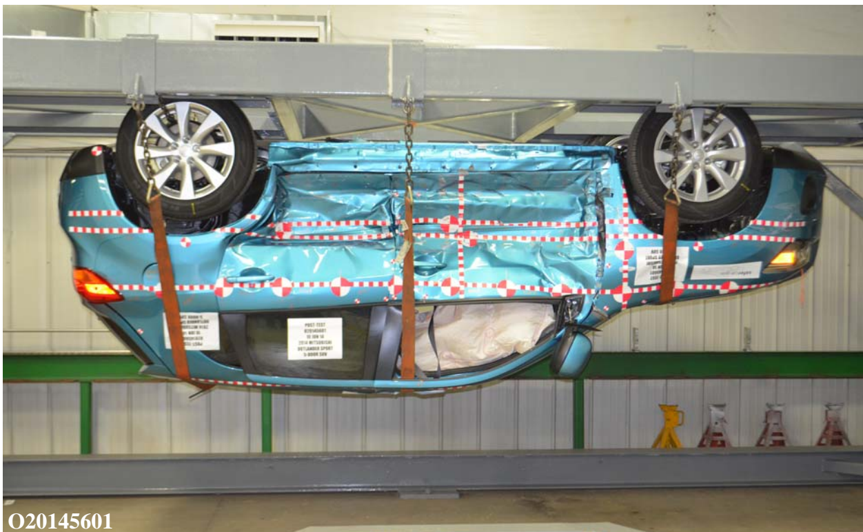
Figure A-98: FMVSS No. 301 Static Rollover 180 Degrees
