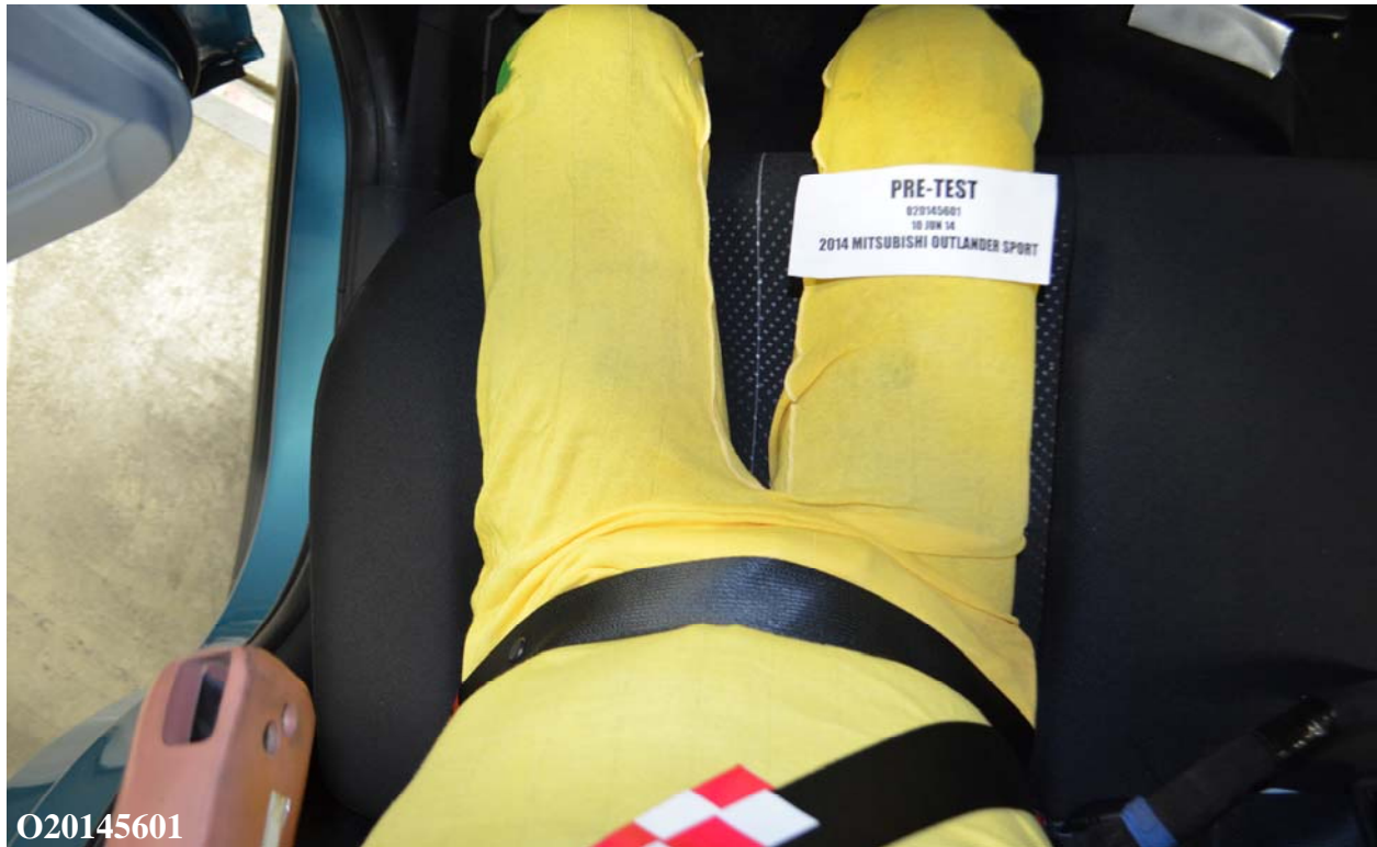
Figure A-61: Pre-Test Overhead View of Rear Passenger Dummy Thighs on Seat Pan
