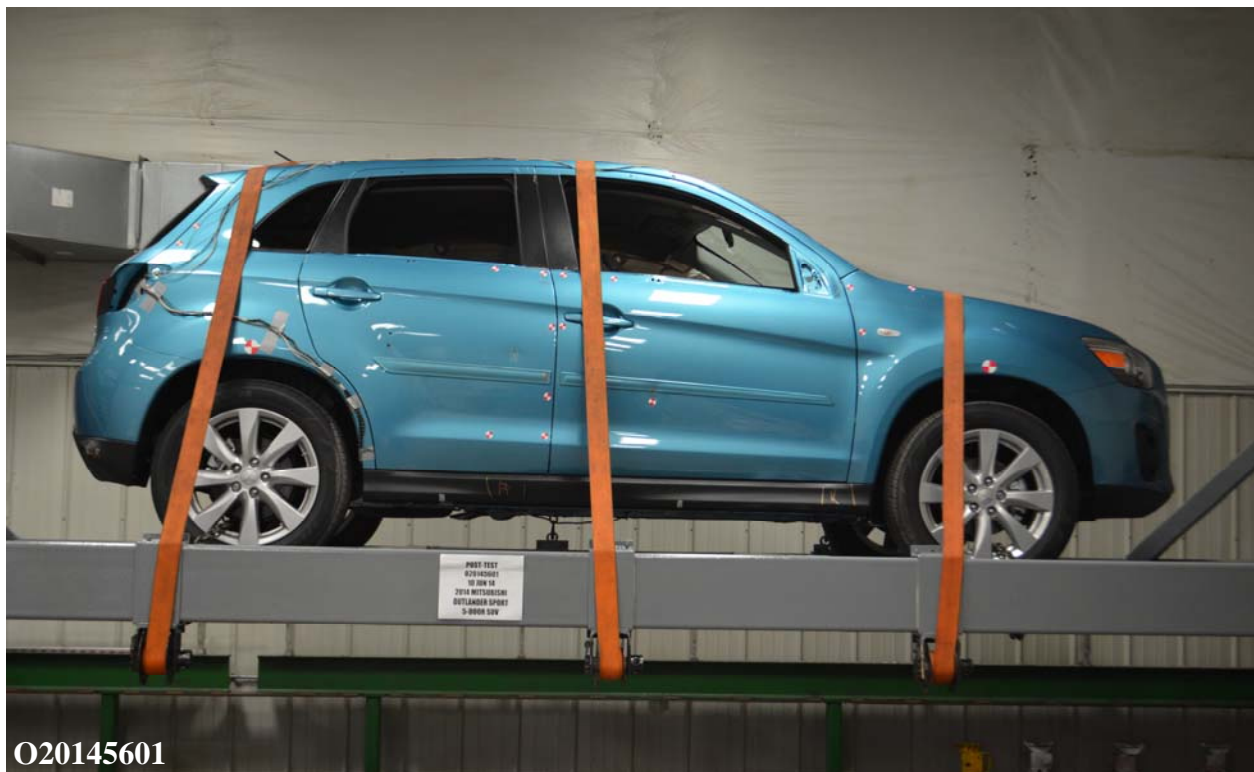
Figure A-96: FMVSS No. 301 Static Rollover 0 Degrees
