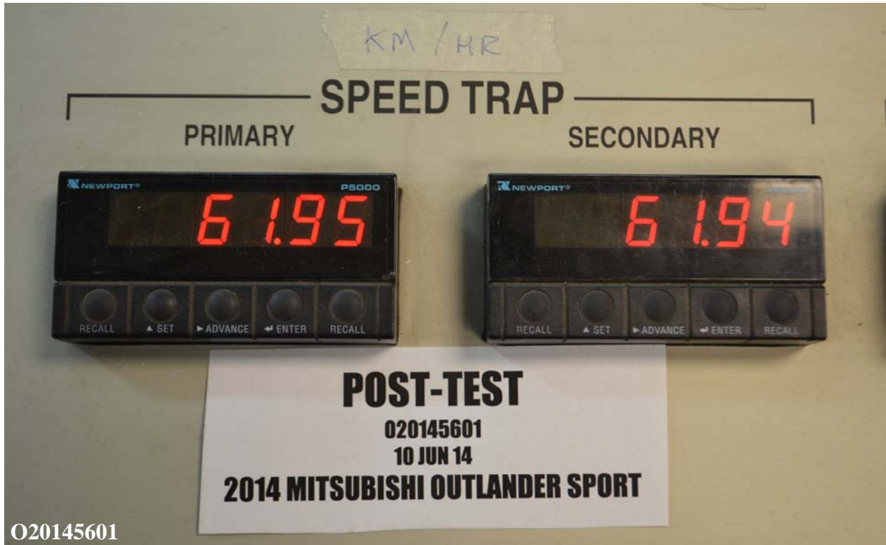
Figure A-95: Post-Test Primary and Redundant Speed Trap Read-Out
