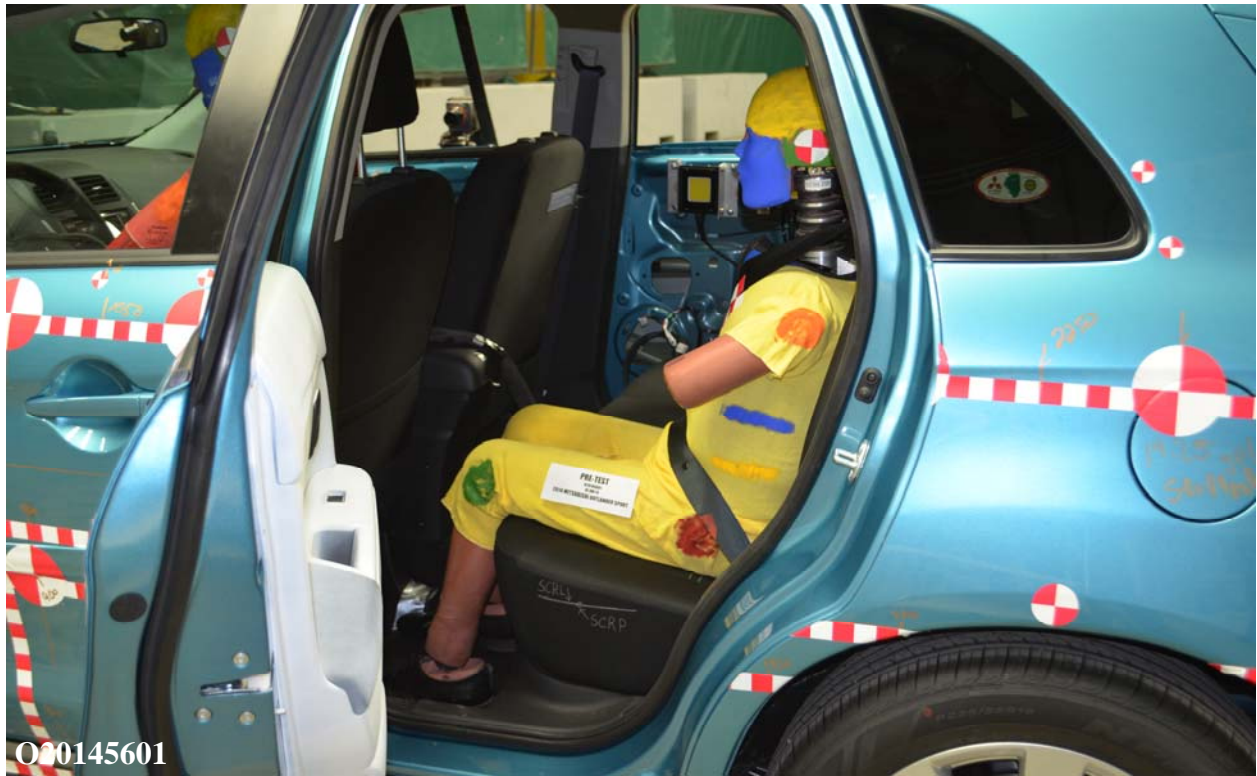
Figure A-55: Pre-Test Left Side View of Rear Passenger Dummy Showing Belt and Chalking
