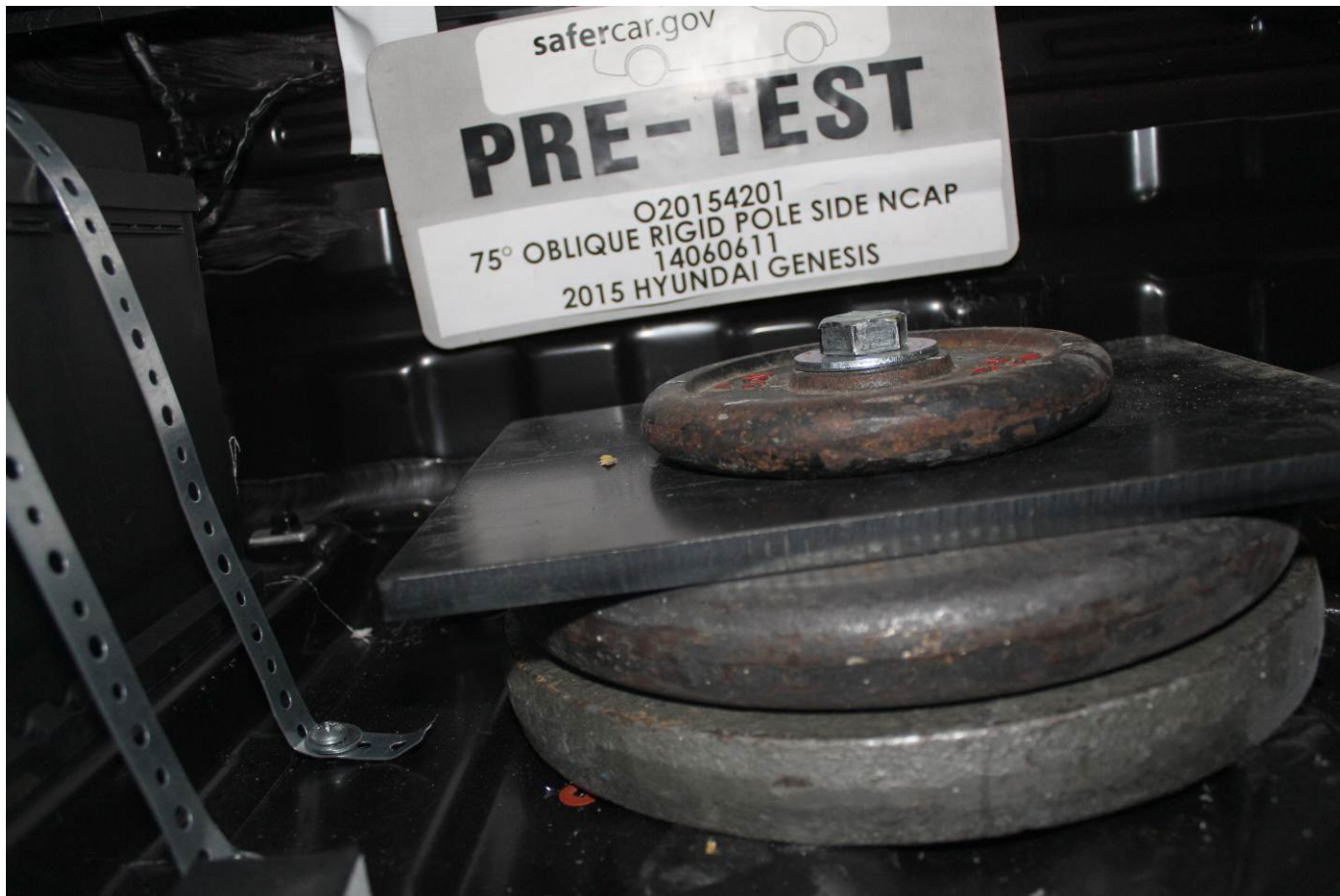
Pre-Test Ballast View
