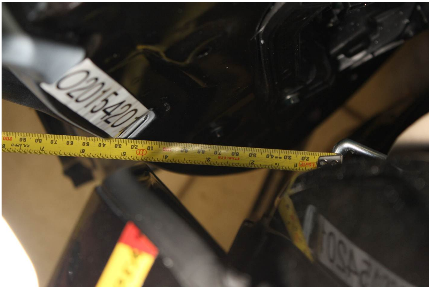
Post-Test View of Left Front Door Opening
