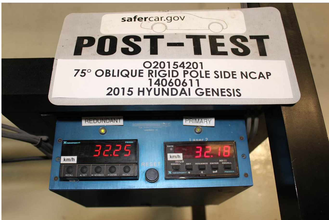
Post-Test Primary and Redundant Speed Trap Read-Out
