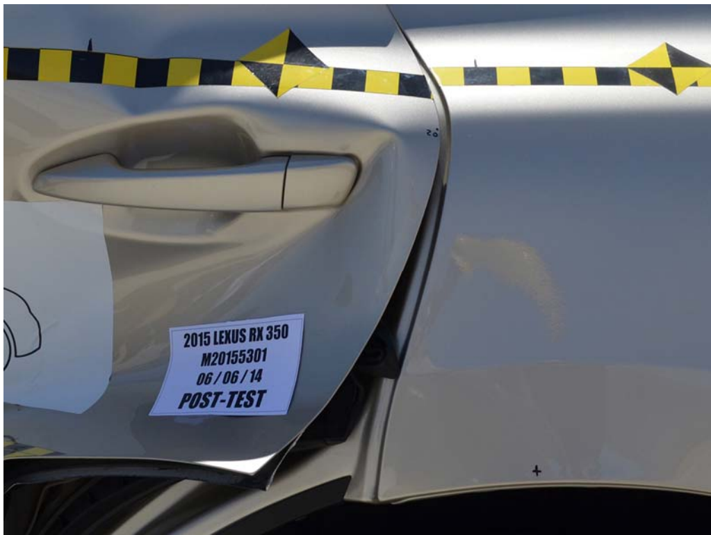
FIGURE 24. Post-Test Left Rear Door Latch Close-Up
