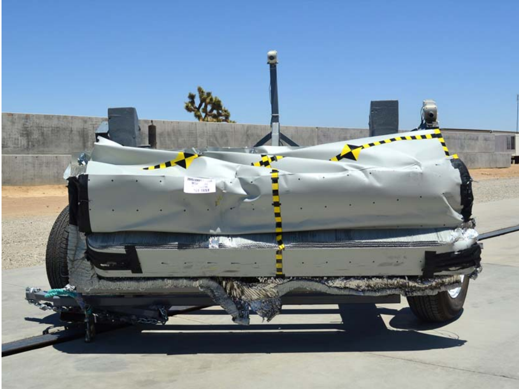
FIGURE 85. Post-Test Front View of MDB Impactor Face
