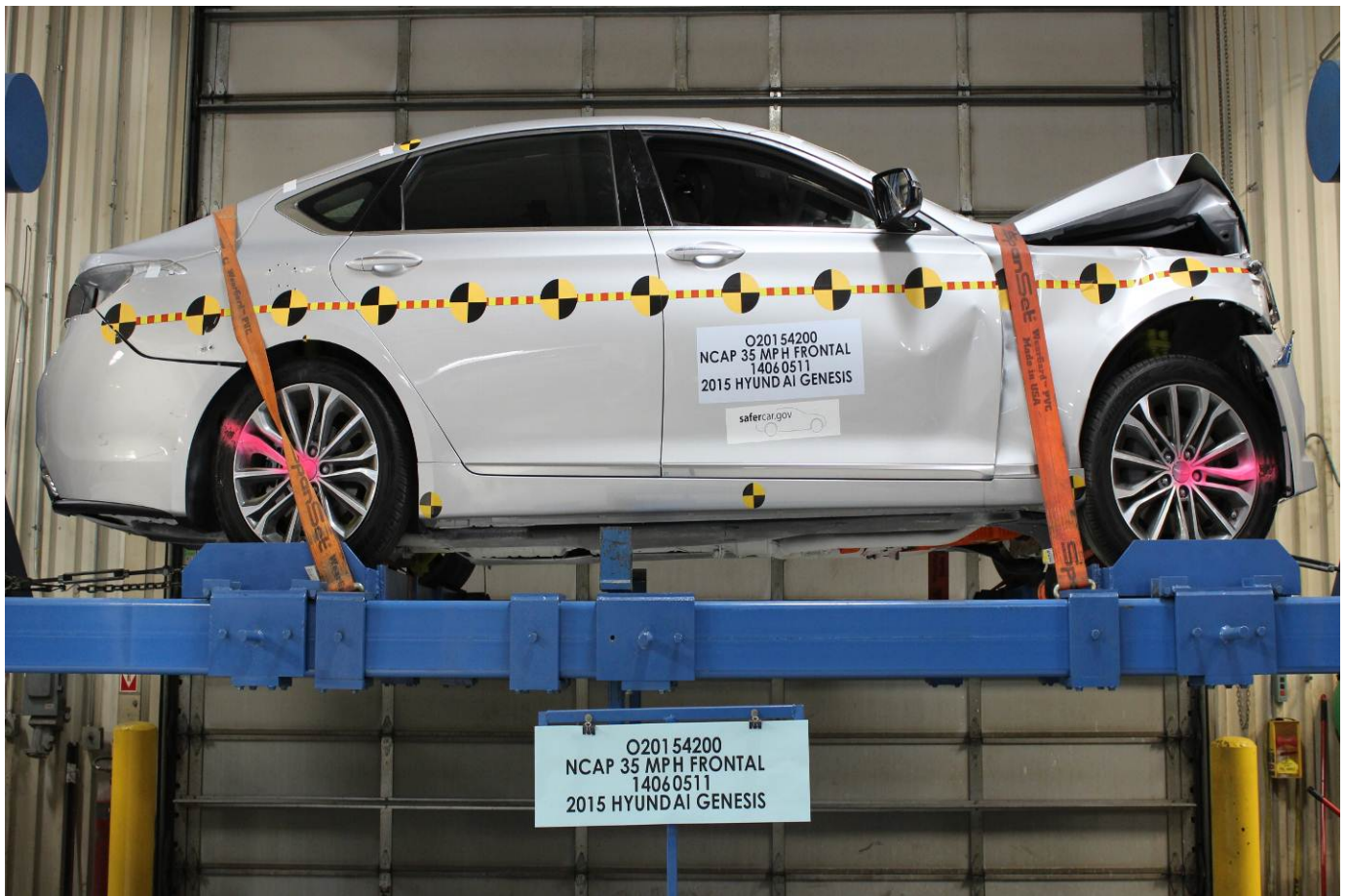
Vehicle at 0 Degree on Static Rollover Device
