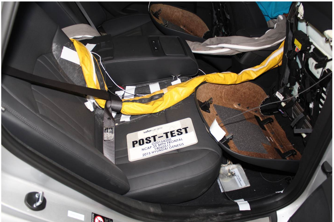
Post-Test Dummy Cable Routing
