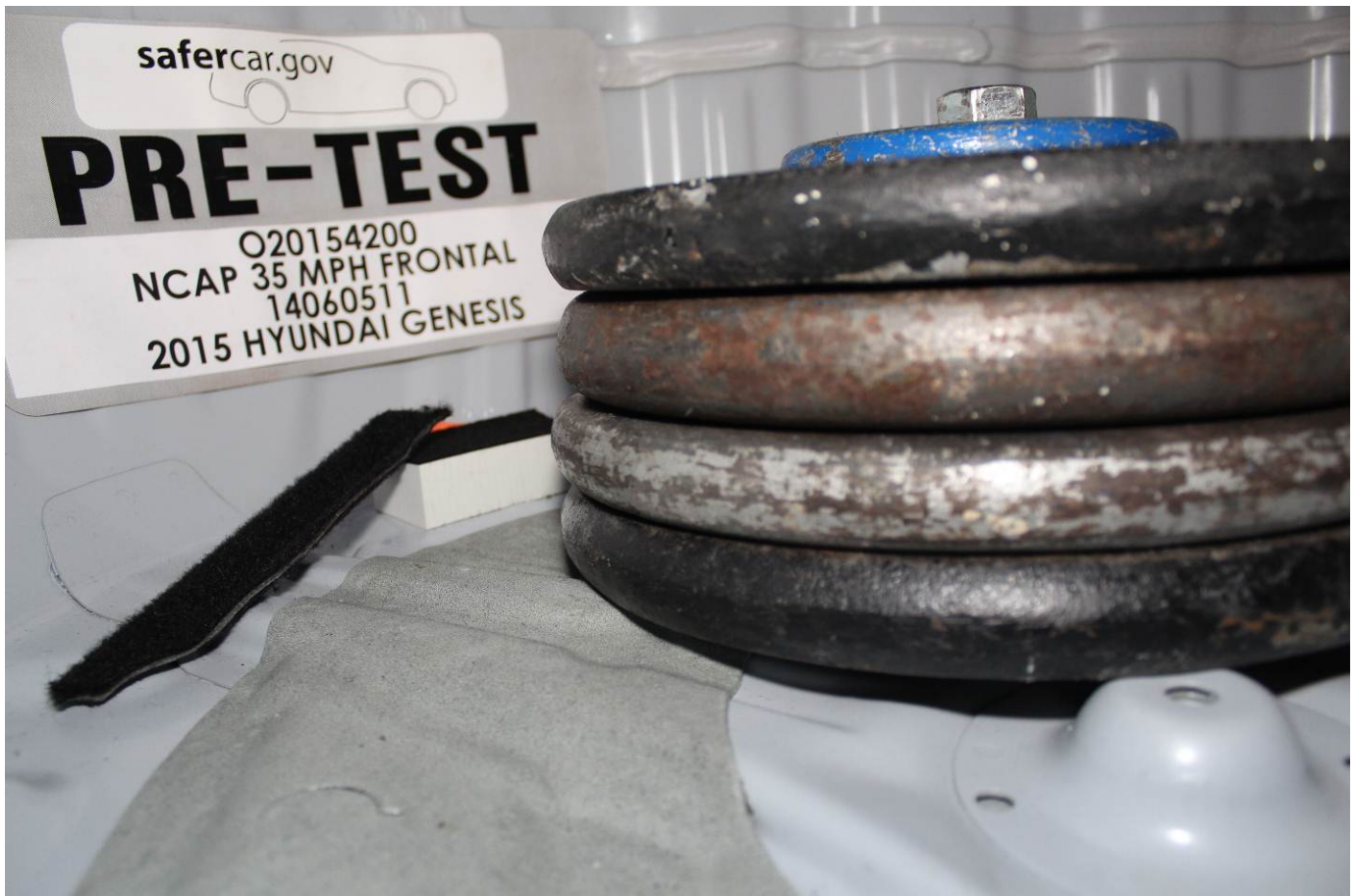
Ballast Installed in Vehicle
