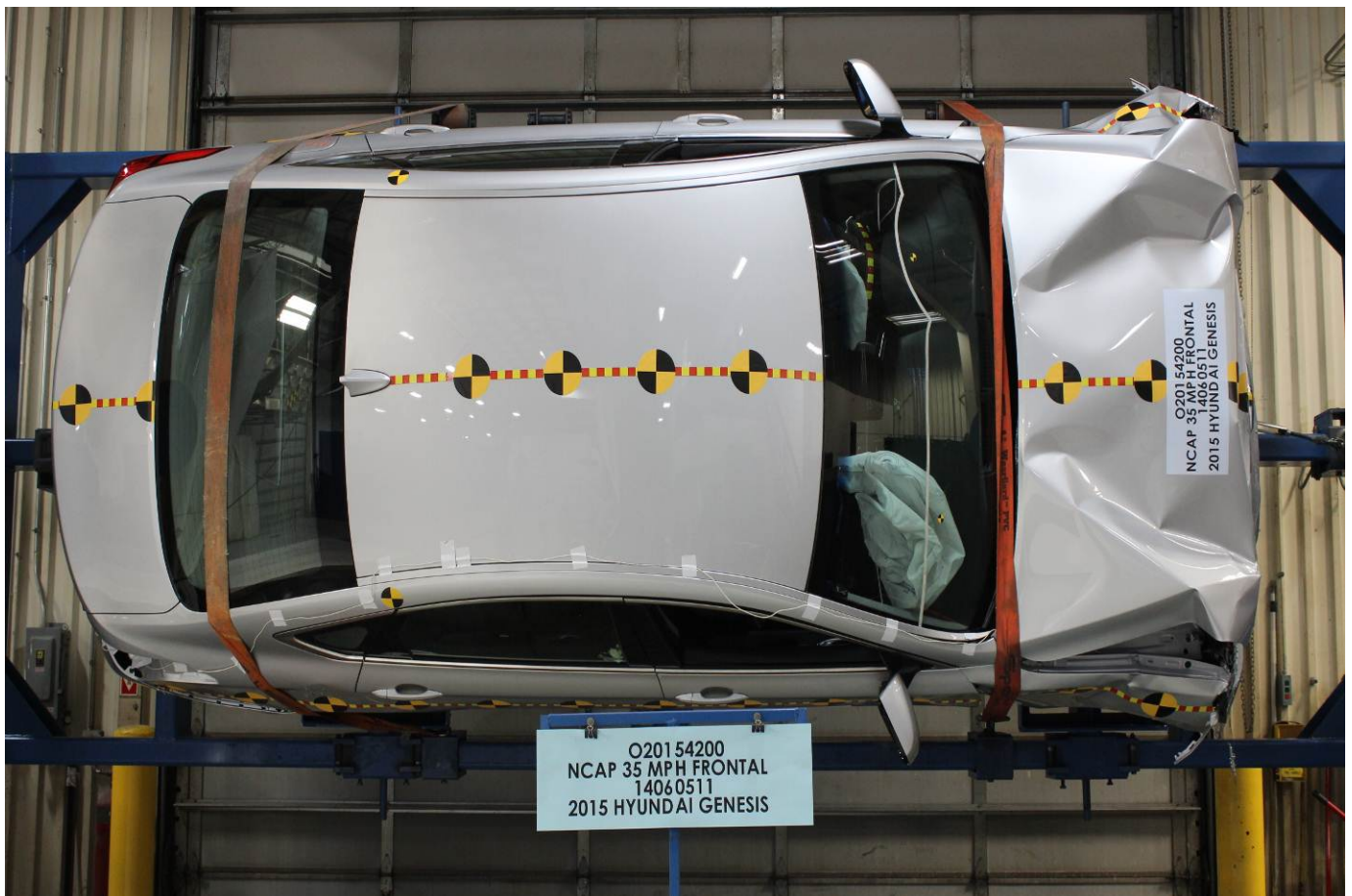
Vehicle at 270 Degrees on Static Rollover Device
