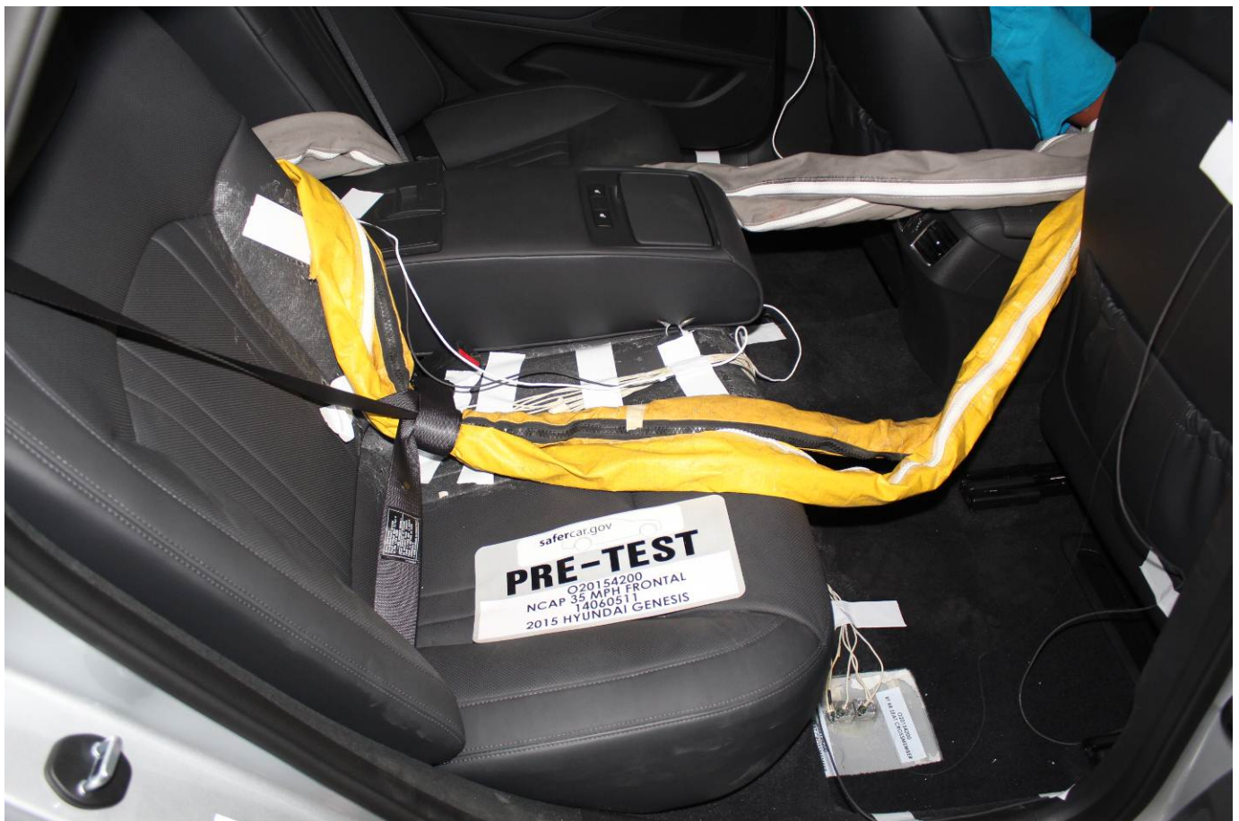
Pre-Test Dummy Cable Routing
