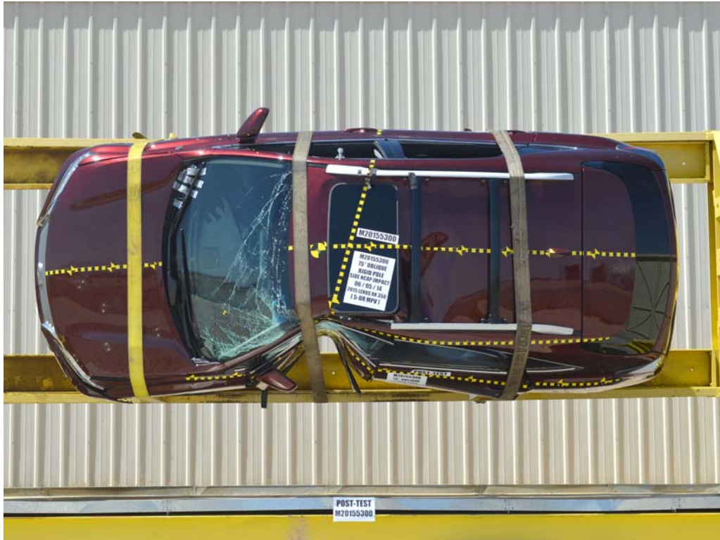
FIGURE 64. FMVSS No. 301 Static Rollover 90 Degrees
