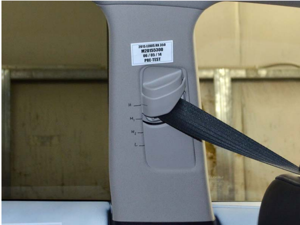
FIGURE 33. Pre-Test View of Belt Anchorage for Dummy
