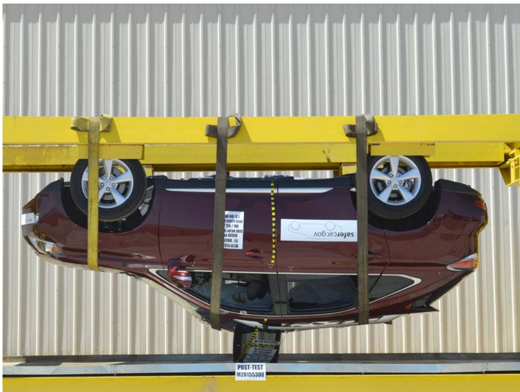
FIGURE 65. FMVSS No. 301 Static Rollover 180 Degrees
