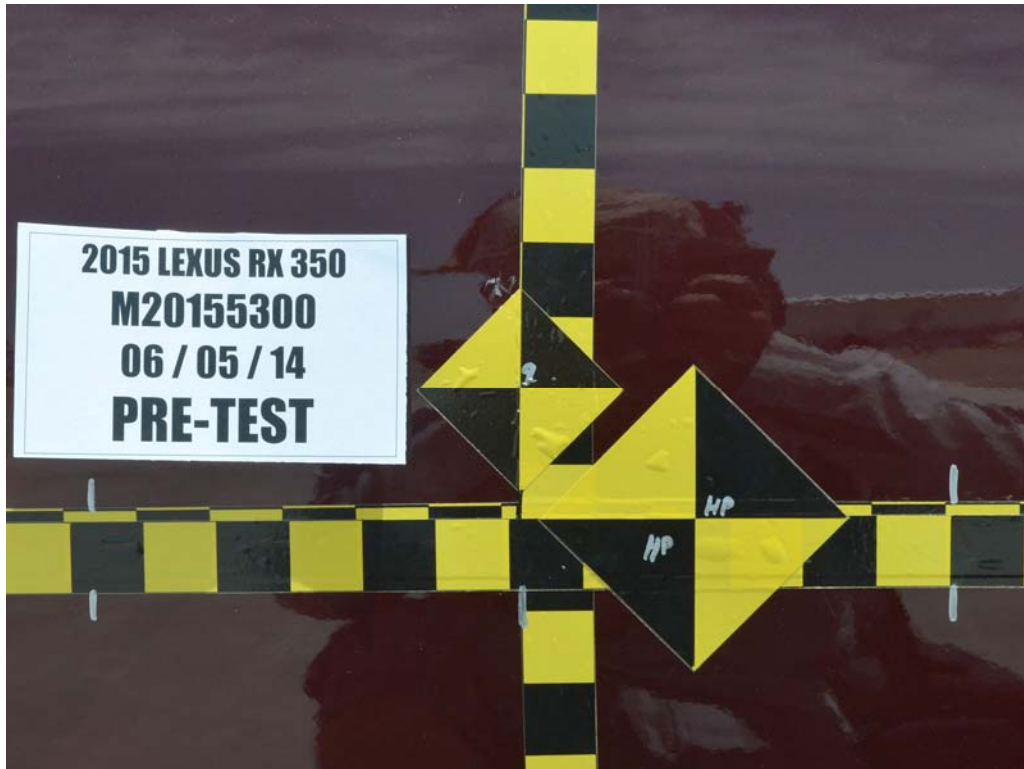
FIGURE 19. Pre-Test Close-Up View of Impact Point Target
