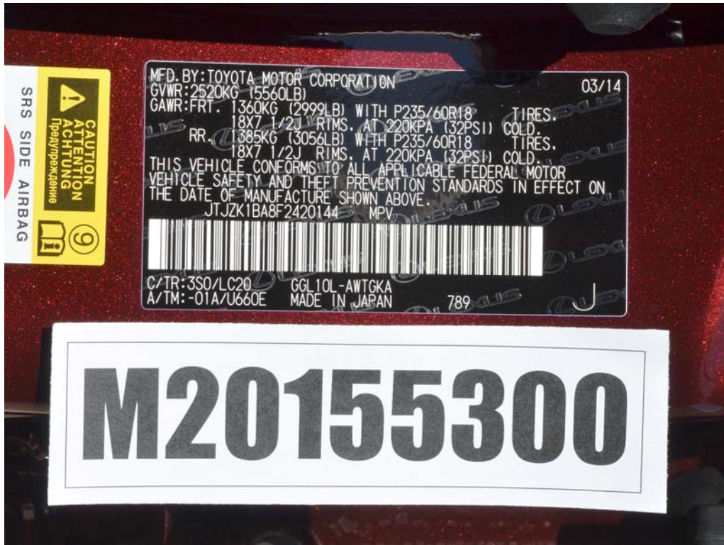
FIGURE 55. Close-Up View of Vehicle's Certification Label
