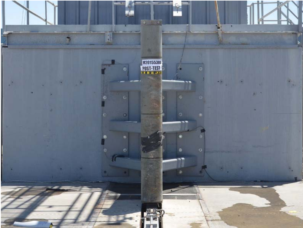
FIGURE 58. Post-Test Pole Barrier Front View
