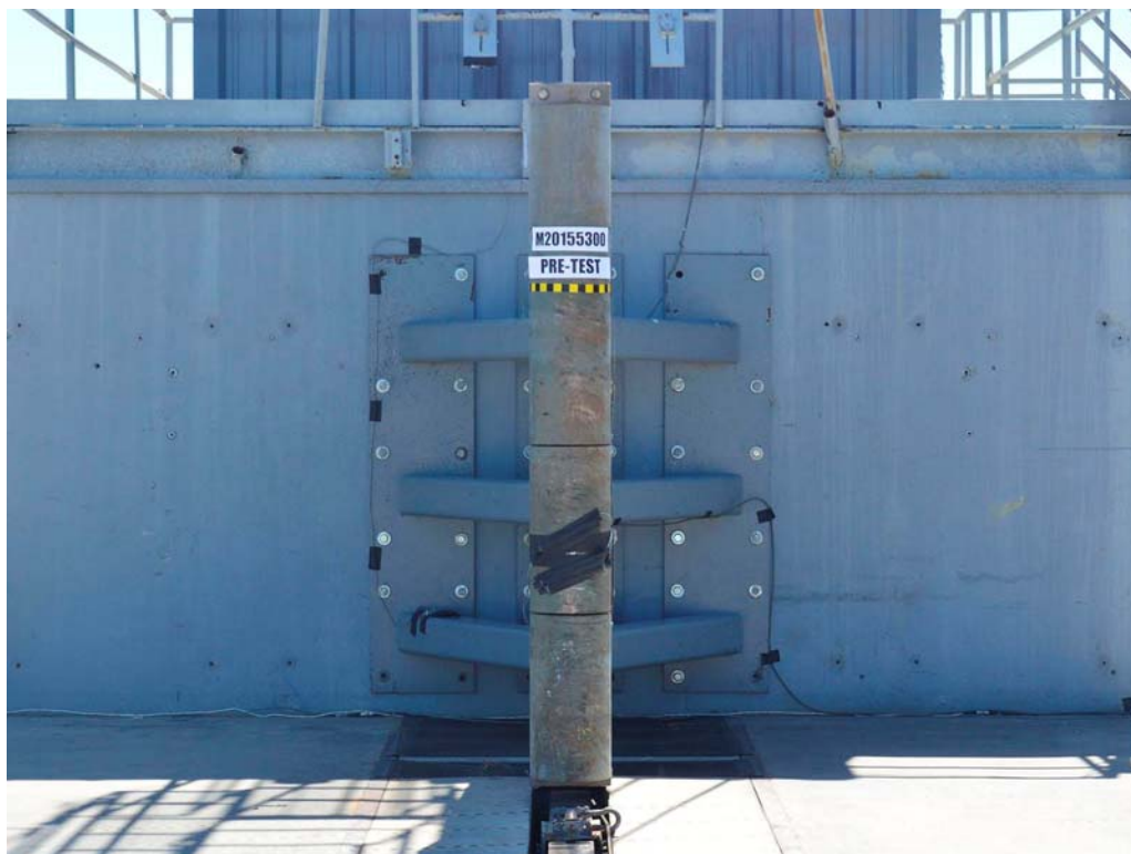
FIGURE 57. Pre-Test Pole Barrier Front View
