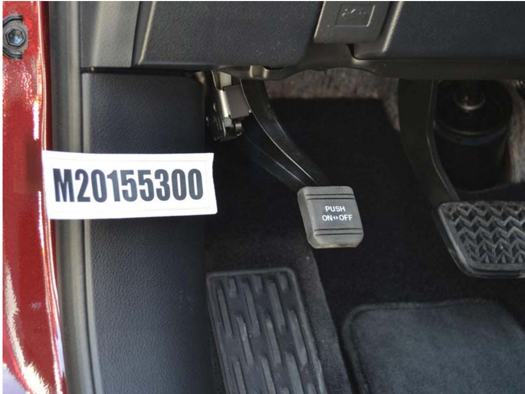
FIGURE 35. View of Disengaged Parking Brake
