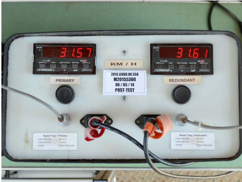
FIGURE 62. Post-Test Primary and Redundant Speed Trap Read-Out
