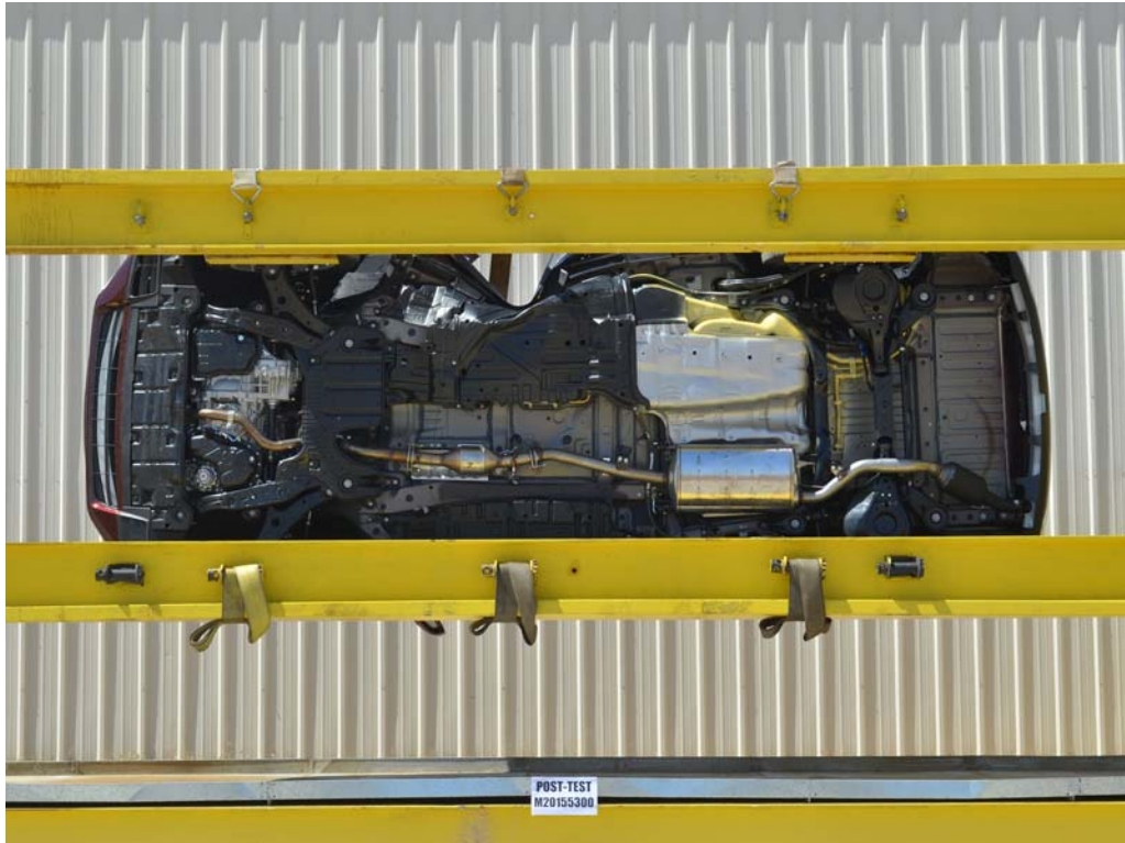
FIGURE 66. FMVSS No. 301 Static Rollover 270 Degrees
