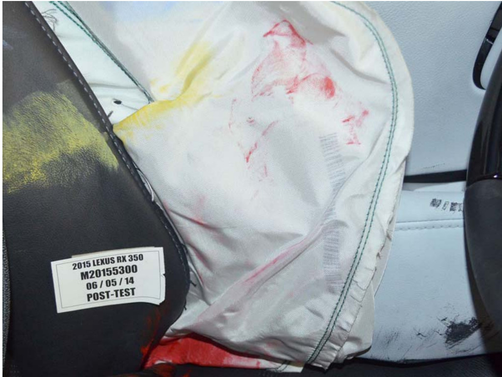
FIGURE 51. Post-Test Dummy Close-Up Pelvis Contact With Side Airbag View
