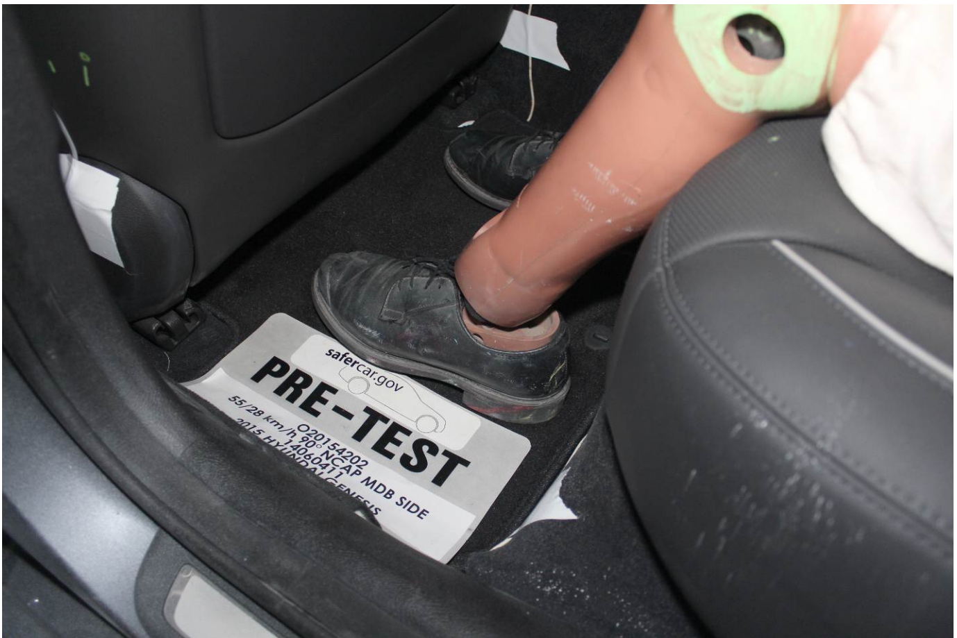
Pre-Test Placement of Rear Passenger Dummy's Feet
