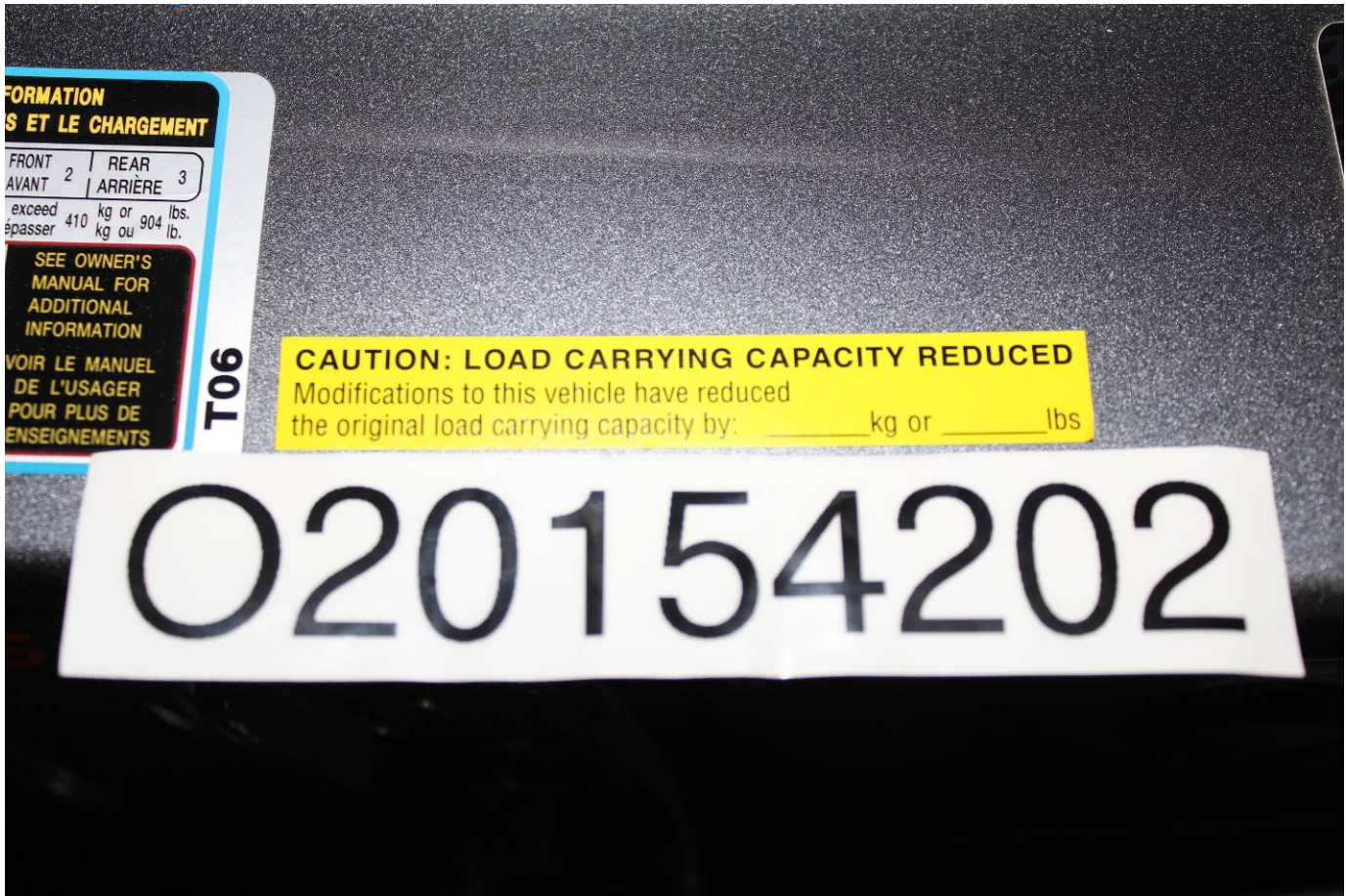
Close-Up View of Load Carrying Capacity Reduced Label
