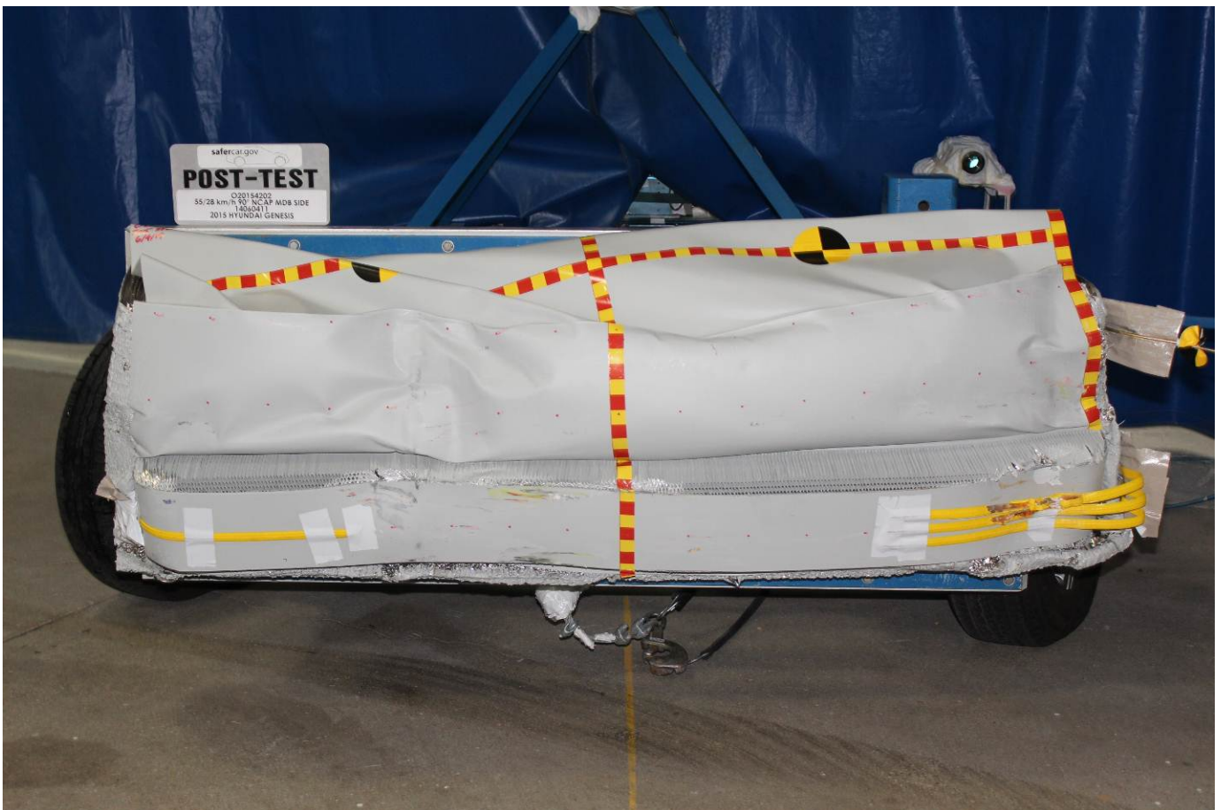
Post-Test Front View of MDB Impactor Face
