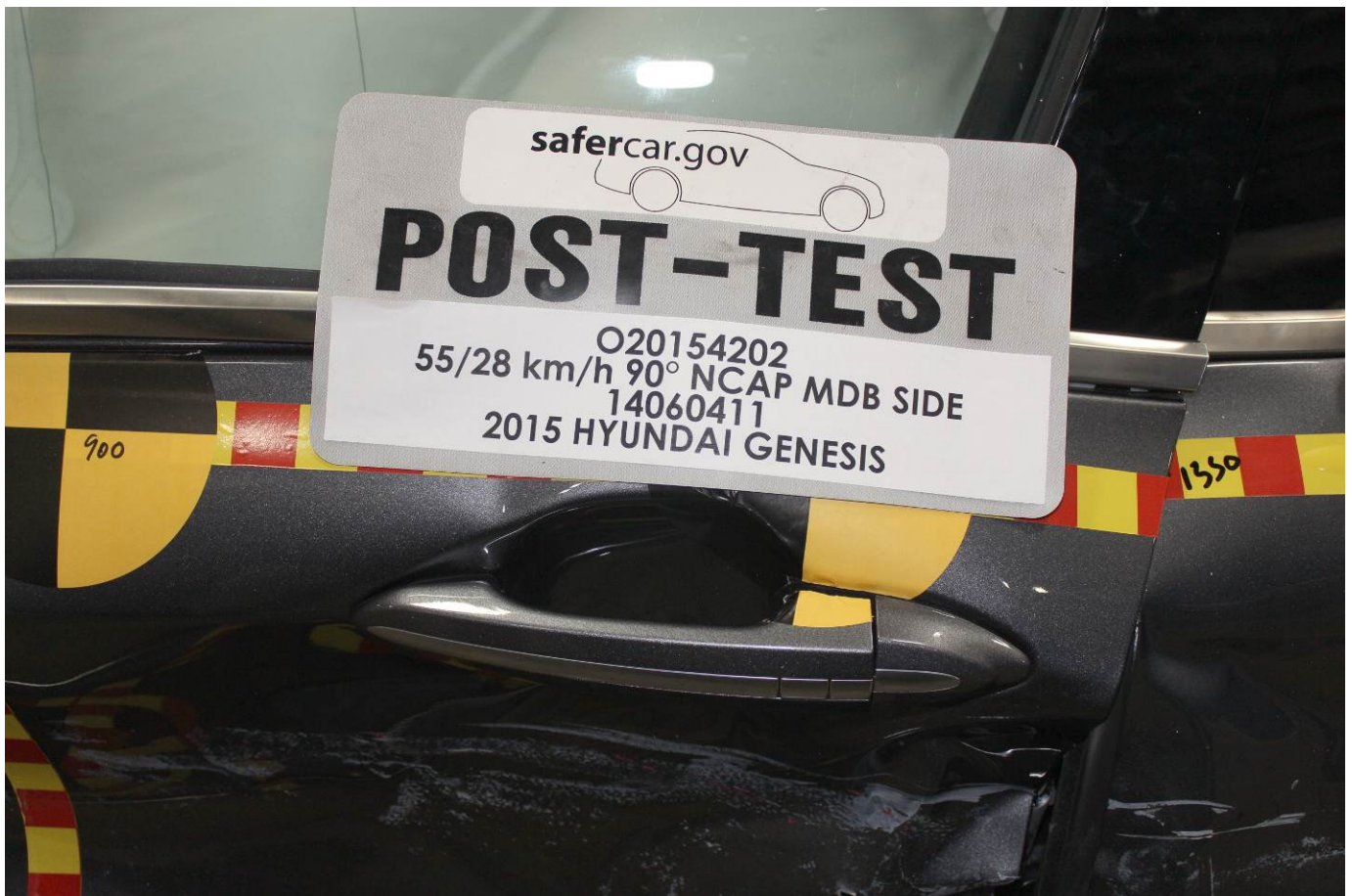
Post-Test Left Front Door Latch Close-Up
