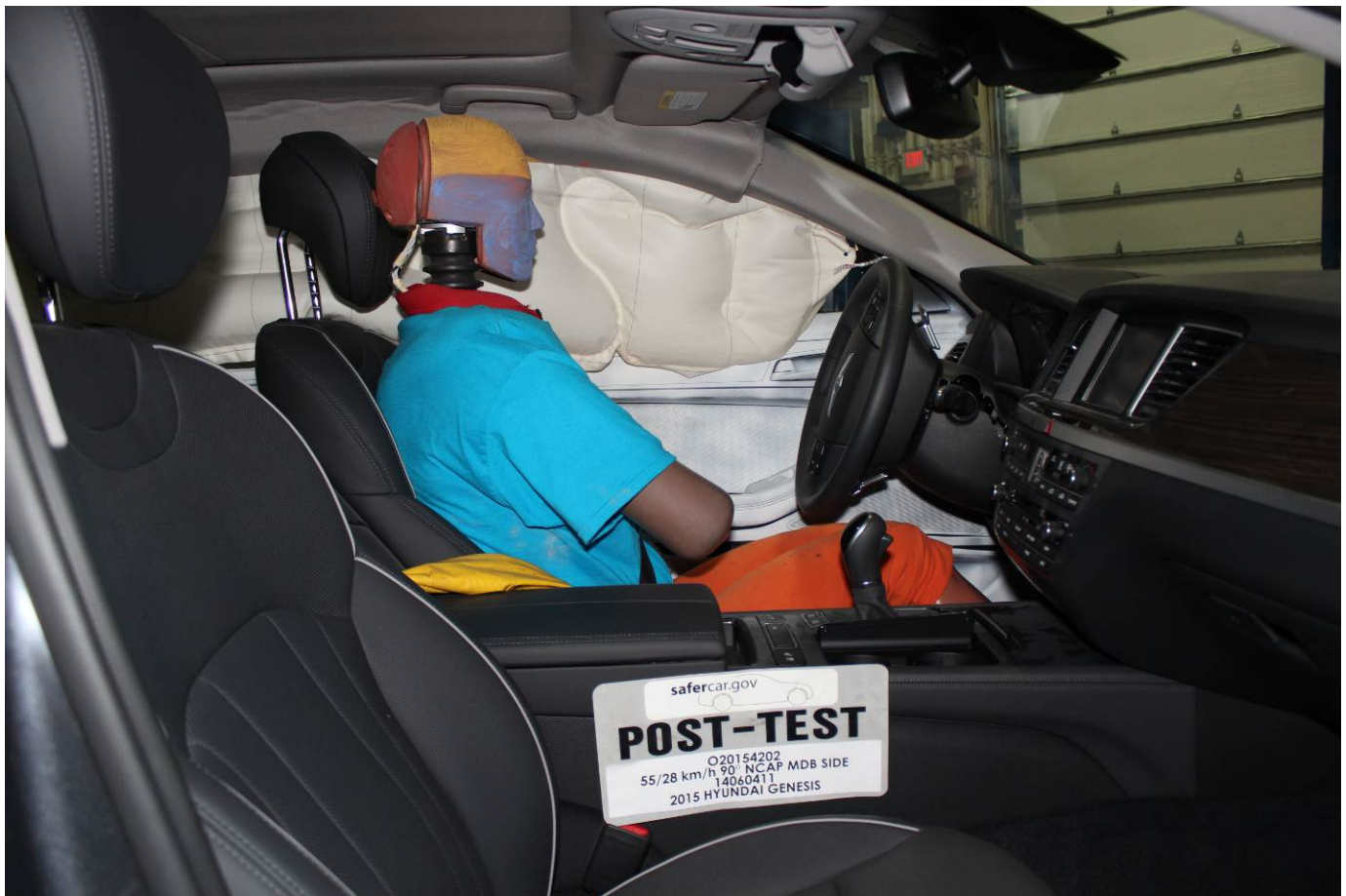
Post-Test Right Side View of Driver Dummy and Front Seat of Occupant Compartment
