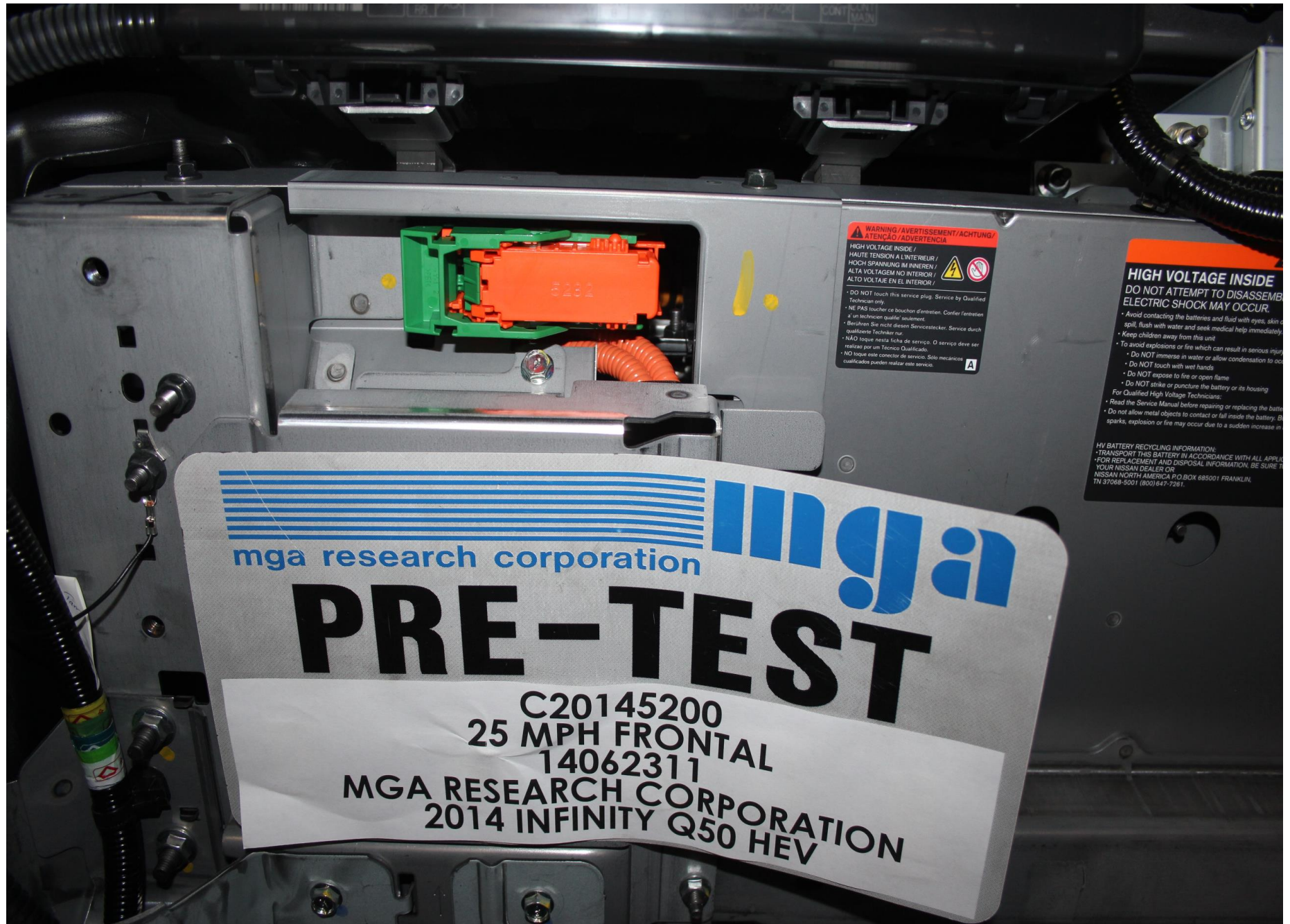
Manual High Voltage Service Disconnect Plug
