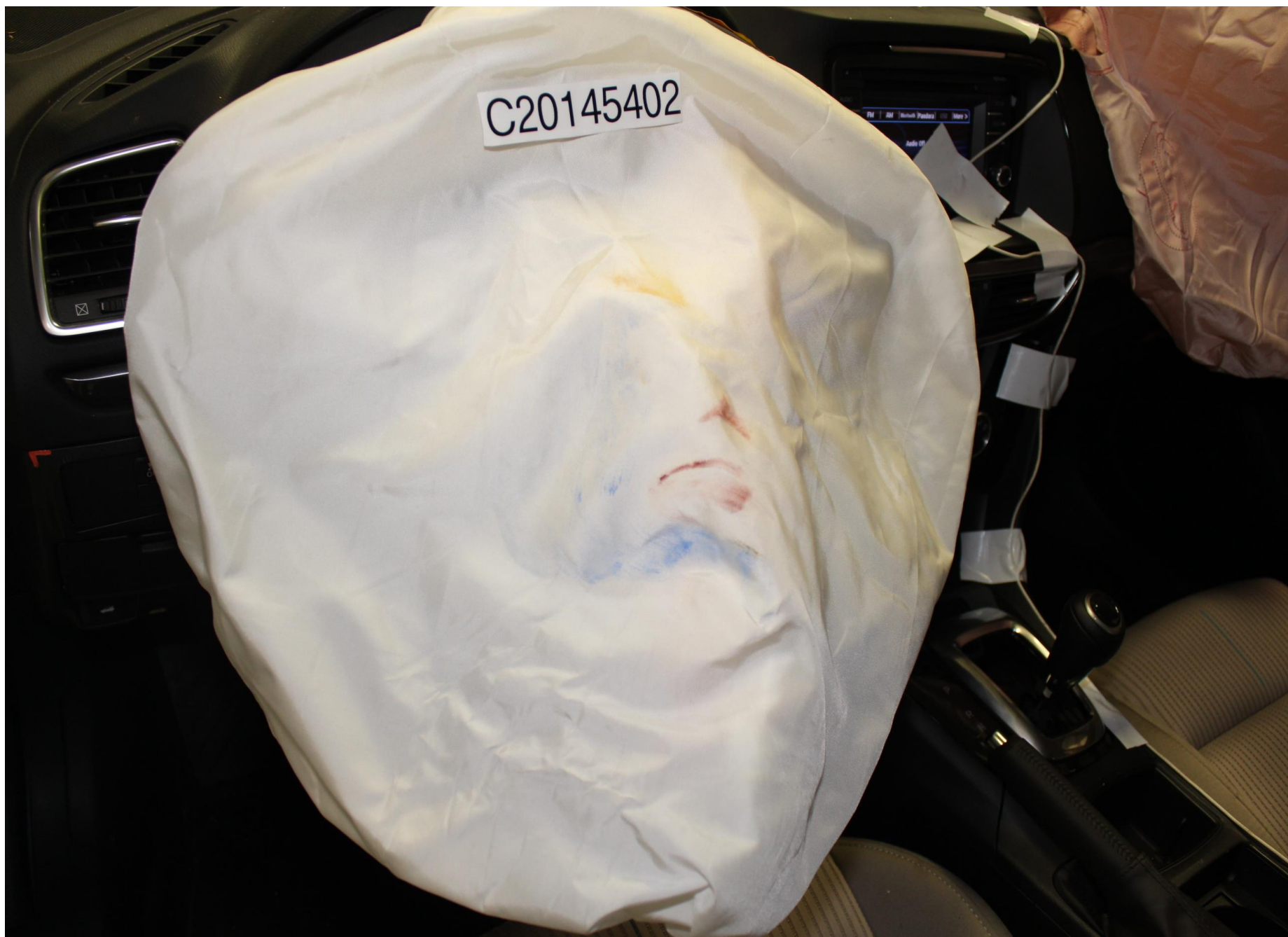
Post-Test Driver Dummy Airbag Contact
