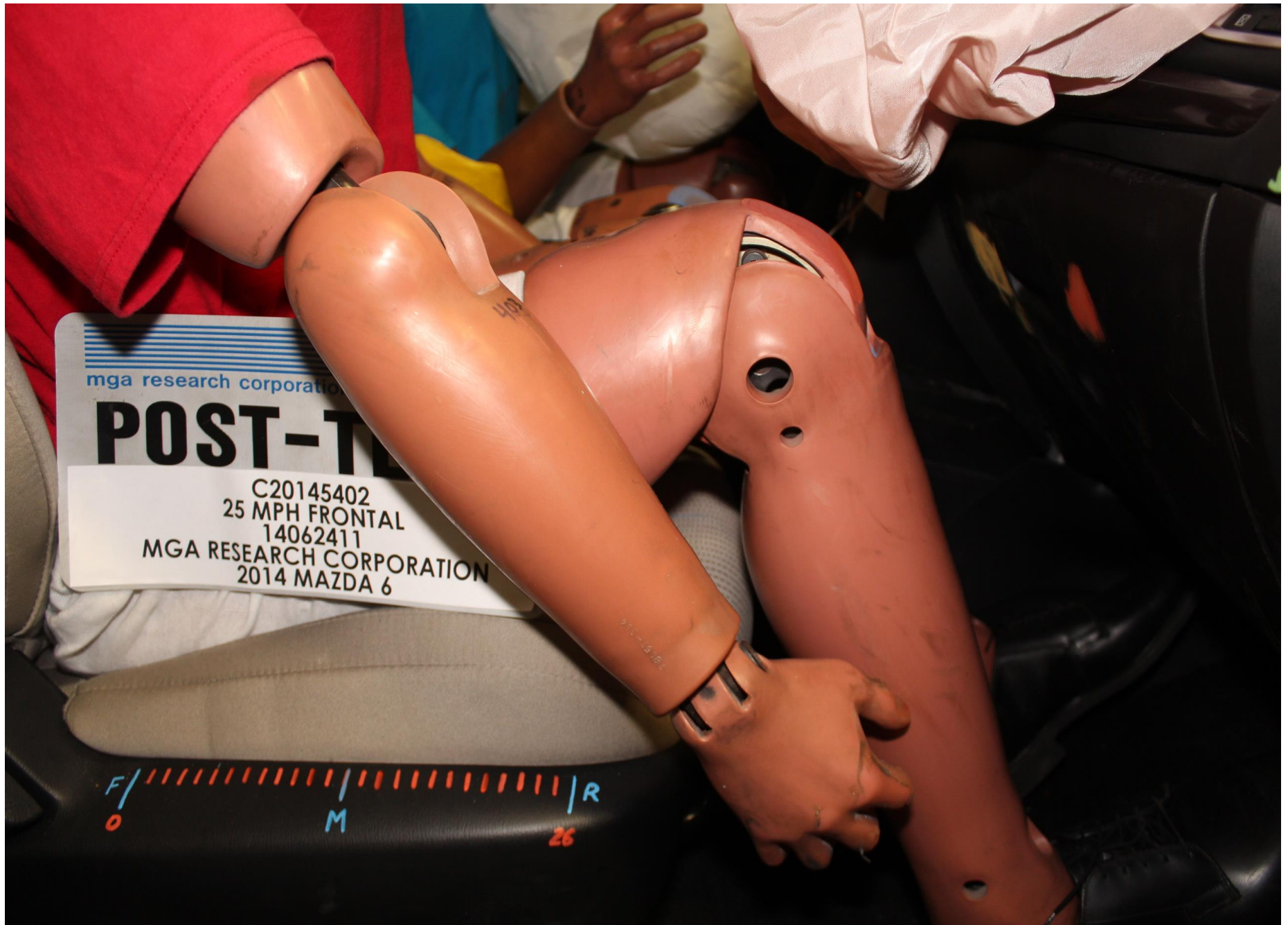
Post-Test Passenger Side Knee Bolster View
