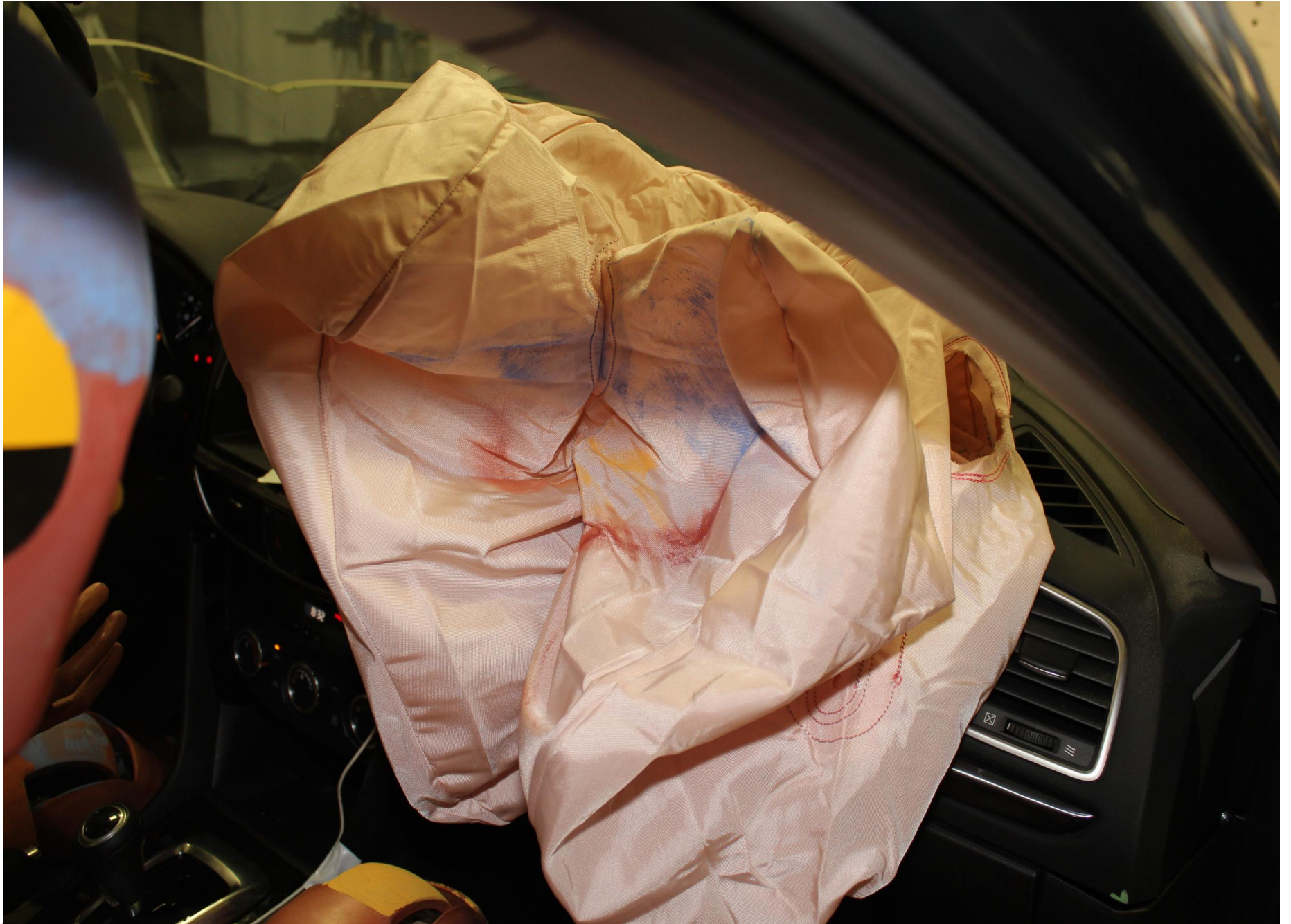
Post-Test Passenger Dummy Airbag Contact
