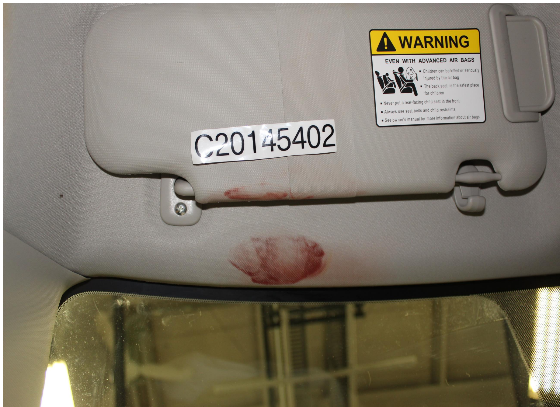
Post-Test Driver Dummy Head Contact (headliner/visor)
