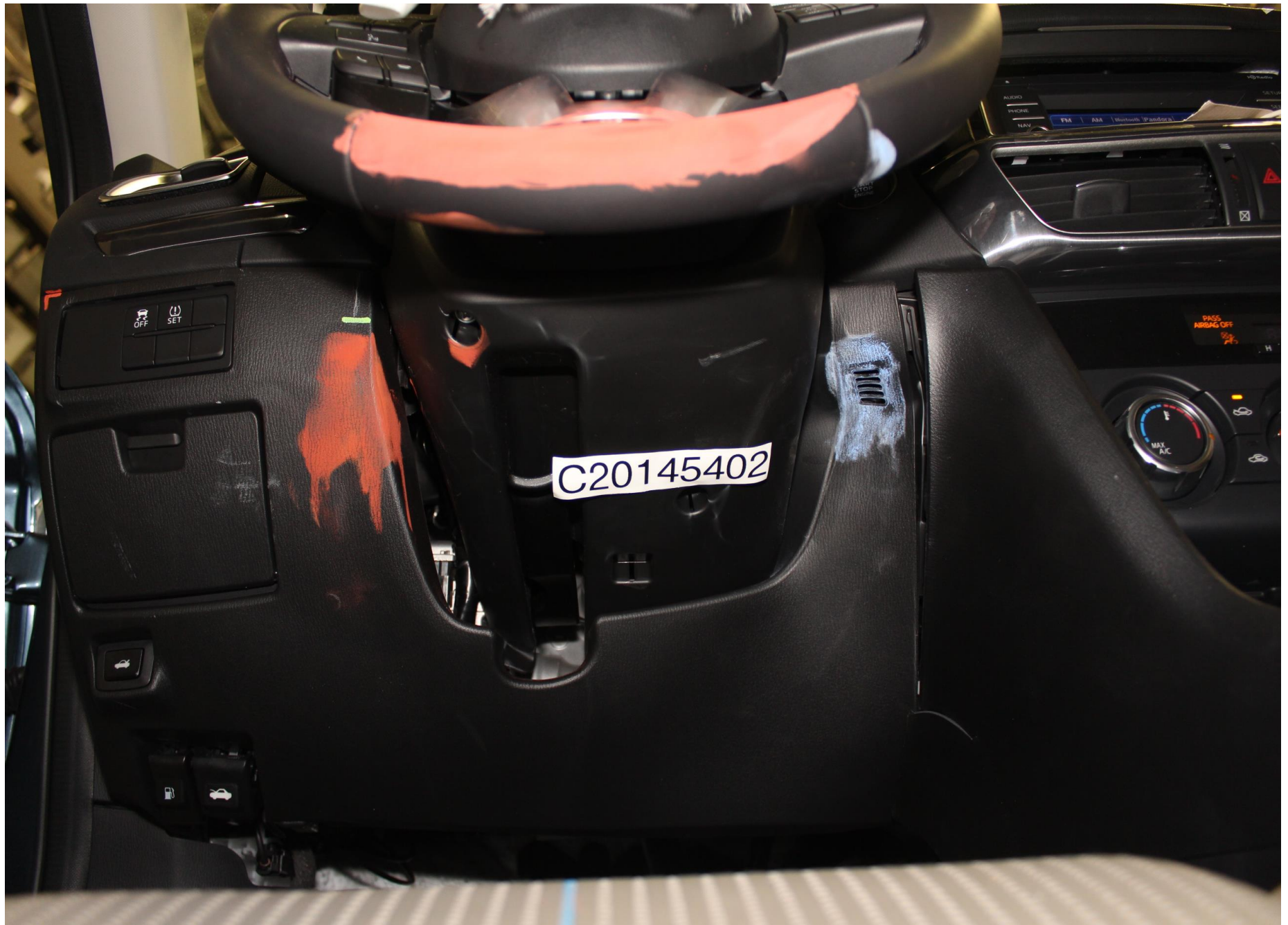
Post-Test Driver Dummy Knee Contact (knee bolster)
