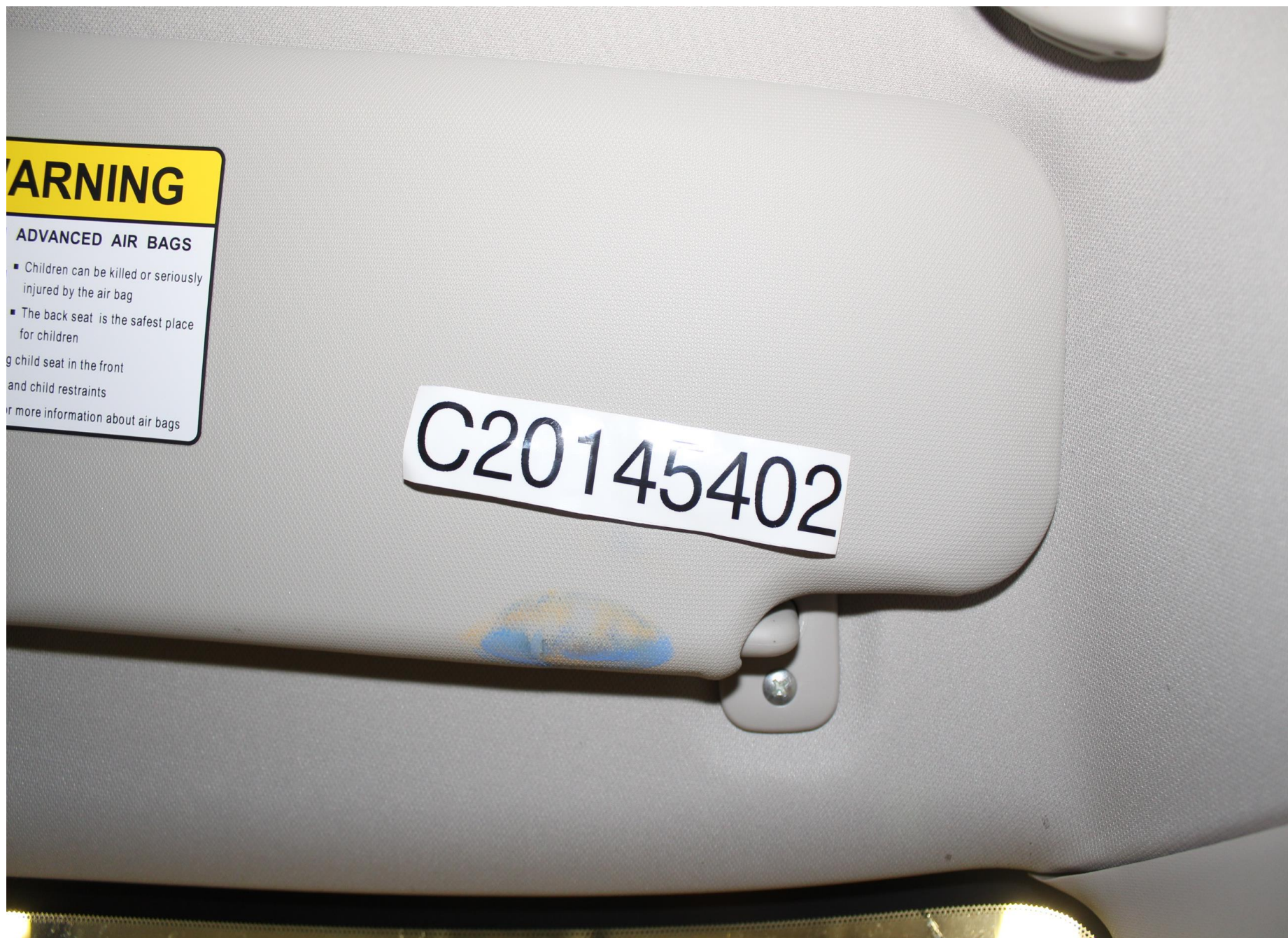
Post-Test Passenger Dummy Head Contact (visor)
