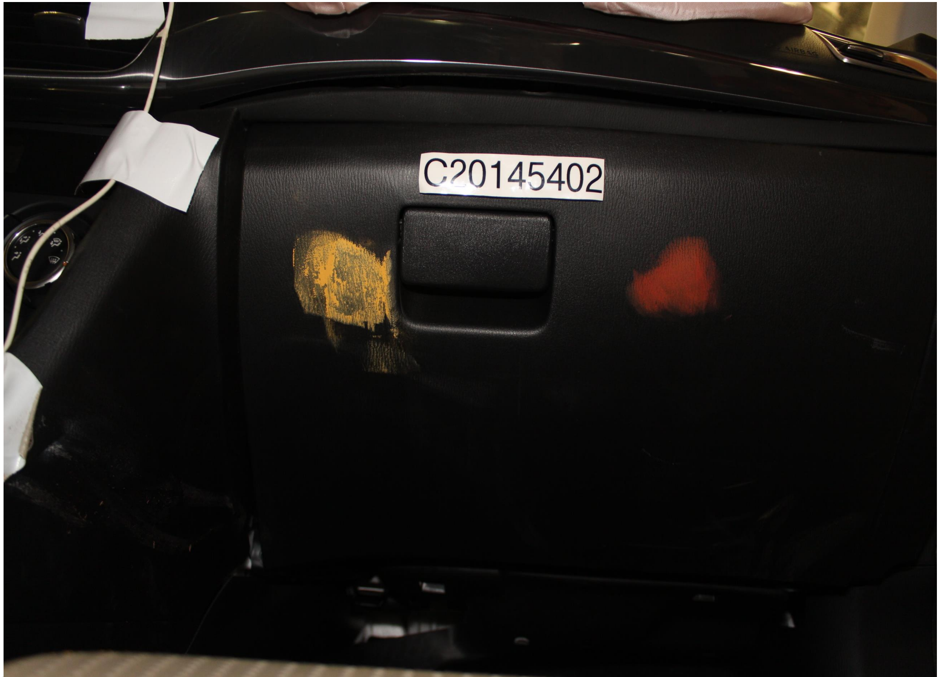
Post-Test Passenger Dummy Knee Contact (glove box)
