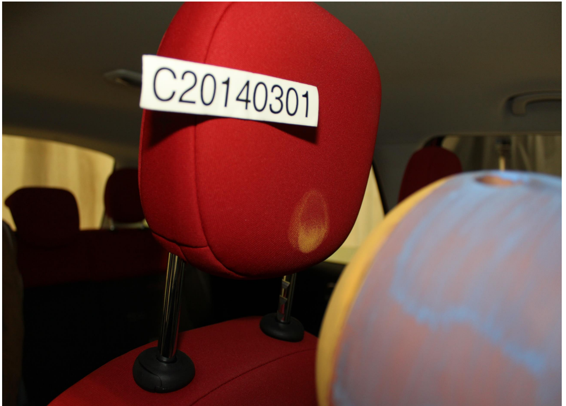
Post-Test Passenger Dummy Head Contact (headrest)
