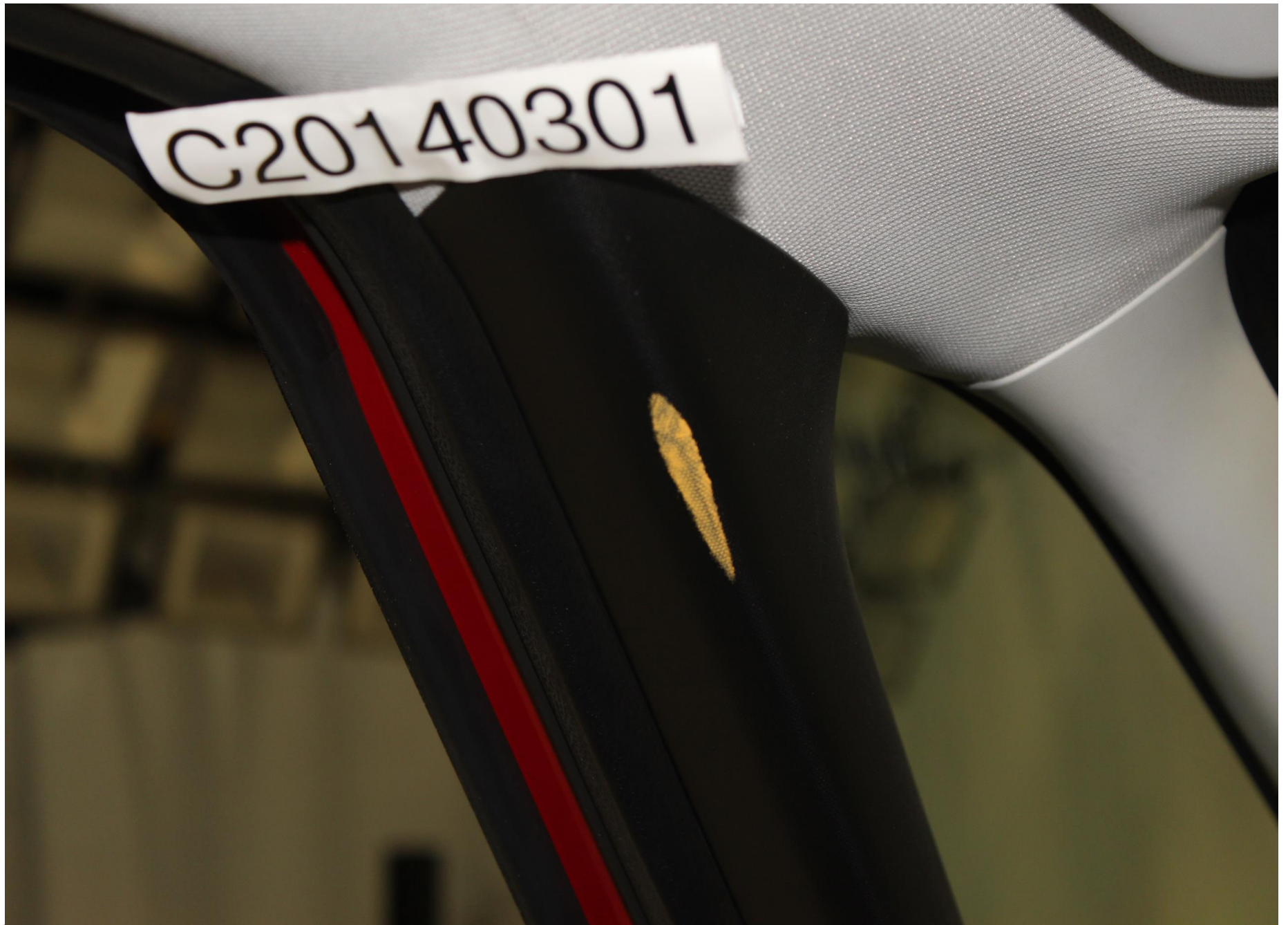
Post-Test Driver Dummy Head Contact (A-pillar)
