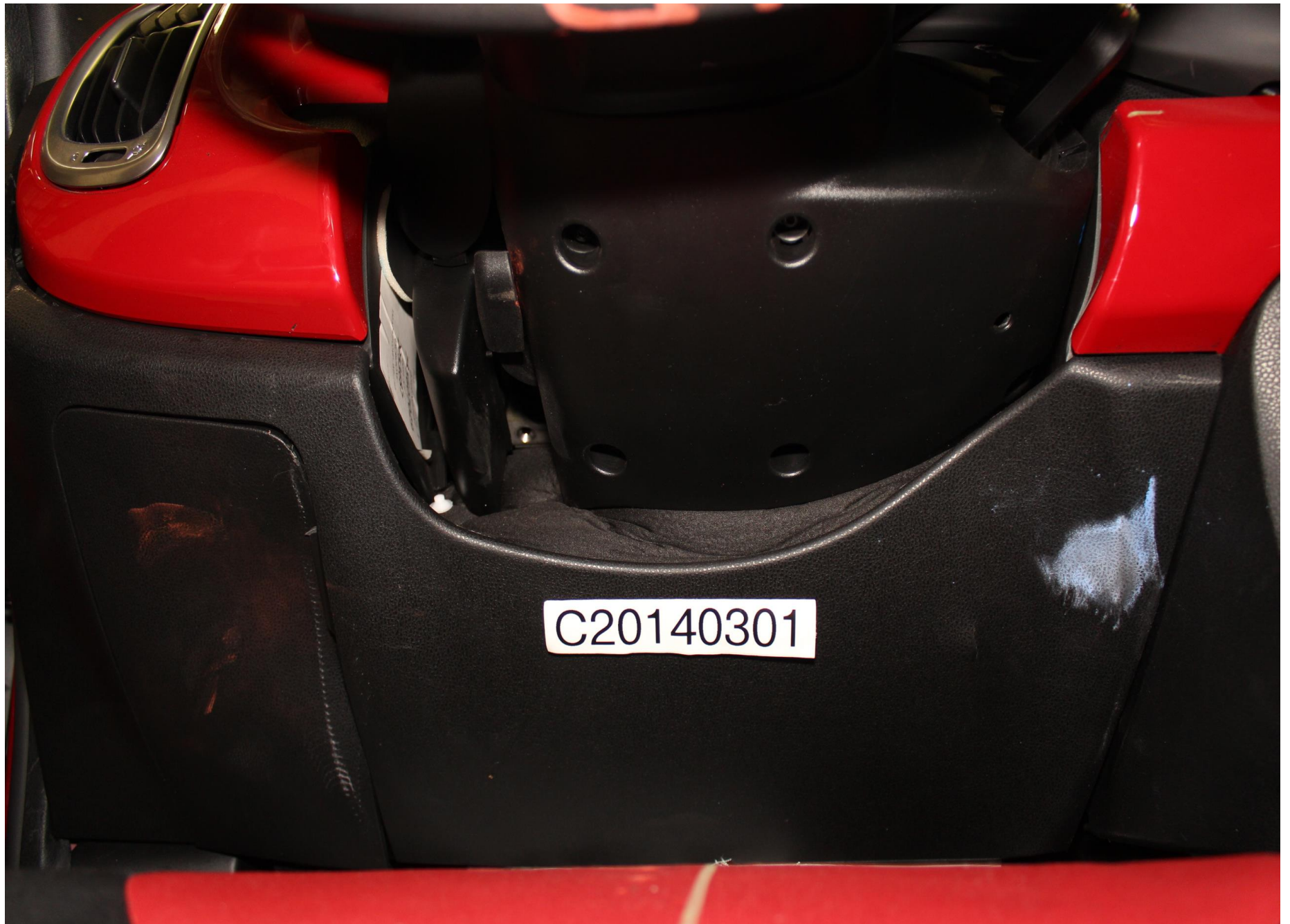
Post-Test Driver Dummy Knee Contact (knee bolster)
