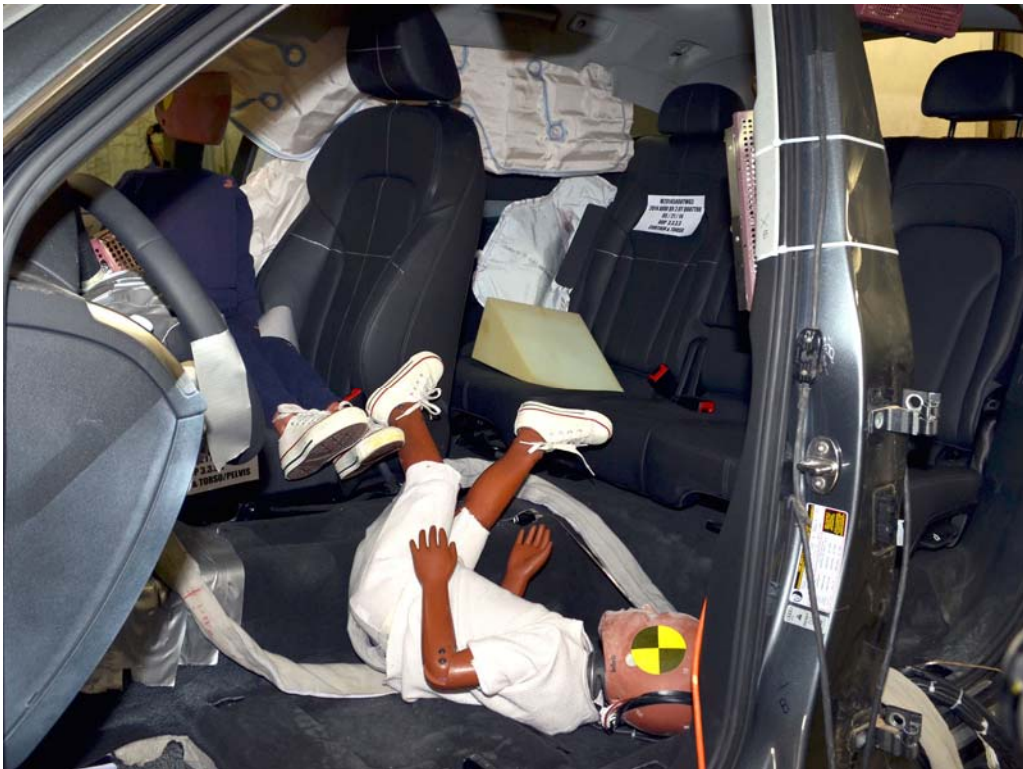
FIGURE 10. Post-Test Dummy Position, \frac{3}{4} View
