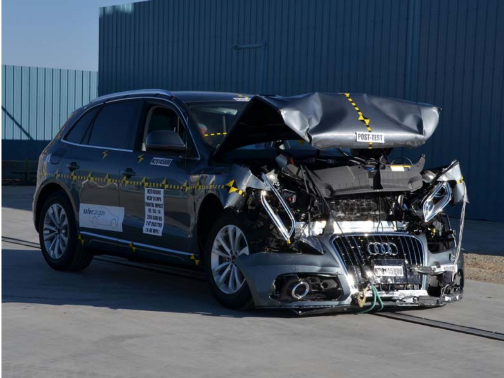
FIGURE 3. Post-Test Right Front 3/4 View of NCAP Frontal Impact Test
