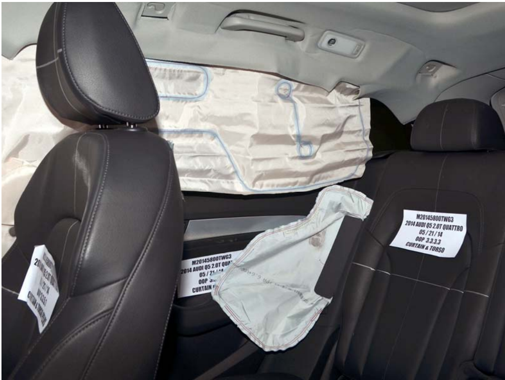
FIGURE 14. Post-Test Airbags, Left Front 3/4 View
