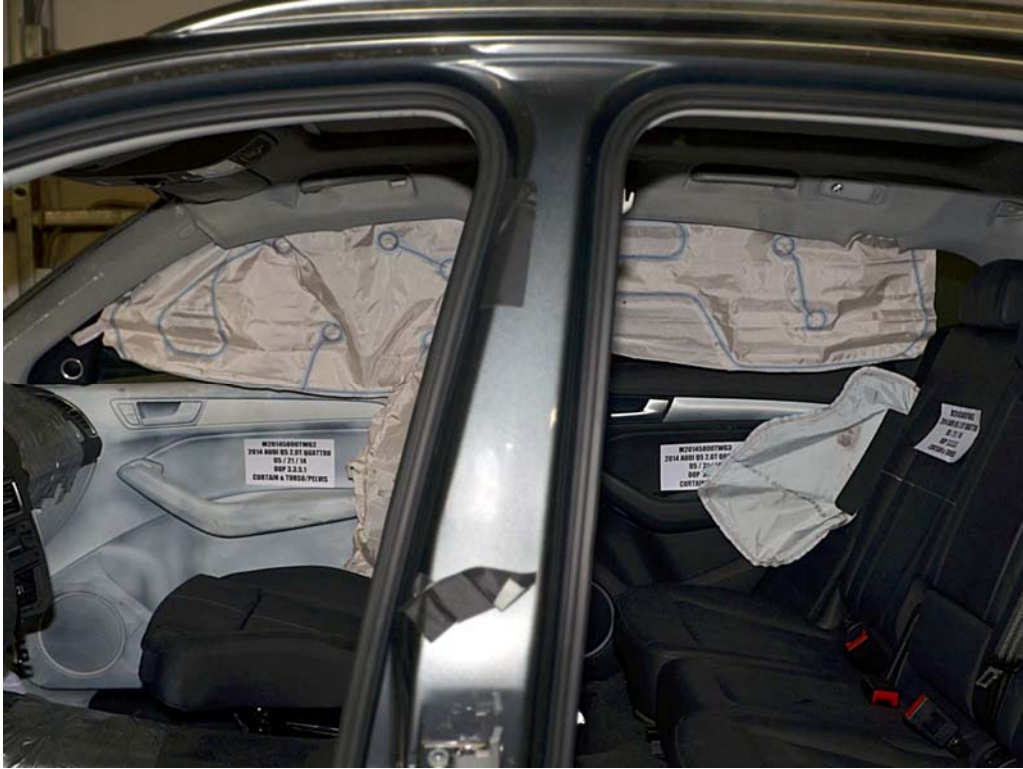
FIGURE 13. Post-Test Airbags, Left Side View
