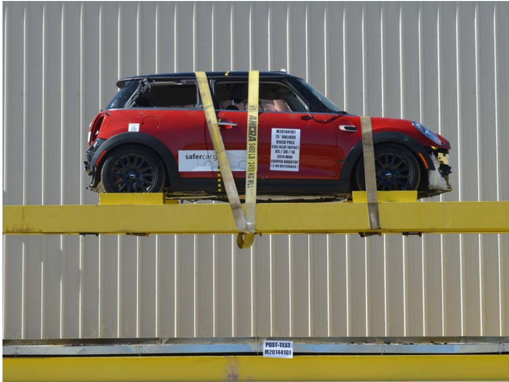
FIGURE 67. FMVSS No. 301 Static Rollover 360 Degrees
