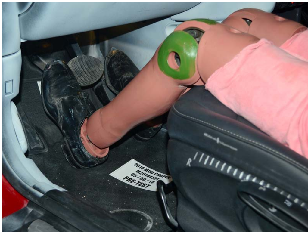
FIGURE 32. Pre-Test Placement of Dummy's Feet
