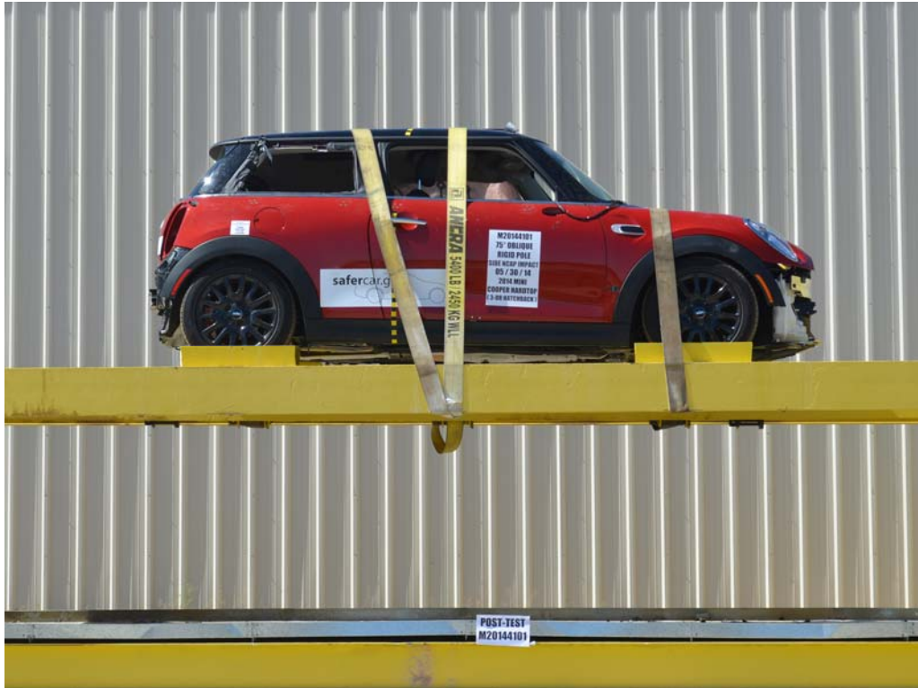
FIGURE 63. FMVSS No. 301 Static Rollover 0 Degrees
