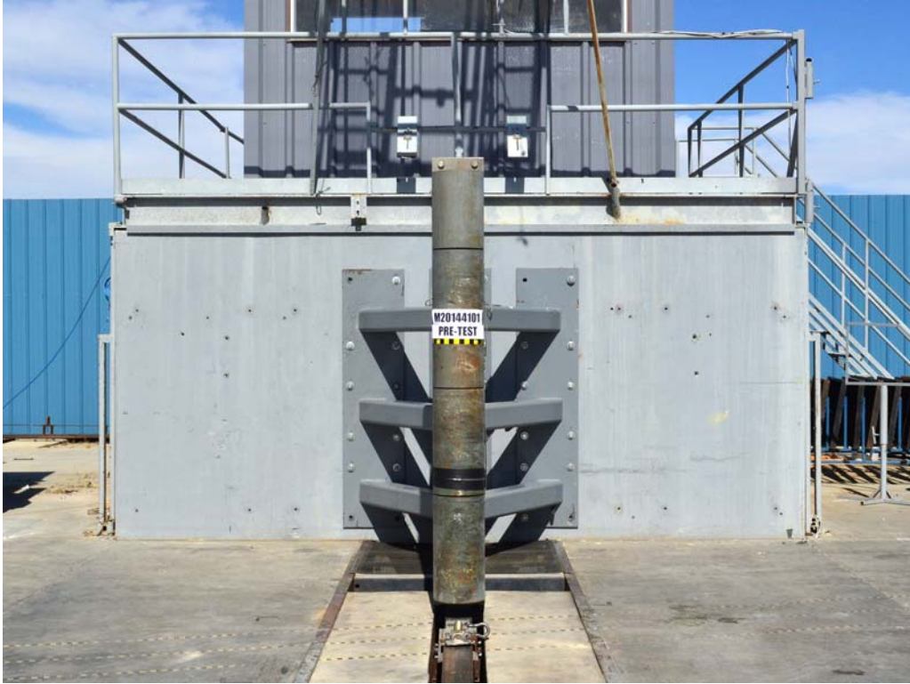
FIGURE 57. Pre-Test Pole Barrier Front View
