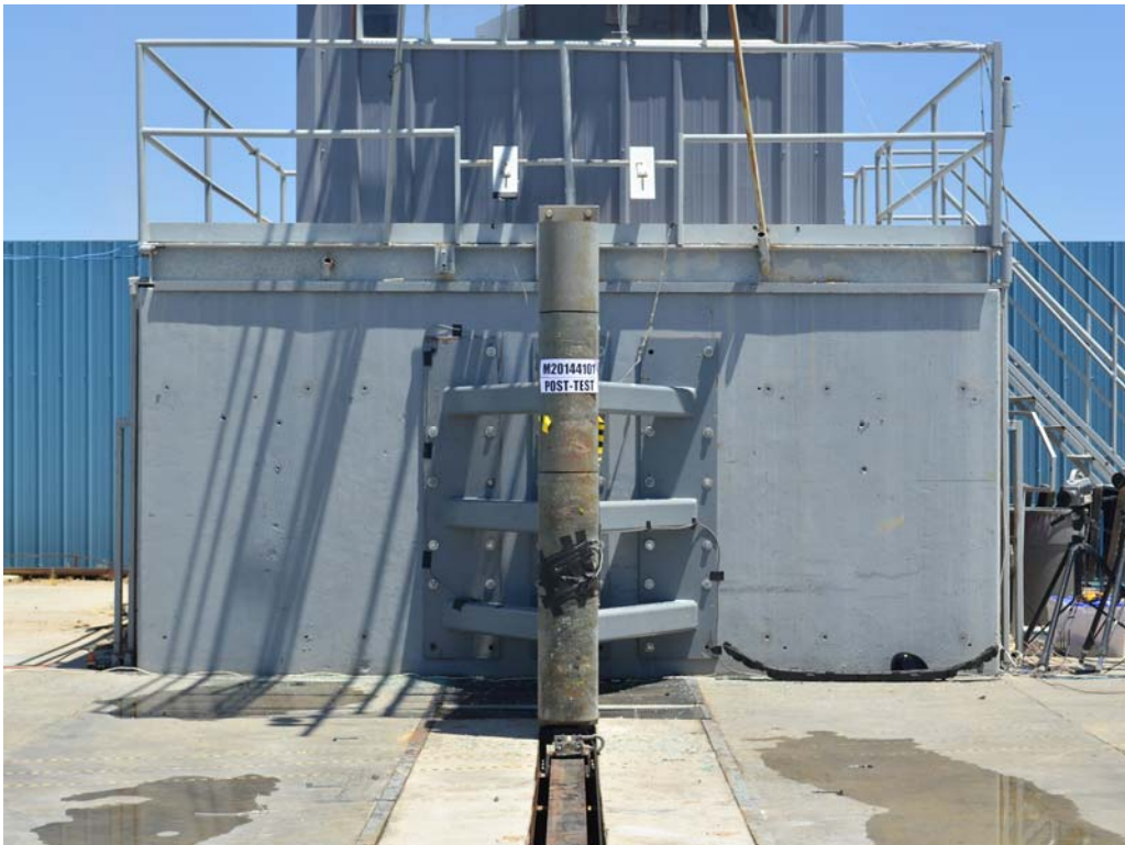
FIGURE 58. Post-Test Pole Barrier Front View
