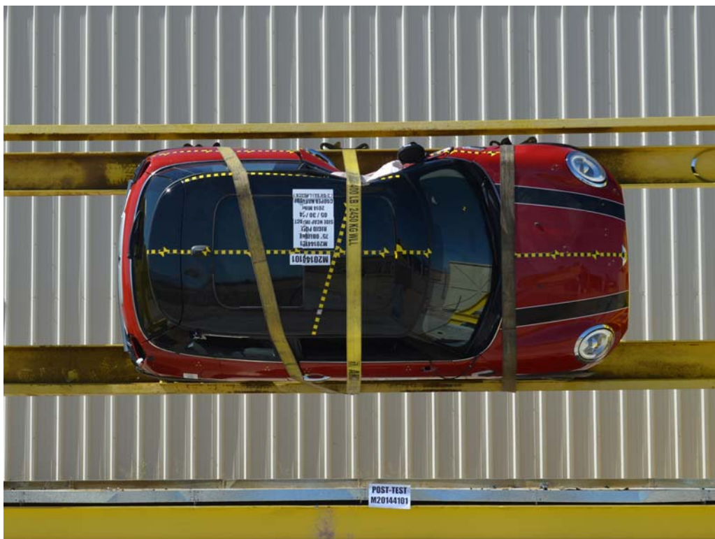
FIGURE 64. FMVSS No. 301 Static Rollover 90 Degrees
