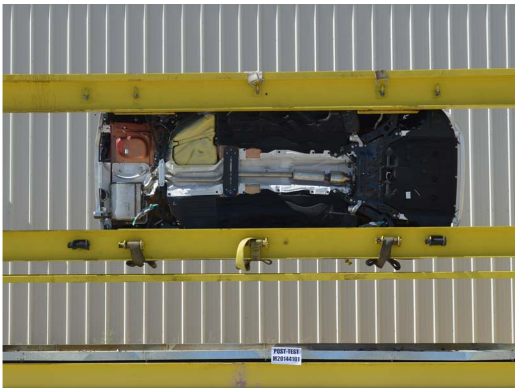
FIGURE 66. FMVSS No. 301 Static Rollover 270 Degrees
