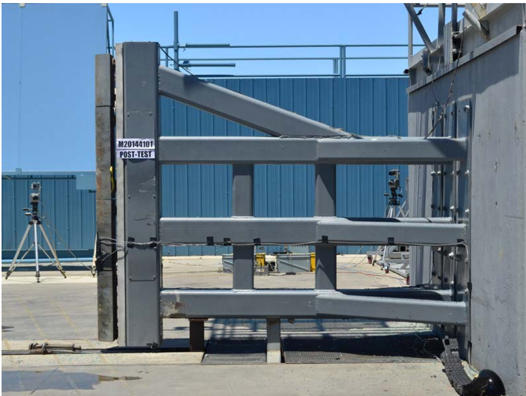
FIGURE 60. Post-Test Pole Barrier Side View
