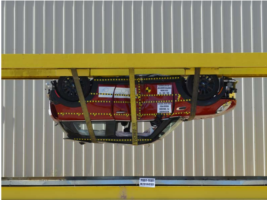
FIGURE 65. FMVSS No. 301 Static Rollover 180 Degrees
