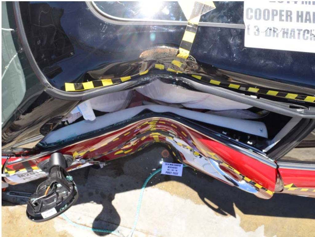
FIGURE 41. Post-Test Dummy and Door Clearance View
