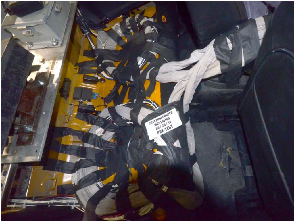
FIGURE 27. Pre-Test Dummy Cable Routing
