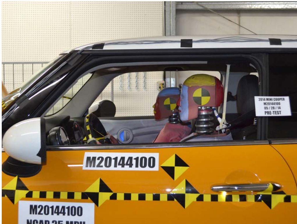
FIGURE 31. Pre-Test Driver Dummy Window View
