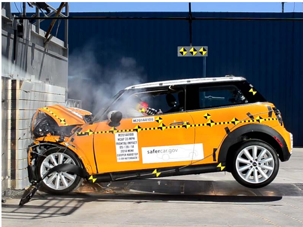
FIGURE 77. 2014 Mini Cooper Hardtop Frontal Impact Event
