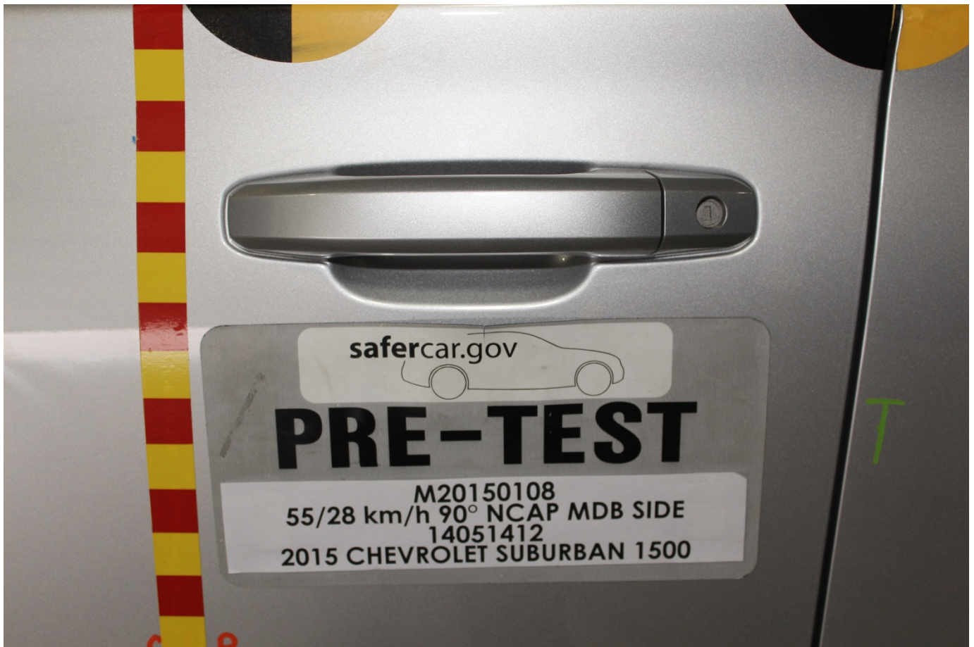
Pre-Test Left Front Door Latch Close-Up
