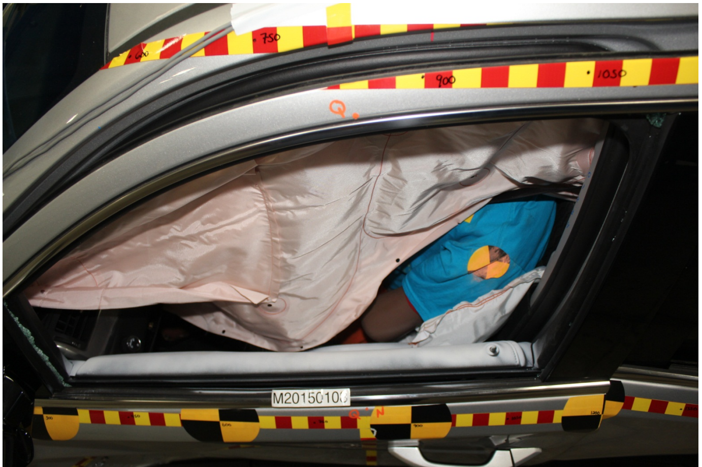
Post-Test Driver Dummy and Door Clearance View
