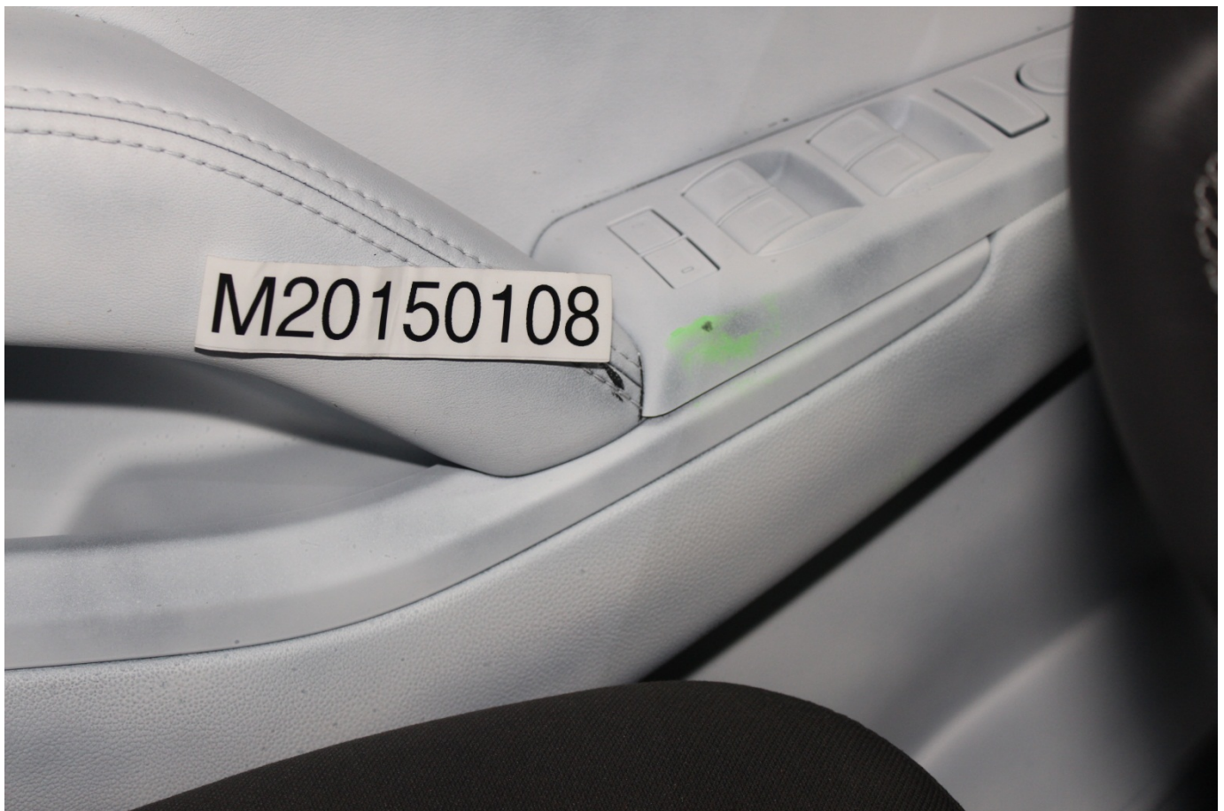
Post-Test Driver Dummy Close-up Knee Contact View
