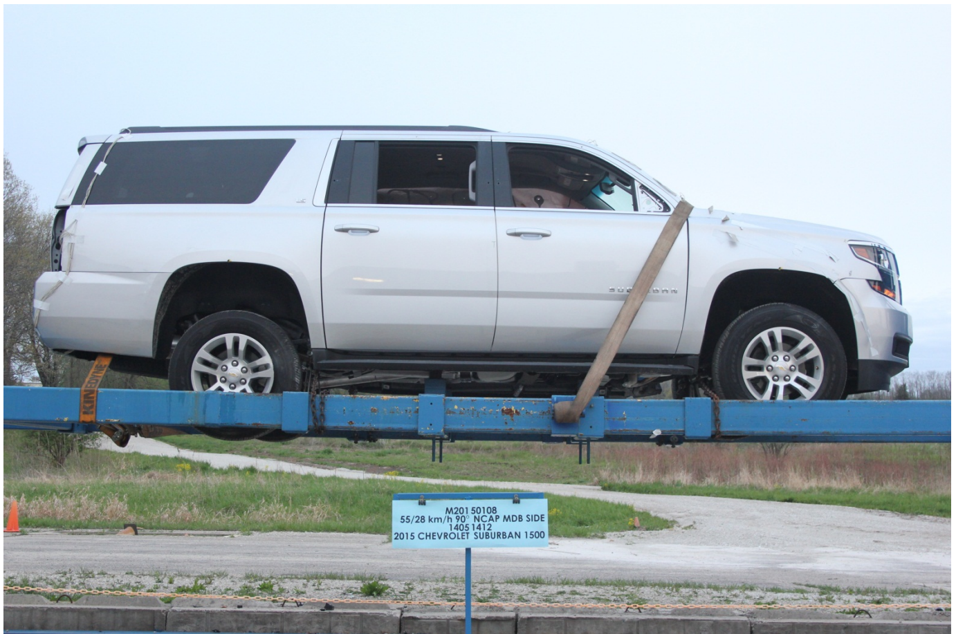
FMVSS No. 301 Static Rollover 360 Degrees
