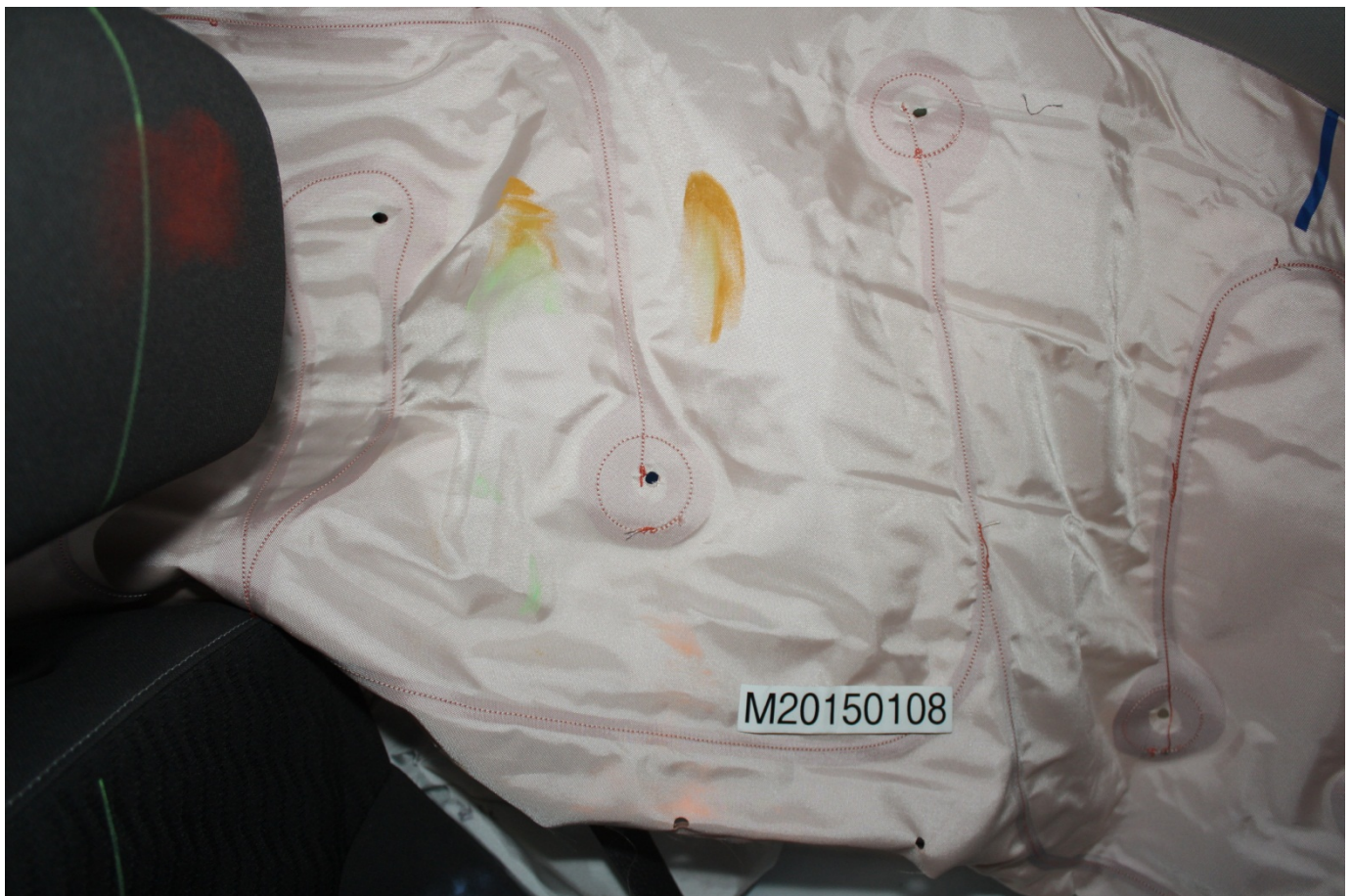
Post-Test Driver Dummy Close-up Head Contact with Side Airbag View
