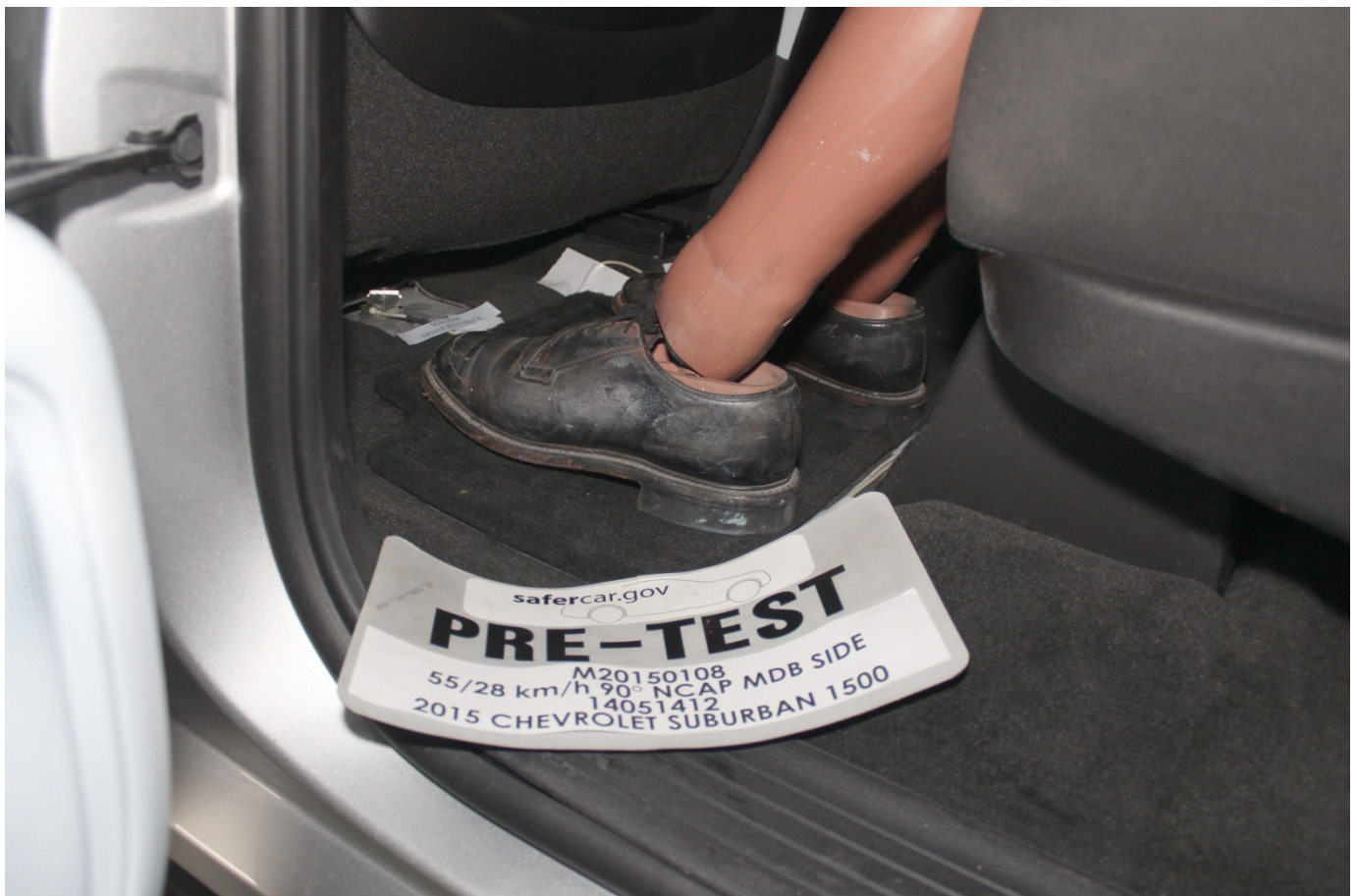
Pre-Test Placement of Rear Passenger Dummy's Feet
