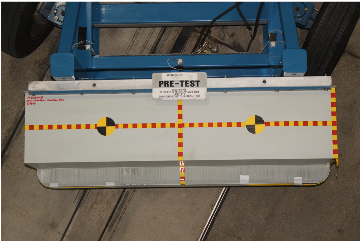
Pre-Test Top View of MDB Impactor Face
