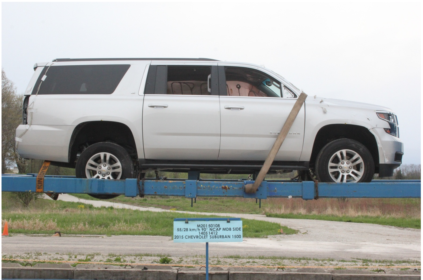
FMVSS No. 301 Static Rollover 0 Degrees
