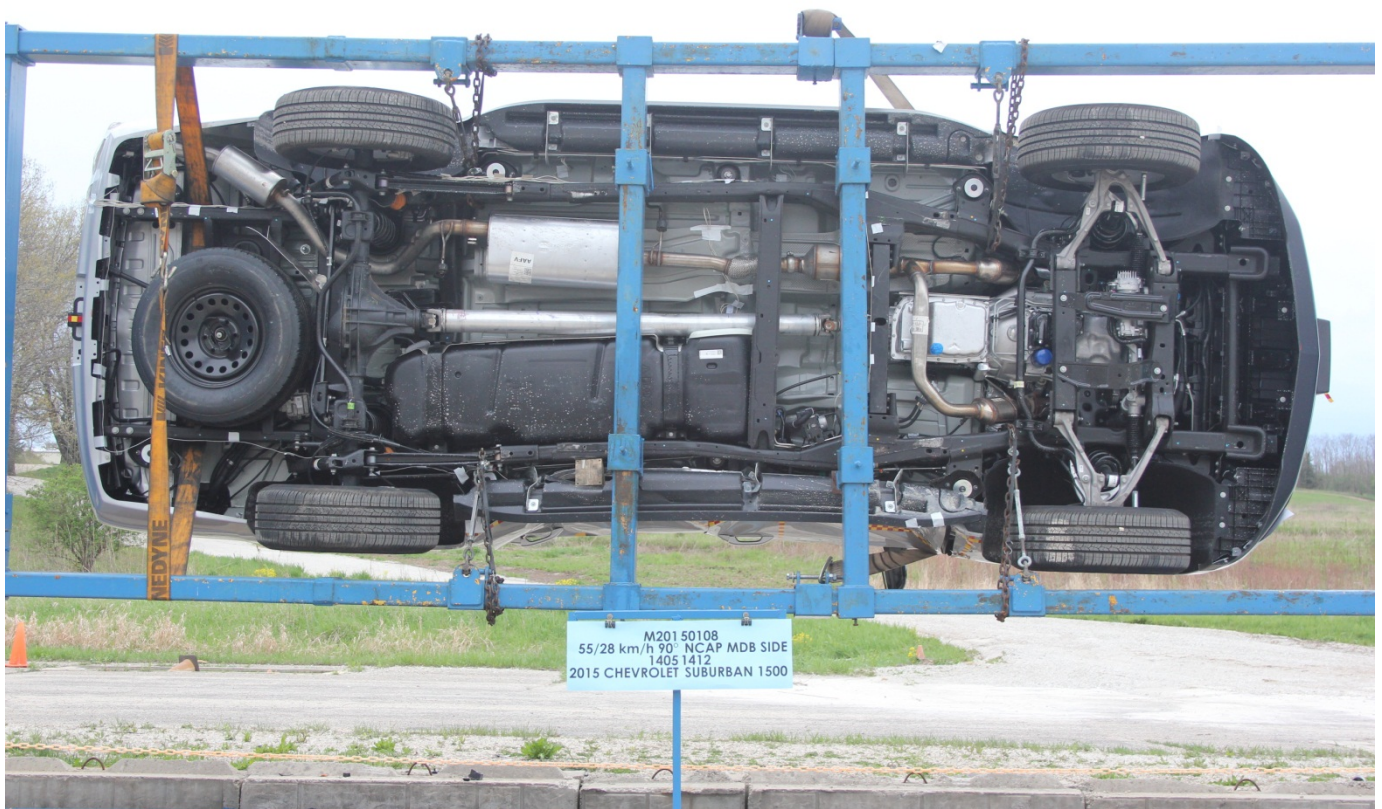
FMVSS No. 301 Static Rollover 90 Degrees
