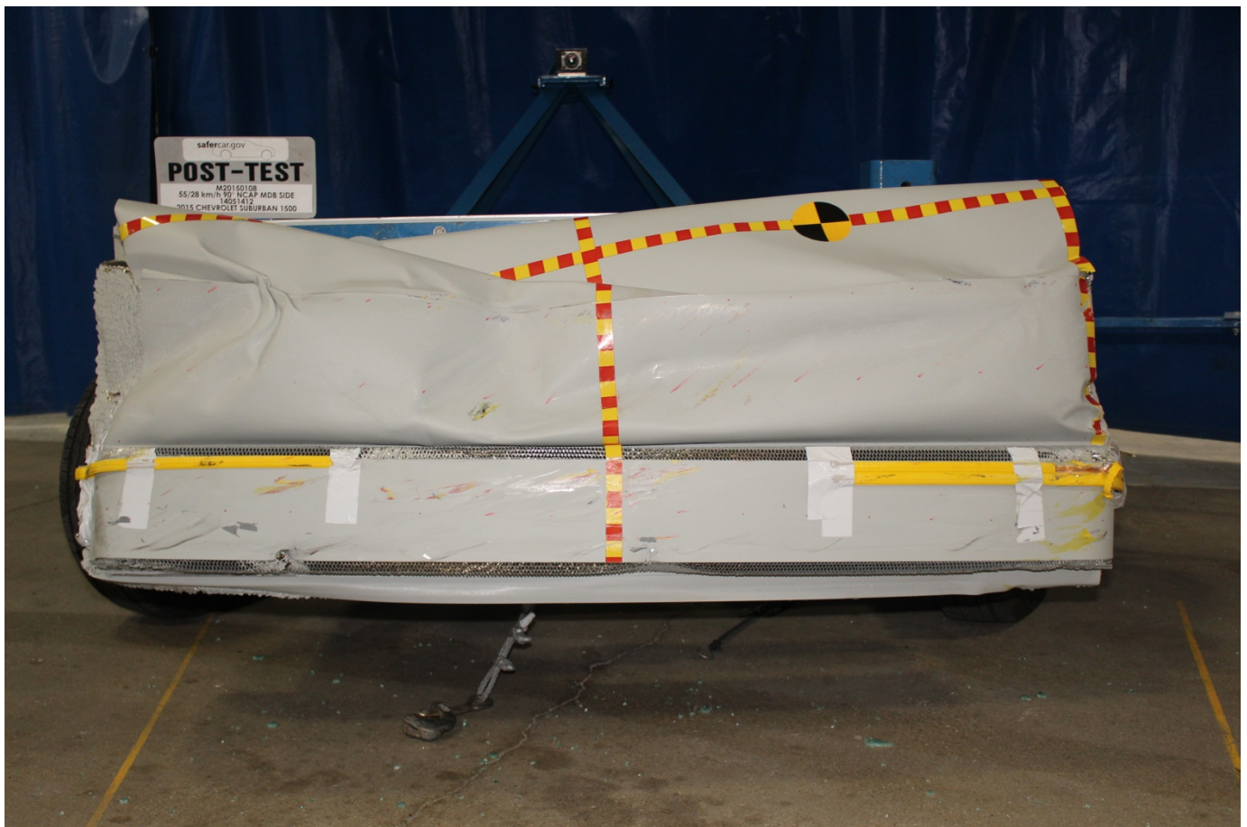
Post-Test Front View of MDB Impactor Face
