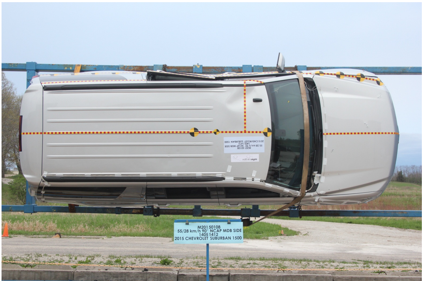
FMVSS No. 301 Static Rollover 270 Degrees
