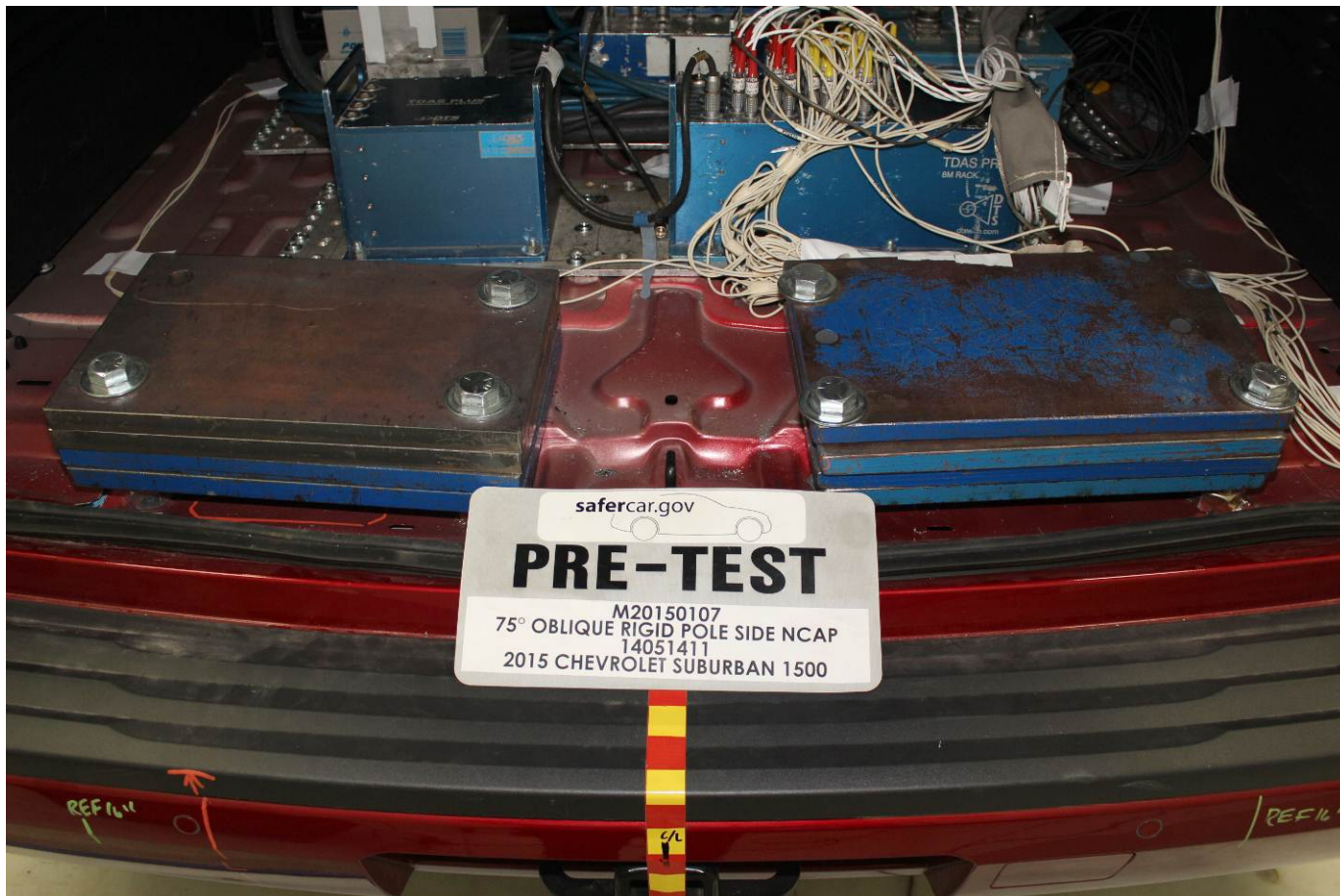
Pre-Test Ballast View
