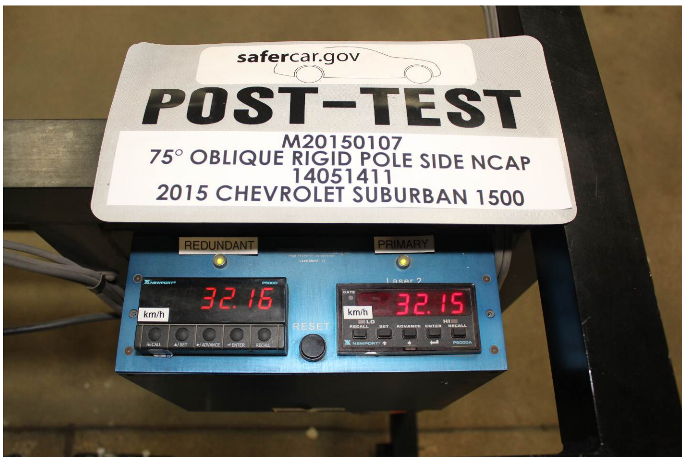
Post-Test Primary and Redundant Speed Trap Read-Out
