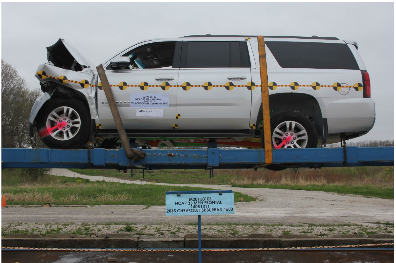
Vehicle at 0 Degree on Static Rollover Device
