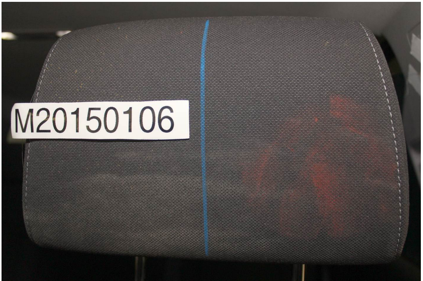
Post-Test Driver Dummy Contact with Headrest
