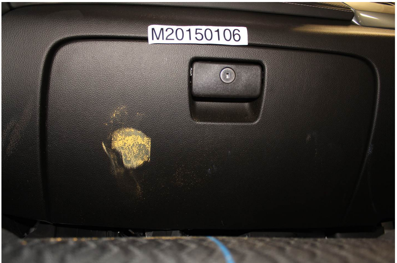
Post-Test Passenger Dummy Contact with Glovebox
