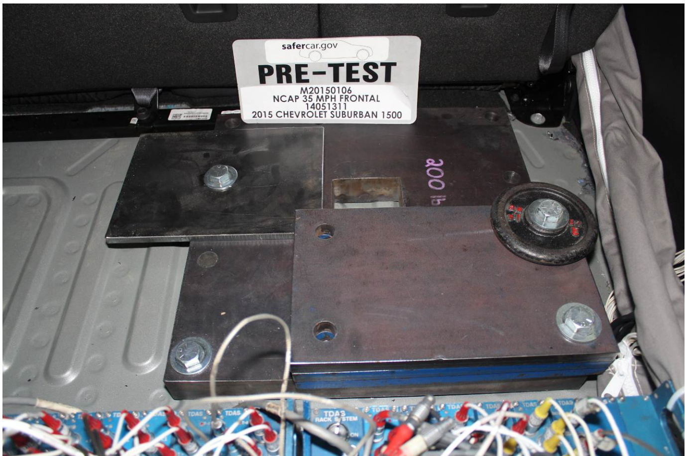
Ballast Installed in Vehicle
