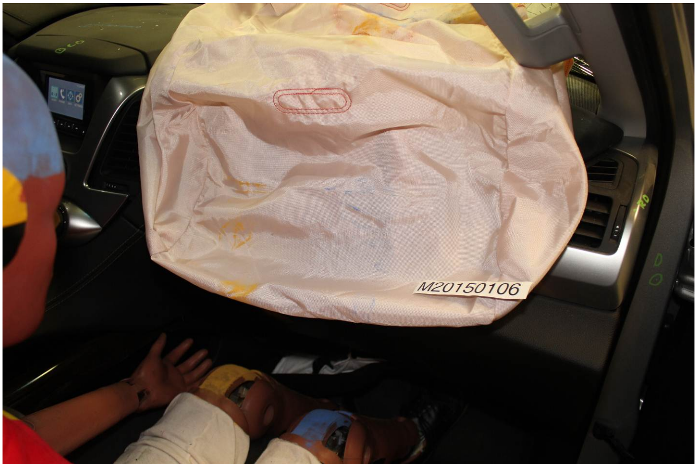
Post-Test Passenger Dummy Contact with Frontal Airbag
