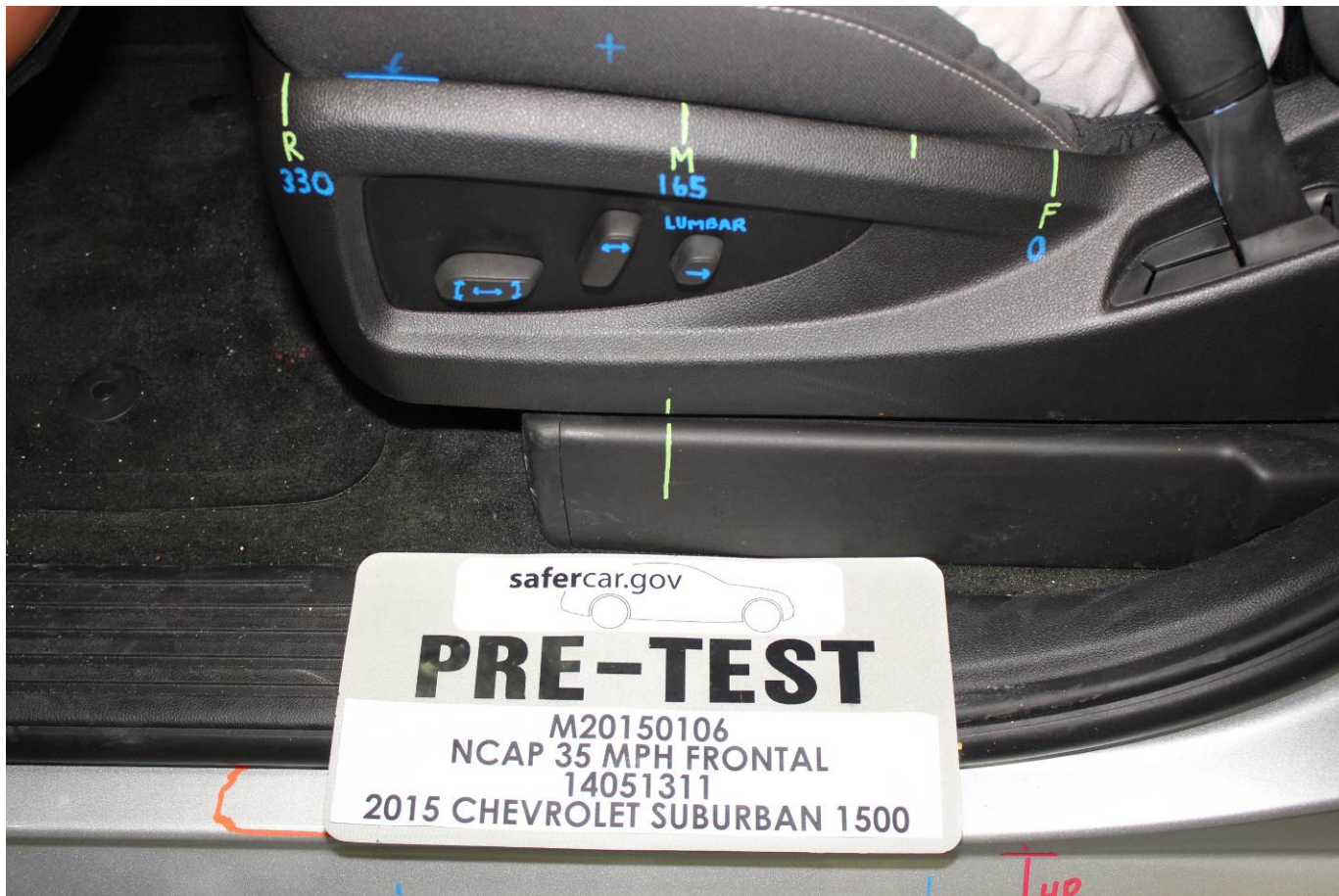
Pre-Test Driver's Seat Fore-Aft Markings
