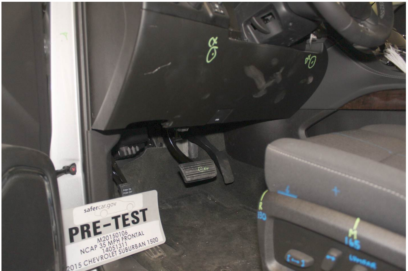
Pre-Test Driver's Side Knee Bolster (without dummy)
