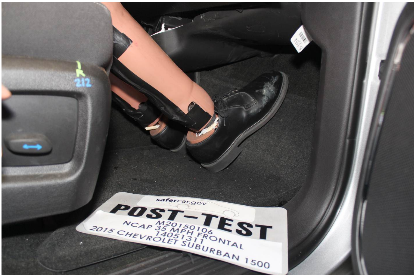
Post-Test Passenger Dummy Feet
