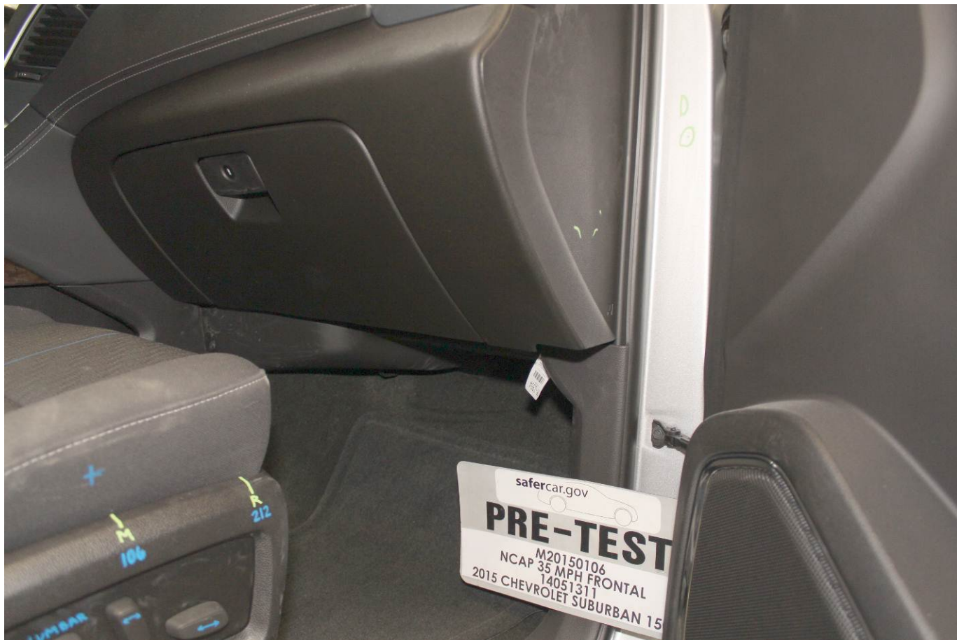
Pre-Test Passenger's Side Knee Bolster (without dummy)
