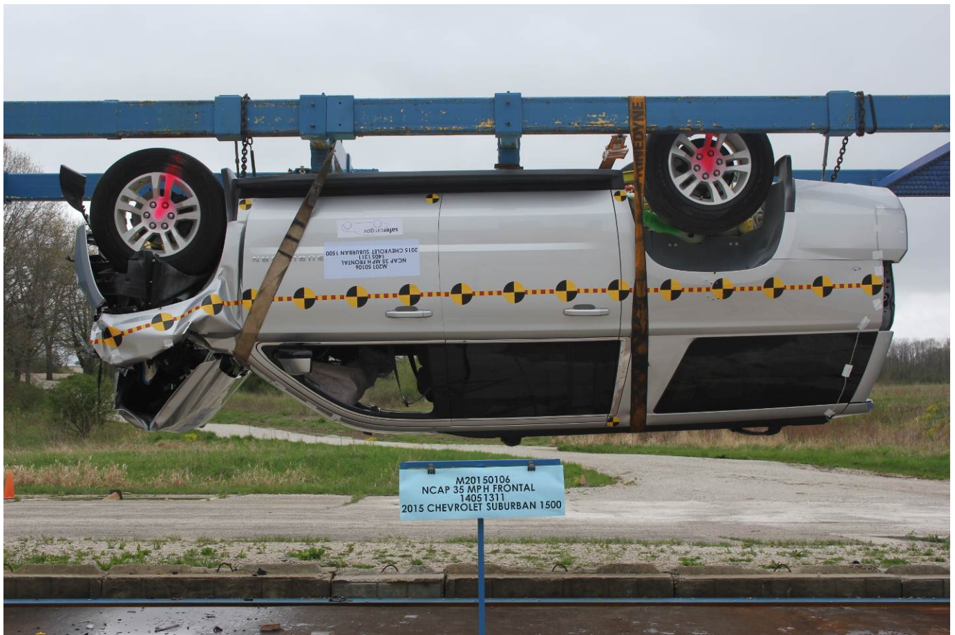
Vehicle at 180 Degrees on Static Rollover Device
