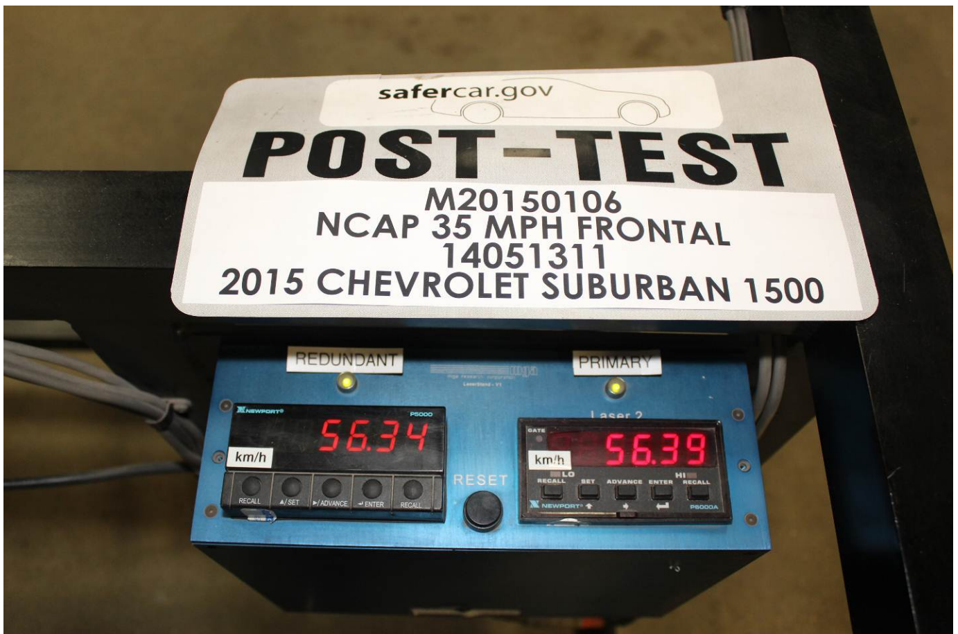
Post-Test Speed Trap Read-Out
