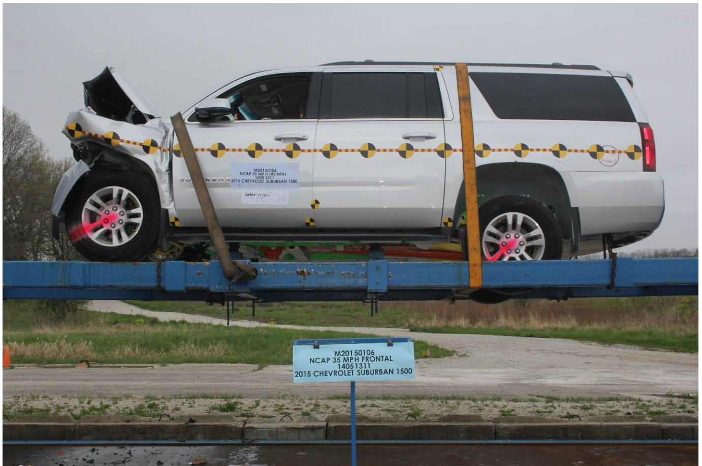
Vehicle at 360 Degrees on Static Rollover Device
