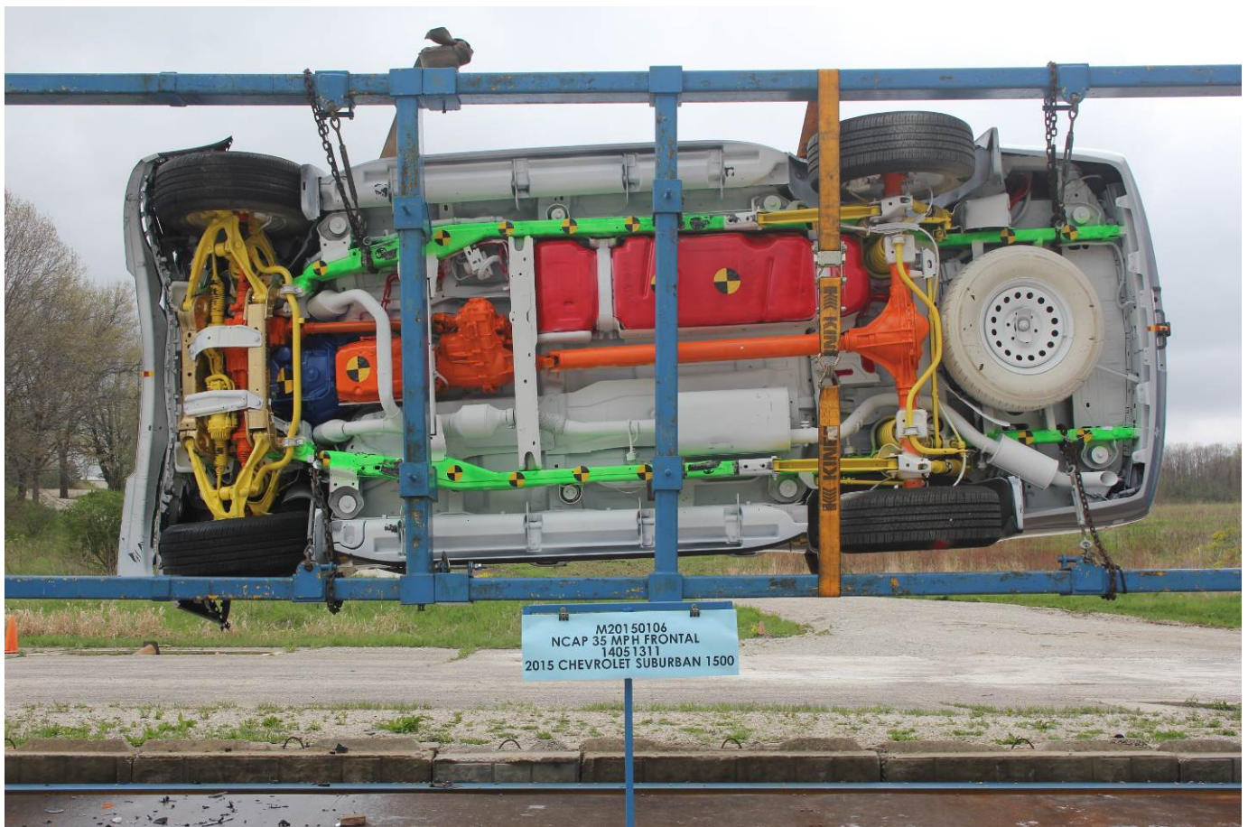
Vehicle at 270 Degrees on Static Rollover Device
