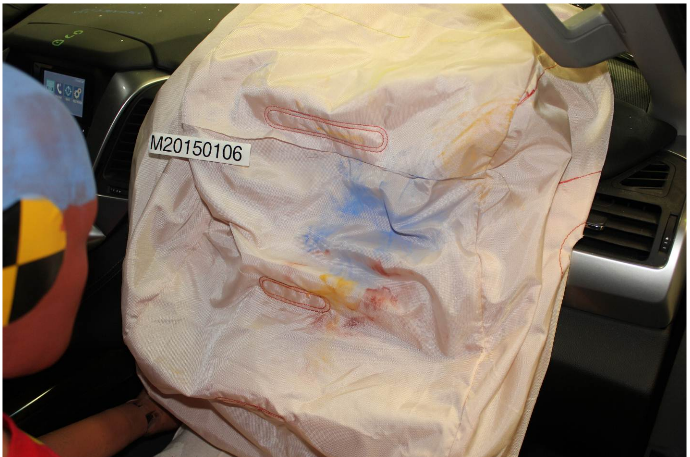
Post-Test Passenger Dummy Contact with Airbag
