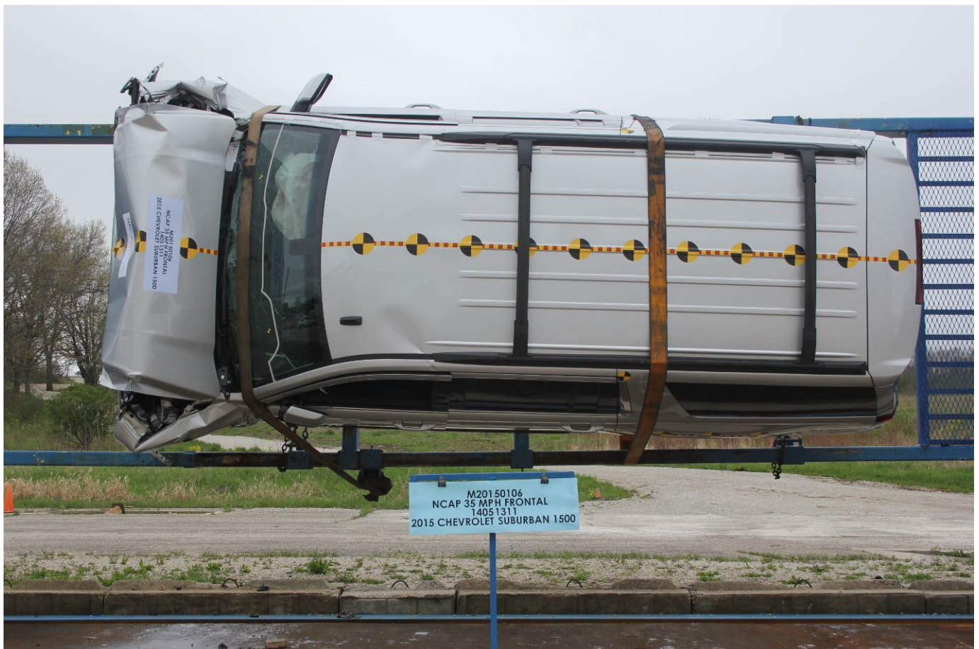
Vehicle at 90 Degrees on Static Rollover Device
