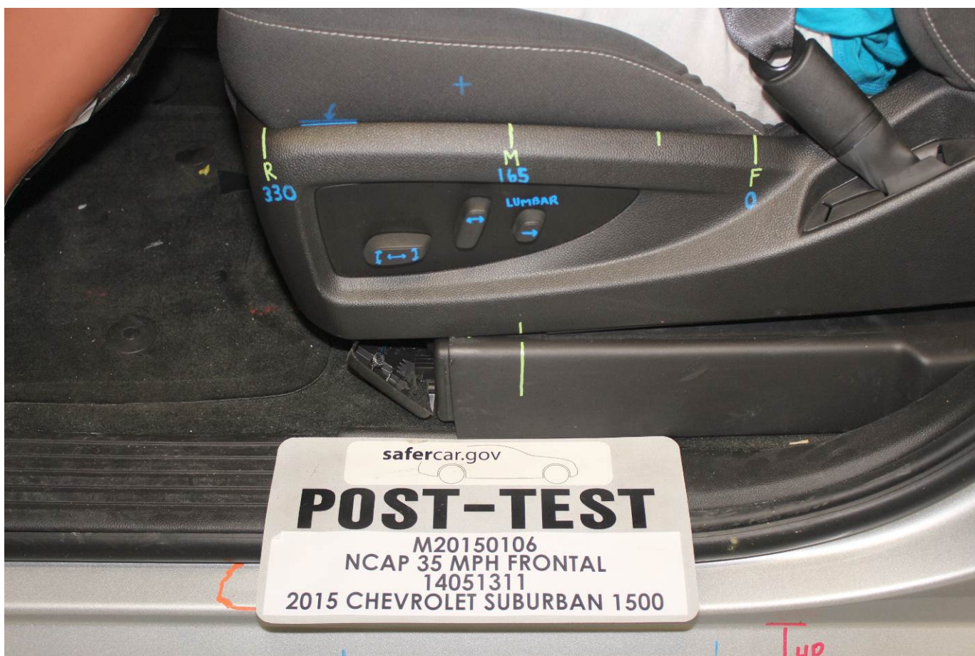
Post-Test Driver's Seat Fore-Aft Markings
