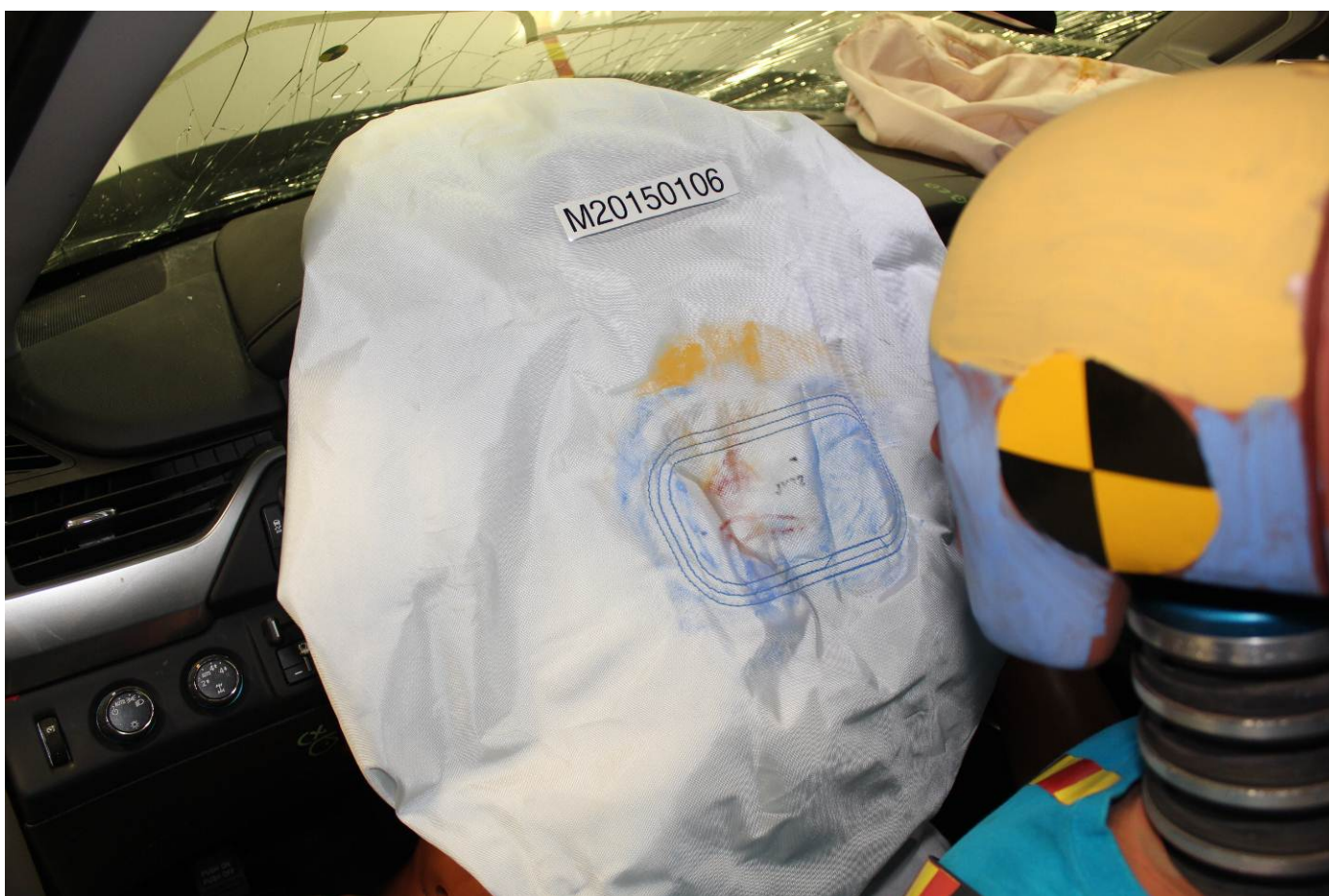
Post-Test Driver Dummy Contact with Airbag
