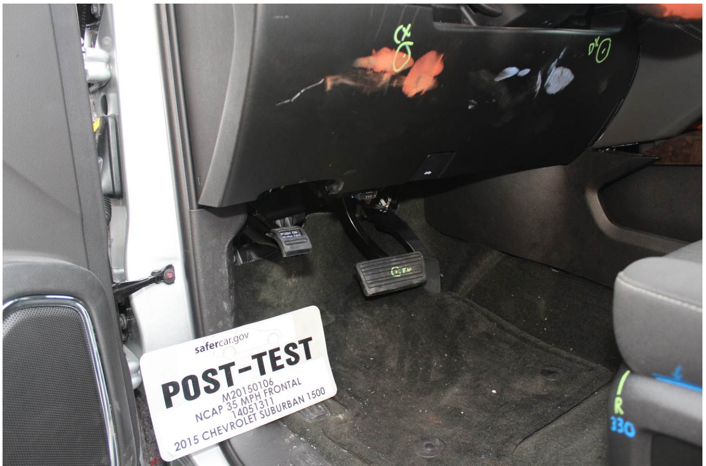
Post-Test Driver's Side Knee Bolster (without dummy)
