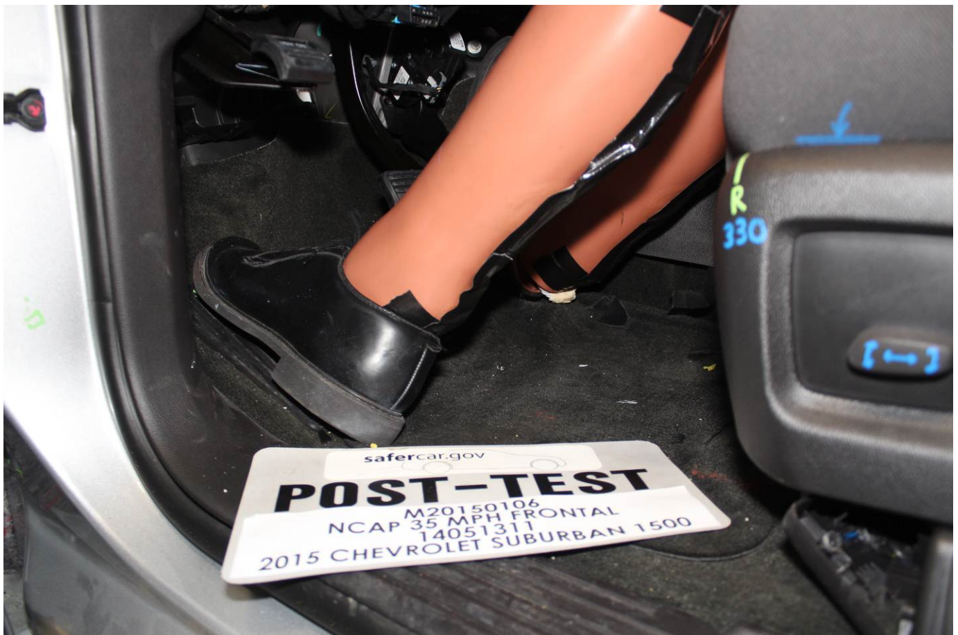
Post-Test Driver Dummy Feet
