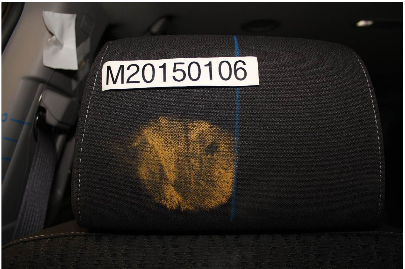
Post-Test Passenger Dummy Contact with Headrest
