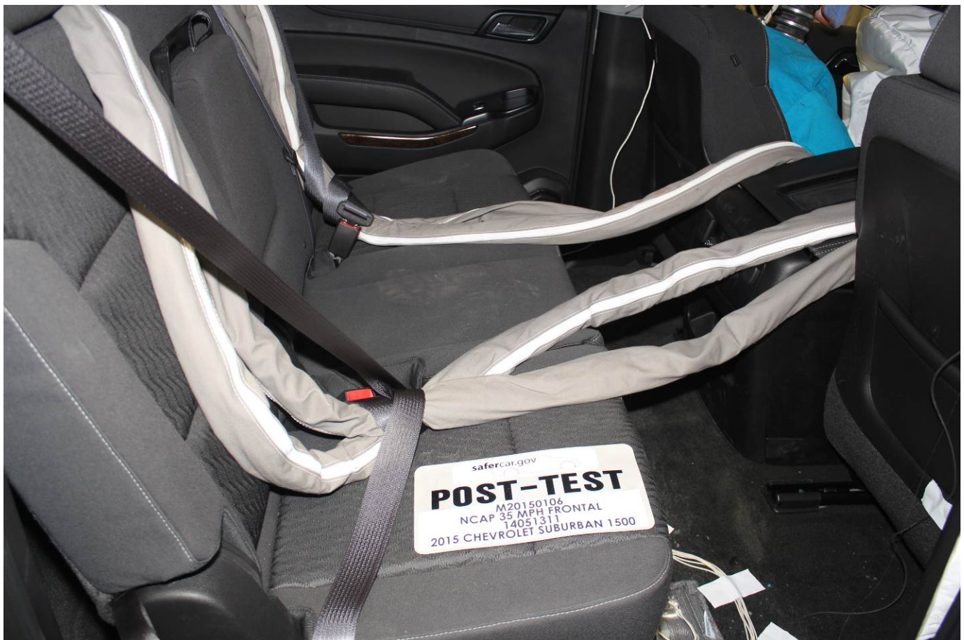
Post-Test Dummy Cable Routing
