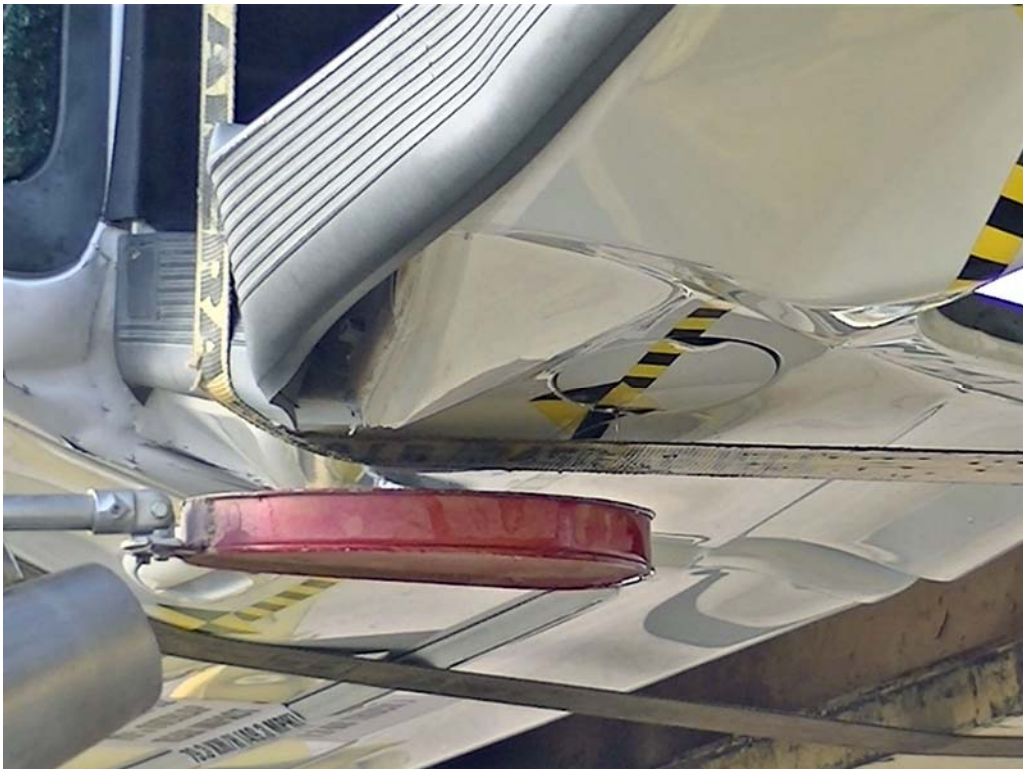
FIGURE 30. Post-Test Stoddard Solvent Spillage Location View
