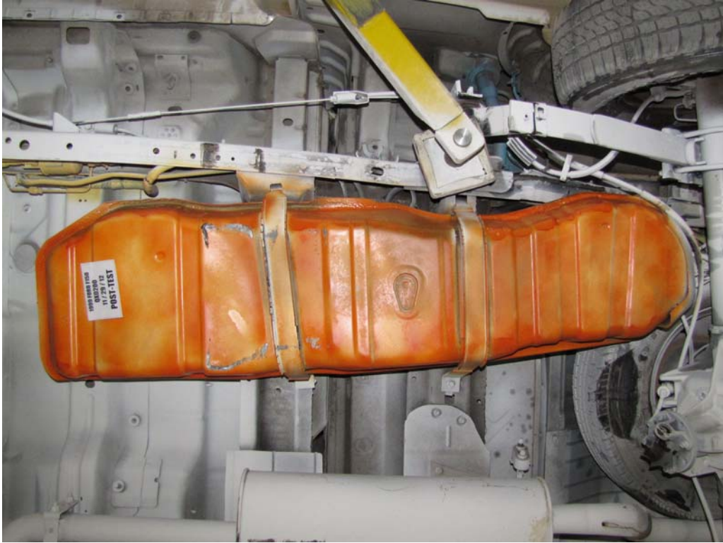
FIGURE 31. Post-Test Stoddard Solvent Spillage Location View
