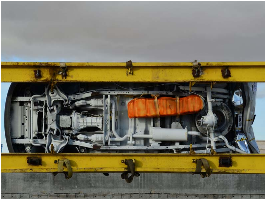
FIGURE 28. Vehicle at 270° on Static Rollover Device
