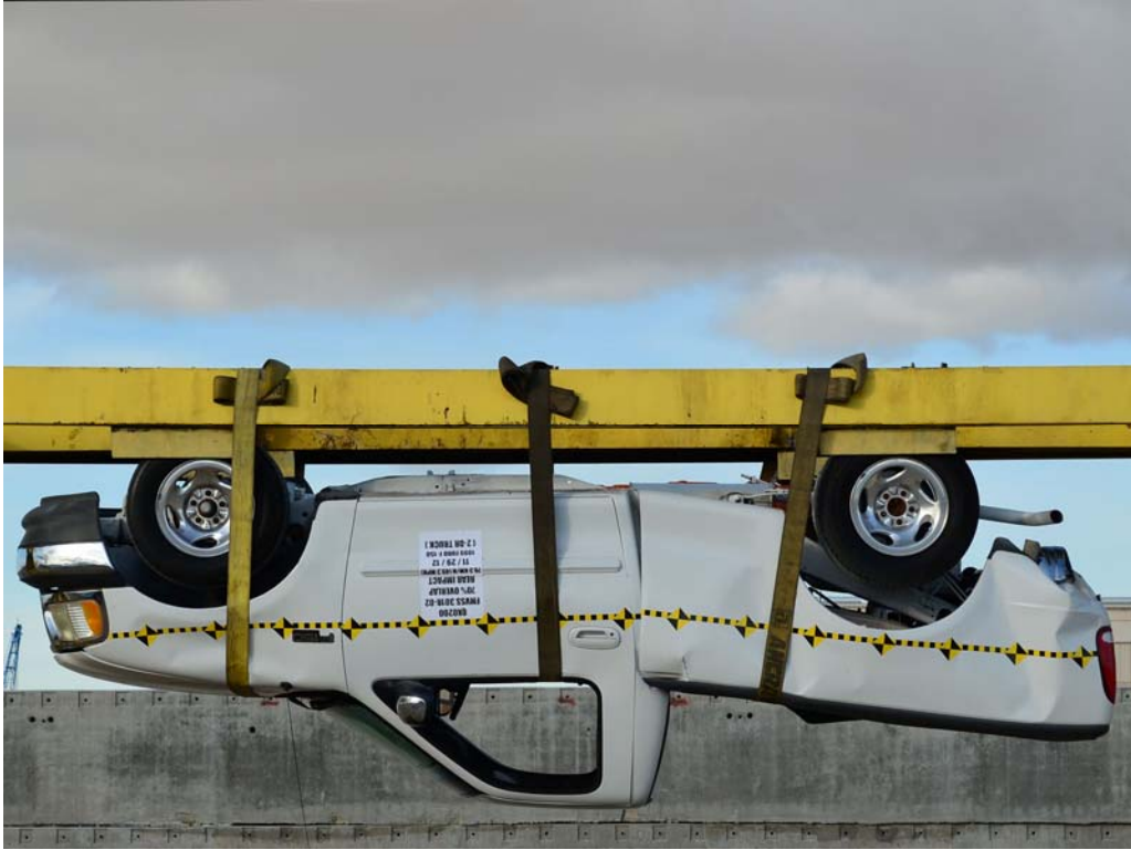
FIGURE 27. Vehicle at 180° on Static Rollover Device
