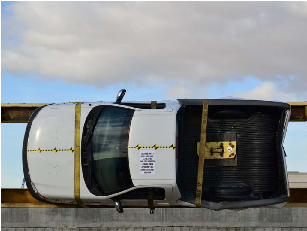
FIGURE 26. Vehicle at 90° on Static Rollover Device
