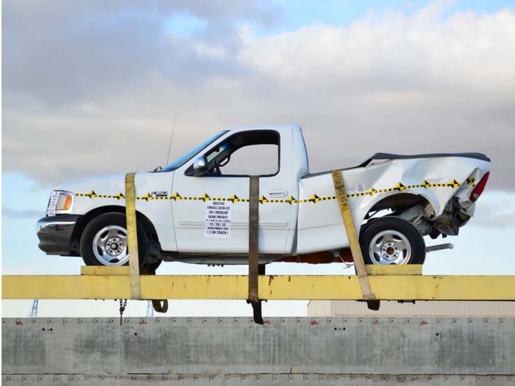
FIGURE 29. Vehicle at 360° on Static Rollover Device
