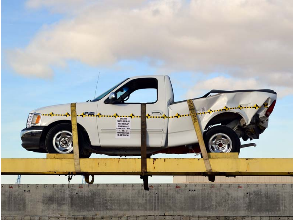
FIGURE 25. Vehicle at 0° on Static Rollover Device
