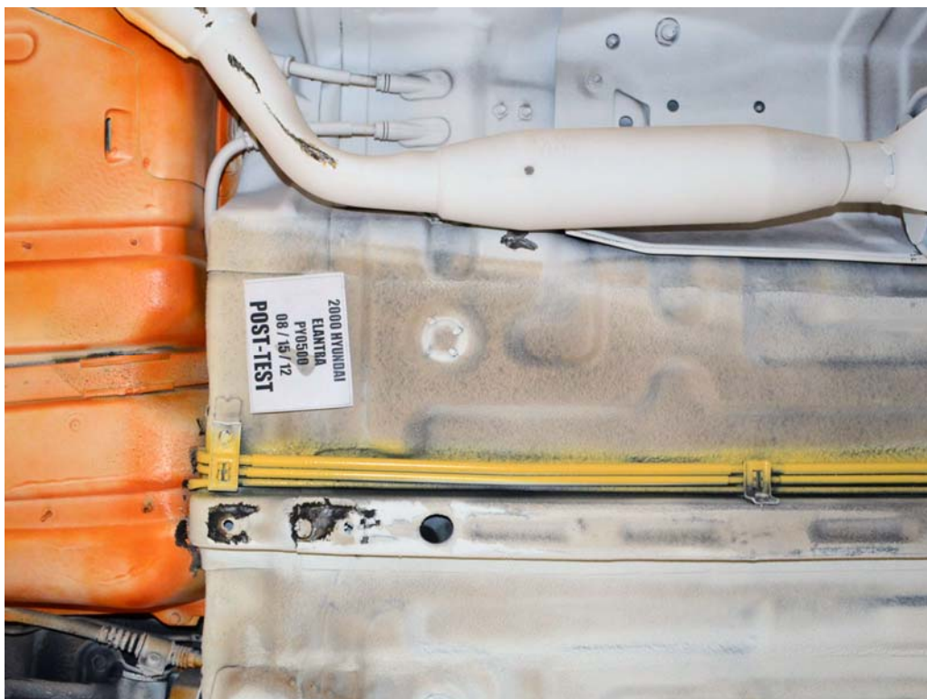
FIGURE 24. Post-Test Underbody, Fuel Line Location
