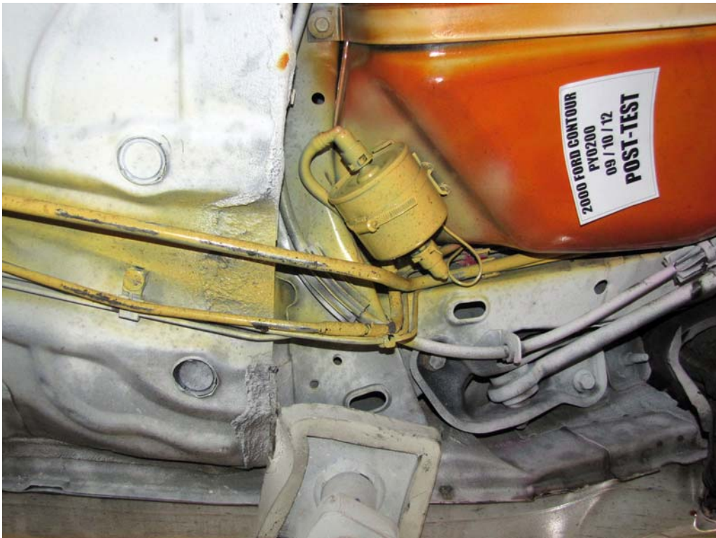
FIGURE 24. Post-Test Underbody, Fuel Line Location
