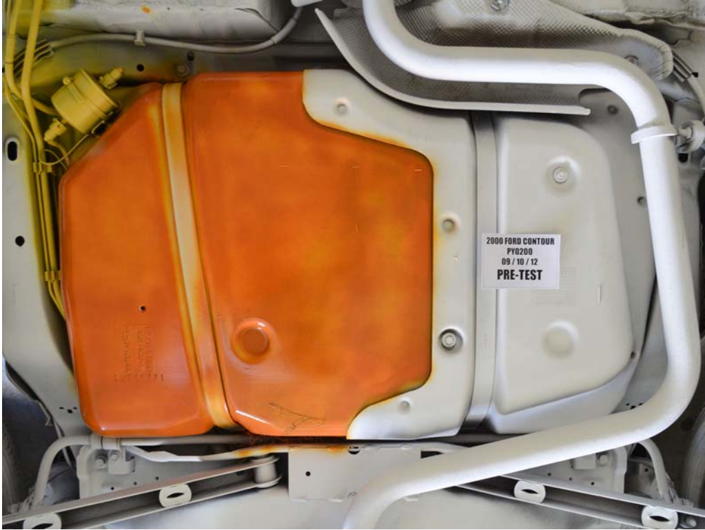
FIGURE 19. Pre-Test Underbody, Fuel Tank Location
