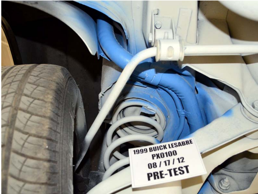
FIGURE 21. Pre-Test Underbody, Fuel Filler Neck Location
