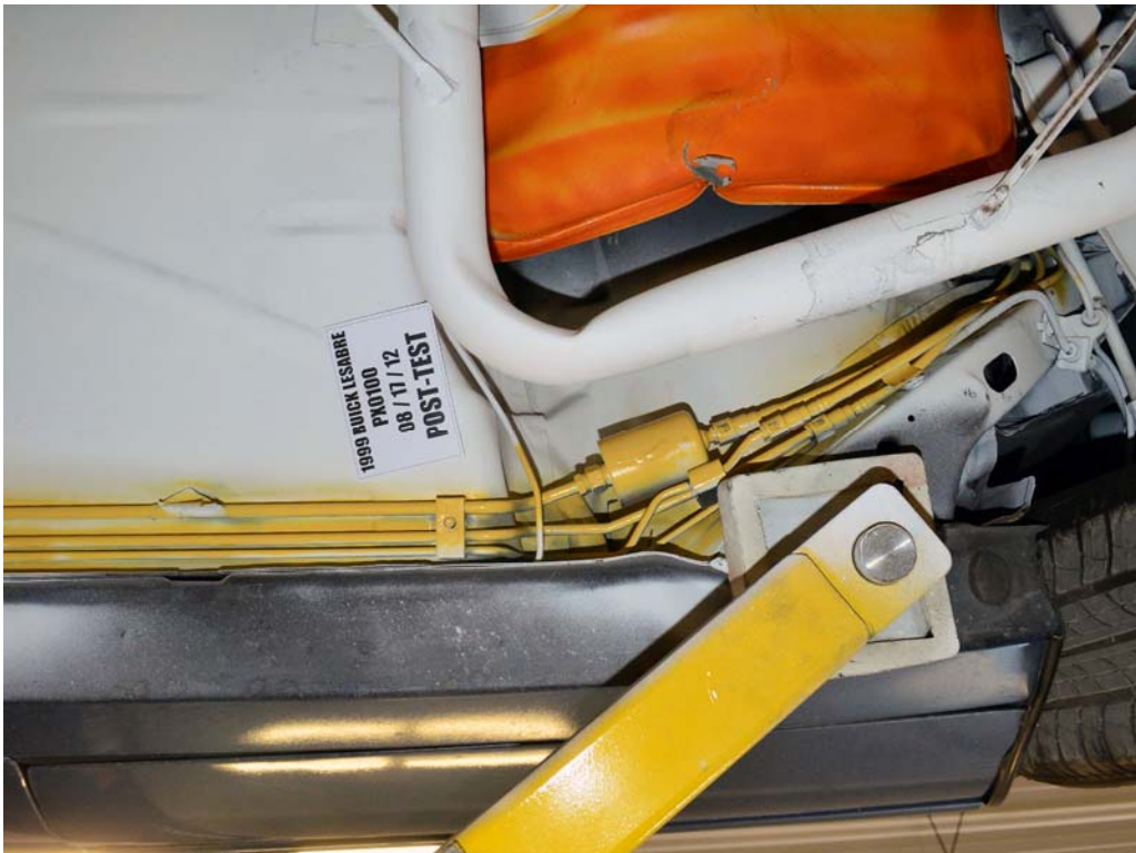
FIGURE 24. Post-Test Underbody, Fuel Line Location
