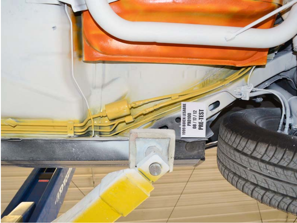
FIGURE 23. Pre-Test Underbody, Fuel Line Location
