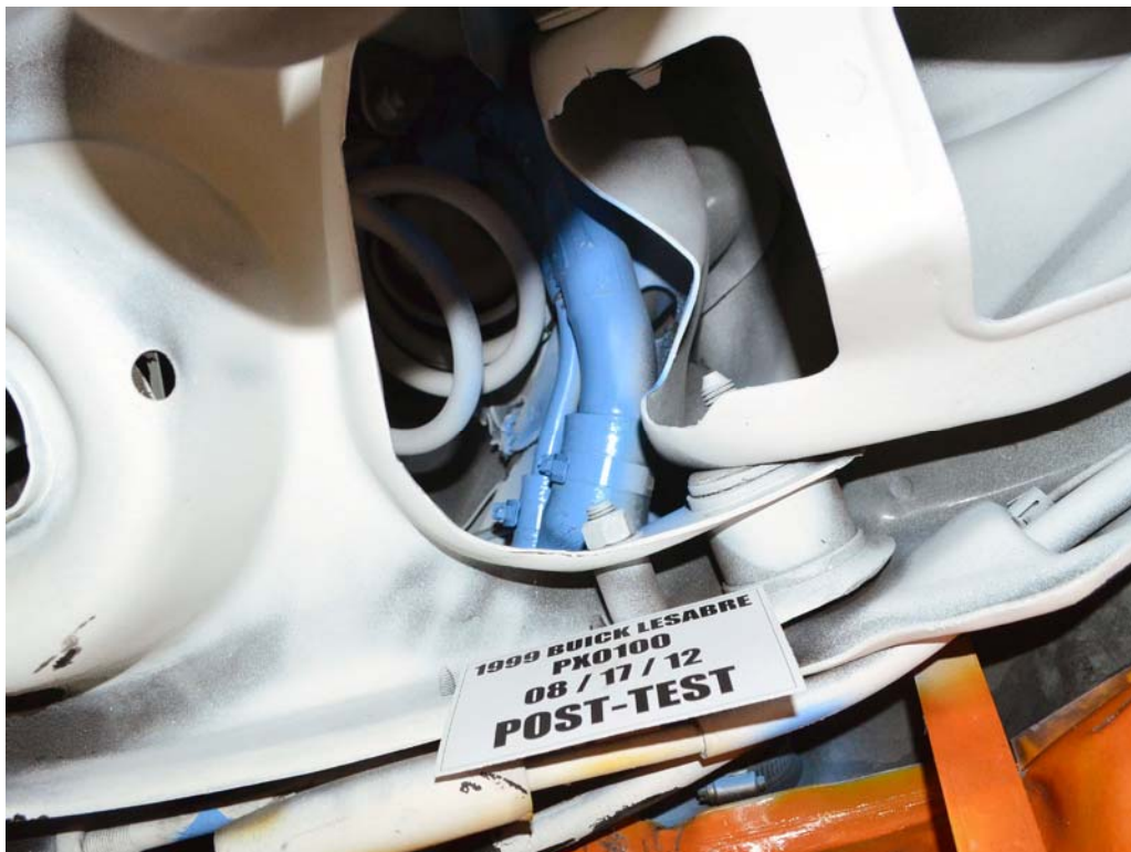
FIGURE 22. Post-Test Underbody, Fuel Filler Neck Location
