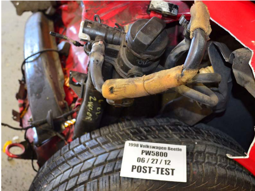
FIGURE 37. Post-Test Stoddard Solvent Spillage Location View
