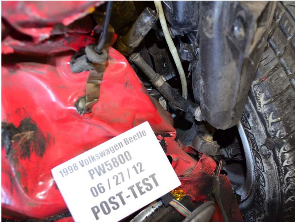
FIGURE 33. Post-Test Stoddard Solvent Spillage Location View
