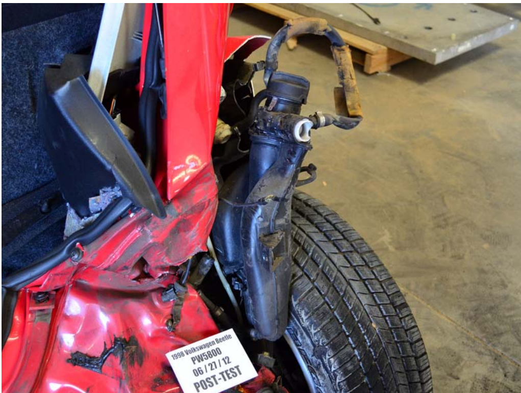
FIGURE 30. Post-Test Stoddard Solvent Spillage Location View
