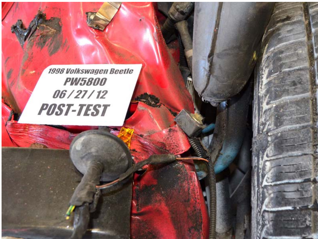
FIGURE 34. Post-Test Stoddard Solvent Spillage Location View
