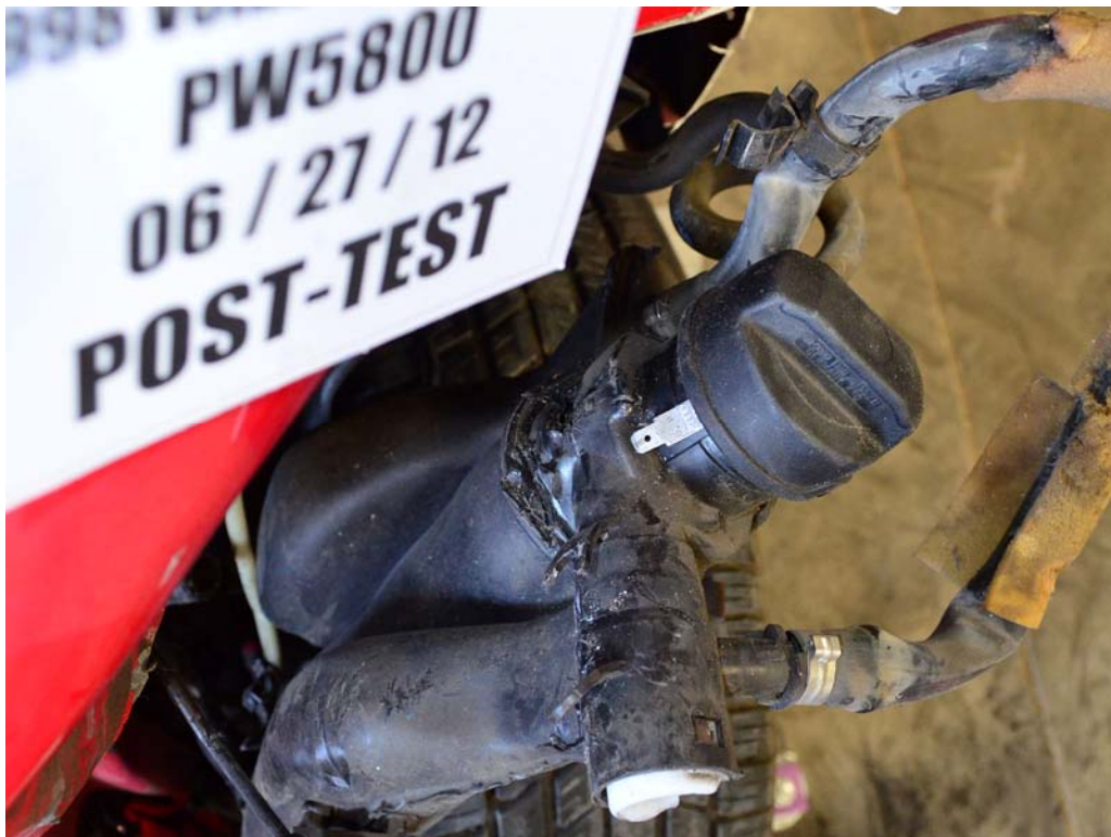
FIGURE 32. Post-Test Stoddard Solvent Spillage Location View
