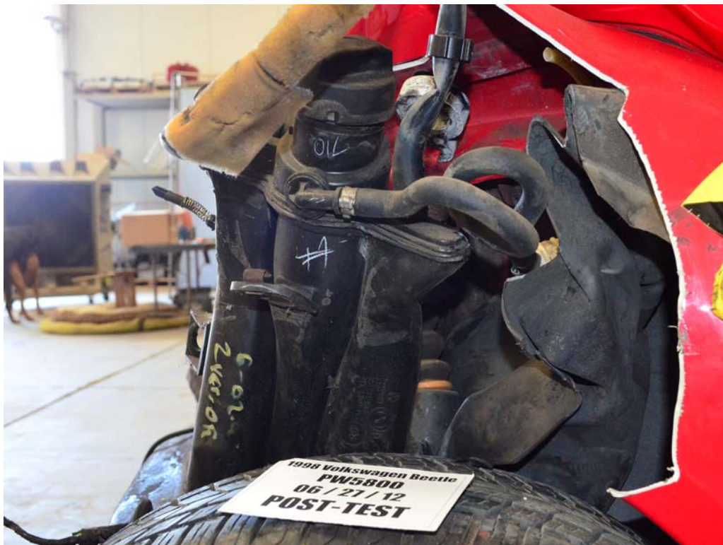
FIGURE 38. Post-Test Stoddard Solvent Spillage Location View
