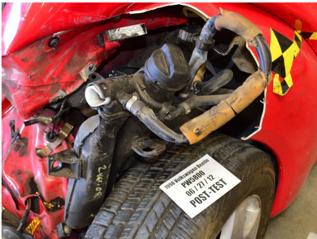
FIGURE 36. Post-Test Stoddard Solvent Spillage Location View
