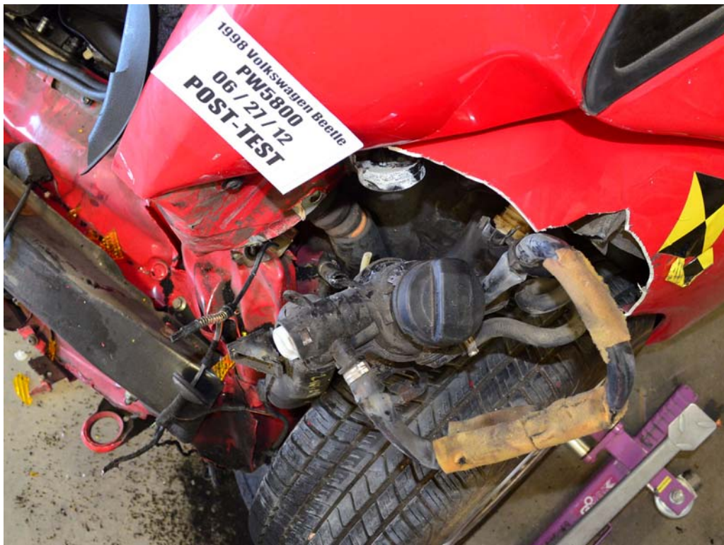
FIGURE 35. Post-Test Stoddard Solvent Spillage Location View
