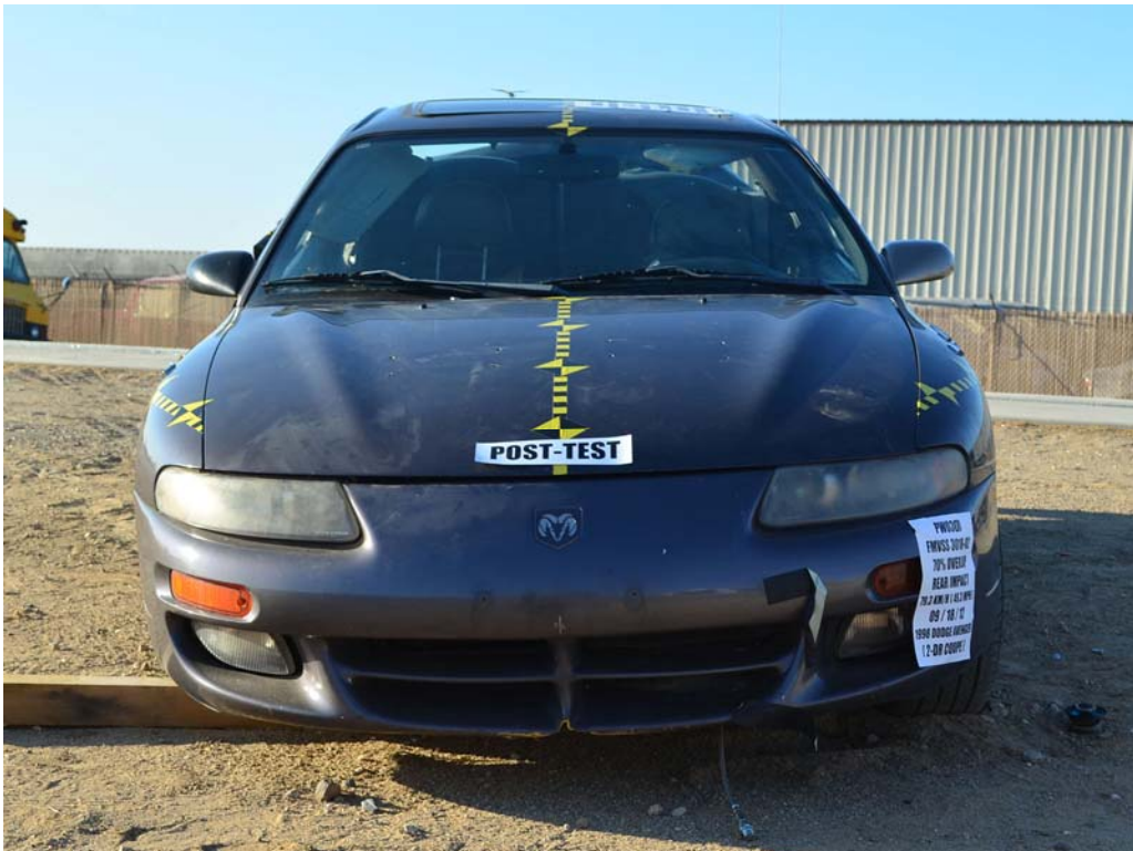
FIGURE 4. Post-Test Front of Test Vehicle
