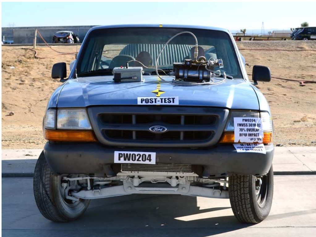
FIGURE 4. Post-Test Front of Test Vehicle
