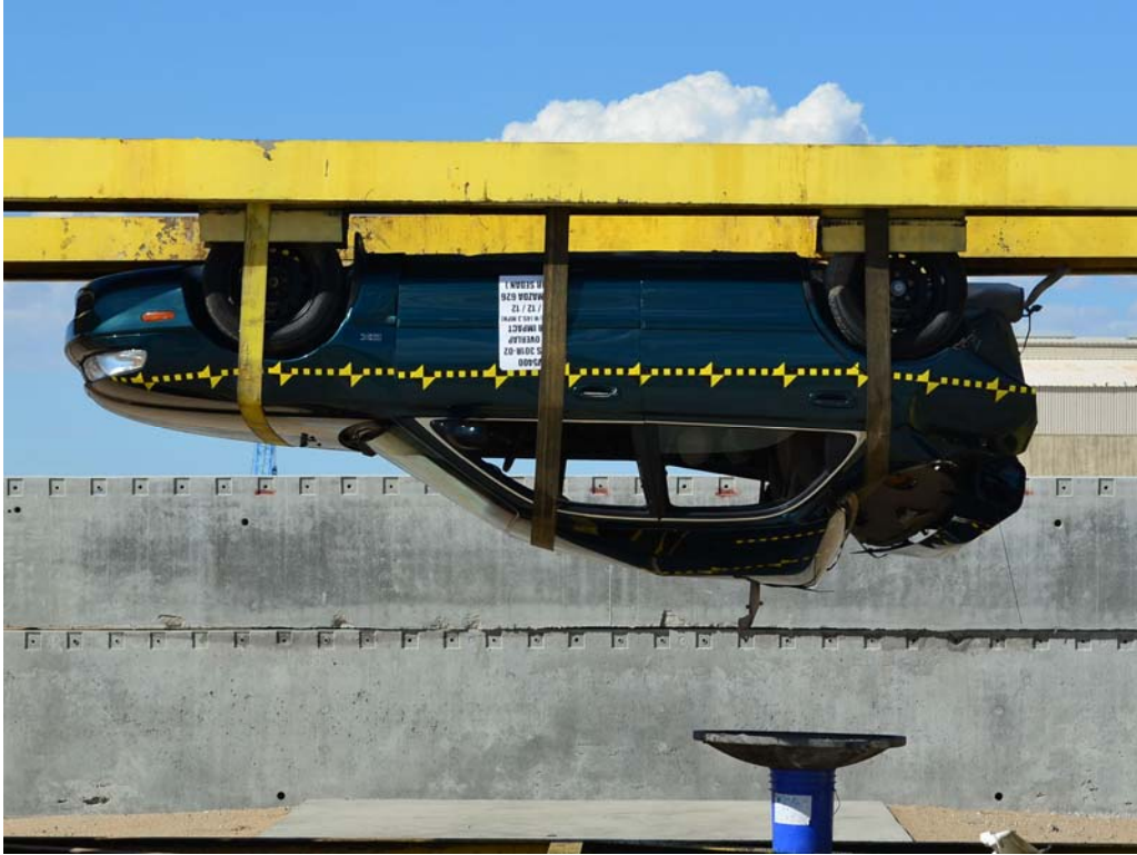
FIGURE 27. Vehicle at 180° on Static Rollover Device
