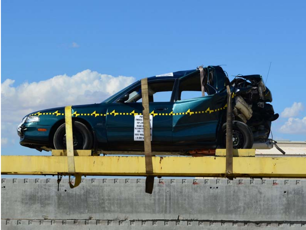
FIGURE 29. Vehicle at 360° on Static Rollover Device
