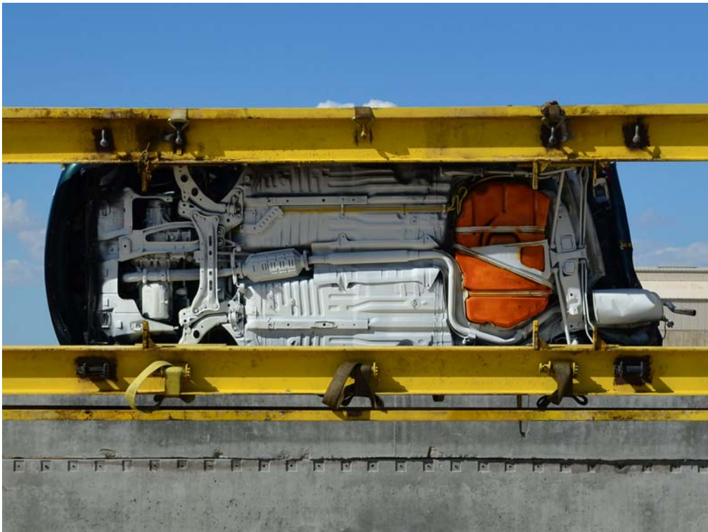
FIGURE 28. Vehicle at 270° on Static Rollover Device
