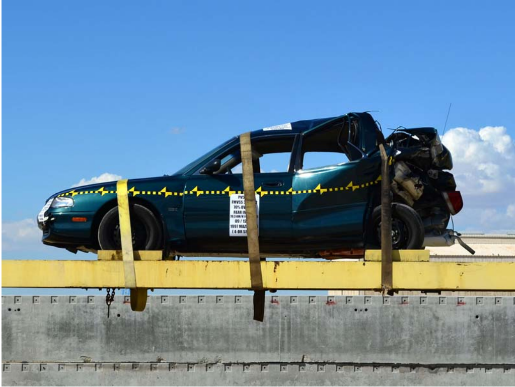
FIGURE 25. Vehicle at 0° on Static Rollover Device
