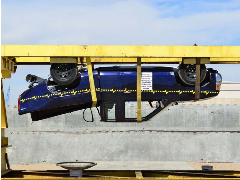
FIGURE 27. Vehicle at 180° on Static Rollover Device
