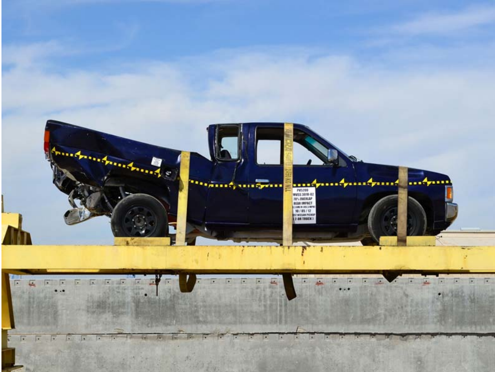
FIGURE 29. Vehicle at 360° on Static Rollover Device
