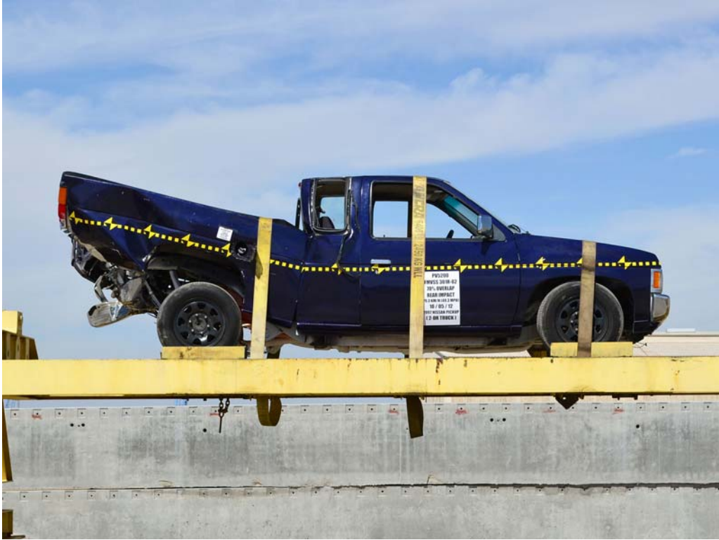
FIGURE 25. Vehicle at 0° on Static Rollover Device
