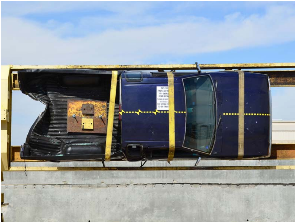
FIGURE 26. Vehicle at 90° on Static Rollover Device
