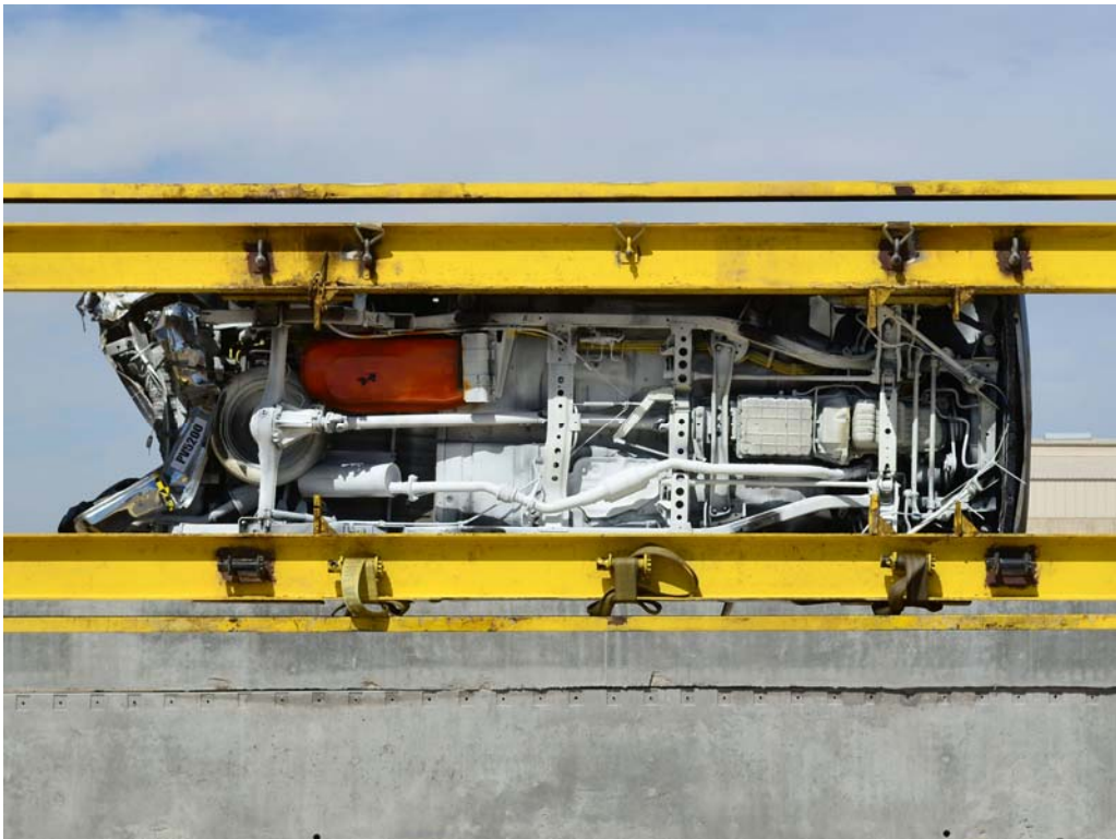
FIGURE 28. Vehicle at 270° on Static Rollover Device
