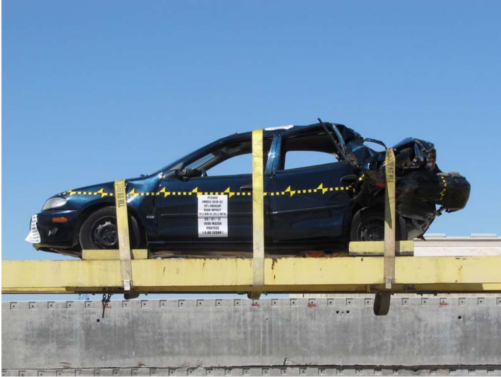
FIGURE 29. Vehicle at 360° on Static Rollover Device
