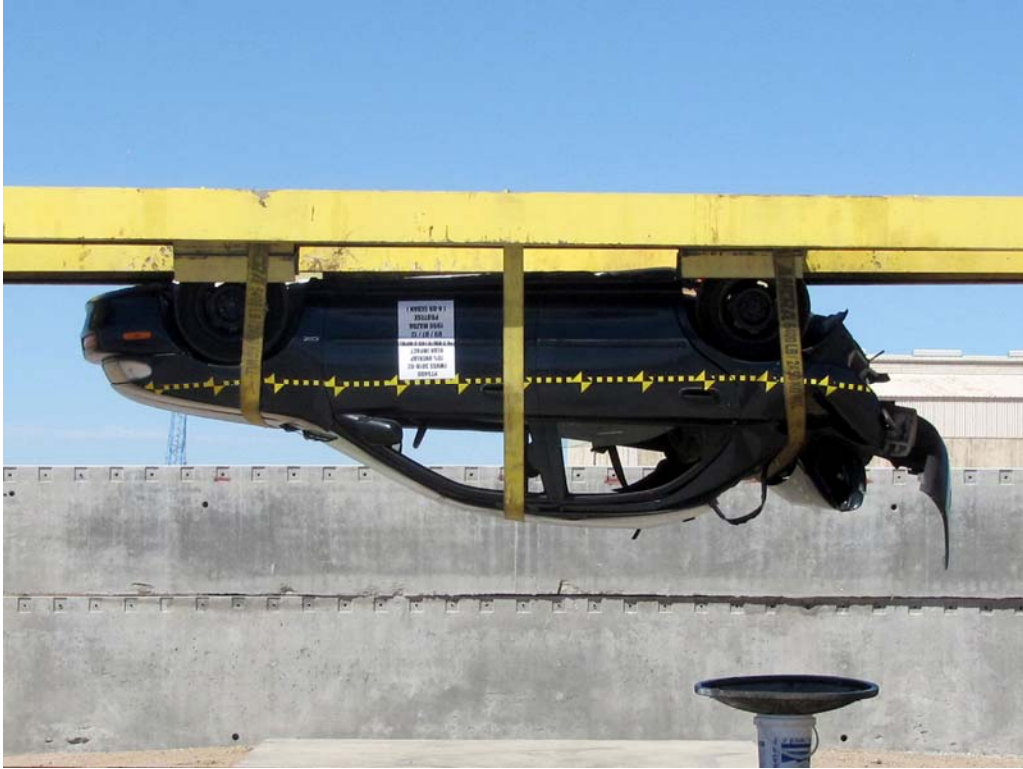
FIGURE 27. Vehicle at 180° on Static Rollover Device
