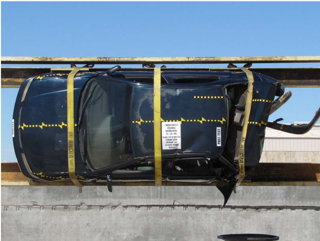
FIGURE 26. Vehicle at 90° on Static Rollover Device
