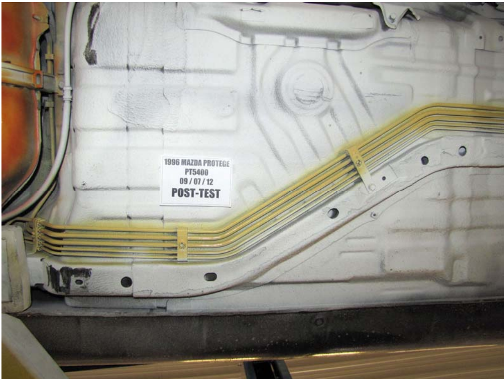
FIGURE 24. Post-Test Underbody, Fuel Line Location
