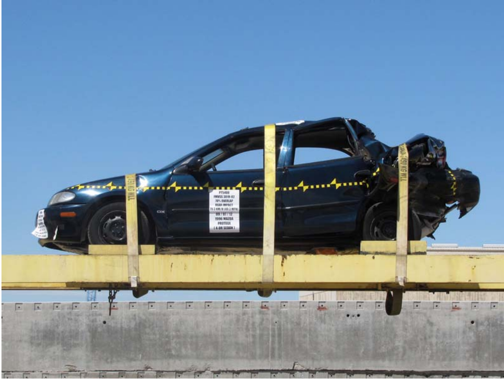
FIGURE 25. Vehicle at 0° on Static Rollover Device
