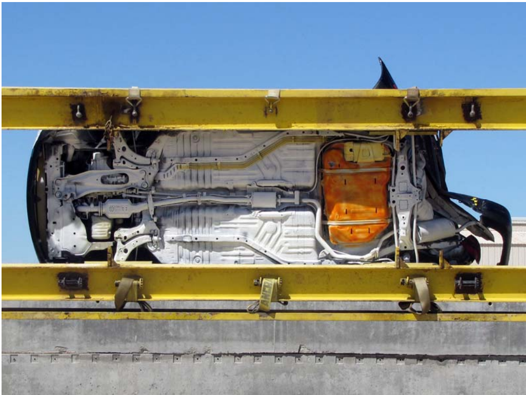
FIGURE 28. Vehicle at 270° on Static Rollover Device
