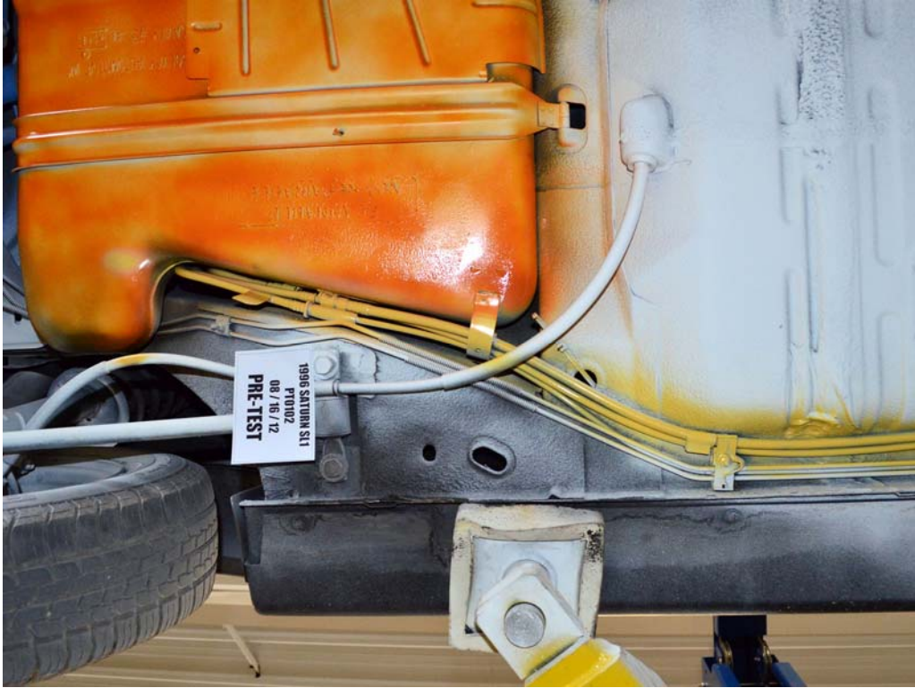
FIGURE 23. Pre-Test Underbody, Fuel Line Location
