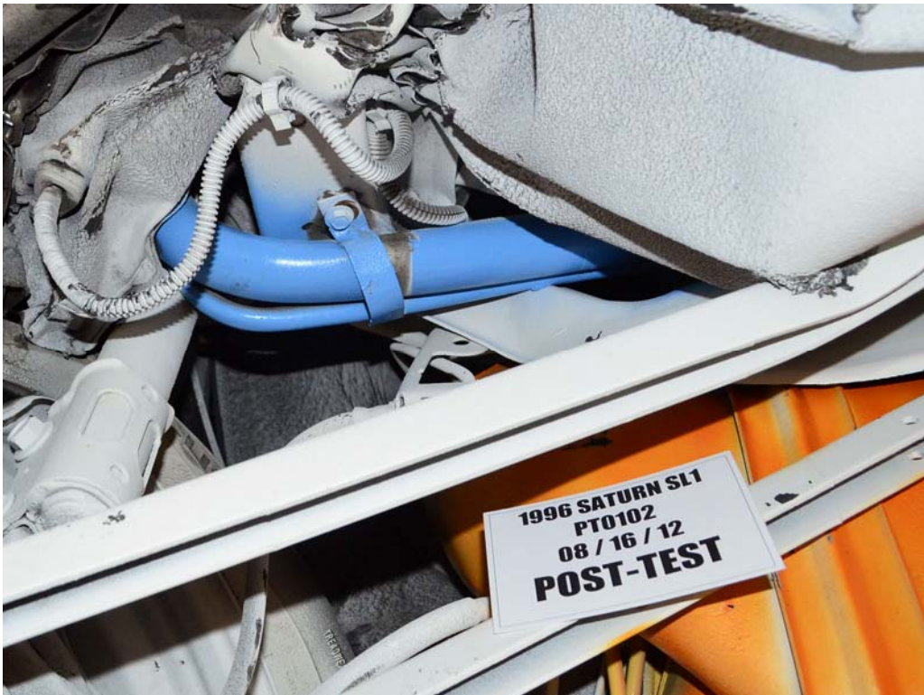
FIGURE 22. Post-Test Underbody, Fuel Filler Neck Location
