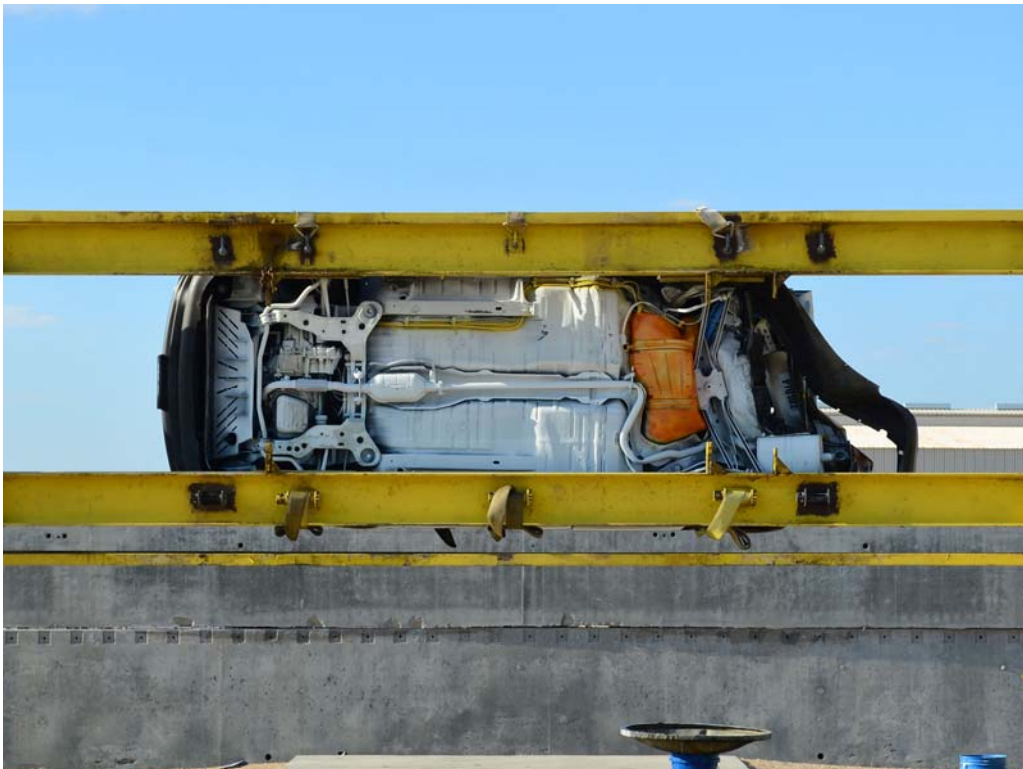
FIGURE 28. Vehicle at 270° on Static Rollover Device
