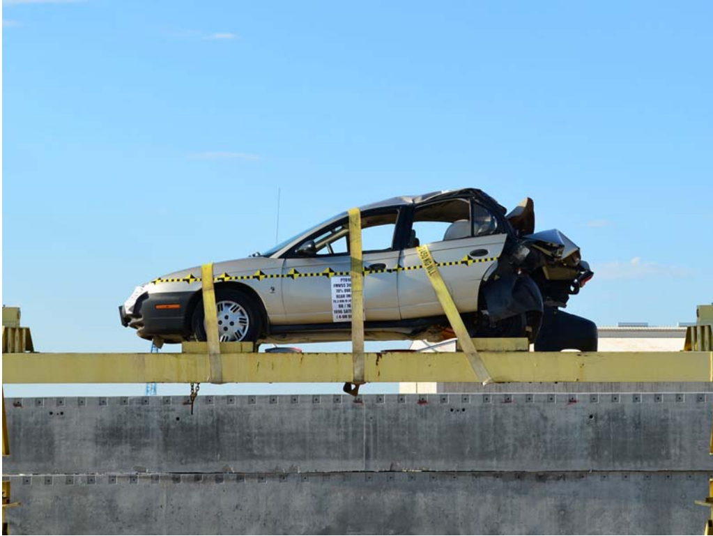
FIGURE 29. Vehicle at 360° on Static Rollover Device
