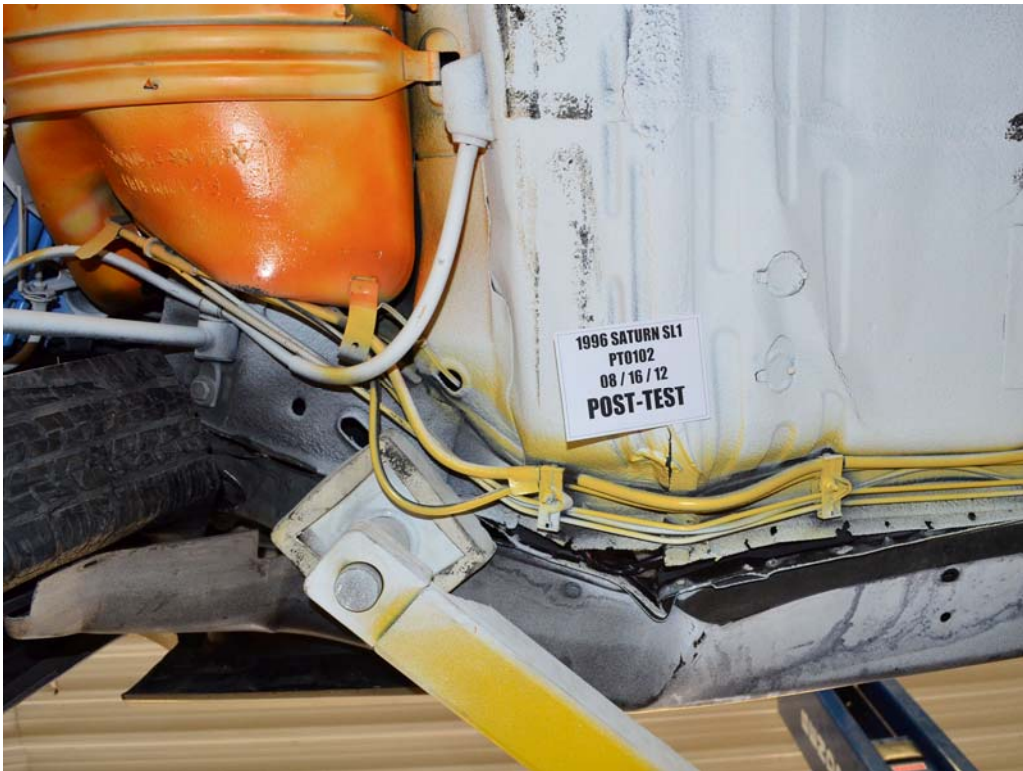
FIGURE 24. Post-Test Underbody, Fuel Line Location
