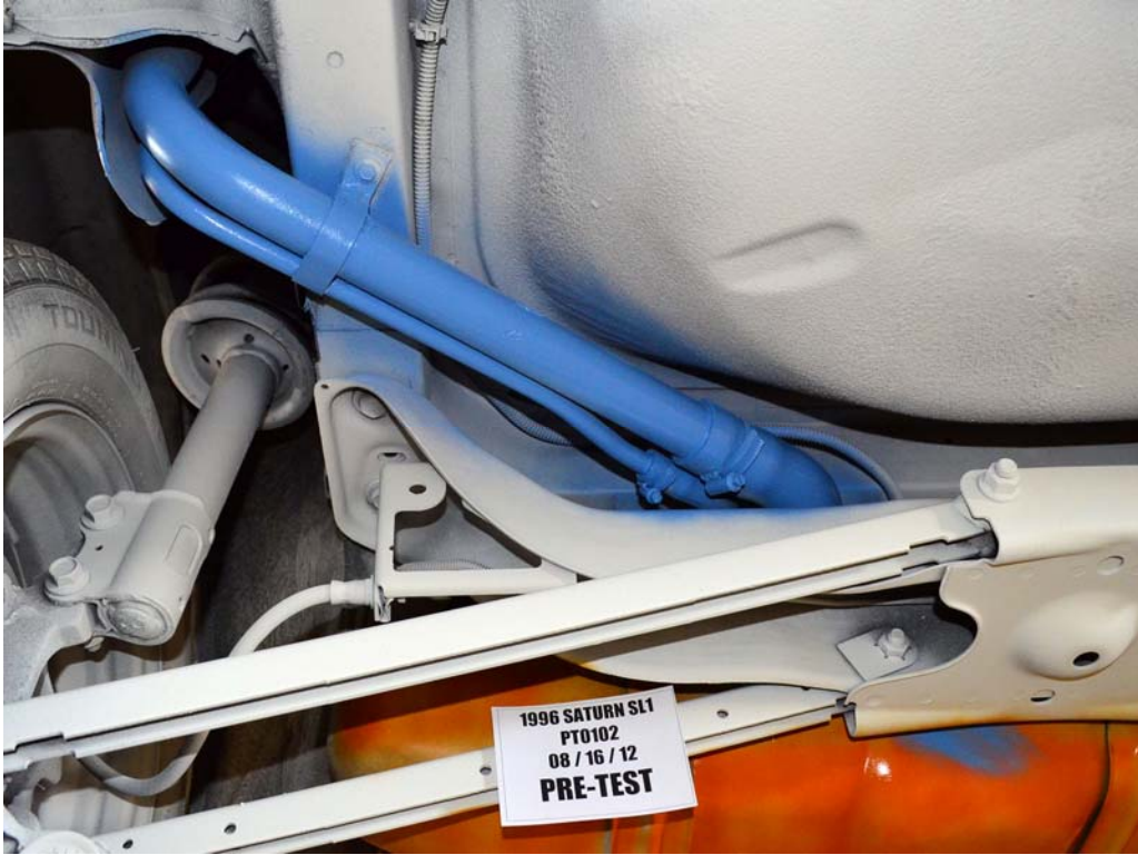
FIGURE 21. Pre-Test Underbody, Fuel Filler Neck Location
