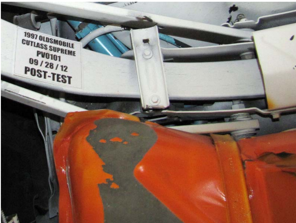
FIGURE 30. Post-Test Stoddard Solvent Spillage Location View
