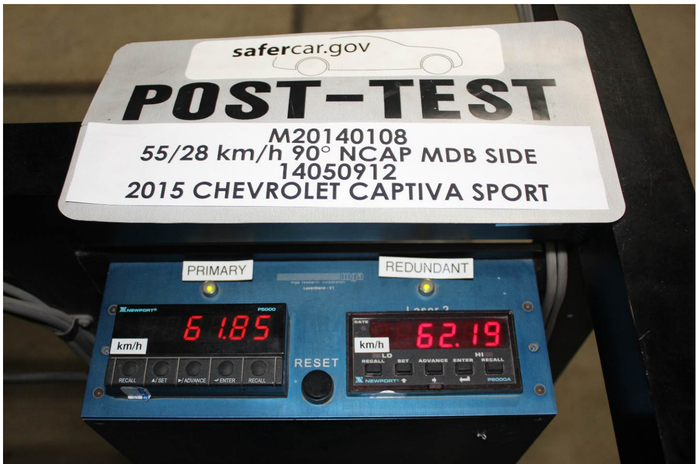
Post-Test Primary and Redundant Speed Trap Read-Out
