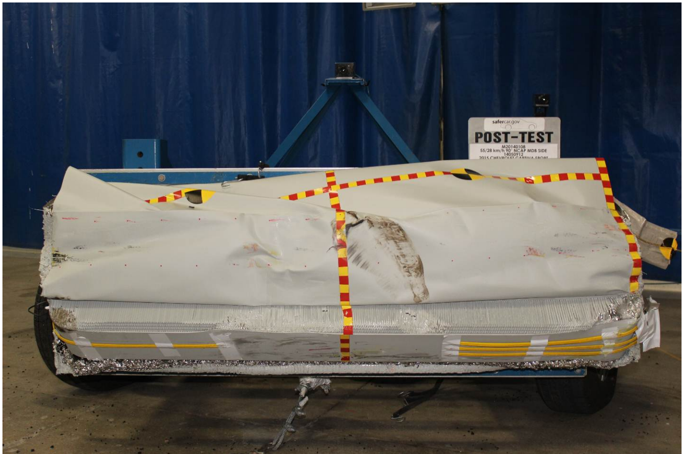
Post-Test Front View of MDB Impactor Face
